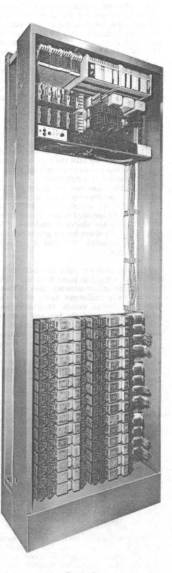
Figure 8 ORIGINATING JUNCTOR FRAME
