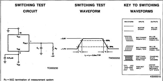
C<sub>L</sub> = 30pF (including stray jig capacitance)
