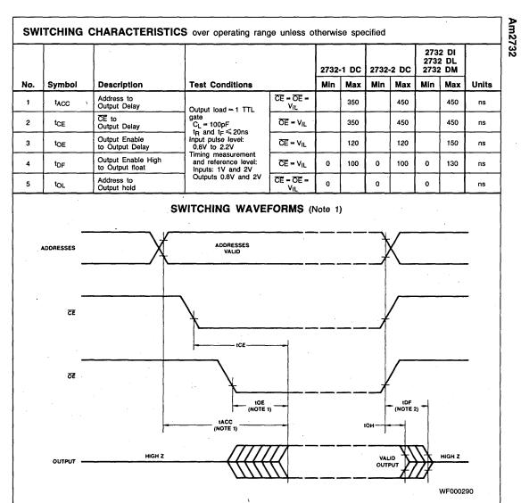
Notes: 1. OE may be delayed up to 330ns after the falling edge of CE without impact on t<sub>ACC</sub> 2. t<sub>DF</sub> is specified from OE or CE, whichever occurs first.
