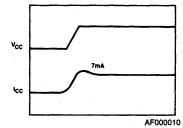
Figure 2. V<sub>CC</sub> Supply Current Waveform during V<sub>CC</sub> Power Up,  $\overline{RAS} = \overline{CAS} = V_{SS}$
