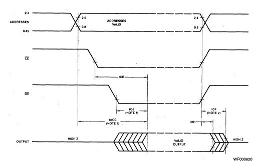
Notes: 1. OE may be delayed up to t<sub>ACC</sub>-t<sub>OE</sub> after the falling edge of CE without impact on t<sub>ACC</sub>. 2. t<sub>DF</sub> is specified from OE or CE, whichever occurs first. **Am27512** 65,536 x 8-Bit UV Erasable PROM
