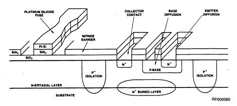
Figure 2. Transistor & Fuse Structures.
