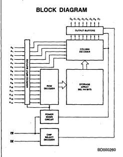
This memory is fully static and requires no clock signals of any kind. A selected chip will output data from a location specified by the address present on the address input lines. Input and output levels are compatible with TTL specifications. A separate  $\overrightarrow{OE}$ , output enable pin, controls outputs providing greater system flexibility and eliminating bus contention.
