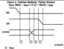
2 t<sub>T</sub> + skew (address input A<sub>0</sub>-A<sub>7</sub> relative to RAS)
