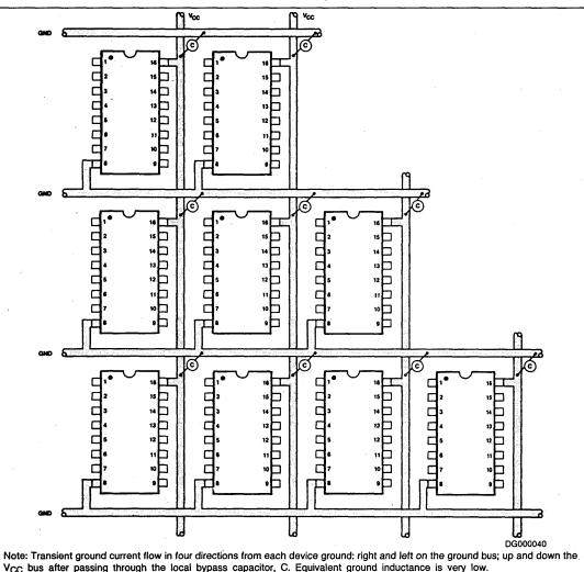
g through the local bypass capacitor, C. Equivalent ground induc
