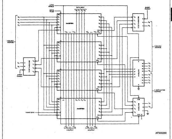
A 64-word by 4-bit three address memory. Data is read from the A address to the YA outputs and from the B address to the YB outputs while the latch enable is HIGH. When the latch enable goes LOW, the YA and YB data is held in the internal latches, and the RAM B address is switched to the Cdestination address lines. A write pulse will then deposit the input data into the location selected by the C address. Am29705A/707
