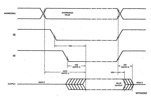
Notes: 1.  $\overline{\text{OE}}$  may be delayed up to  $t_{\text{ACC}}$ - $t_{\text{OE}}$  after the falling edge of  $\overline{\text{CE}}$  without impact on  $t_{\text{ACC}}$ . 2.  $t_{\text{DF}}$  is specified from  $\overline{\text{OE}}$  or  $\overline{\text{CE}}$ , whichever occurs first.
