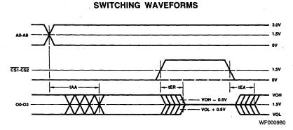
Note: Level on output while either CS is HIGH is determined externally.
