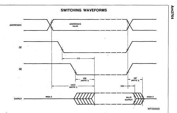
Notes: 1. OE may be delayed up to t<sub>ACC</sub>-t<sub>OE</sub> after the falling edge of  $\overline{CE}$  without impact on t<sub>ACC</sub>. 2. t<sub>DF</sub> is specified from  $\overline{OE}$  or  $\overline{CE}$ , whichever occurs first.
