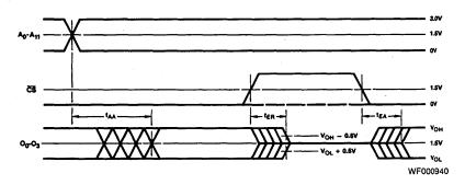
Note: Output level while  $\overline{CS}$  is HIGH is determined externally.
