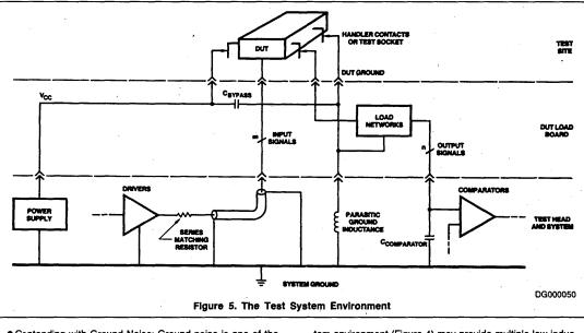
Contending with Ground Noise: Ground noise is one of the most common and troublesome test problems. As defined above, ground noise is caused by switching currents flowing through the ground network impedance. Whereas the system environment (Figure 4) may provide multiple low inductance ground paths into a ground mesh or plane, the tester provides one long, higher inductance path back to the test system ground (Figure 5). This path includes handler con-
