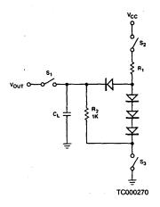
$$R_1 = \frac{5.0 - V_{BE} - V_{OL}}{I_{OL} + V_{OL}/1K}$$
