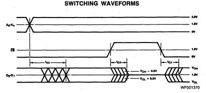
Note: Level on output while  $\overline{CS}$  is HIGH is determined externally.
