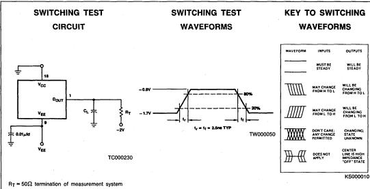
C<sub>L</sub> = 30pF (including stray jig capacitance)
