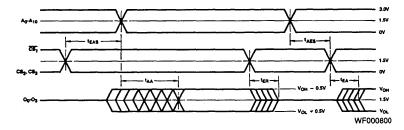
Note: Level on output while  $\overline{CS}_1$  is HIGH or CS<sub>2</sub> or CS<sub>3</sub> are LOW is determined externally.
