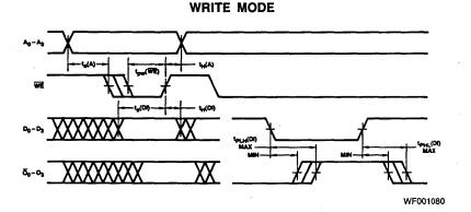
Write Cycle Timing. The cycle is initiated by an address change. After  $t_s(A)$  min, the write enable may begin. The chip select must also be LOW for writing. Following the write pulse,  $t_h(A)$  min must be allowed before the address may be changed again. The output will be inactive (floating for the Am54S/74S189) while the write enable is (WE) LOW.
