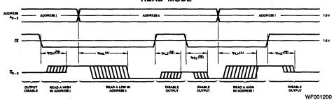
Switching delays from address and chip select inputs to the data output. For the Am27S03A/03 disabled output is "OFF", represented by a single center line. For the Am27S02A/02, a disabled output is HIGH.
