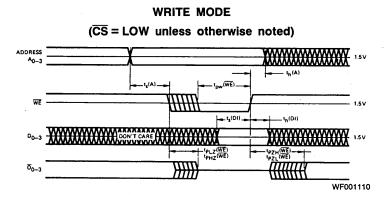
Write Cycle Timing. The cycle in initiated by an address change. After  $t_s(A)$ min, the write enable may begin. The chip select must also be LOW for writing. Following the write pulse,  $t_h(A)$ min must be allowed before the address may be changed again. The output will be inactive (floating for the Am27S07A/07) while the write enable is LOW.
