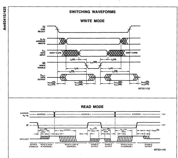
Switching delays from address and chip select inputs to the data output. For the Am93425A/425 disabled output is "OFF", represented by a single center line. For the Am93415A/415 a disabled output is HIGH.
