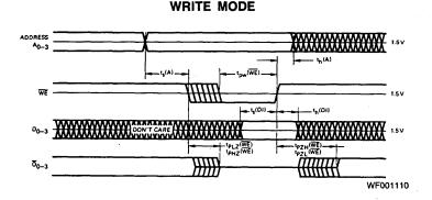
Write Cycle Timing. The cycle is initiated by an address change. After  $t_8(A)$  min, the write enable may begin. The chip select must also be LOW for writing. Following the write pulse,  $t_h(A)$  min must be allowed before the address may be changed again. The output will be inactive (floating for the Am54S/74S189) while the write enable is (WE) LOW.
