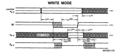
Write Cycle Timing. The cycle is initiated by an address change. After  $t_s(A)$ min, the write enable may begin. The chip select must also be LOW for writing. Following the write pulse,  $t_h(A)$ min must be allowed before the address may be changed again. The output will be inactive (floating for the Am27S03A/03) while the write enable is (WE) LOW.
