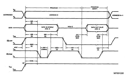
Notes: 1. All times shown in ( ) are minimum in  $\mu sec$  unless otherwise specified. 2. t<sub>DV</sub> and t<sub>DF</sub> are characteristics at the device but must be accommodated by the programmer.
