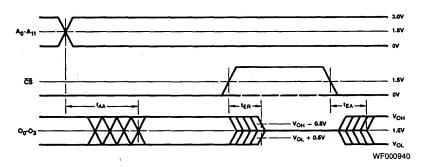
Note: Level on output while  $\overline{\text{CS}}_1$  is HIGH or  $\text{CS}_2$  LOW is determined externally.
