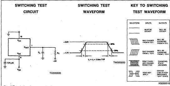
$R_T = 50\Omega$  temination of measurement system  $C_L = 30pF(including stray jig capacitance)$
