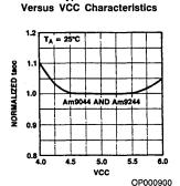
Typical C Load Versus Normalized tacc Characteristics
