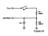
SWITCHING TEST CIRCUIT
