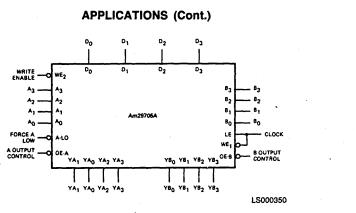
A 16-word by 4-bit two-port RAM with LE and WE<sub>1</sub> connected by to make the device appear edge triggered. WE<sub>1</sub> and WE<sub>2</sub> are logically identical but are electrically slightly different. For
