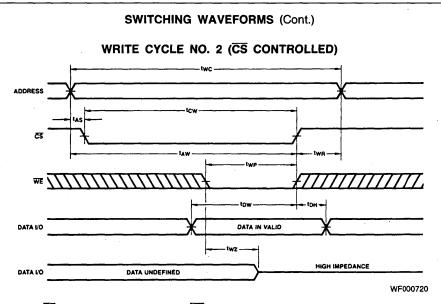
Note: If CS goes high simultaneously with WE high, the output remains in a high impedance state.
