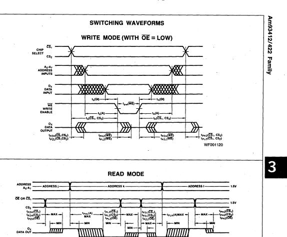
Switching delays form address input, output enable input and the chip select inputs to the data output. For the Am93422A/422 disabled output is "OFF", represented by a single center line. For the Am93412A/412, a disabled output is HIGH.
