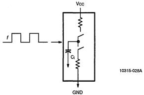
Figure 4–3. Lumped Equivalent Circuit Capacitance
