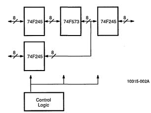
Figure 2-1. 8/16-bit Bus Funnel Using 3 Bidirectional Buffers and a Latch
