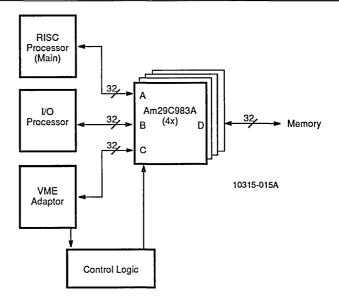
The Am29C983A has 9-bit wide data paths, so parity can be carried along with data. The Am29C985 can be substituted for the Am29C983A if parity generation and checking is desired.
