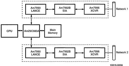
Figure 2–22. Ethernet Bridge Application
