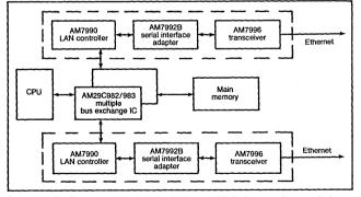
In a typical communication task, the multiple bus exchange links two Ethernets, for example. With the bus exchange's true logical crosspoint interconnection, two operations can occur simultaneously, or data can be broadcast from any one port to any or all of the other three ports.
