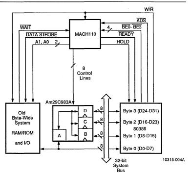
Figure 2–3. 8/32-bit Dynamic Bus Sizing
