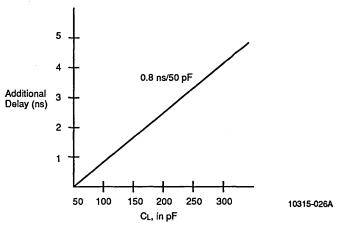
Figure 4–1. Typical Propagation Delay vs. Load Capacitance
