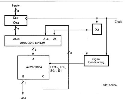
Figure 2-4. Expansion of a ROM-Based Finite-State Machine
