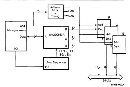
Figure 2–6. Graphics Display – 8/24-bit Bus Expansion
