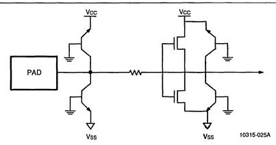
Figure 4-7. Equivalent MBE Input with ESD Structure
