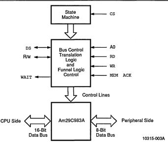
Figure 2–2. 8/16-bit Bus Funnel Using Am29C983A with Control Logic
