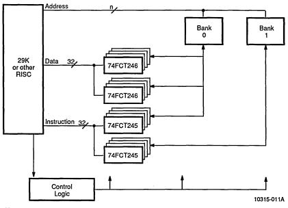
This application requires 19 ns delay time (Buffer + Transceiver/Register) to access the instruction via the data bus.
