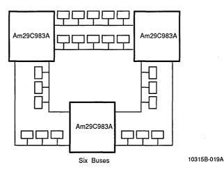
The Am29C983A has 9-bit wide data paths, so parity can be carried along with data. The Am29C985 can be substituted for the Am29C983A if parity generation and checking is desired.
