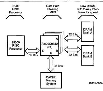
The Am29C983A has 9-bit wide data paths, so parity can be carried along with data. The Am29C985 can be substituted for the Am29C983A if parity generation and checking is desired.
