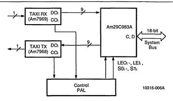
Figure 2–5. TAXI System Interface - 9/18-bit Bus Expansion
