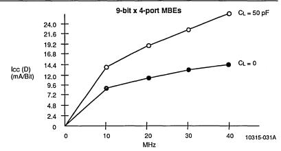
Figure 4-6. Am29C983, 983A, 985 Dynamic Power Supply Current vs. Frequency
