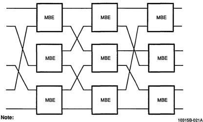
The Am29C983A has 9-bit wide data paths, so parity can be carried along with data. Figure 2–20. Bidirectional Switching Network
