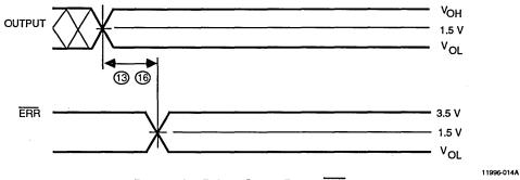
Propagation Delay—Output Port to ERR
