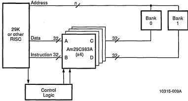
The Am29C983A has 9-bit wide data paths, so parity can be carried along with data. The Am29C985 can be substituted for the Am29C983A if parity generation and checking is desired.
