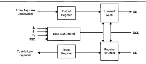
Figure 13. Time Slot Control and IOM 2 Interface
