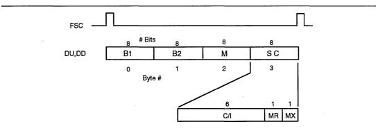
Figure 3. IOM 2 Time Slot Structure (256 kb/s)
