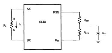
Feed Current programmed by R<sub>DC1</sub> and R<sub>DC2</sub>.
