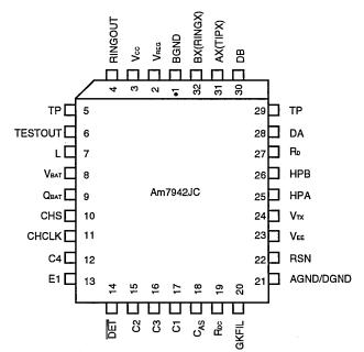
Notes: 1. Pin 1 is marked for orientation. 2. TP is a thermal conduction pin tied to substrate (Q<sub>BAT</sub>).
