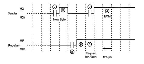
Figure 7. Abort Request on Multiple Byte Message Transfer
