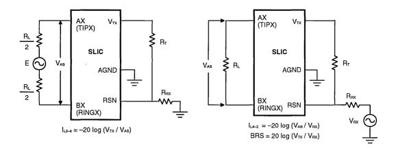
A. Two-to-Four Wire Insertion Loss
