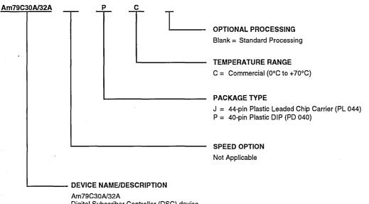
Digital Subscriber Controller (DSC) device ISDN Data Controller (IDC) device
