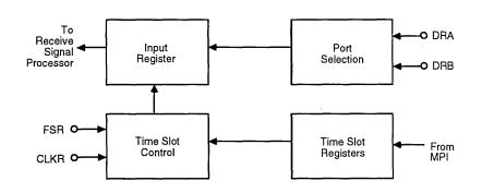
Figure 6. Receive PCM Interface
