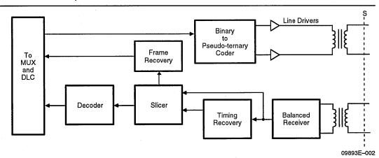
Figure 1. LIU Block Diagram
