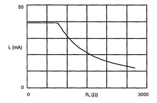
Load Current versus Load Resistance – Am79M531/Am79M535  $V_{\text{BAT}}$  = –47.3 V  $R_{\text{DC}}$  = 62.5K See Figure 1c.
