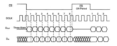
Figure 10. Serial I/O Interface Timing Diagram
