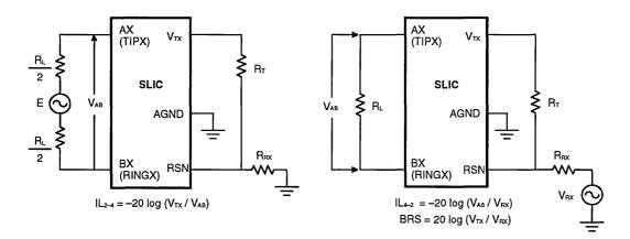
A. Two-to-Four Wire Insertion Loss
