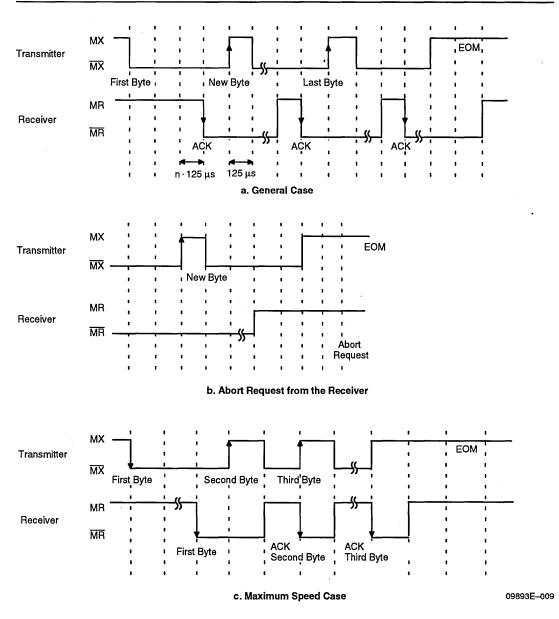
Figure 8. Monitor Handshake Timing
