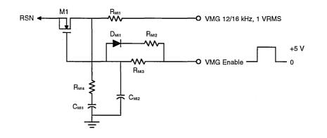
Figure 3. Metering Injection Circuit
