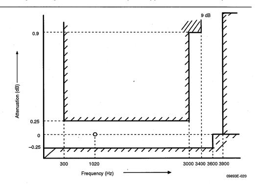
Figure 17. Attenuation/Frequency Distortion (Receive)
