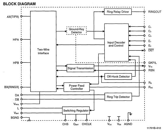
Notes: Am79M531—E₀ and E₁ inputs; ring relay driver sourced internally to BGND; no test relay driver; ground-key filter pin. Am79M535—E₀ and E₁ inputs; ring relay driver sourced internally to BGND; ground-key filter pin. Current gain (K₁) = 1000 for all parts.
