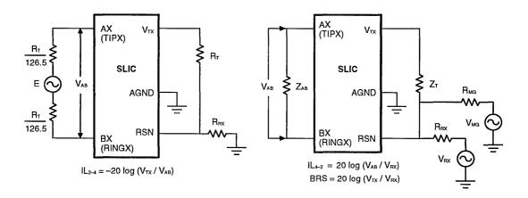
A. Two-to-Four Wire Insertion Loss
