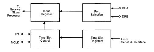
Figure 6. Receive PCM Interface
