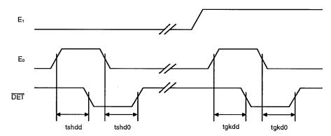
Note: All delays measured at 1.4-V level.
