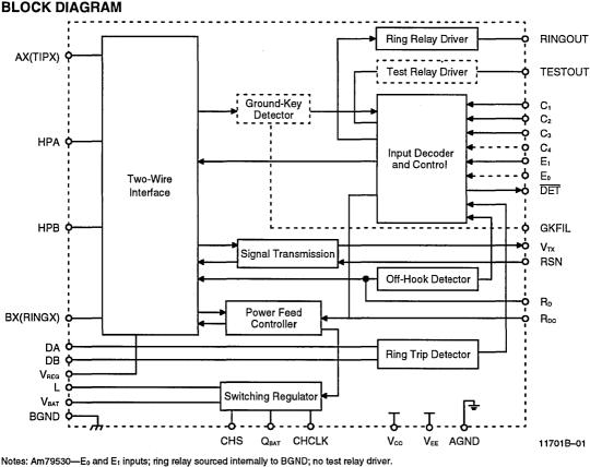
Am79531-E₀ and E₁ inputs; ring relay sourced internally to BGND; no test relay driver, ground key filter pin.
