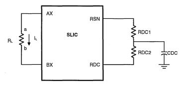
Feed Current programmed by  $R_{\text{DC1}}$  and  $R_{\text{DC2}}$
