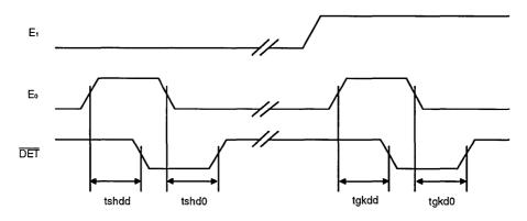
Note: All delays measured at 1.4-V level.
