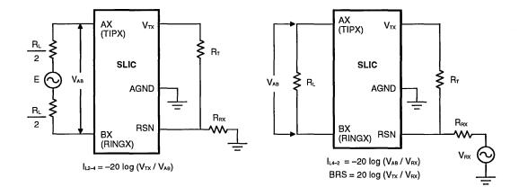
A. Two-to-Four Wire Insertion Loss
