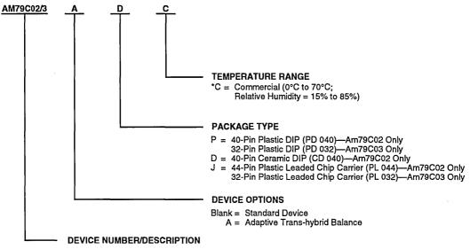
Am79C02/3 Dual Subscriber Line Audio-Processing Circuit (DSLAC Device)
