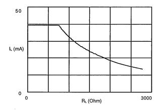
Load Current versus Load Resistance—Am79530/Am79531/Am79534/Am79535  $V_{BAT} = -47.3 V$  $R_{DC} = 62.5K$ See Figure 1c.
