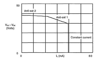
$$\begin{array}{ll} \text{Constant current region:} & I_{L} = \frac{2500}{R_{DC}} \\ & \text{Anti-sat 1 region:} & V_{AX-BX} = 45.78 - \frac{R_{DC}}{152.6} & I_{L} \\ & \text{Anti-sat 2 region:} & V_{AX-BX} = 1.067 \mid V_{BAT} \mid -12.22 - \left(0.0128 + \frac{R_{DC}}{1523}\right) \mid_{L} \\ & \text{See Figure 1c.} \end{array}$$
