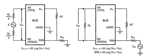
A. Two-to-Four Wire Insertion Loss
