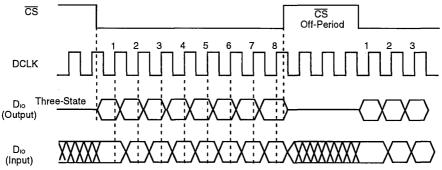
Figure 10. Serial I/O Interface Timing Diagram
