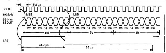
Note: SBIN is sampled on the rising edge of SCLK, SBOUT is changed on the falling edge of SCLK.
