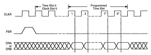
\*For linear code, the 7th and 8th clock cycles correspond to the 15th and 16th clock cycles.
