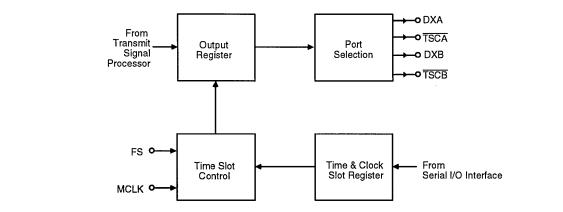
Figure 4. Transmit PCM Interface
