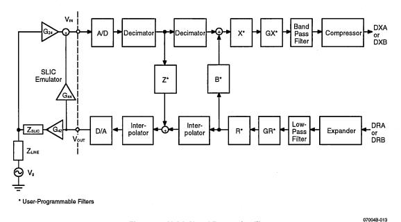
Figure 11. SLAC Signal Processing Flow
