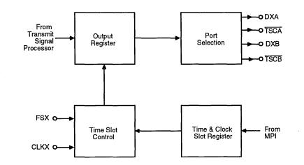
Figure 4. Transmit PCM Interface
