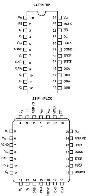
Note: Pin 1 is marked for orientation.
