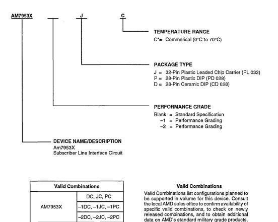
\*The performance specifications contained in this data sheet are valid for the commercial temperature range only. See the SLIC Extended Temperature Supplement for information on industrial temperature range (-40°C to +85°C) specifications.
