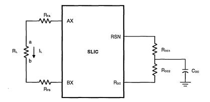
Feed Resistance programmed by  $R_{\text{DC1}}$  and  $R_{\text{DC2}}$ .
