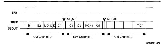
Figure 7. IOM 2 Terminal Mode Frame Structure
