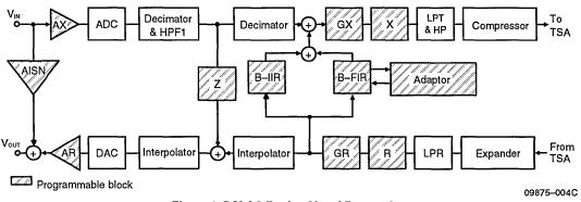
Figure 1. DSLAC Device Signal Processing
