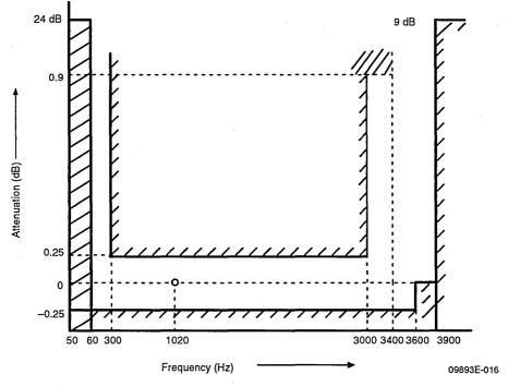
Figure 13. Attenuation/Frequency Distortion (Transmit)
