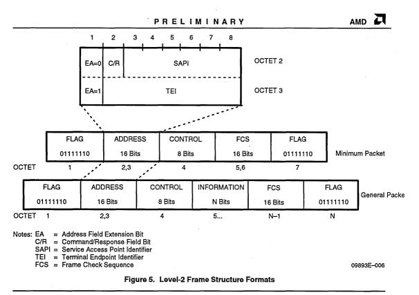
In the case of the LAPD operating environments, the address is a 2-byte address where the first byte is analogous to the Service Access Point Identifier (SAPI) and the second byte is analogous to the Terminal Endpoint Identifier (TEI) as defined by the CCITT recommendations.
