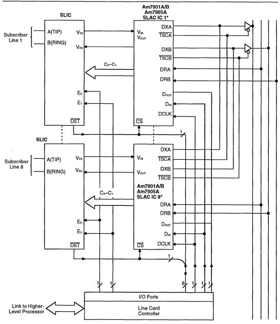
\*1/2 of an Am79C02 DSLAC IC per line can be used. Note: Am7905A combines  $D_{IN}$  and  $D_{OUT}$  into a single pin called  $D_{IO}$ .
