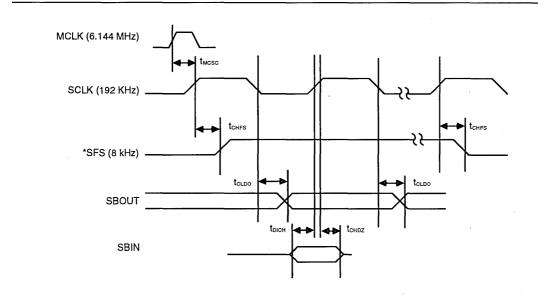
Note 1. CH2STRB timing is identical to SFS timing, but delayed by eight SCLK cycles. Note 2. This timing diagram reflects SCLK for PPCR2(0)=0. For PPCR2(0)=1, the diagram is identical except that the SCLK waveform should be inverted.
