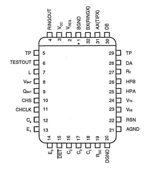
Notes: 1. Pin 1 is marked for orientation. 2. TP is a thermal conduction pin tied to substrate (Q<sub>BAT</sub>).
