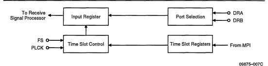
Figure 3. Receive PCM Interface
