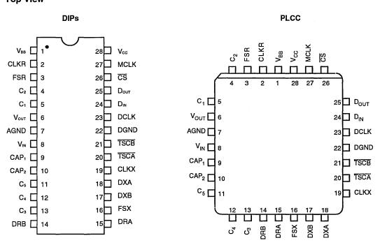
Note: Pin 1 is marked for orientation.
