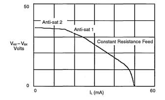
Constant resistance region:  $V_{AX-BX} = 50 - \frac{R_{DC}}{50} I_{L}$ Anti-sat 1 region:  $V_{AX-BX} = 42.72 - \frac{R_{DC}}{76.66} I_L$ Anti-sat 2 region:  $V_{AX-BX} = |V_{BAT}| - 11.86 - \left(\frac{.01 + \frac{R_{DC}}{.036}}{.01 + \frac{.01}{.036}}\right) |_{L}$ See Figure 1c.
