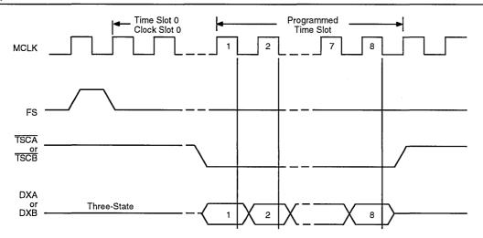
Figure 5. Transmit PCM Timing Diagram
