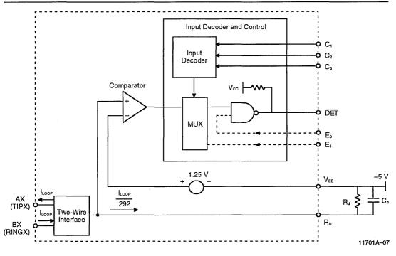
Figure 5. Signaling Off-Hook Detection
