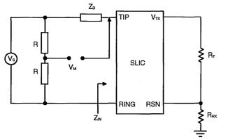
Z<sub>D</sub>: The desired impedance; for example, the characteristic impedance of the line.
