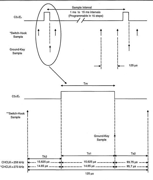
\*Programmed through CHF bit in Ground-Key Sampling Internal Register. \*\*Switch-hook samples occur at the beginning of selected time slot.
