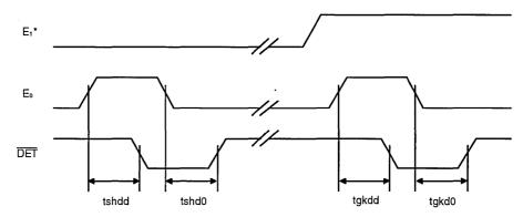
\*This waveform is not applicable to the Am79573. E<sub>1</sub> is internally connected to a logical 0. Note: All delays measured at 1.4-V level.
