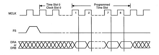
Figure 7. Receive PCM Timing Diagram
