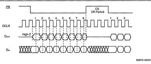
Figure 5. Microprocessor Interface Timing Diagram
