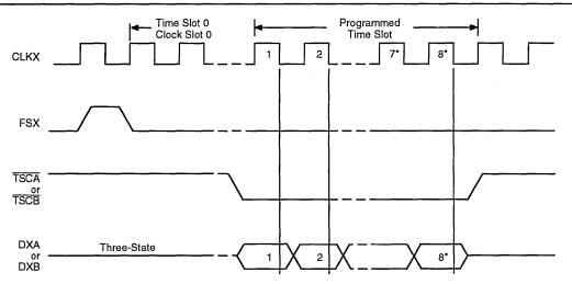
\*For linear code, the 7th and 8th clock cycles correspond to the 15th and 16th clock cycles.
