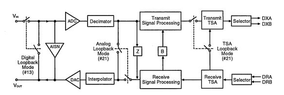
Figure 6. Test Mode Operation
