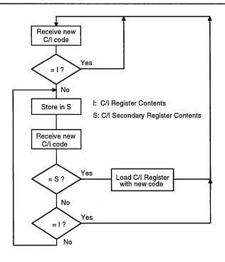
Figure 5. Security Procedure for C/I Downstream Byte
