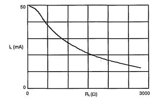
Load Current versus Load Resistance—Am79571/Am79573/Am79574  $V_{BAT}$  = -47.3 V  $R_{DC}$  = 40K See Figure 1c.
