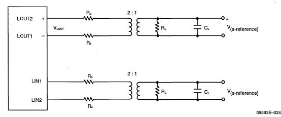
V (s-interface): Transmitter output at the S-interface reference point.
