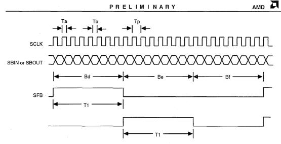
Notes: 1. For PPCR2(0) = 0, SBIN data is sampled on the rising edge of SCLK, SBOUT data is changed on the falling edge of SCLK. For PPCR2(0) = 1, SBIN data is sampled on the falling edge of SCLK; SBOUT data is changed on the rising edge of SCLK. 2. T1 width is eight SCLK periods.
