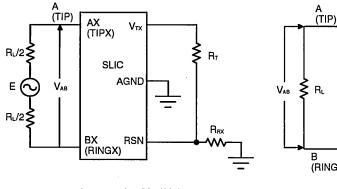
$I_{L2-4} = -20 \log (V_{TX} / V_{AB})$
