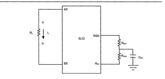
Current programmed by  $R_{DC1}$  and  $R_{DC}$ .
