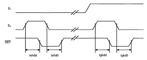
Note: All delays measured at 1.4-V level.
