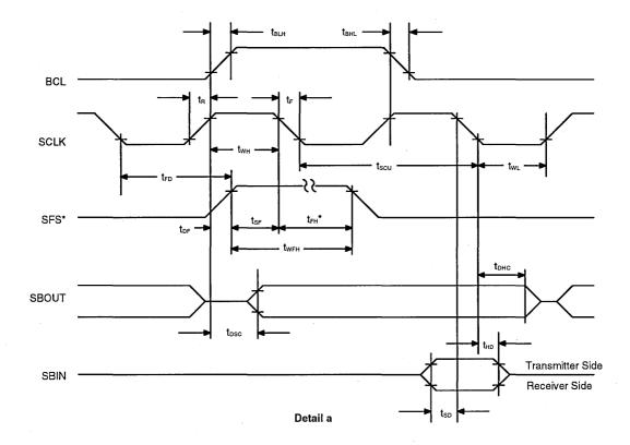
\* In Master Mode, SFS is 16 SCLK cycles + set-up time + hold time in length
