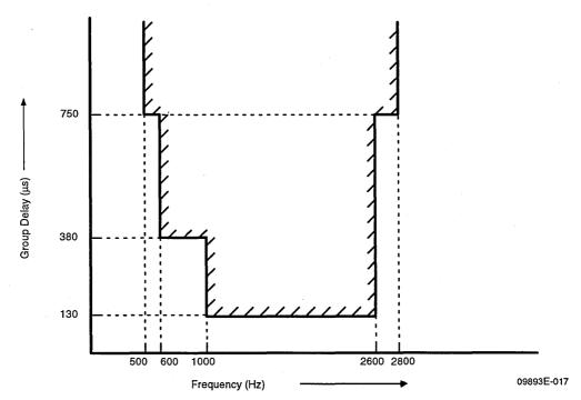
Figure 14. Group Delay Variation with Frequency (Transmit)
