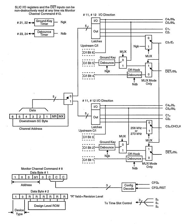
Figure 11. SLIC I/O Architecture
