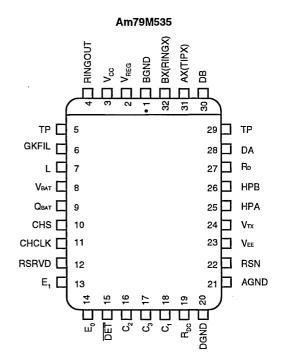
Notes: 1. Pin 1 is marked for orientation. 2. TP is a thermal conduction pin tied to substrate (QBAT).
