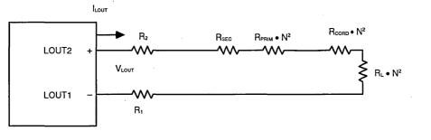
$\begin{array}{l} R_{\text{SEC}} \text{ is the DC impedance of the transformer secondary (IC side of transformer).} \\ R_{\text{PRIM}} \text{ is the DC impedance of the transformer primary (line side of transformer).} \\ R_{\text{CORD}} \text{ is the DC impedance of the TE connecting cord; typically 4–6 ohms.} \end{array}$
