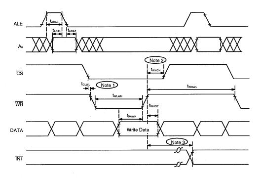
Notes: 1. If  $t_{CLWL}$  is negative,  $t_{WHWL}$  and  $t_{WLWH}$  are measured from  $\overline{CS}$  rather than  $\overline{WR}$ .
