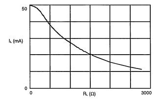
Load Current vs Load Resistance  $V_{BAT} = -47.3 V$  $R_{DC} = 40K$ See Figure 1c.
