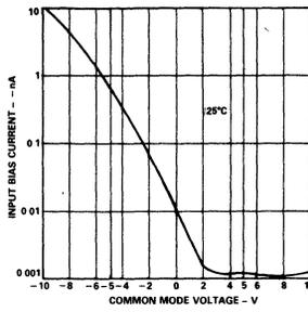
Figure 14. Input Bias Current vs. Common Mode Voltage
