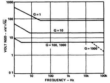
Figure 15. RTI Noise Spectral Density vs. Gain
