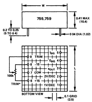
\*Optional 100kΩ external trim pot. Input offset voltage may be adjusted to zero with trim pot connected as shown. With trim terminal 9 left open, input offset voltage will be ±0.4mV (755) or ±2mV (759) maximum.
