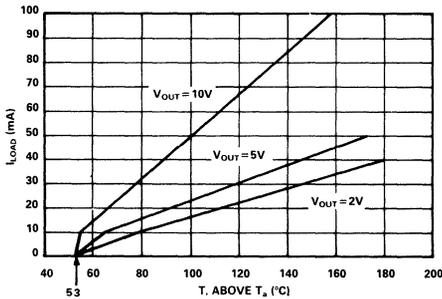
Figure 8. Junction Temp. Rise vs. Load Current
