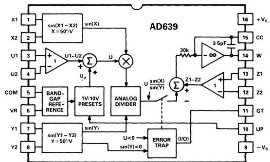
The differential angle arguments are proportional to the input voltages X and Y scaled by  $50^\circ/\text{V}$ . Using the 1.8V on-board reference any of the angular inputs can be preset to  $90^\circ$ . This provides the means to set up a fixed numerator or denominator ( $\sin 90^\circ = 1$ ) or to convert either sine function to a cosine ( $\cos \theta = \sin(90^\circ - \theta)$ ). Using the ratio of sines, all trigonometric functions can be generated (see Table I).
