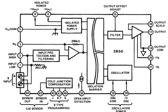
In thermocouple temperature measurement applications, outstanding features such as low drift, high noise rejection, and 1500V isolation make the 2B50 an ideal choice for systems used in harsh industrial environments.
