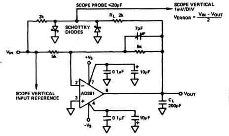
Figure 22. AD381 Unity Gain Inverter Settling Time Test Circuit
