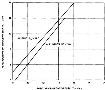
Curve 1. Input/Output Signal Range Vs. Supply Voltages
