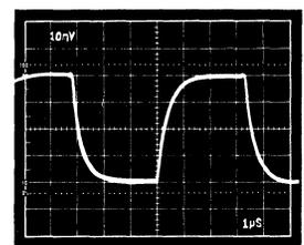
Figure 23. Unity Gain Inverter Small Signal Pulse Response
