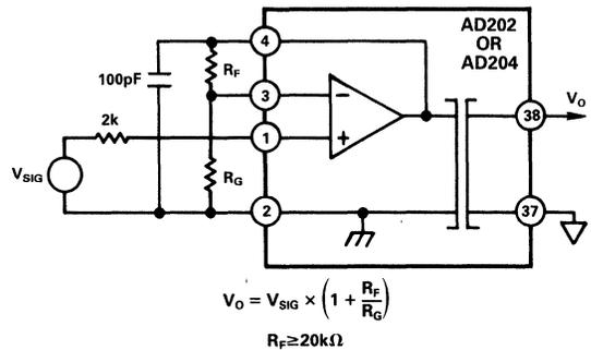
Figure 6. Input Connections for Gain > 1
