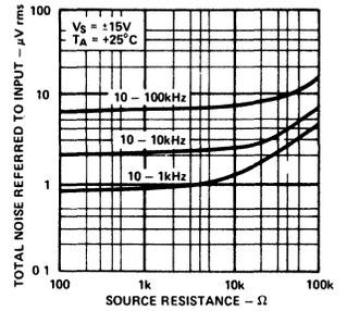
Figure 6. Broad Band Noise vs. Source Resistance
