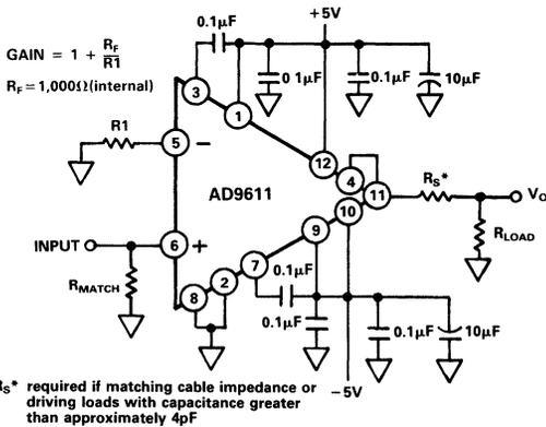
Figure 3. AD9611 Noninverting Operation
