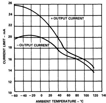
Figure 8. Short Circuit Current Limit vs. Temperature
