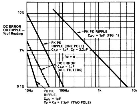
Figure 8. Performance Features of Various Filter Types
