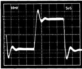
Figure 34. Inverter Pulse Response with 1 MΩ Source and Feedback Resistance
