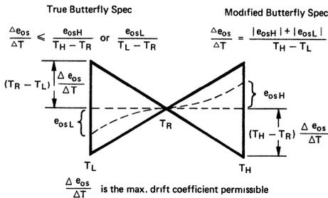
The lowest-cost second-source IC amplifiers are specified only in terms of the maximum value of the parameter (e.g., offset voltage) over temperature in the specified range.
