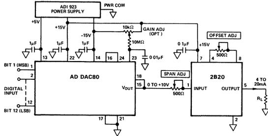
Figure 6. AD DAC80 - 4 to 20mA Current Loop Interface
