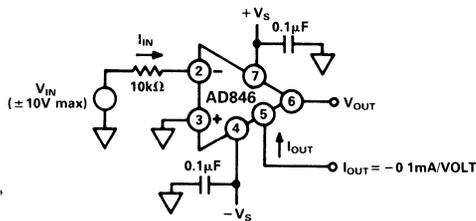
Figure 45. A Precision Transconductance Amplifier
