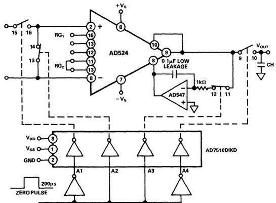
Figure 45. Auto-Zero Circuit
