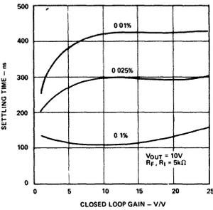
Figure 7. Settling Time vs. Closed Loop Gain
