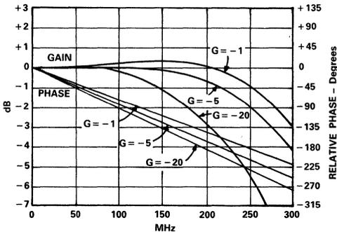
Gain and Phase vs. Frequency – Inverting
