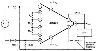
Figure 35c. Ground Returns for Bias Currents with AC Coupled Inputs
