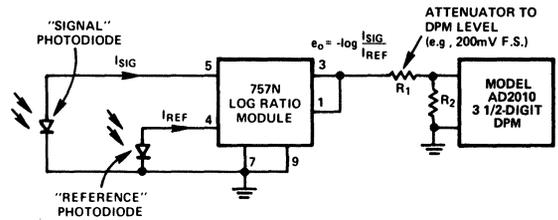
Figure 6. Model 757N Applied to Absorbance Measurements
