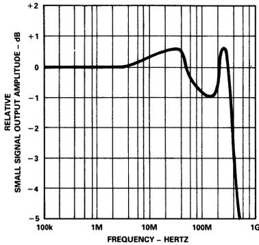
Figure 26. Response of the Gain of 3 Follower Circuit
