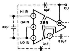
Figure 3. Model 289 Terminal Capacitance
