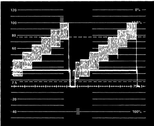
Figure 35. A Six-Step Modulated Staircase Waveform of the 20dB Video Amplifier Circuit
