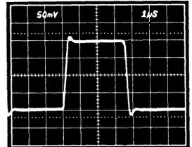
Figure 22c. Unity Gain Inverter Pulse Response (Small Signal)
