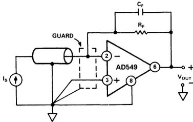
Figure 28. Inverting Amplifier with Guard
