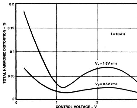
Figure 3b. Total Harmonic Distortion vs. Control Voltage
