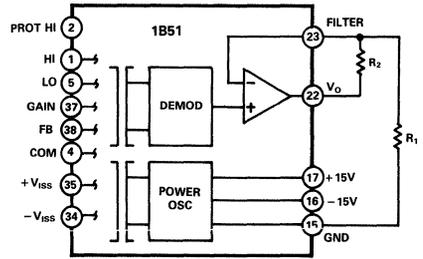
Figure 3. Increasing Output Range
