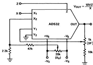
Figure 13. Divider Connection
