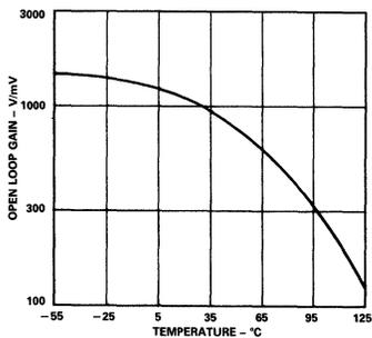
Figure 7. Open Loop Gain vs. Temperature
