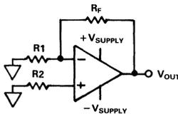
$$\Delta V_{OUT} = [-CMS] [R_F] [\Delta V_{CM}] - [+CMS] [R_2] \left[ 1 + \frac{R_F}{R_1} \right] [\Delta V_{CM}]$$
