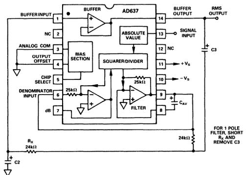
Figure 8. Two Pole Sallen-Key Filter
