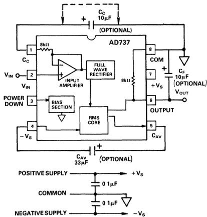
Figure 1. AD737 True rms Circuit
