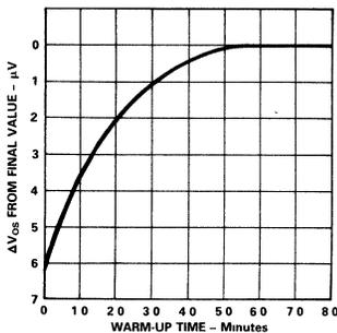
Figure 7. PGA Offset Voltage, RTI, Turn On Drift
