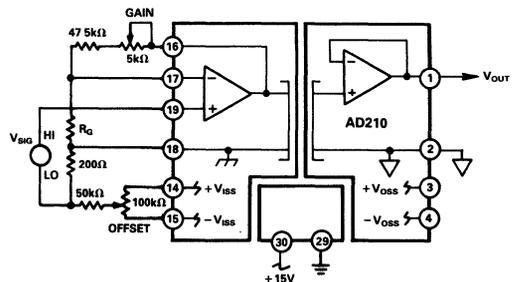
Figure 5. Adjustments for Noninverting Input
