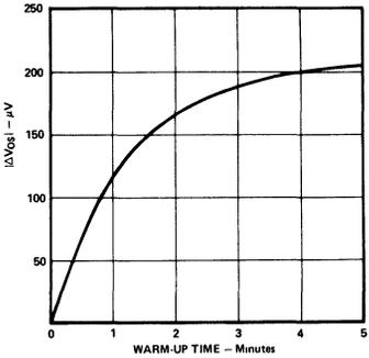
**Figure 7. Change in Offset Voltage vs. Warm-Up Time**
