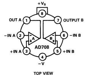
NOTE PIN 4 CONNECTED TO CASE
