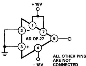
Figure 2. Burn-In Circuit
