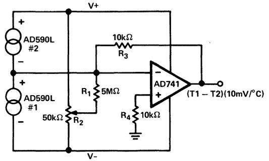
Figure 12. Differential Measurements
