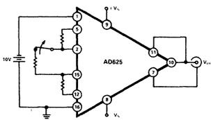
Figure 11. Overage and Gain Switching Test Circuit ( $G=8$ ,  $G=1$ )
