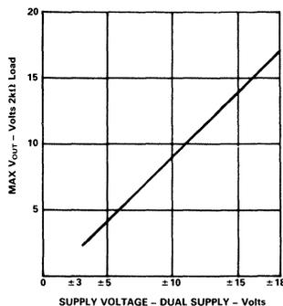
Figure 3. AD637 max  $V_{OUT}$  vs. Supply Voltage
