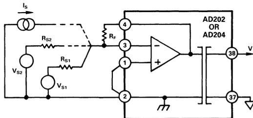
$$V = - \left( V_{S1} \frac{R_F}{R_{S1}} + V_{S2} \frac{R_F}{R_{S2}} + I_S R_F + \dots \right)$$
