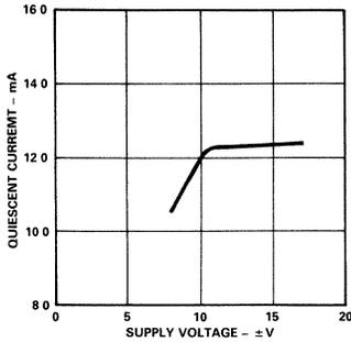
Figure 1. AD365 Quiescent Current vs. Supply Voltage
