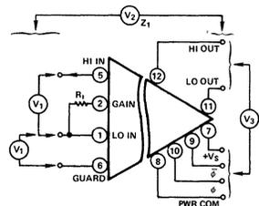
Figure 1. Model 290A and 292A Terminal Ratings
