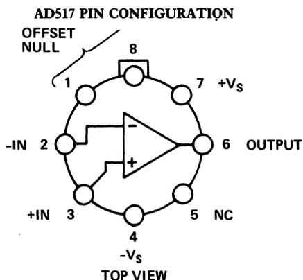
The circuit is packaged in a hermetically sealed TO-99 metal can, and is available in three performance versions (J, K, and L) specified over the commercial 0 to +70 $^{\circ}$ C range; and one version (AD517S) specified over the extended temperature range, -55 $^{\circ}$ C to +125 $^{\circ}$ C.
