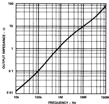
Figure 33. Output Impedance vs. Frequency
