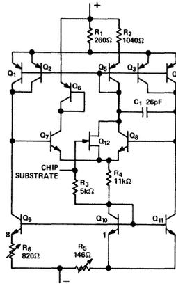
Figure 1. Schematic Diagram
