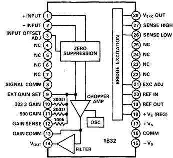
The 1B32 is fully specified over the industrial ( $-25^\circ\text{C}$  to  $+85^\circ\text{C}$ ) temperature range.
