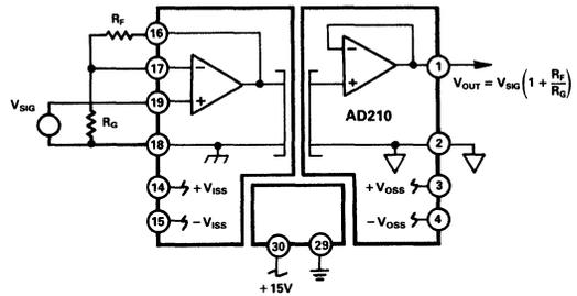
Figure 3. Input Configuration for  $G > 1$
