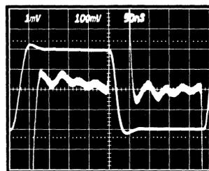
Figure 25c. Unity Gain Inverter Small Signal Response
