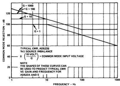
Figure 5. Common Mode Rejection vs. Frequency and Gain
