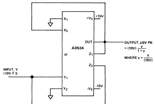
Figure 12. Bridge-Linearization Function
