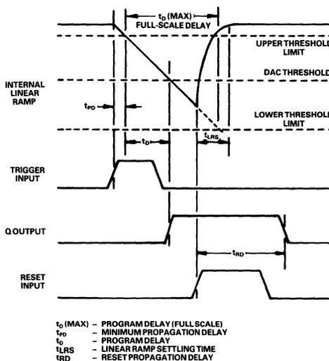
Internal Timing Diagram
