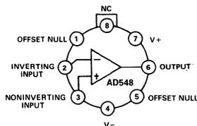
NOTE: PIN 4 CONNECTED TO CASE
