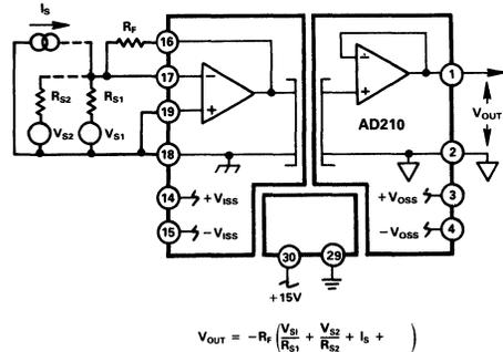
Figure 4. Summing or Current Input Configuration
