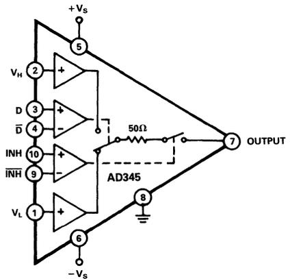
Figure 3. AD345 Block Diagram
