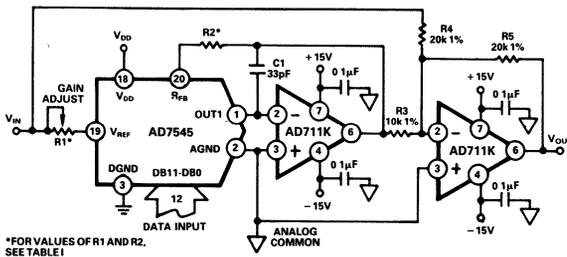
Figure 32. Bipolar Operation
