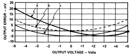
Figure 10. Gain and Offset Adjustment
