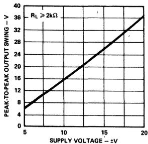
Figure 10. Output Voltage Swing vs. Supply Voltage
