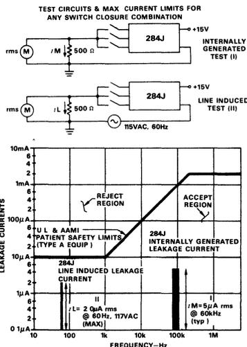
Figure 5. Model 284J Leakage Current Performance from Line Induced and Internally Generated (Modulator) Operating Conditions
