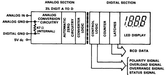
readout is available as BCD data. Application of the metering system in a computer or data logging system is made easy with the availability of the "overrange," "polarity," "overload," and "status" signals.
