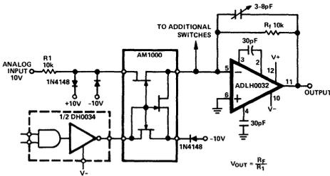
Figure 3. Current Mode Multiplexer
