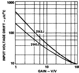
Figure 10. Typical Input Offset Voltage Drift vs. Gain
