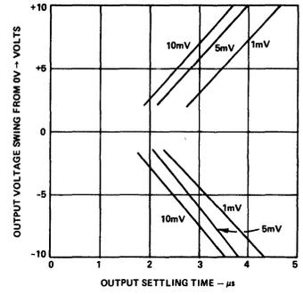
Figure 15. Output Settling Time vs. Output Swing and Settling Time (Circuit of Figure 23)
