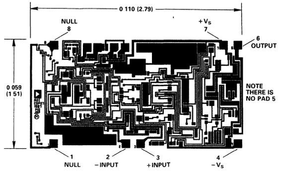
THE AD OP-07 IS AVAILABLE IN WAFER-TRIMMED CHIP FORM FOR PRECISION HYBRIDS. CONSULT THE FACTORY FOR DETAILS.
