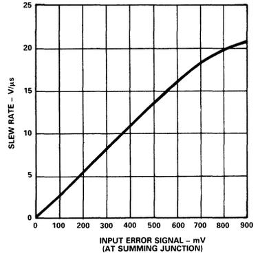
Figure 18. Slew Rate vs. Input Error Signal
