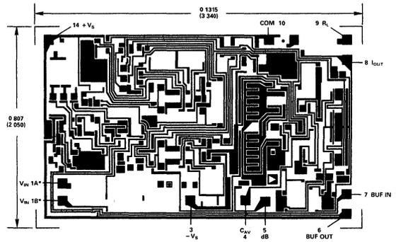
PAD NUMBERS CORRESPOND TO PIN NUMBERS FOR THE TO 116 14 PIN CERAMIC DIP PACKAGE
