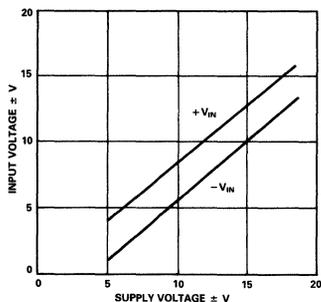
Figure 1. Input Voltage Range vs. Supply Voltage
