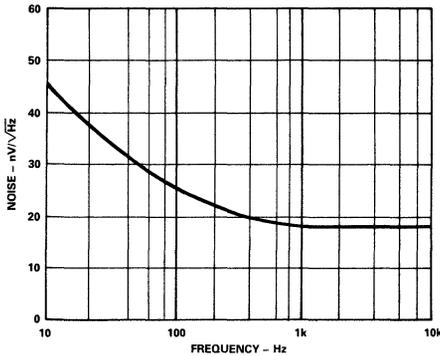
Figure 11. Input Noise vs. Frequency
