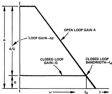
Figure 4. Closed Loop Bandwidth and Loop Gain
