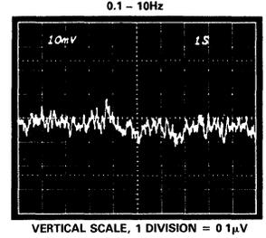
Figure 18. Low Frequency Noise -  $G = 1000$  (System Gain = 100,000)
