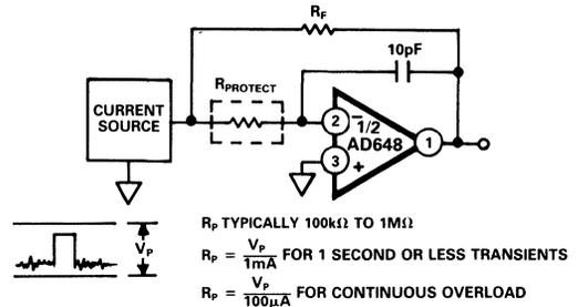
Figure 23a. Input Protection of I-to-V Converter
