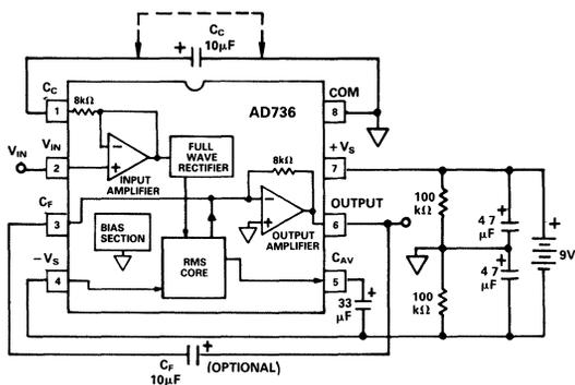
Figure 4. Connection for Battery Powered Operation.
