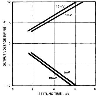
Figure 15. Output Settling Time Vs. Output Swing and Error Voltage
