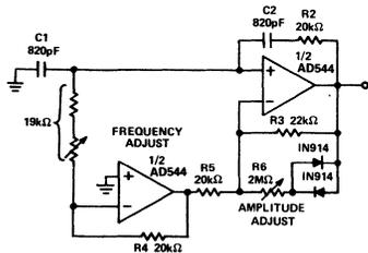
Figure 36. Wien-Bridge Oscillator -  $f_o = 10kHz$
