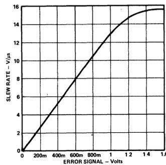
Figure 18. Slew Rate vs. Error Signal
