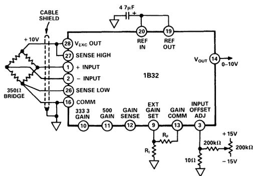
Figure 3. External Gain Setting
