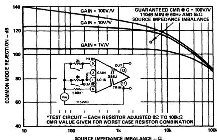
Figure 8. Common Mode Rejection vs. Source Impedance Imbalance
