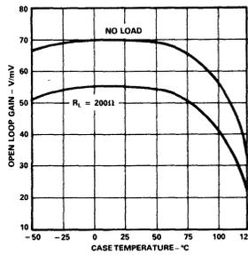
Figure 8. Gain vs. Temperature
