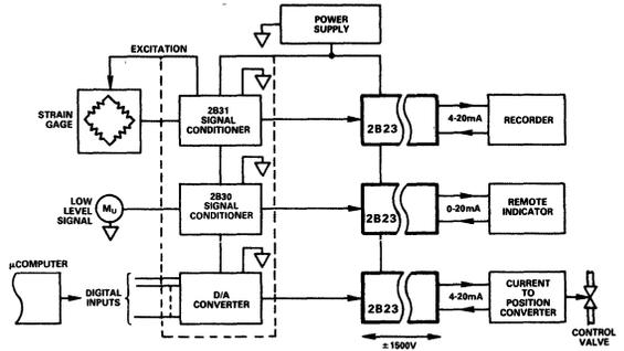
Figure 6. Multiloop Isolation
