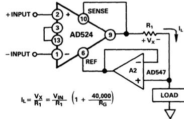
$$I_L = \frac{V_X}{R_1} = \frac{V_{IN}}{R_1} \left( 1 + \frac{40,000}{R_G} \right)$$
