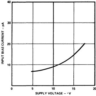
Figure 4. Input Bias Current vs. Supply Voltage
