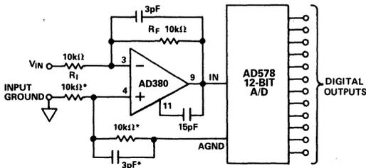
\*Optional Differential Input Components Used to Reject Noise Between Input Ground and the A/D Analog Ground
