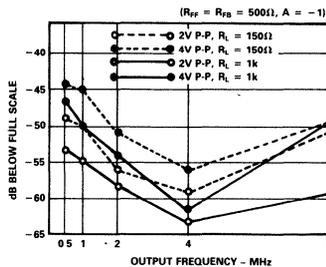
Figure 5. Harmonic Distortion - Inverting
