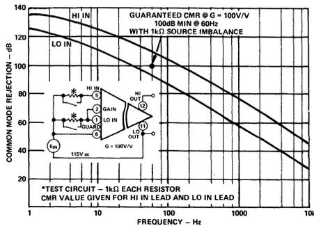
Figure 6. Typical Common Mode Rejection vs. Frequency
