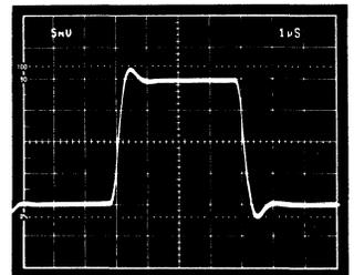
Figure 20c. Unity Gain Inverter Pulse Response (Small Signal)
