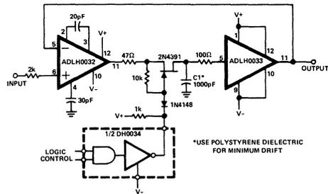
Figure 5. High Speed Sample and Hold
