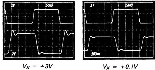
Figure 4b. Multiplier Pulse Response Using ADLH0032 Op Amps
