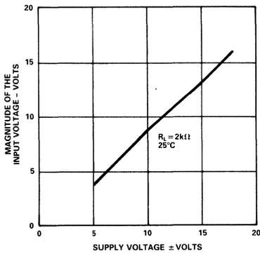
Figure 1. Input Voltage Swing vs. Supply Voltage
