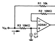
Figure 37. Capacitance Multiplier
