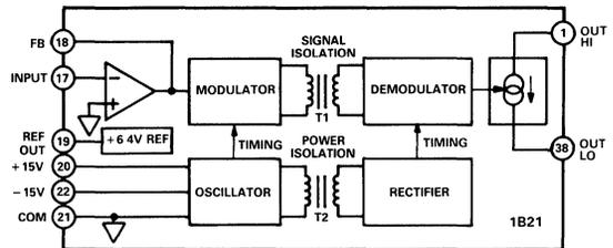
Designed for multichannel applications, the 1B21 requires an external loop supply and can accept up to 30V max. This would provide a loop compliance of 27V, which is sufficient to drive a 1.35k $\Omega$  load resistance.
