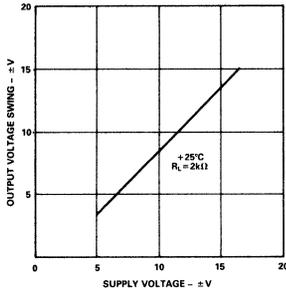
Figure 1. Output Voltage vs. Supply Voltage,  $G = 16$
