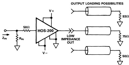
Figure 2. Impedance Transformations for 50Ω, 75Ω, and 93Ω Cables
