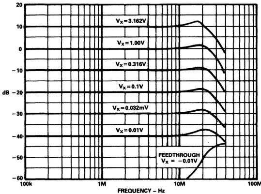
Figure 4a. Multiplier HF Response Using ADLH0032 Op Amps
