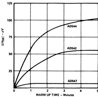
Figure 7. Change in Offset Voltage vs. Warm-Up Time
