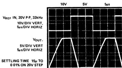
Figure 31b. Voltage Output DAC Settling Characteristic
