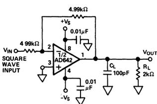
Figure 22a. Unity Gain Inverter Pulse Response (Large Signal)
