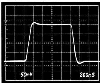
Figure 23c. Unity Gain Inverter Pulse Response (Small Signal)
