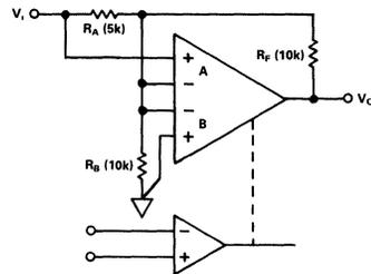
Figure 12. AD630 Symmetric Gain ( $\pm 2$ )
