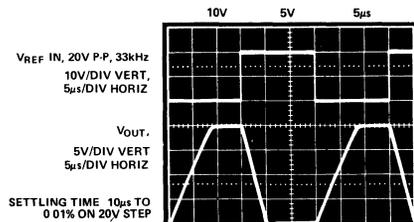
Figure 27b. Voltage Output DAC Settling Characteristic
