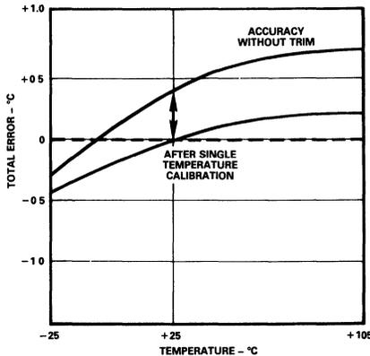
Figure 5. Effect of Scale Factor Trim on Accuracy
