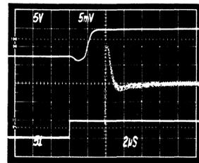
Figure 27. Gain Change Settling Time\*, Gain Change 1 to 4
