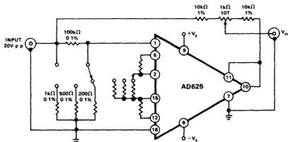
Figure 23. Settling Time Test Circuit
