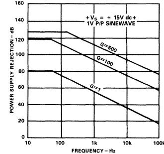
Figure 9. Positive PSRR vs. Frequency
