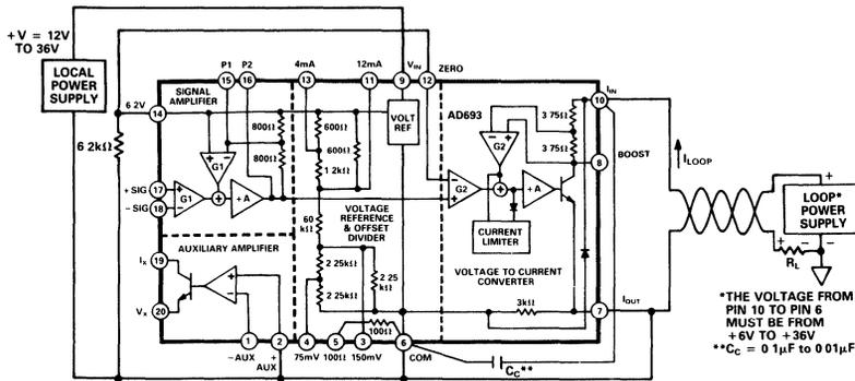
Figure 15. Local Powered Operation with 0-20mA Output
