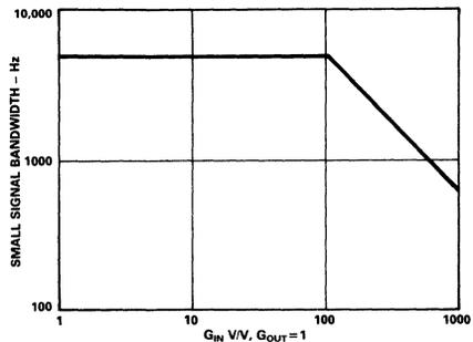
Figure 11. Typical AD295 - Small Signal Bandwidth vs. Gain
