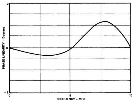
Figure 5c. Phase Linearity Error in Minimal Configuration
