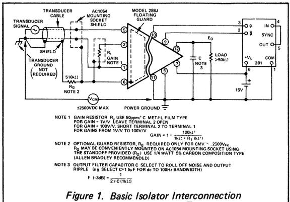
Figure 1. Basic Isolator Interconnection
