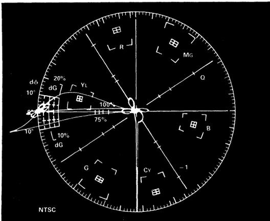
Figure 36. The 20dB Video Amplifier's Response Plotted on a Vector Scope
