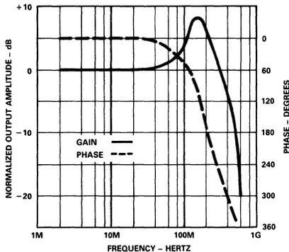
Figure 14. AD5539 Uncompensated Response, Closed-Loop Gain = 7
