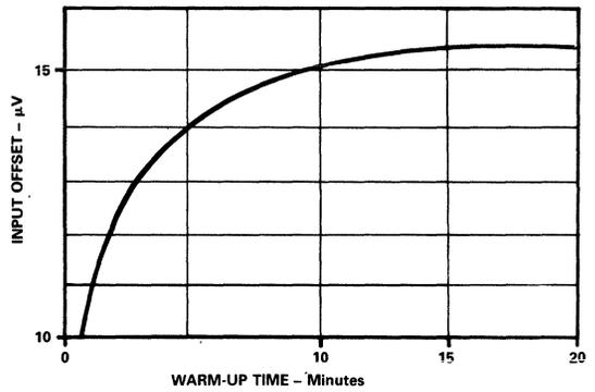
Figure 11. Offset voltage RTI, Turn-On Drift
