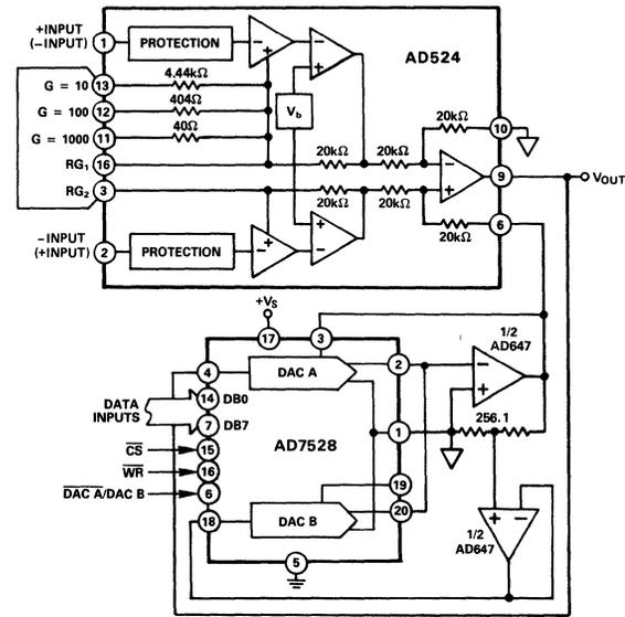
Figure 43. Programmable Output Gain Using a DAC
