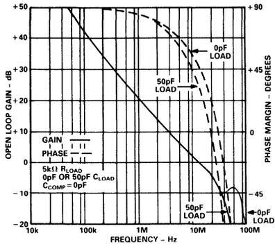
Figure 10. Open Loop Gain and Phase vs. Frequency  $C_{COMP} = 0pF$
