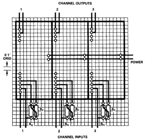
Figure 8. PCB Layout for Multichannel Applications with Gain
