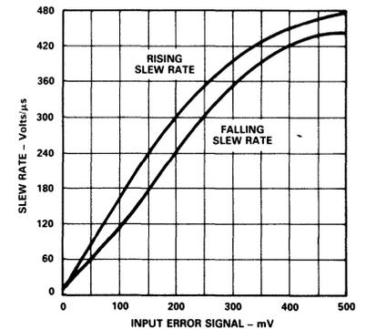
Figure 18. Slew Rate vs. Input Error Signal
