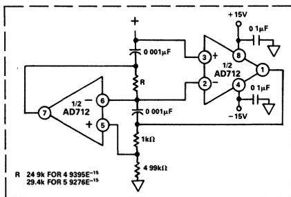
Figure 41. FDNR for 9 Pole Chebychev Filter
