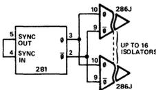
Figure 14. Model 281/286 Connection for Driving from 1 to 16 Isolators
