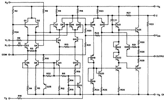
Figure 2. AD532 Schematic Diagram
