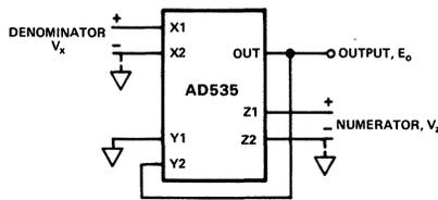
$$V_x (-E_o) = 10V V_z \quad E_o = -10 \frac{V_z}{V_x}$$
