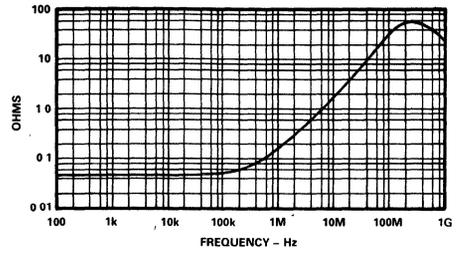
Small-Signal Output Resistance vs. Frequency ( $G = -10$ )
