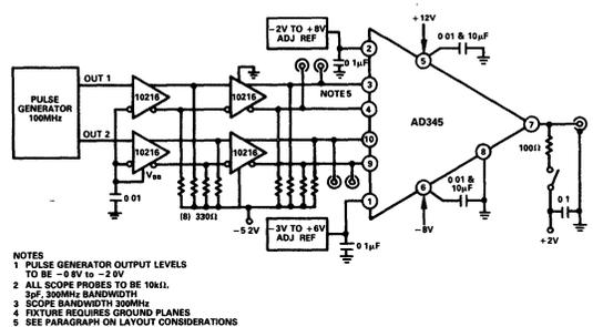
Figure 10. AD345 Test Setup
