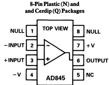
NOTE: PIN 4 CONNECTED TO CASE
