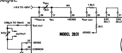
Figure 4. Constant Current Excitation Connections (V<sub>COMPL</sub> = 0 to +10V)
