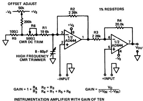
$$\text{GAIN} = 1 + \frac{R_4}{R_3}$$
