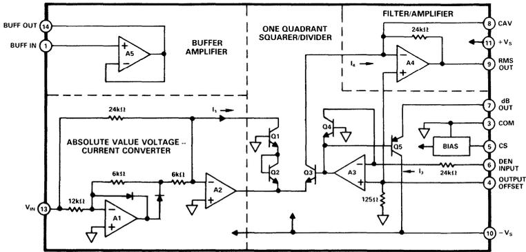
Figure 1. Simplified Schematic
