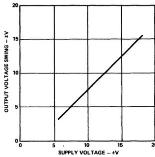
Figure 2. Output Voltage Swing vs. Supply Voltage
