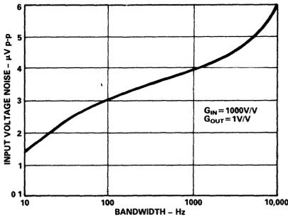
Figure 7. Typical AD295 - Input Voltage Noise vs. Bandwidth
