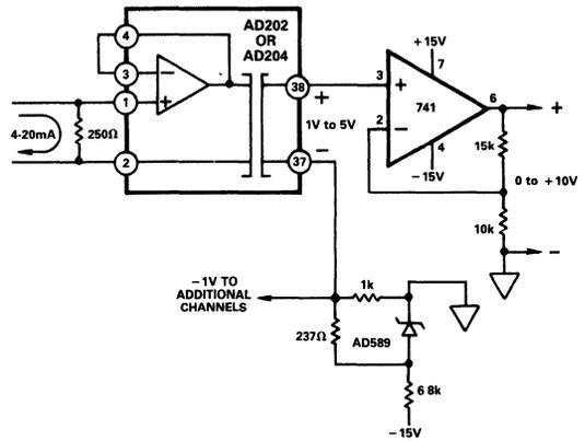
Figure 18. Process Current Input Isolator with Offset
