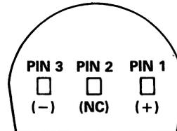
**\*PIN 2 CAN BE EITHER ATTACHED OR UNCONNECTED**
