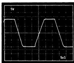
Figure 22. Unity Gain Inverter Large Signal Pulse Response
