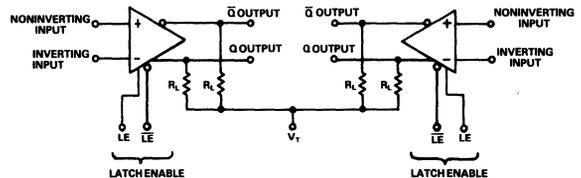
THE OUTPUTS ARE OPEN EMITTERS, REQUIRING EXTERNAL PULL-DOWN RESISTORS. THESE RESISTORS MAY BE IN THE RANGE OF 50Ω-200Ω CONNECTED TO -2.0V, OR 200Ω-2000Ω CONNECTED TO -5.2V
