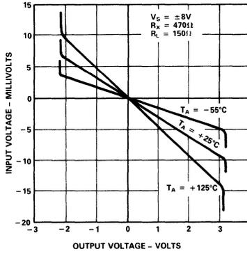
Figure 5. Input Voltage vs. Output Voltage for Various Temperatures
