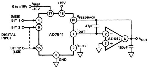
Figure 31a. AD547 Used as DAC Output Amplifier
