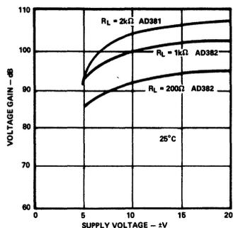
Figure 12. Open Loop Voltage Gain vs. Supply Voltage
