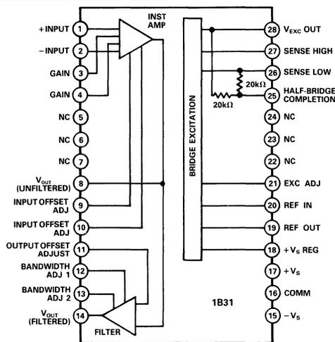
Figure 1. Block Diagram and Pinout
