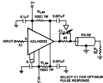
Figure 3. Coaxial Cable Drive
