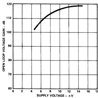
Figure 11. Open Loop Voltage Gain vs. Supply
