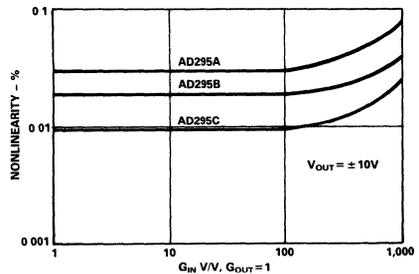
Figure 12. Typical AD295 - Gain Nonlinearity vs. Gain
