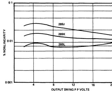
Figure 9. Typical Gain Nonlinearity vs. Output Swing
