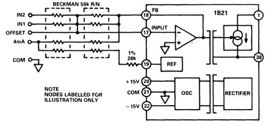
Figure 4. Low Tempco Resistor Network Configuration
