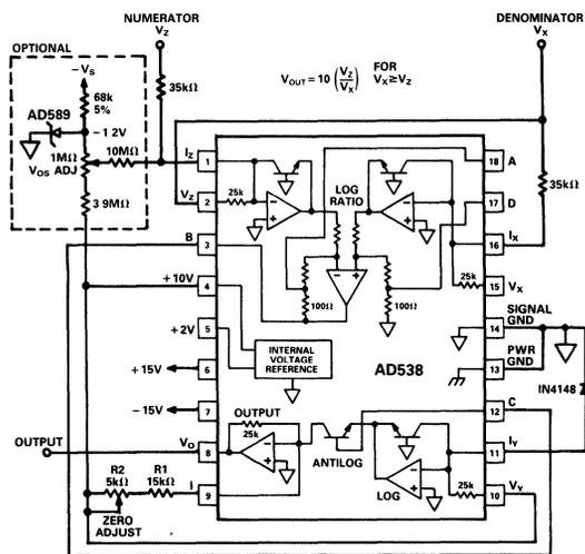
Figure 5. Two-Quadrant Division with 10V Scaling
