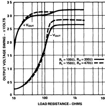
Figure 2. Output Voltage Swing vs. Resistive Load
