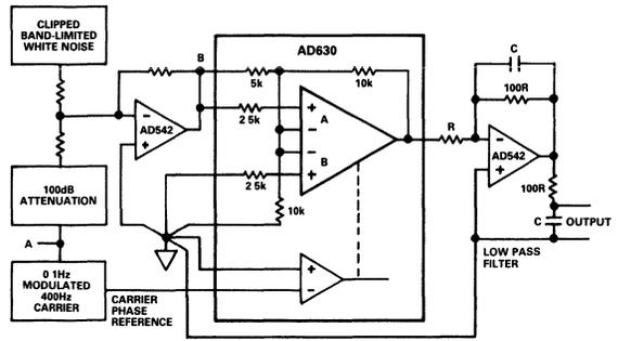
Figure 24. Lock-In Amplifier
