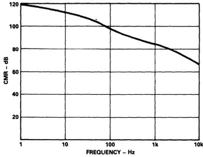
Figure 6. Typical AD295 - CMR vs. Frequency
