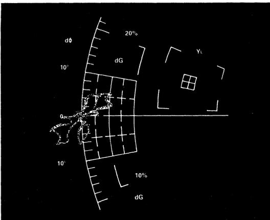
Figure 37. Differential Gain/Differential Phase Target with Generator Output Connected Directly to Vector Scope Input
