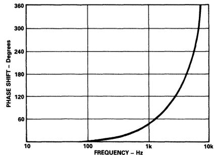
Figure 5. Typical AD295 - Phase Shift vs. Frequency
