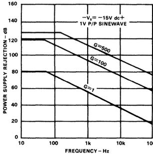
Figure 8. Negative PSRR vs. Frequency
