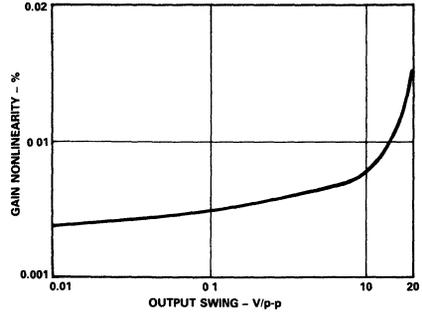
Figure 9. Typical AD295 - Gain Nonlinearity vs. Output Swing
