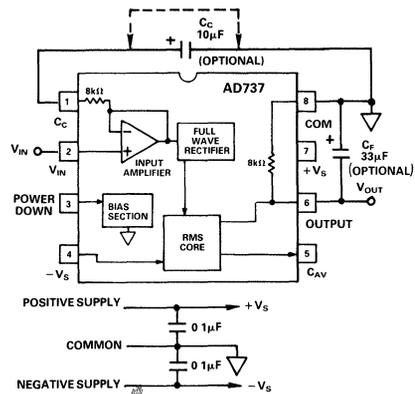
Figure 2. AD737 Average Responding Circuit
