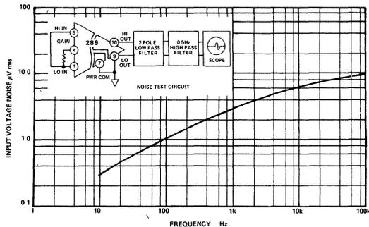
Figure 8. Typical Input Voltage Noise vs. Bandwidth
