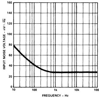
Figure 17. Input Noise Voltage Spectral Density
