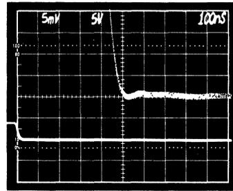
Figure 35. Upper Trace: AD744 Output Voltage for a +10V to 0V Step, Scale: 5mV/division.
