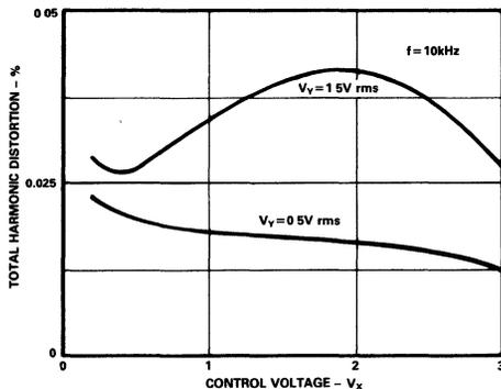
Figure 7b. Distortion in Differential Mode Using ADLH0032 Op-Amp
