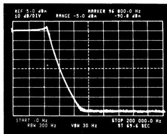
Figure 42. High Frequency Response for 9 Pole Chebychev Filter
