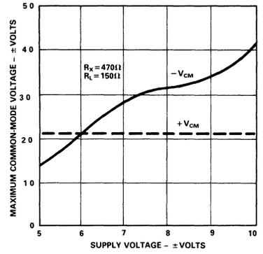
Figure 3. Maximum Common-Mode Voltage vs. Supply Voltage
