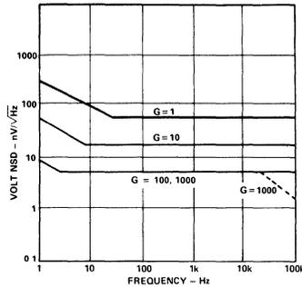
Figure 14. RTI Noise Spectral Density vs. Gain
