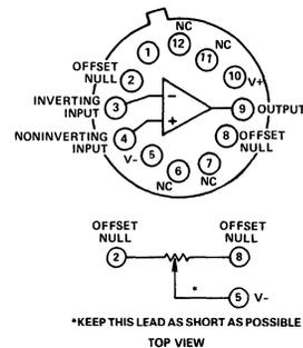
3. Internal frequency compensation, low offset voltage, and full device protection eliminate the need for external components and adjustments. This reduces circuit size and complexity and increases reliability.
