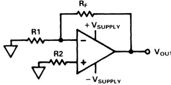
$$\Delta V_{OUT} = [-CMS] [R_f] [\Delta V_{SUPPLY}] + [+CMS] [R_2] \left[ 1 + \frac{R_f}{R_1} \right] [\Delta V_{SUPPLY}] + [CMS_{VOLT}] \left[ 1 + \frac{R_f}{R_1} \right] [\Delta V_{SUPPLY}]$$
