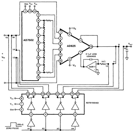
Figure 36. Auto-Zero Circuit
