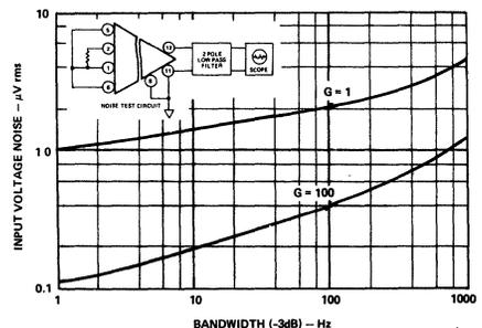
Figure 9. Typical Input Voltage Noise vs. Bandwidth
