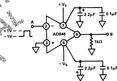
Figure 37. Overload Recovery Test Circuit
