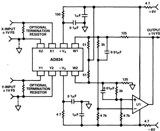
Figure 6. Wideband dc-Coupled Multiplier with  $\pm 1V$  Output
