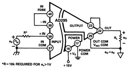
Input to output gain greater than unity can be independently set at the input, output, or both. For input gain configuration see Figures 4b and 4c. Output gain configuration is shown in Figure 4d.
