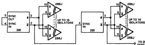
Figure 15. Model 281/286 Connection for Driving > 16 Isolators
