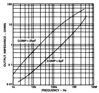
Figure 6. Magnitude of Output Impedance vs. Frequency
