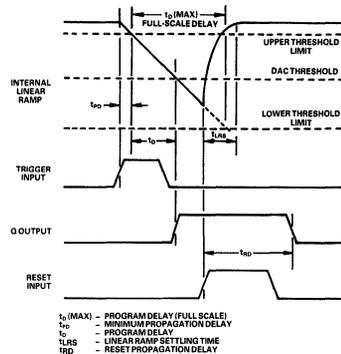
AD9500 Internal Timing Diagram
