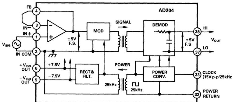
Figure 1b. AD204 Functional Block Diagram
