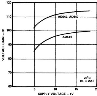
Figure 10. Open Loop Voltage Gain vs. Supply Voltage
