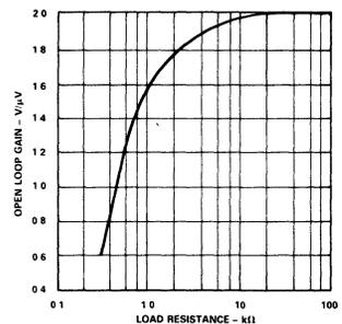
Open Loop Gain vs. Resistive Load
