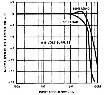
Figure 20. Close Loop Gain vs. Frequency vs. Load
