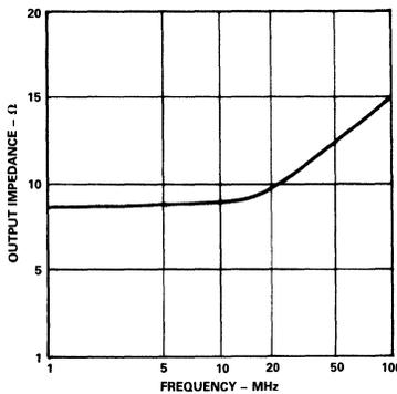
Figure 7. Output Impedance vs. Frequency
