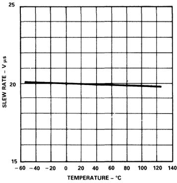
Figure 19. Slew Rate vs. Temperature
