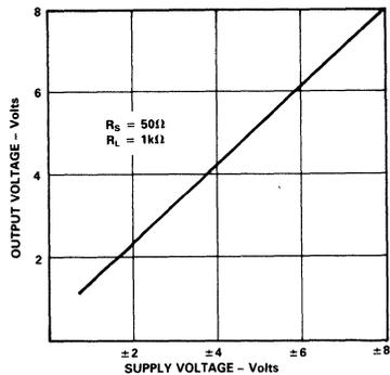
Figure 5. Output Voltage vs. Supply Voltage
