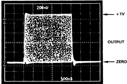
Figure 48. The Control Response of the Video Switcher
