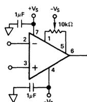
Figure 20. Standard Null Circuit
