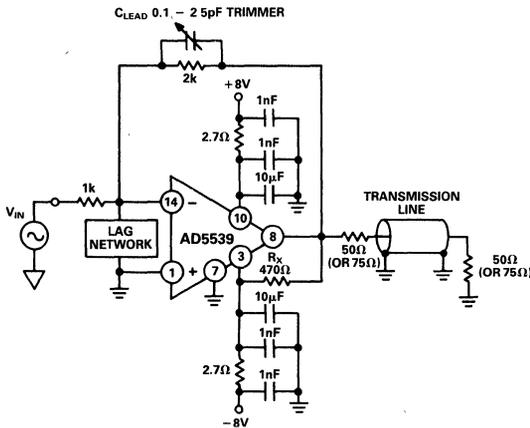
Figure 17. A General Purpose Inverter Circuit
