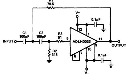
Figure 4. Wideband Two Pole High Pass Filter
