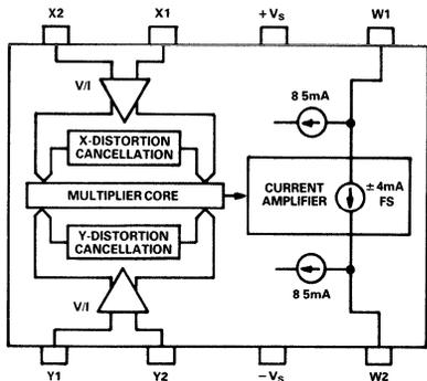
Figure 2. AD834 Functional Block Diagram
