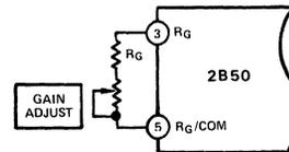
Figure 3. Gain Adjustment
