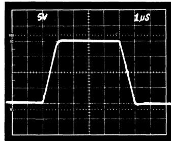
Figure 37. Transient Response  $R_L = 2k\Omega$ ,  $C_L = 500pF$
