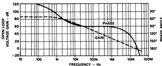
Figure 6. Open Loop Frequency and Phase Response
