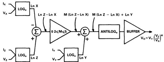
Figure 2. Model Circuit
