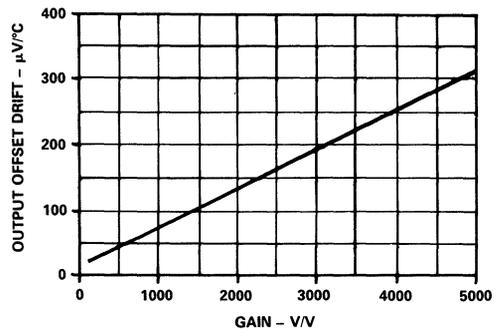
Figure 7. Total Output Offset Drift vs. Gain
