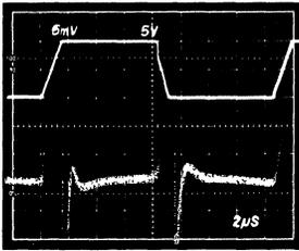
Figure 13. Large Signal Pulse Response and Settling Time\*,  $G=1$
