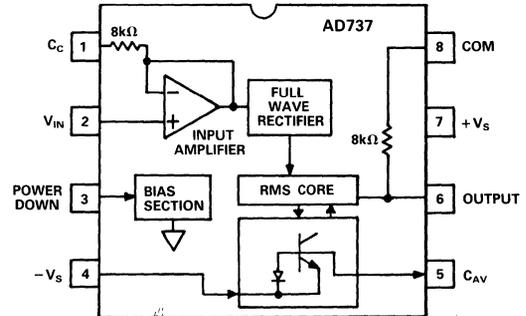
Requiring only 160 $\mu\text{A}$  of power supply current, the AD737 is optimized for use in portable multimeters and other battery powered applications. This converter also provides a "power down" feature which reduces the power supply standby current to less than 30 $\mu\text{A}$ .
