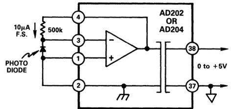
Figure 22. Photodiode Amplifier
