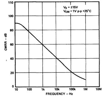
**Figure 12. Common Mode Rejection Ratio vs. Frequency**
