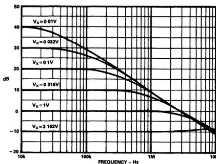
Figure 10b. HF Response of Figure 10a Divider
