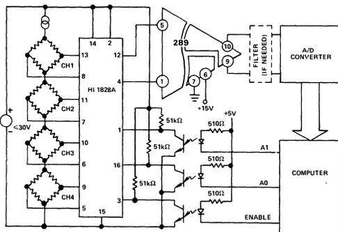
Figure 12. DAS with MUX Ahead of Isolator
