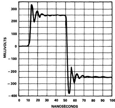
Figure 8. Small-Signal Settling ( $\pm 250\text{mV}$  Square Wave Input)
