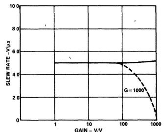
Figure 12. Slew Rate vs. Gain
