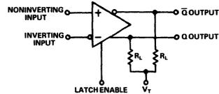
THE OUTPUTS ARE OPEN EMITTERS, REQUIRING EXTERNAL PULL-DOWN RESISTORS. THESE RESISTORS MAY BE IN THE RANGE OF 50Ω-200Ω CONNECTED TO -2.0V, OR 200Ω-2000Ω CONNECTED TO -5.2V
