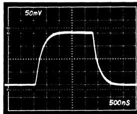
Figure 20. Small Signal Pulse Response,  $G=8$
