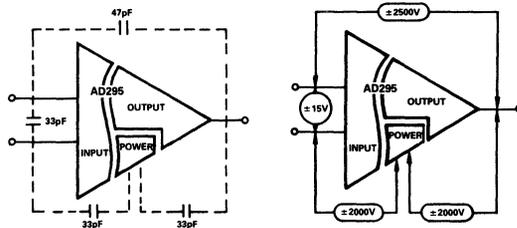
Figure 3. Interelectrode Capacitance and Terminal Ratings
