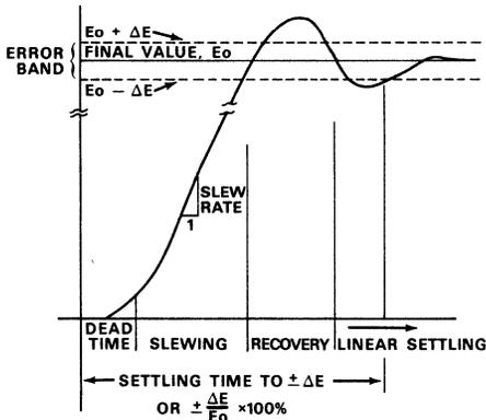
Figure 1. Settling Time
