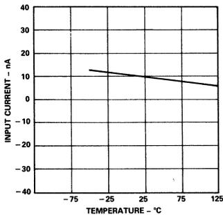
Figure 10. PGA Input Bias Current vs. Temperature
