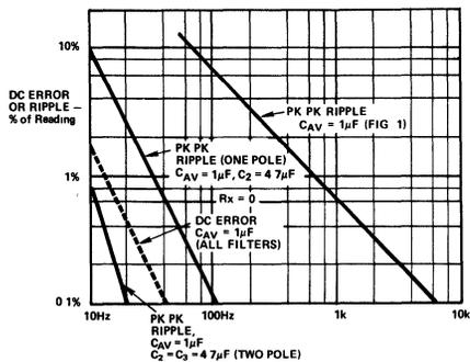
Figure 8. Performance Features of Various Filter Types
