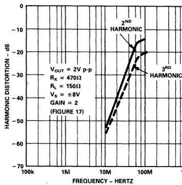
Figure 8. Harmonic Distortion vs. Frequency - Low Gain
