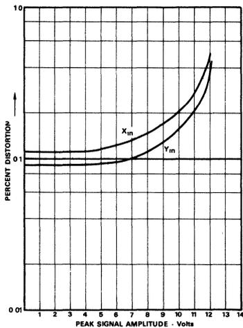
Figure 3. Percent Distortion vs. Input Signal
