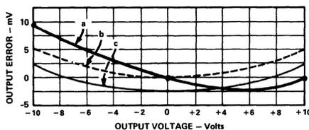
8. Adjust  $R_G$  until the output error is one half that measured in step 6 (see Curve b).
