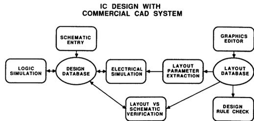
In addition to using these commercial CAD tools, Analog Devices has developed a proprietary compiler for mixed-signal IC design, called JANUS. By integrating all design functions into one environment with a common database, JANUS reduces design time by an order of magnitude.
