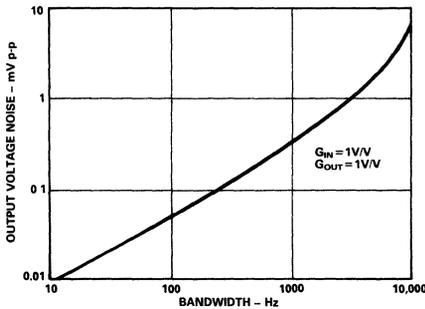
Figure 8. Typical AD295 - Output Voltage Noise vs. Bandwidth
