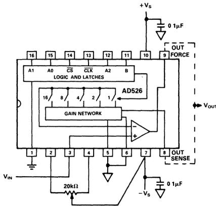
Figure 39. Offset Voltage Null Circuit
