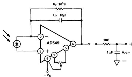
Figure 41. Photodiode Preamp
