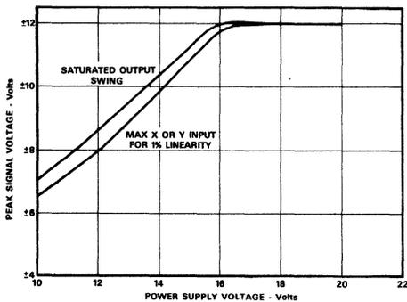
Figure 9. Signal Swing vs. Supply
