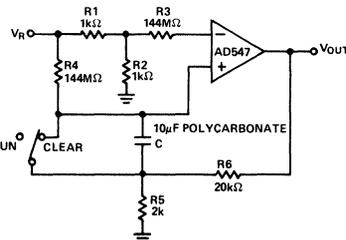
Figure 38. Long Interval Timer - 1,000 Seconds
