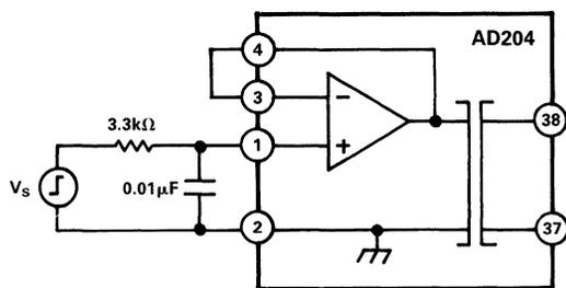
Figure 12. Input Filter for Improved Step Response
