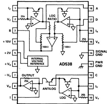
Direct log ratio computation is possible by utilizing only the log ratio and output sections of the chip. Access to the multiple summing junctions adds further to the AD538's flexibility. Finally, a wide power supply range of ±4.5V to ±18V allows operation from standard ±5V, ±12V and ±15V supplies.
