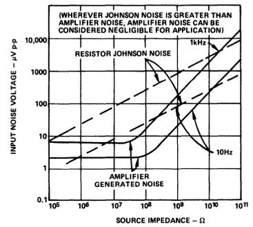
Figure 18. Total rms Noise vs. Source Resistance
