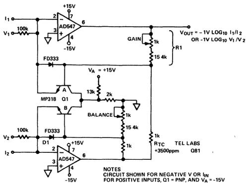
Figure 33. Log-Ratio Amplifier
