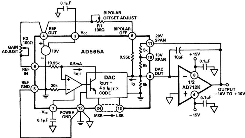
Figure 24.  $\pm 10\text{V}$  Voltage Output Bipolar DAC
