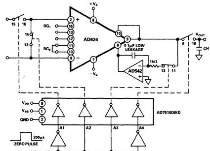
Figure 42. Auto-Zero Circuit
