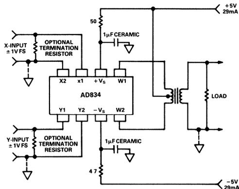
Figure 4. Transformer-Coupled Output
