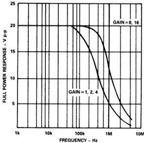
Figure 7. Large Signal Frequency Response
