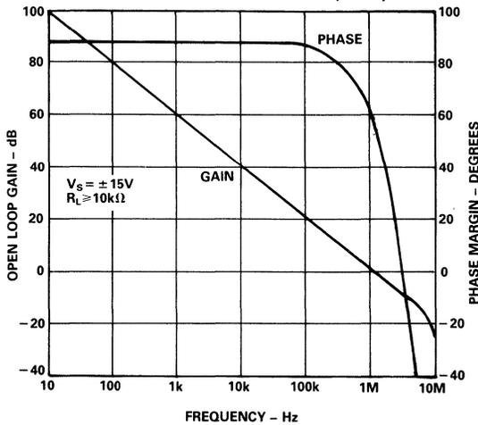
Figure 5. Open Loop Frequency Response
