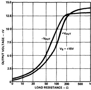
Figure 3b. Output Voltage Swing vs. Load Resistor for AD382
