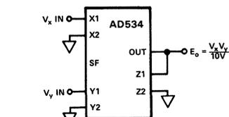
$$\text{BASIC RELATIONSHIP: } (X_1 - X_2)(Y_1 - Y_2) = 10V(Z_1 - Z_2) \\ V_x V_y = 10V E_o$$
