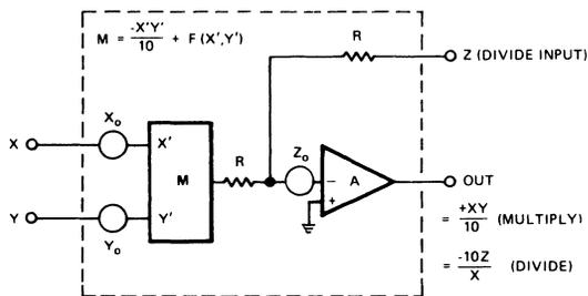
Functional Block Diagram of Typical Multiplier/Divider
