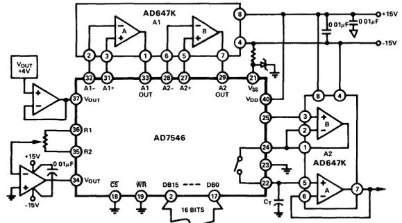
Figure 24. AD647 Used with AD7546 16-Bit DAC
