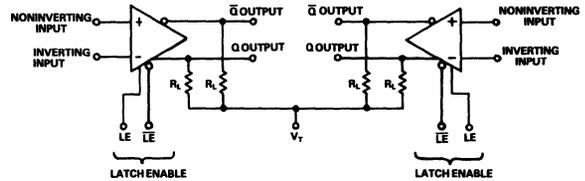
THE OUTPUTS ARE OPEN EMITTERS, REQUIRING EXTERNAL PULL-DOWN RESISTORS. THESE RESISTORS MAY BE IN THE RANGE OF 50Ω-200Ω CONNECTED TO -2.0V, OR 200Ω-2000Ω CONNECTED TO -5.2V.
