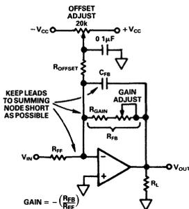
Figure 4. HOS-060 Offset and Gain Adjust
