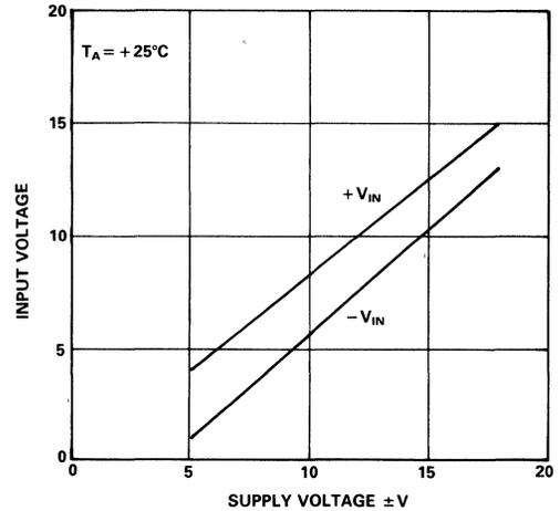
Figure 6. Input Common-Mode Range vs. Supply Voltage
