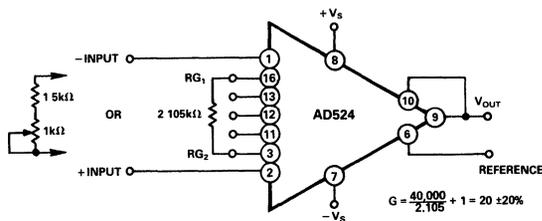
Figure 31. Operating Connections for  $G = 20$
