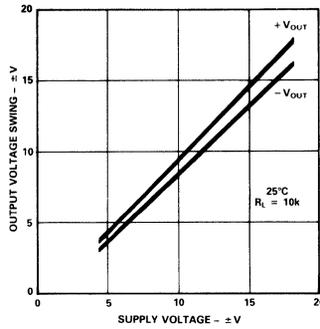
Figure 2. Output Voltage Swing vs. Supply Voltage
