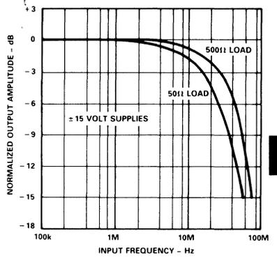
Figure 28. Closed-Loop Gain vs. Frequency vs. Load
