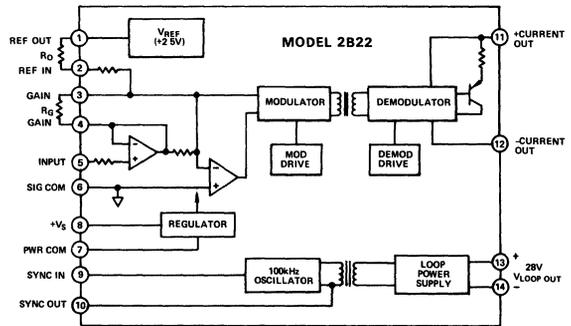
meets the requirements of the Instrument Society of America Std. 50.1 "Compatibility of Analog Signals for Electronic Industrial Process Instruments" for Type 4, Class U isolated current loop transmitters.
