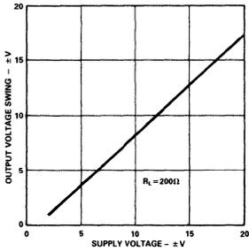
Figure 19. Output Voltage Swing vs. Supply Voltage
