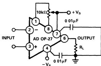
Figure 1. Optional Offset Nulling Circuit and Power Supply Bypassing
