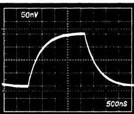
Figure 22. Small Signal Pulse Response, Gain = 16
