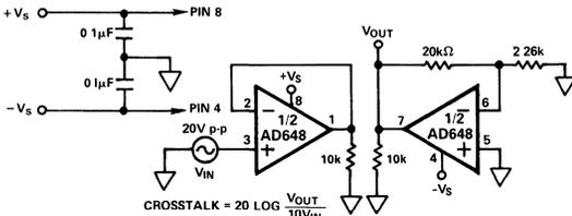
Figure 21. Crosstalk Test Circuit
