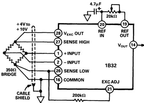
Figure 5. Constant Voltage Excitation: +4 to +10V Range
