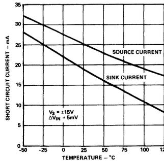
Figure 4a. Short Circuit Current vs. Temperature for AD381
