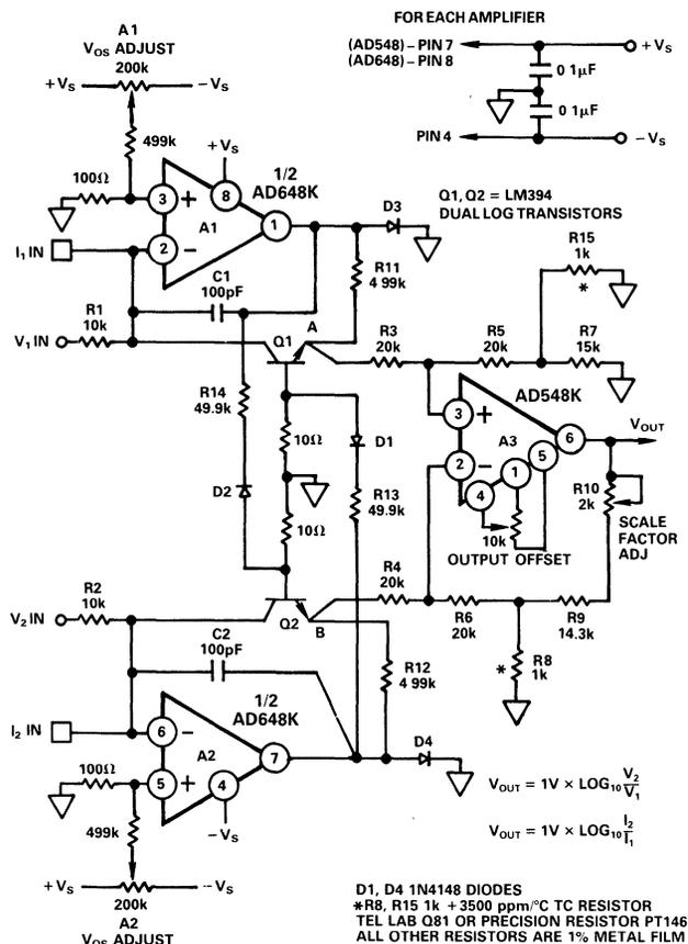
Figure 30. Precision Log Ratio Amplifier
