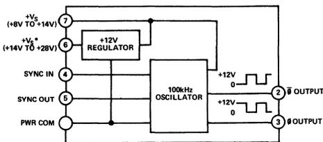
\*LEAVE TERMINAL 6 OPEN, WHEN POWER IS APPLIED TO TERMINAL 7
