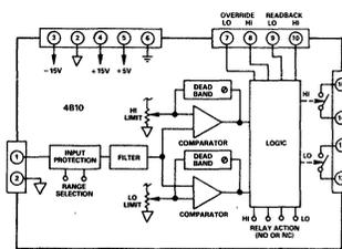
Figure 1. 4B10 Functional Block Diagram
