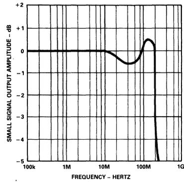
Figure 18. Response of the (Figure 17) Inverter Circuit Without a Lag Compensation Network
