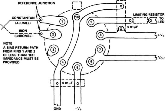
Figure 4. PCB Connections
