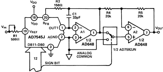
Figure 24. 12-Bit Plus Sign Magnitude D/A Converter
