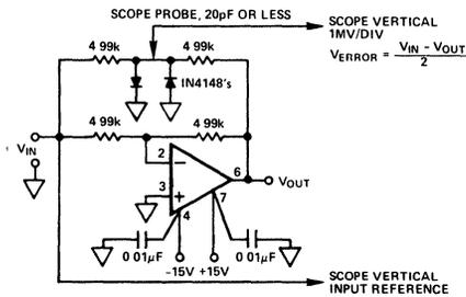
Figure 25. Settling Time Test Circuit
