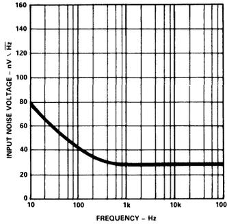
Figure 17. Input Noise Voltage Spectral Density
