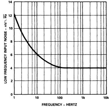
Figure 6. Low Frequency Input Noise vs. Frequency
