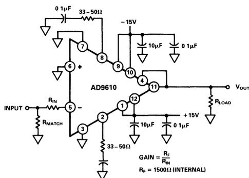
Figure 6. AD9610 Inverting Operation
