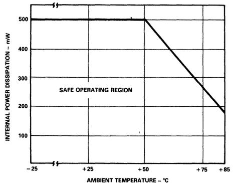
Figure 13. Excitation Source Internal Power Dissipation vs. Temperature
