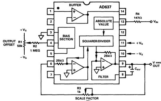
Figure 5. Optional External Gain and Offset Trims
