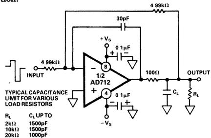
Figure 36. Circuit for Driving a Large Capacitive Load
