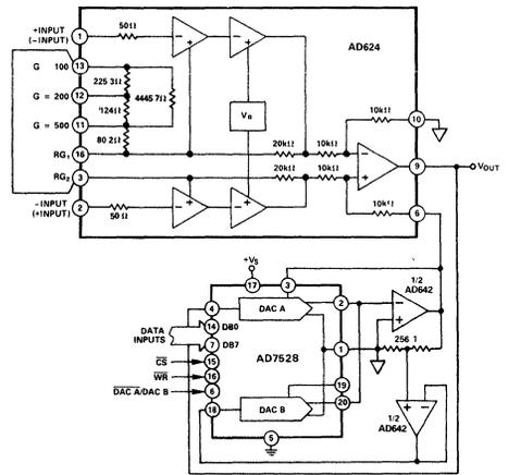
Figure 40. Programmable Output Gain Using a DAC
