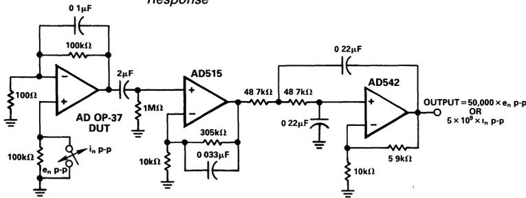
NOTE: ALL CAPACITORS MUST BE NONPOLARIZED
