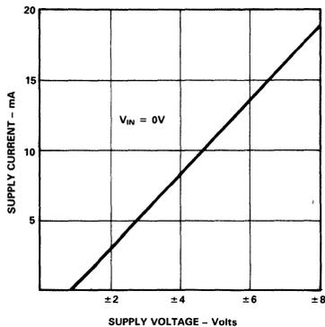
Figure 6. Supply Current vs. Supply Voltage
