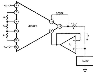
Figure 31. Voltage-to-Current Converter
