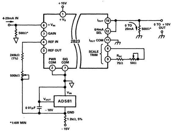
Figure 7. 4-20mA to 0 to +10V Isolated Converter
