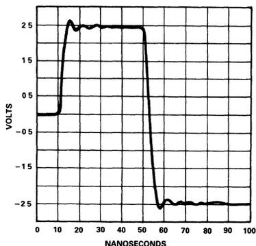
Figure 9. Large-Signal Settling ( $\pm 2.5\text{V}$  Square Wave Input)
