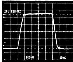
Figure 8. Large Signal 50ns Pulse
