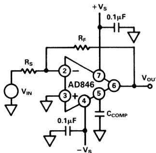
Figure 43. AD846 Inverting Amplifier Showing External Compensation Connection
