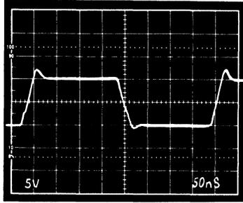
Figure 27b. Large Signal Pulse Response, Gain of 10
