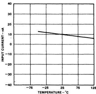
Figure 10. Input Bias Current vs. Temperature
