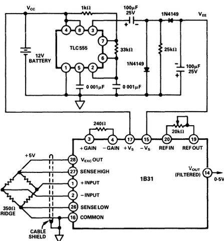
Figure 18. Negative Supply Generation for 1B31
