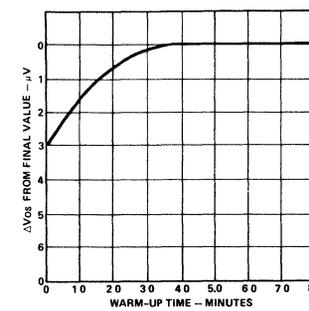
Figure 8. Offset Voltage, RTI, Turn On Drift
