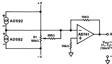
Figure 10. Differential Measurements
