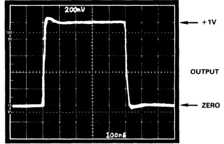
Figure 49. The Signal Response of the Video Switcher
