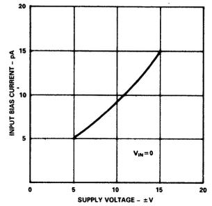
Figure 3. Input Bias Current vs. Supply Voltage
