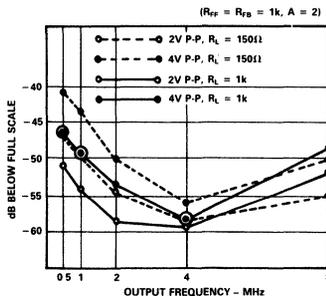
Figure 6. Harmonic Distortion - Noninverting
