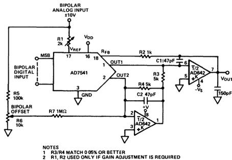
Figure 27a. AD642 Used as DAC Output Amplifier
