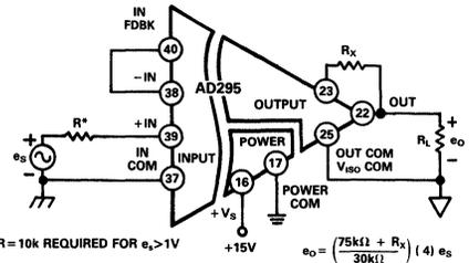
d. Output Gain Noninverting Configuration
