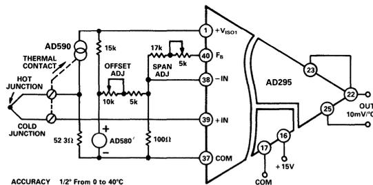
Figure 14. Isolated Temperature Measurement with Cold Junction Compensation
