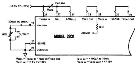
Figure 3. Constant Current Excitation Connections (V<sub>COMPL</sub> = 0 to +5V)
