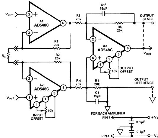
Figure 29. Low Power Instrumentation Amplifier
