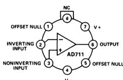
NOTE: PIN 4 CONNECTED TO CASE
