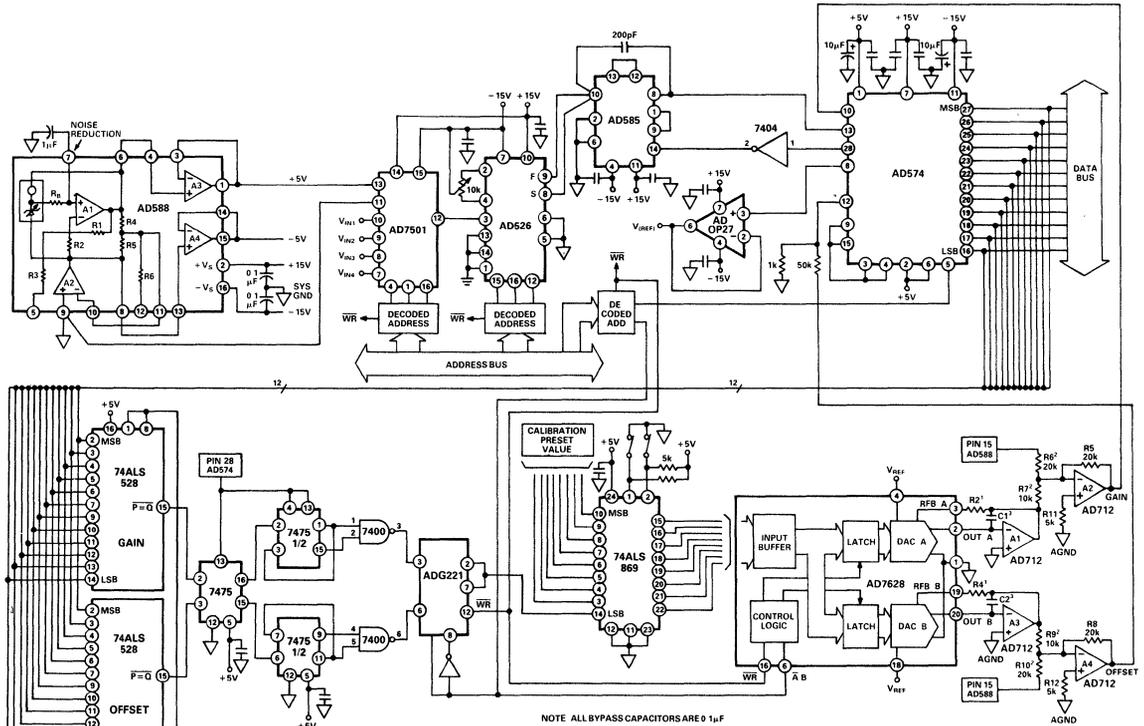
Figure 43. High Accuracy A/D Converter
