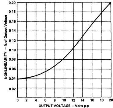
Figure 8. Typical Gain Nonlinearity vs. Output Voltage
