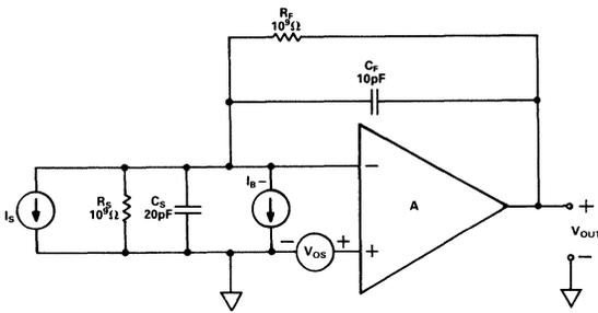
Figure 42. Photodiode Preamp DC Error Sources
