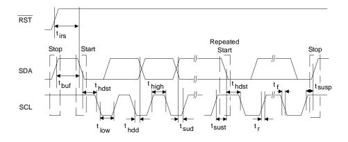
Figure 3. I<sup>2</sup>C Control Port Timing
