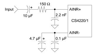
Figure 7. Single-ended Input Application
