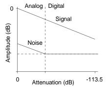
Figure 10. Hybrid Analog/Digital Attenuation
