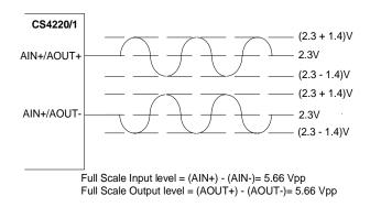
Figure 8. Full Scale Input/Output Voltage
