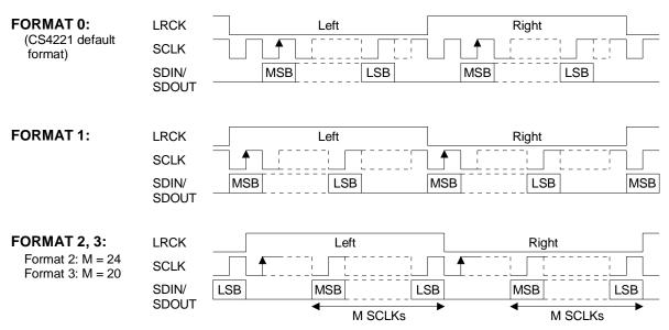
Note: SCLK shown for DSCK = 0. SCLK inverted for DSCK = 1. SCLK must be 64 Fs for Right Justified SDOUT (Formats 2 and 3.) SDIN and SDOUT can be set to different formats through the Control Port in the CS4221.
