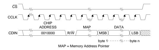
Figure 12. Control Port Timing, SPI mode
