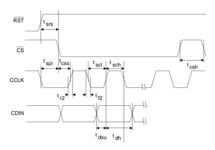
Figure 2. SPI Control Port Timing
