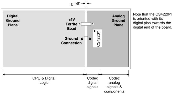
is oriented with its digital pins towards the digital end of the board.
