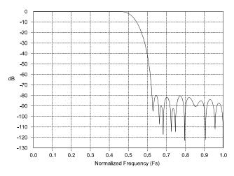
Figure 16. ADC Filter Response
