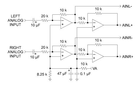
Figure 6. Optional Line Input Buffer
