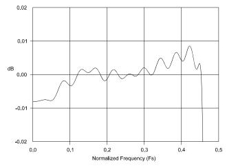
Figure 20. DAC Passband Ripple
