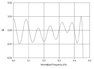
Figure 16. 20-bit ADC Passband Ripple
