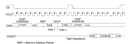
Figure 11. Control Port Timing, SPI Mode
