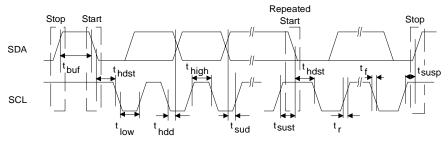
Figure 4. Control Port I<sup>2</sup>C Mode
