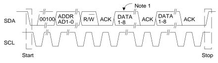
Note 1: If operation is a write, this byte contains the Memory Address Pointer, MAP.
