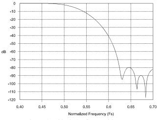
Figure 17. 20-bit ADC Transition Band
