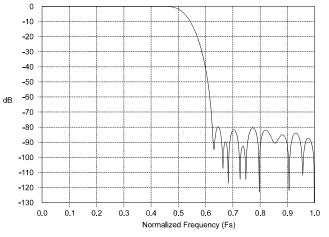
Figure 15. 20-bit ADC Filter Response
