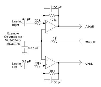
Figure 6. Optional Line Intput Buffer
