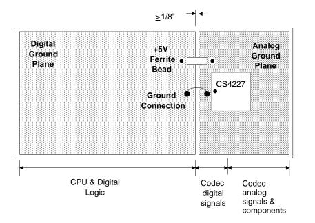
Note that the CS4227 is oriented with its digital pins towards the digital end of the board.
