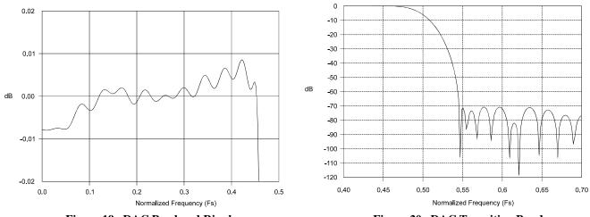
Figure 19. DAC Passband Ripple
