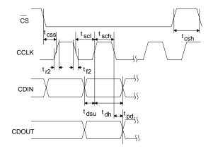
Figure 3. Control Port SPI Mode
