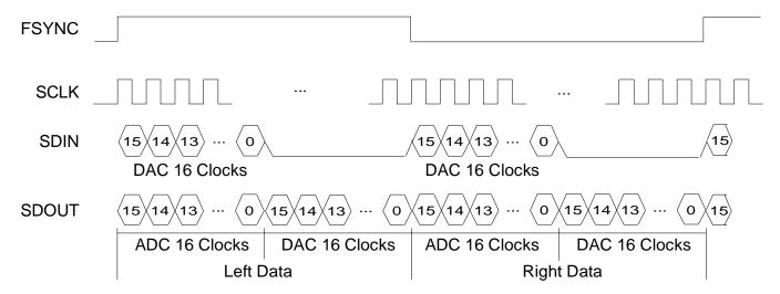
Figure 9. ADC/DAC Mode (SF1,0 = 11)
