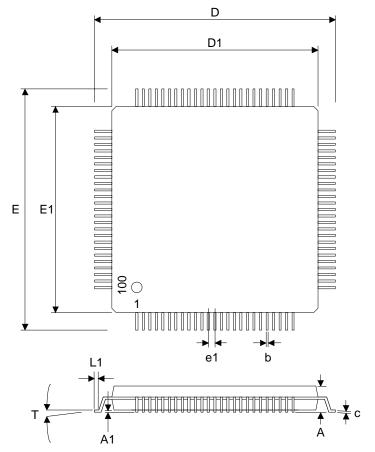
100-pin TQFP - Package Code 'Q'
