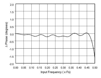
Figure 32. Deviation from Linear Phase
