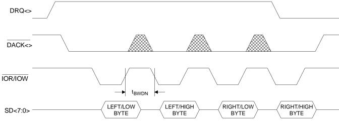
16-Bit Stereo DMA Cycle
