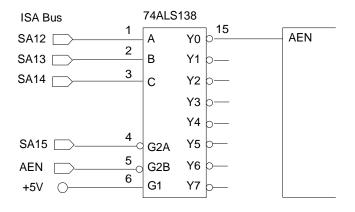
Figure 2. 16-bit Decode Circuit
