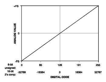
Figure 12. Linear Transfer Functions
