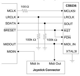
Figure 11. CS9236 Wavetable Serial Port Interface
