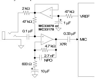
Figure 21. Microphone Input
