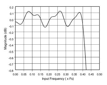
Figure 30. DAC Passband Ripple
