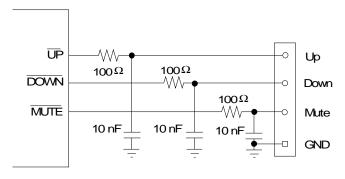
Figure 17. Volume Control Circuit
