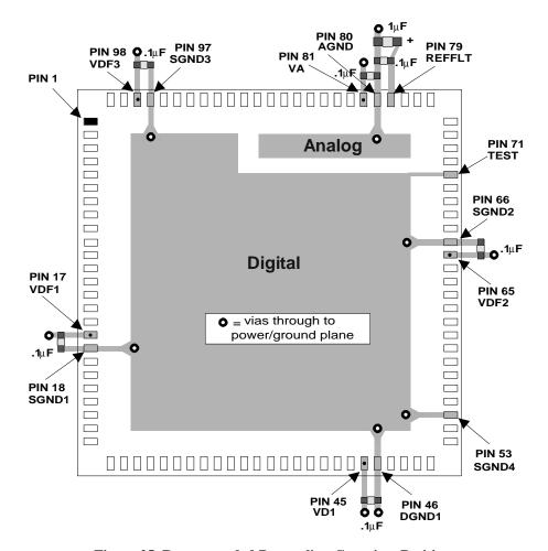
Figure 25. Recommended Decoupling Capacitor Positions
