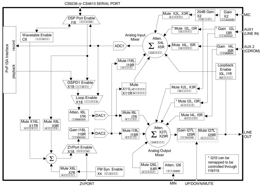
Figure 4. Mixer Block Diagram
