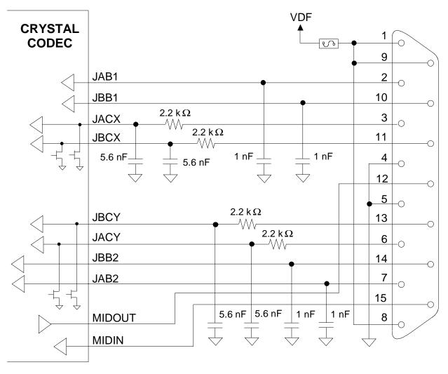
Figure 5. Joystick Logic
