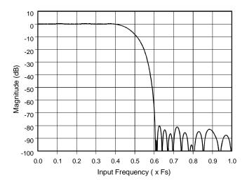
Figure 26. ADC Filter Response
