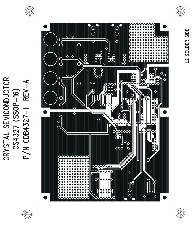
Figure 12. CDB4327 Solder Side (bottom)
