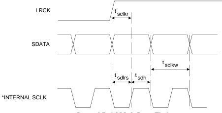
Internal Serial Mode Input Timing.
