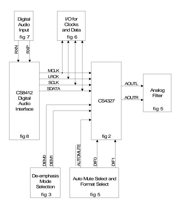
Figure 1. System Block Diagram and Signal Flow
