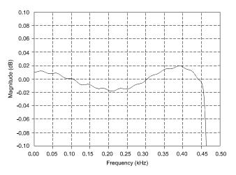
Figure 8. CS4327 Combined digital and Analog Filter Passband Response
