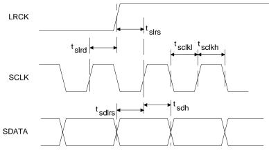
**External Serial Mode Input Timing**
