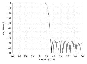
Figure 7. CS4327 Combined Digital and Analog Filter Stopband Rejection
