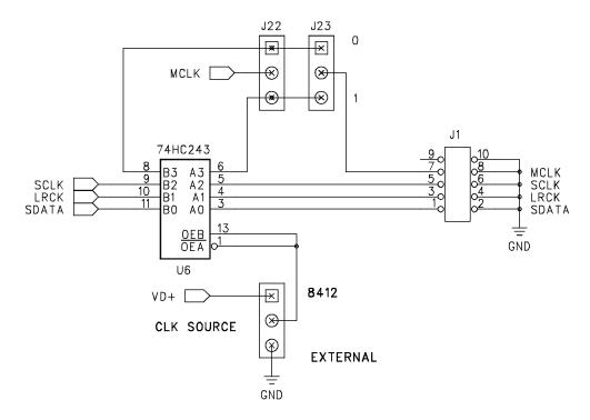
Figure 6. I/O Interface for Clocks and Data
