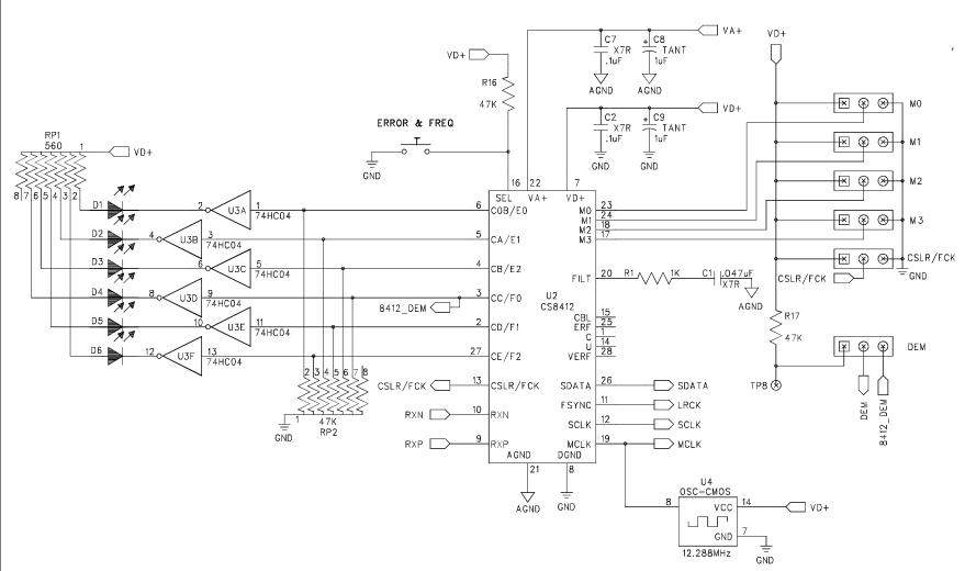
Note: U2 and U4 can not be installed simultaneously
