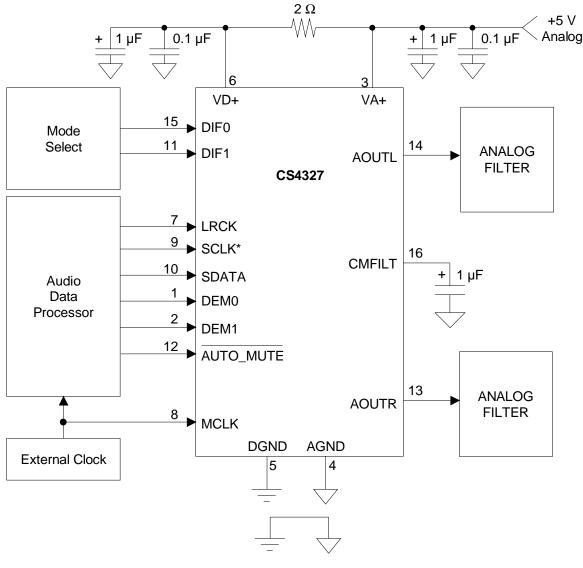
\* SCLK must be connected to DGND for operation in Internal SCLK Mode
