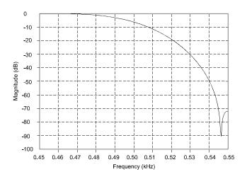
Figure 9. CS4327 Combined Digital and Analog Filter Transition Band
