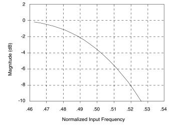
Figure 5. CS5330A/31A Digital Filter Stopband Rejection
