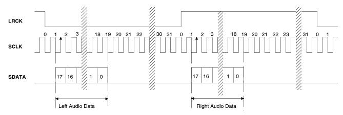
Figure 3. Data Output Timing - CS5331A (I<sup>2</sup>S compatible)
