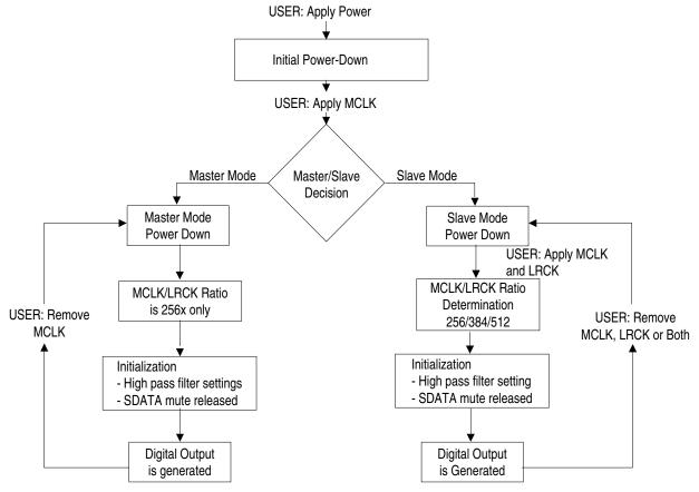
Figure 4. CS5330A/31A Initialization and Power-Down Sequence
