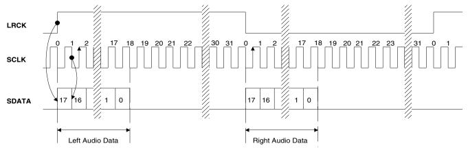
Figure 2. Data Output Timing-CS5330A
