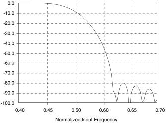
Figure 7. CS5330A/31A Digital Filter Passband Ripple
