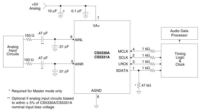
Figure 1. Typical Connection Diagram
