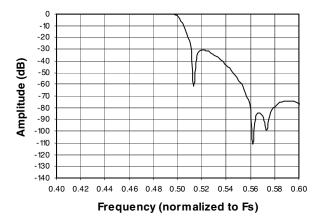
Figure 5. Double Speed Mode Stopband Rejection Figure 6. Double Speed Mode Stopband Rejection
