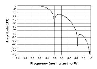
Figure 9. Quad Speed Mode Stopband Rejection
