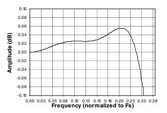
Figure 12. Quad Speed Mode Passband Ripple
