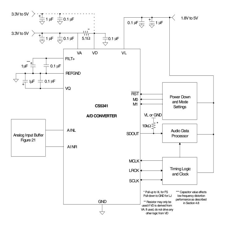
Figure 17. Typical Connection Diagram
