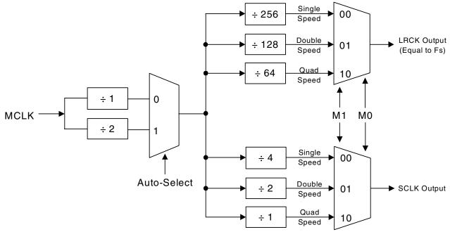
Figure 18. CS5341 Master Mode Clocking
