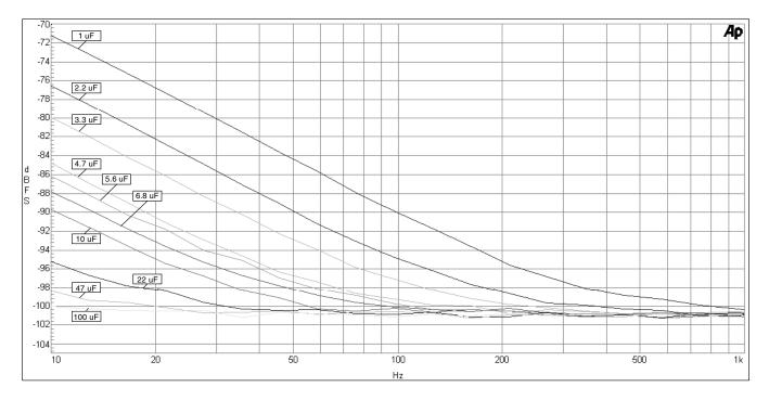
Figure 22. CS5341 THD+N versus Frequency
