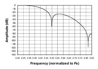
Figure 10. Quad Speed Mode Stopband Rejection
