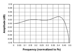
Figure 4. Single Speed Mode Passband Ripple
