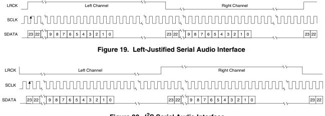
Figure 20. I<sup>2</sup>S Serial Audio Interface
