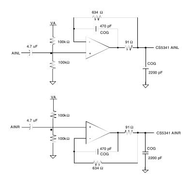
Figure 21. CS5341 Recommended Analog Input Buffer
