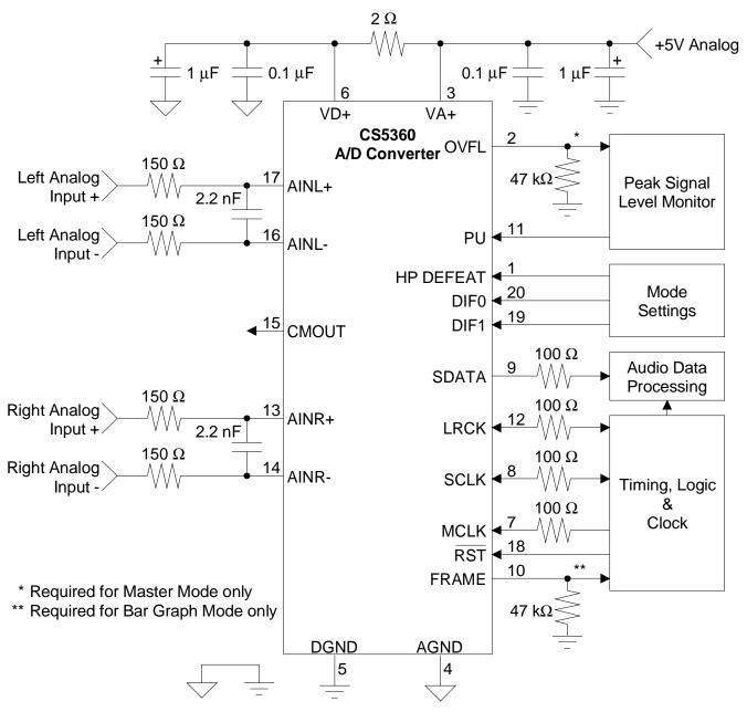
Figure 1. Typical Connection Diagram
