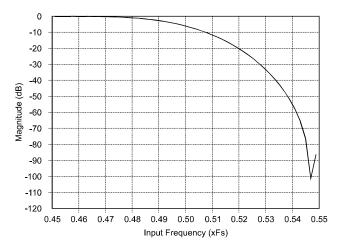
Figure 10. CS5360 Digital Filter Transition Band
