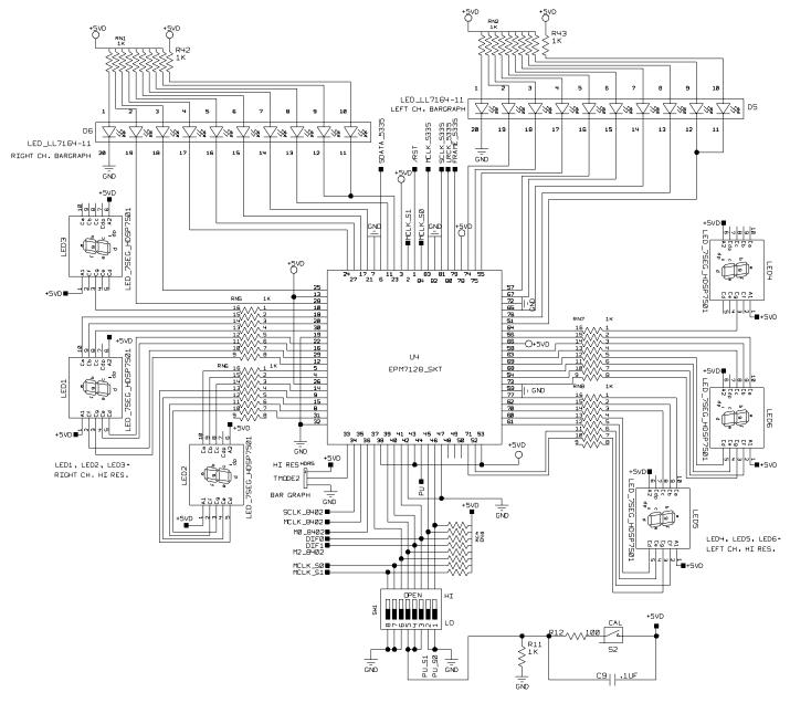
Figure 8. Altera PLD and Display LEDs
