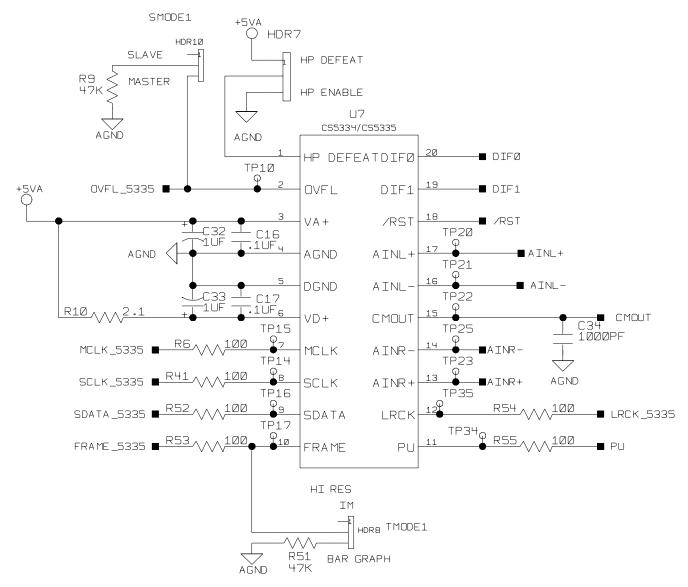
Figure 4. CS5334, CS5335, and CS5360 Connections
