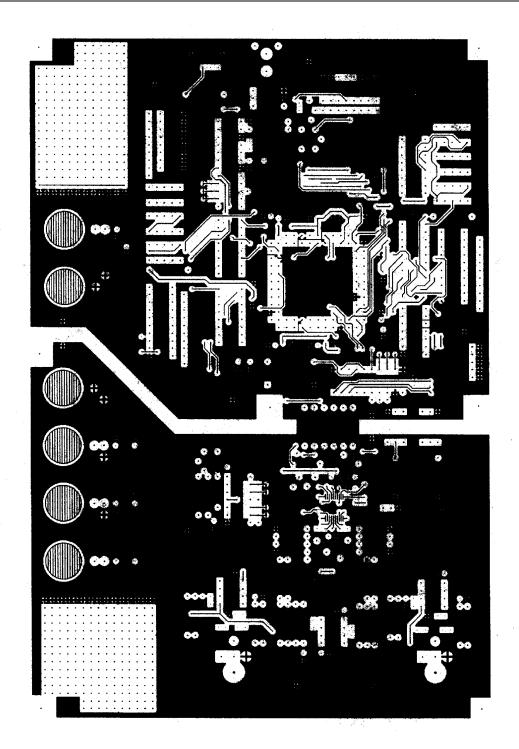
Figure 11. CDB5334/35/60 Solder side (bottom)
