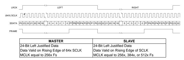
Figure 3. Serial Data Format 0
