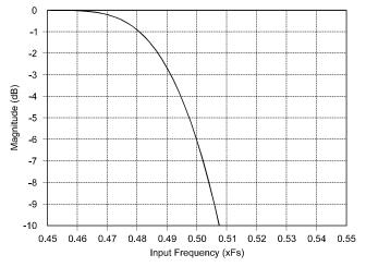
Figure 8. CS5360 Digital Filter Transition Band
