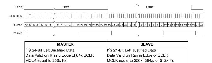
Figure 5. Serial Data Format 2
