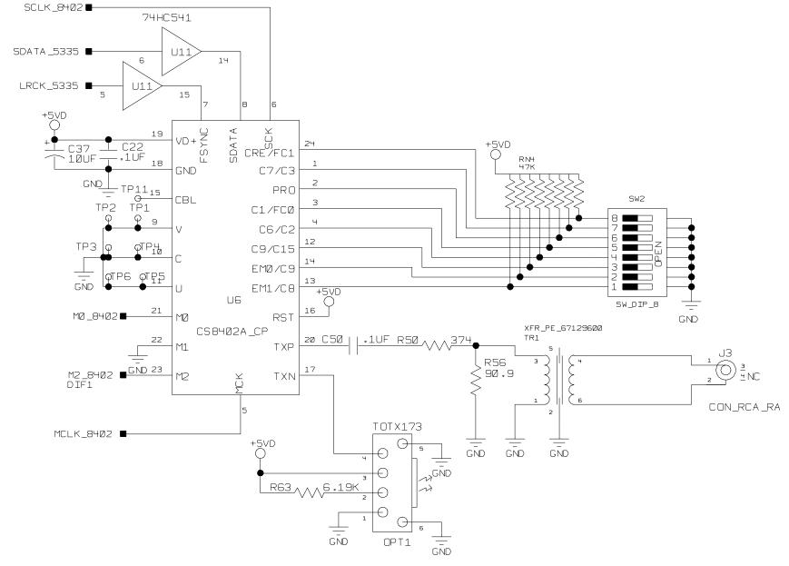
Figure 5. CS8402A Digital Audio Trnamitter and Connections
