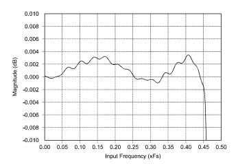
Figure 9. CS5360 Digital Filter Passband Ripple
