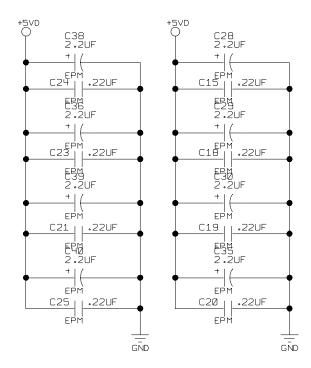
Figure 7. Decoupling Caps for PLD
