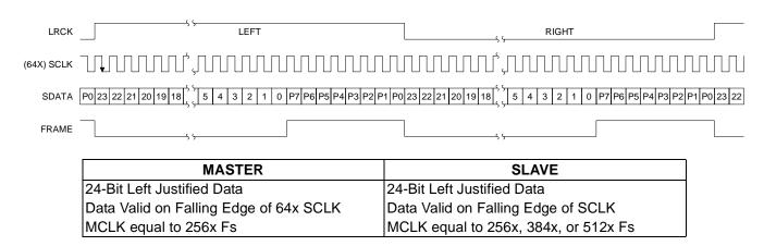
Figure 4. Serial Data Format 1
