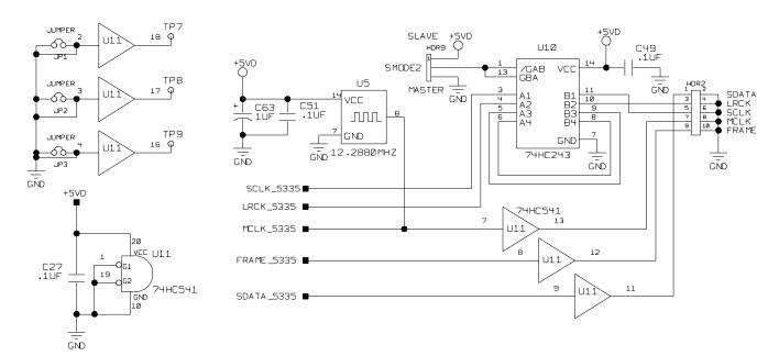
Figure 6. I/O Interface for Clocks and Data
