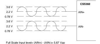
Figure 6. Full Scale Input Levels
