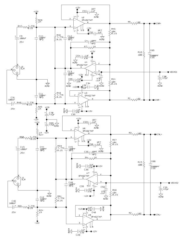
Figure 4. Analog Input Buffer
