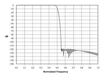
Figure 5. CS5394 Stopband Attenuation
