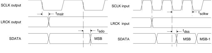
SCLK to SDATA & LRCK - MASTER mode Serial Data Format, DFS high I<sup>2</sup>S compatible
