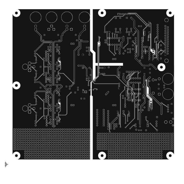
BOTTOM SIDE Figure 12. CDB5394 and CDB5396/7 Component Copper Side (bottom)
