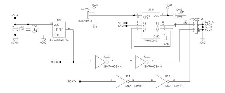
Figure 6. I/O Interface for Clocks & Data
