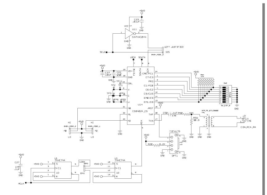
Figure 3. CS8404A Digital Audio Transmitter and Connections
