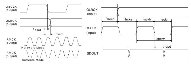
Figure 1. Audio Port Master Mode Timing
