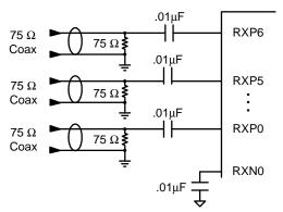
Figure 13. Consumer Input Circuit
