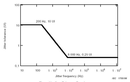
Figure 20. Jitter Tolerance Template
