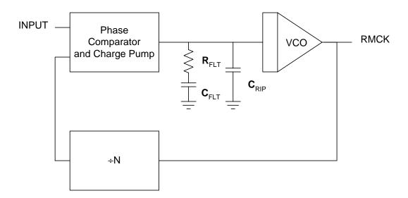
Figure 18. PLL Block Diagram
