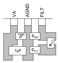
Figure 19. Recommended Layout Example
