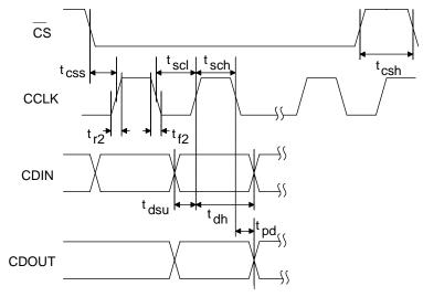
Figure 3. SPI Mode Timing
