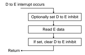
Figure 17. Flowchart for Reading the E Buffer
