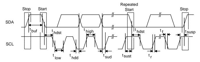
Figure 4. I<sup>2</sup>C Mode Timing
