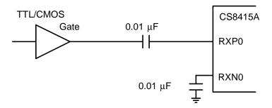
Figure 15. TTL/CMOS Input Circuit
