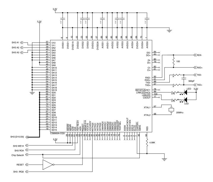
Figure 5. CS8900A Interface to Hitachi SH3
