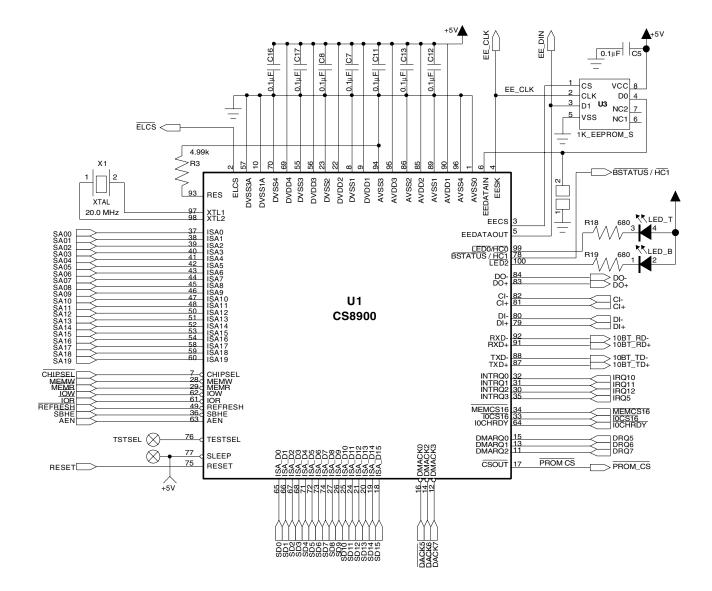
Figure 13. CS8900A Schematic (Combo Card Application)
