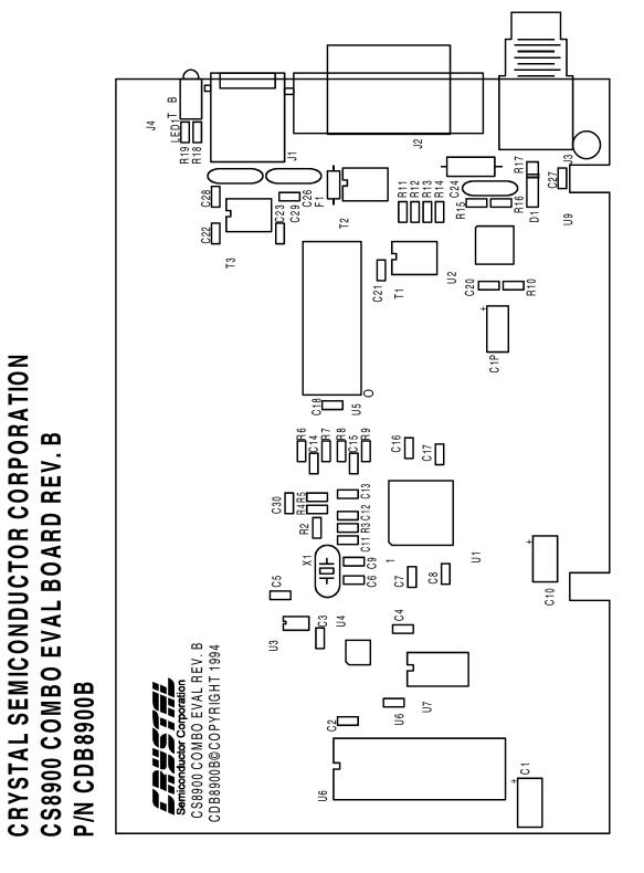
Figure 12. Placement of Components
