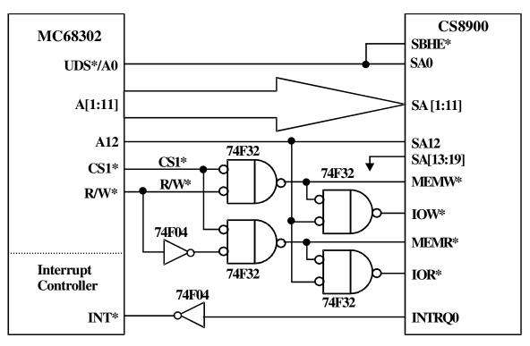
Figure 3. Connection of CS8900A to MC68302
