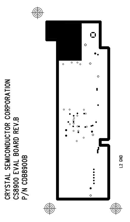
Figure 29. Ground Plane of four-layer board
