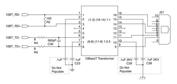
Figure 8. 10BASE-T Schematic 3.3V
