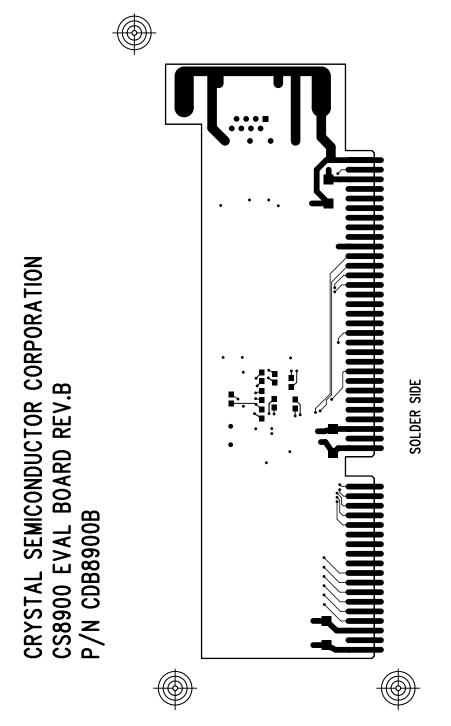
Figure 30. Solder side (bottom) of four-layer board
