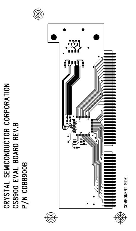
Figure 27. Component (top) side of four-layer board
