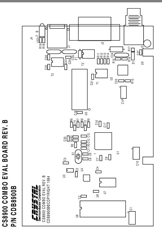
Figure 24. General placement on an ISA adapter card
