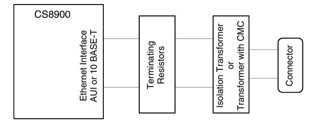
Figure 22. Typical CS8900A Ethernet Connection
