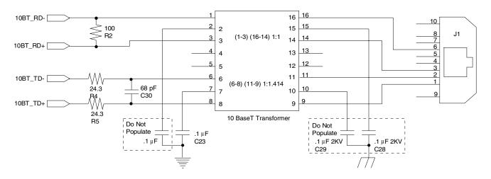
Figure 10. 10BASE-T Schematic 5V
