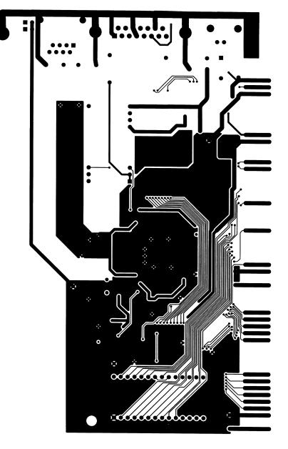
Figure 20. CRD8900 Bottom Side Routing
