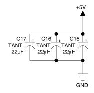
Figure 11. Decoupling Capacitors Schematic
