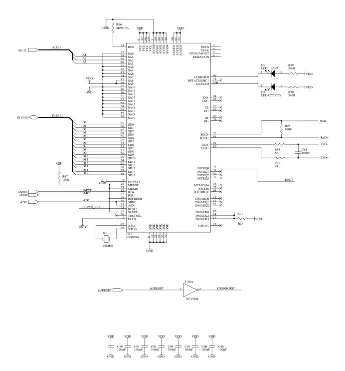
Figure 4. CS8900A Interface to Cirrus Logic CL-PS7211
