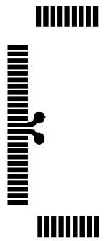
Figure 32. Routing of Decoupling Capacitor (Top side, component side)
