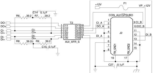
Figure 16. AUI Schematic
