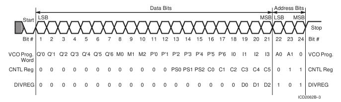
Figure 4. Serial Data Timing
