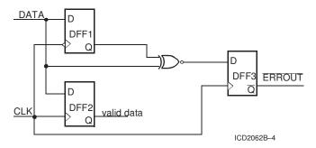
Figure 5. Modified Manchester Decoder Circuit
