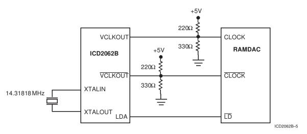
Figure 6. ICD2062B to RAMDAC Interface Example
