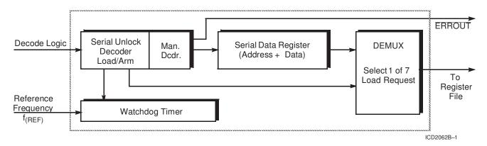
Figure 2. Serial Programming Block Diagram—Detail
