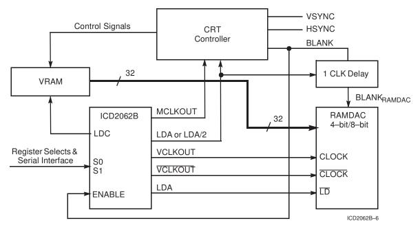
Figure 7. ICD2062B Typical Interface Circuit
