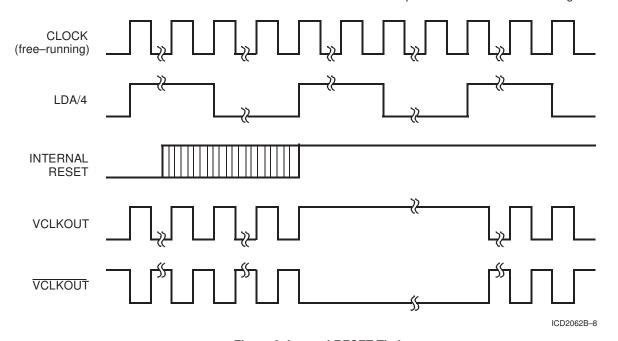
Figure 9. Internal RESET Timing
