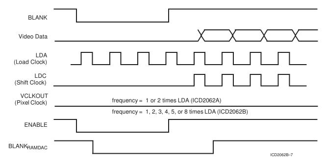
Figure 8. Timing Diagram for Interface Circuit
