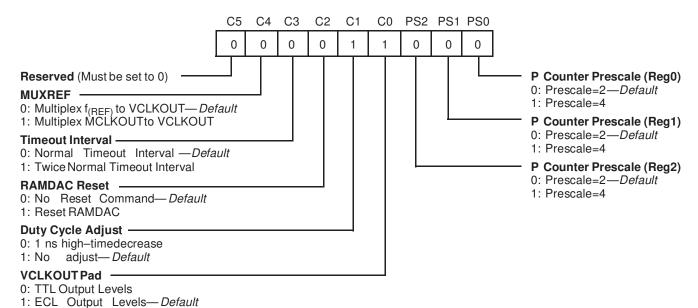
Figure 1. Control Register Definition
