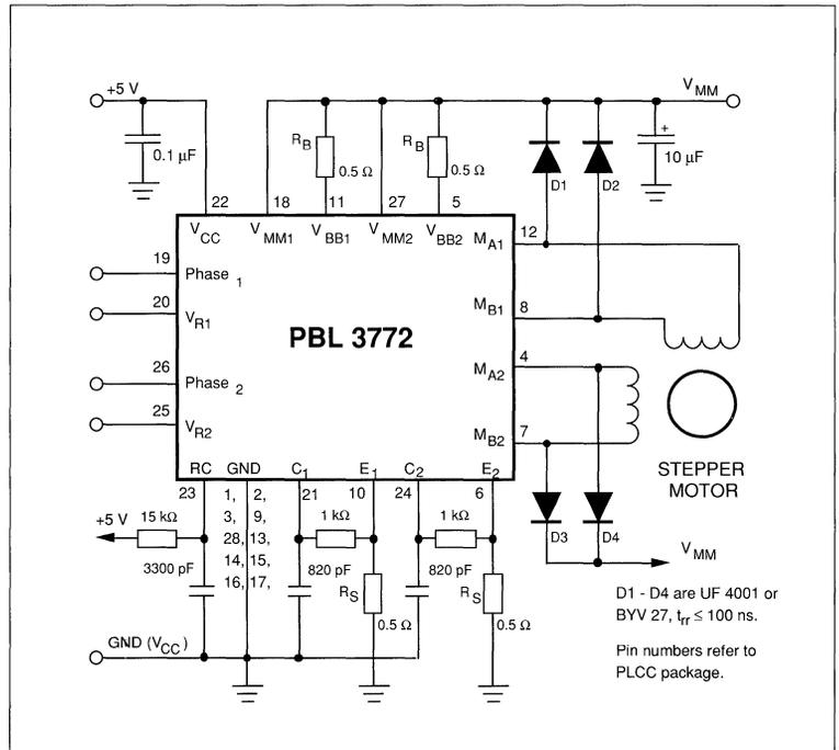
Figure 6. Typical stepper motor driver application with PBL 3772.
