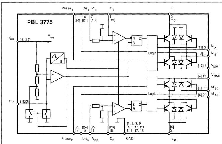
Figure 1. Block diagram.
