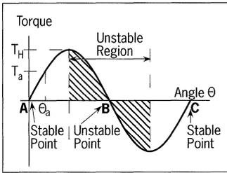
Figure 4. Torque vs. rotor angular position.
