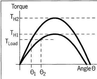
Figure 5. Torque vs. rotor angle position at different holding torque.
