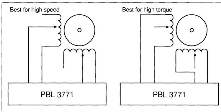
Figure 11. Connection of unipolar motors.
