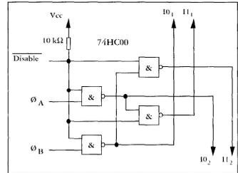
Figure 1. Logic circuit which, when added to design in figure 3, allows it to perform modified-half-step driving.
