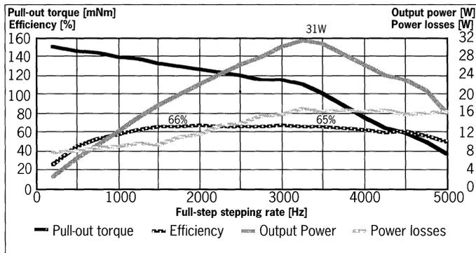
Figure 8. Performance curves for a 2.8ohm bipolar 57mm hybrid stepper (length 42mm) driven by PBL3770A constant-current driver (Chopper voltage 40V, winding current 750mA).
