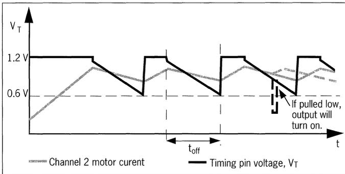
Figure 4. Motor current and  $V_T$  voltage vs. time.
