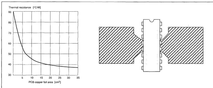
Figure 15. Copper foil used as a heatsink.
