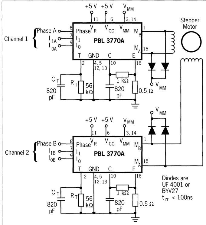
Figure 1. Typical stepper motor driver application with PBL 3770A.
