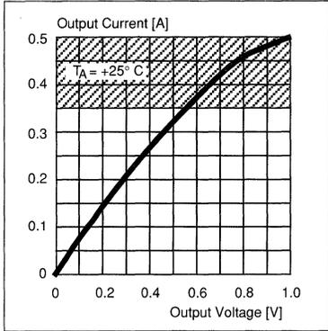
Figure 6. Typical  $I_p$  vs.  $V_{PCE Sat}$  Phase output saturation.
