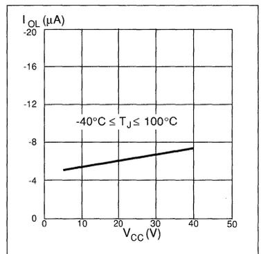
Figure 12. Output leakage current vs. supply voltage.  $0 \text{ V} \leq V_{in} \leq 0.8 \text{ V}$ . Output = 0 V.
