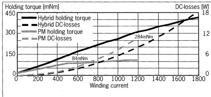
Figure 9. Holding torque and DC-loss as functions of winding currents for a 57mm PM motor and for a 57mm hybrid motor.
