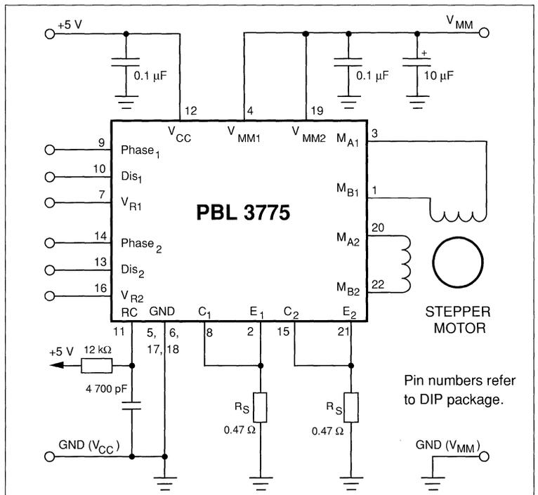
Figure 6. Typical stepper motor driver application with PBL 3775.
