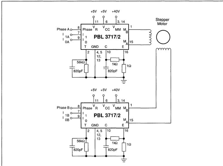
Figure 8. Typical stepper motor driver application with PBL 3717/2.
