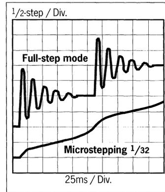
Figure 4. Rotor position as function of stepping mode.
