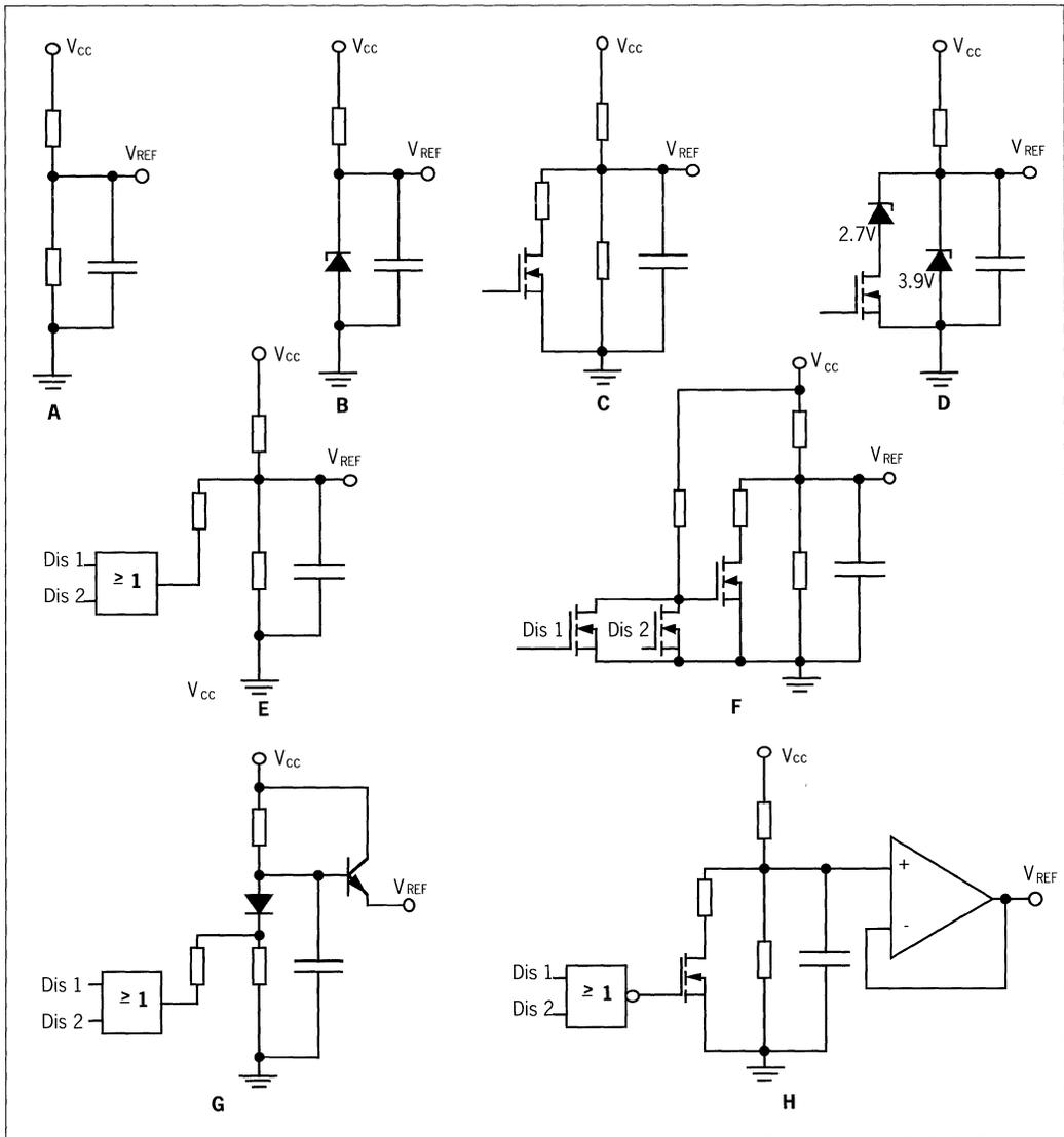
Figure 13. Examples of different voltage reference circuits.
