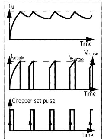
Figure 12. Current waveform in the basic chopper circuit.
