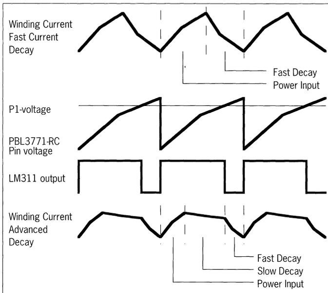
Figure 2. TB307i advanced current decay control.
