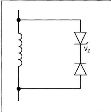
Figure 23. Zener diode turn-off circuit.
