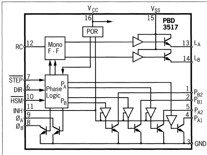
Figure 12. PBD 3517 block diagram.
