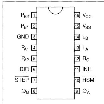
Figure 13. Pin configuration.
