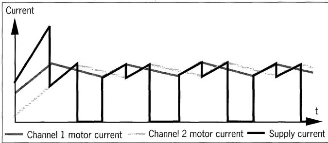
Figure 3. Timing diagram with two channels during synchronized operation.
