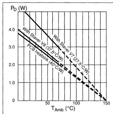
Figure 13. Allowable power dissipation vs. ambient temperature.
