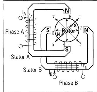
Figure 1. Two phase stepper motor
