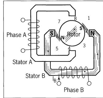
Figure 2. Magnetic flux path through a two-pole stepper motor with a lag between the rotor and stator.
