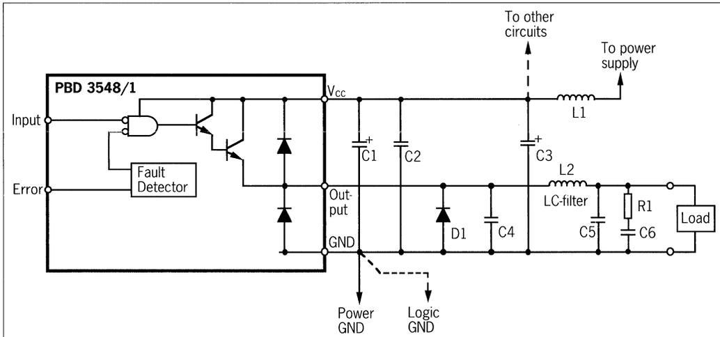
Figure 4. Circuit diagram showing worst case filtering arrangement for suppression of transients.
