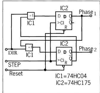
Figure 10. Two direction TTL full step generator.
