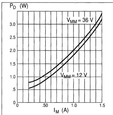
Figure 12. Typical power dissipation vs. motor current.
