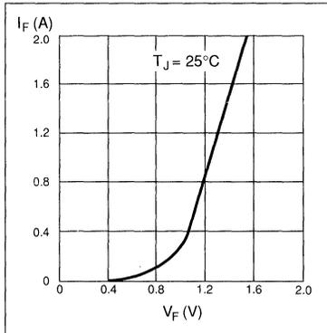
Figure 8. Diode forward voltage drop vs. forward current.
