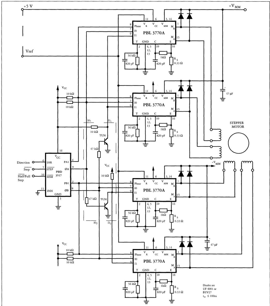
Figure 3. High-current design (2.5 A/Phase) using four PBL 3770A.
