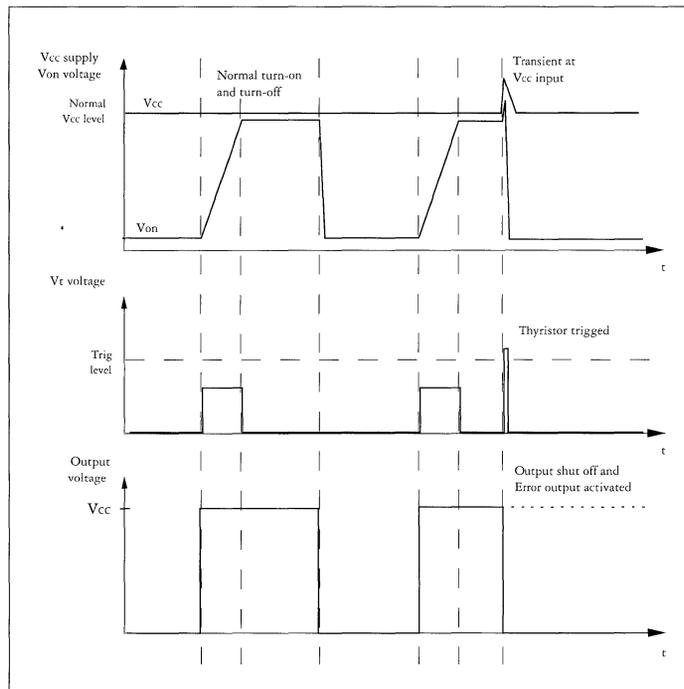
Figure 2. Waveforms at normal operation and at transient turn-off.
