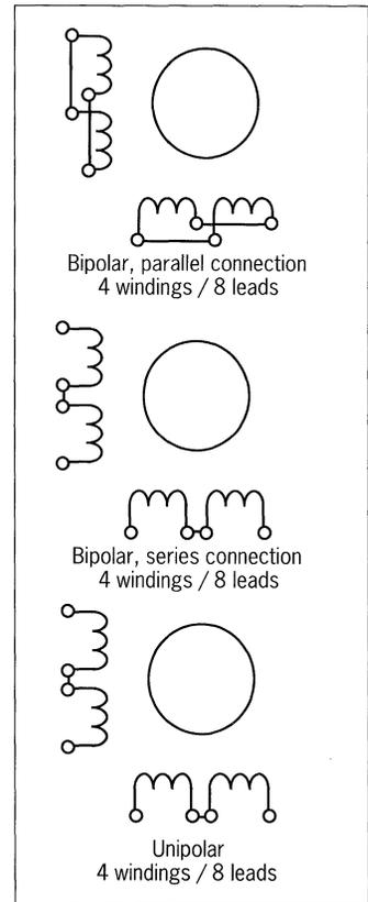
Figure 8. Different winding configurations for bipolar and unipolar drive using an 8-lead motor.
