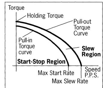
Figure 7. Torque vs. speed characteristics of a stepper motor.
