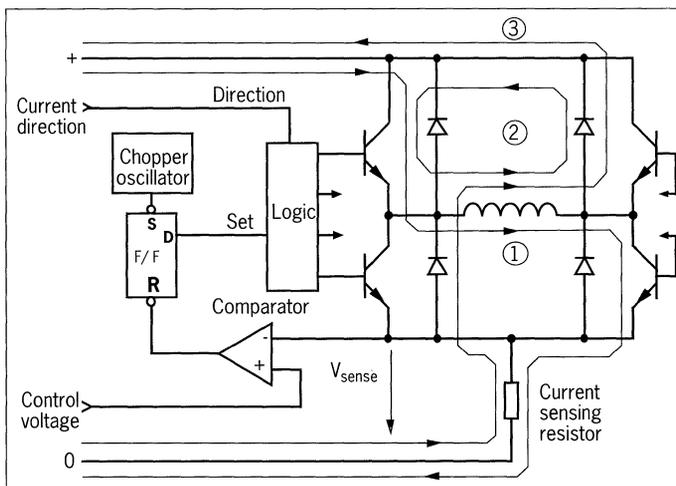
Figure 13. An H-bridge configured as a constant current chopper.
