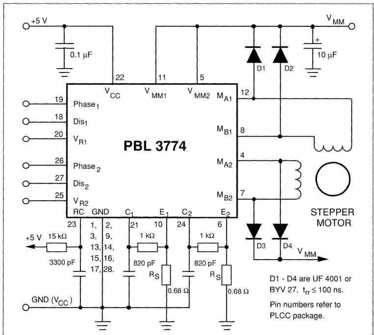
Figure 6. Typical stepper motor driver application with PBL 3774.
