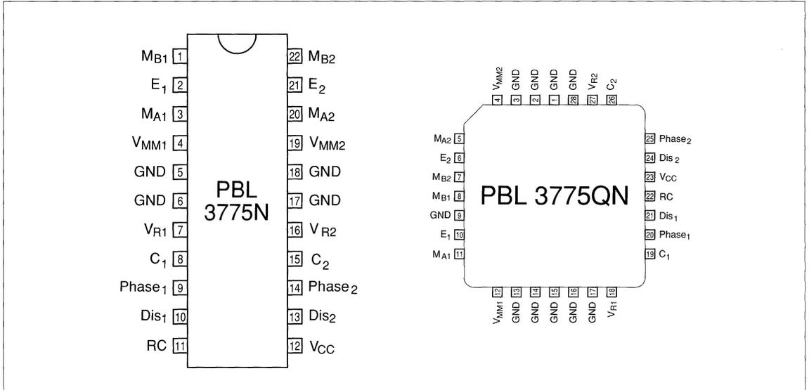
Figure 4. Pin configuration.
