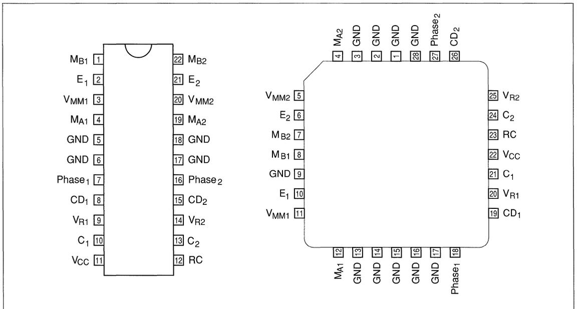
Figure 3. Pin configuration.
