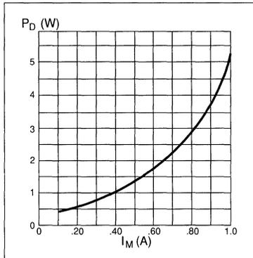
Figure 13. Typical power dissipation vs. motor current.
