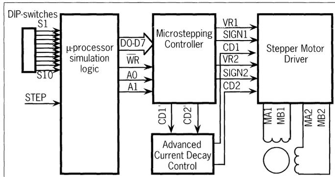
Figure 1. TB370I block diagram.
