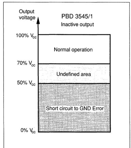
Figure 6. Error state vs. output voltage, inactive output ( $0 \text{ V} \leq V_{IN} \leq 0.8 \text{ V}$ ),  $5 \text{ V} \leq V_{CC} \leq 40 \text{ V}$ ,  $-40^\circ \text{C} < T_J < +100^\circ \text{C}$ .
