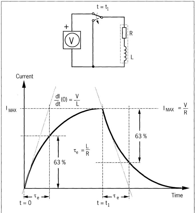
Figure 2. Current wave form in an inductive-resistive circuit.
