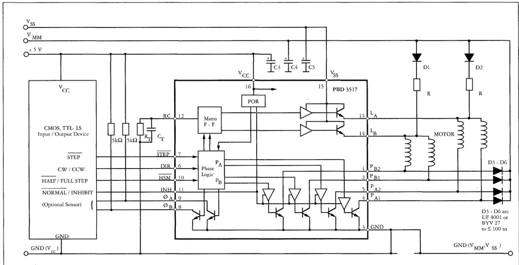
Figure 1. Typical unipolar stepper motor drive application with PBD 3517.
