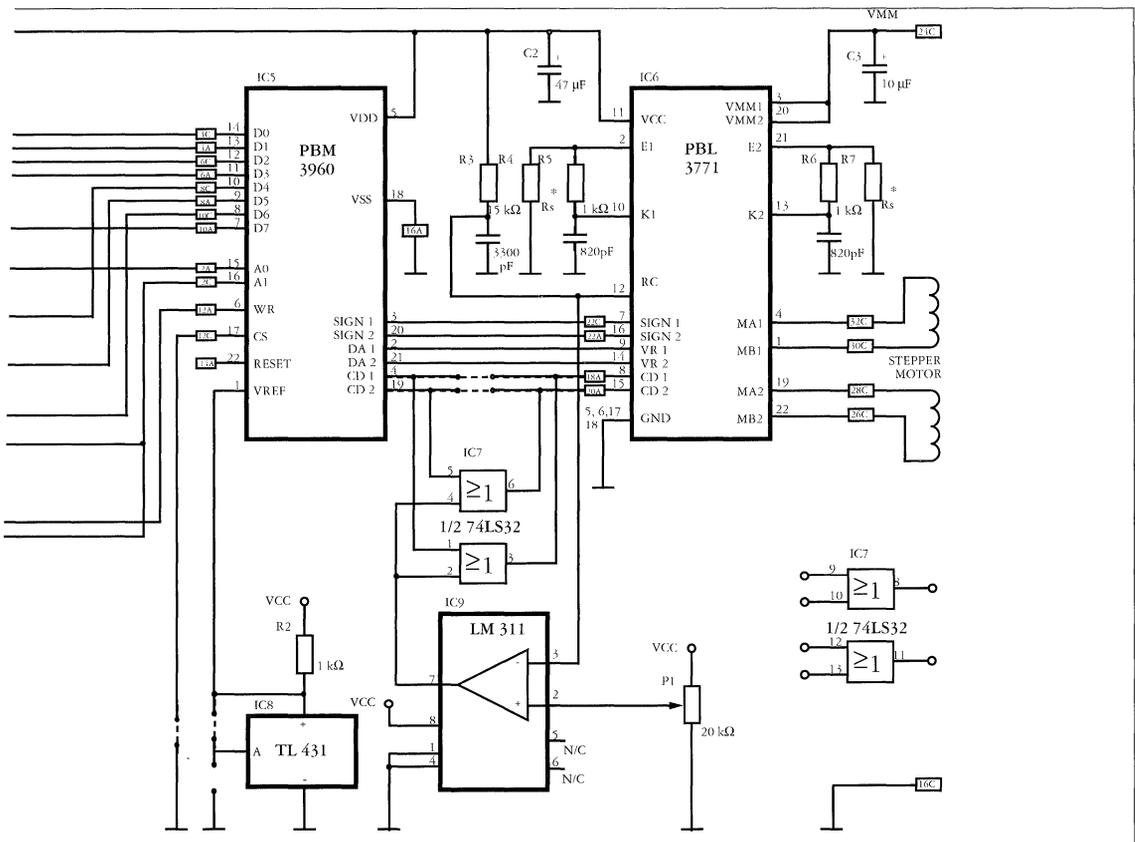
When fast current decay is selected then the driver connects the winding in opposition to the power supply. In this case the excessive energy in the winding and rotor is quickly removed thus eliminating the current dragging. But, if too much energy is removed the winding current ripple will increase. This will cause switching noise, increased power losses, current wave form distortion and in some cases also increased resonances.
