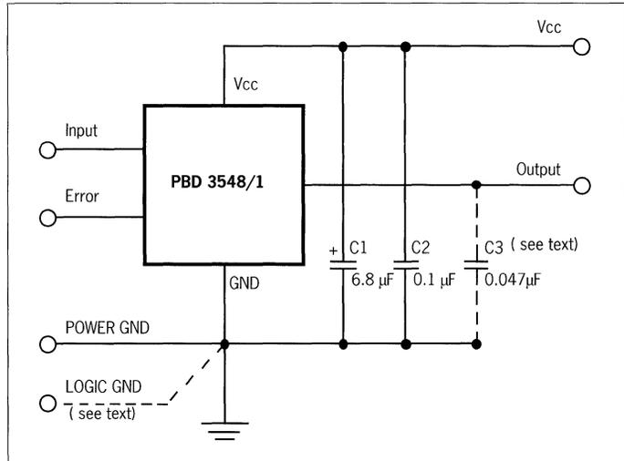
Figure 1. Basic decoupling in a typical application.
