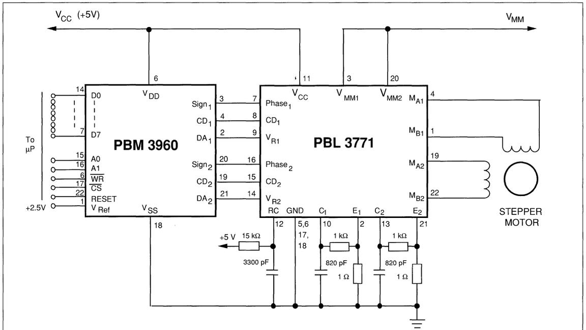
Figure 4. Microstepping system with PBM 3960 and PBL 3771.
