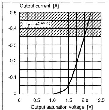
Figure 4. Typical  $I_L$  vs.  $V_{LCE Sat}$ . Second level output saturation.
