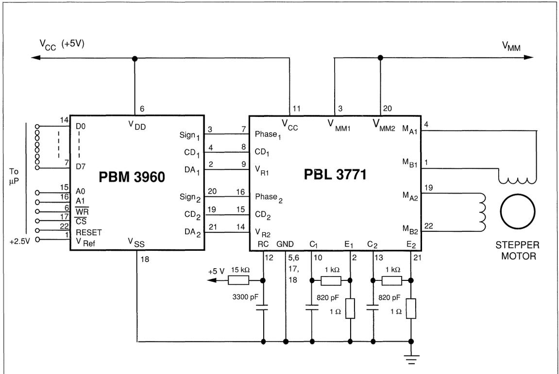
Figure 14. Typical application in a microprocessor based system.
