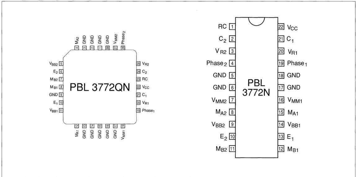
Figure 4. Pin configuration.
