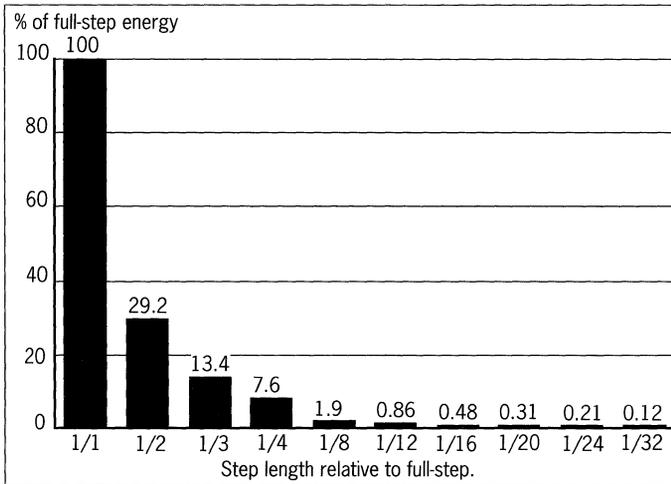
Figure 3. Relative excitation energy as function of electrical step length.
