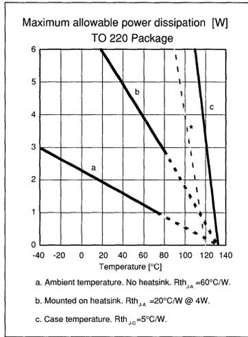
Figure 21. Maximum allowable power dissipation. TO 220 package.
