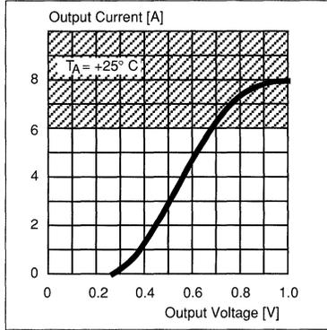
Figure 7. Typical  $I_o$  vs.  $V_{OCE Sat}$  "Zero output" saturation.
