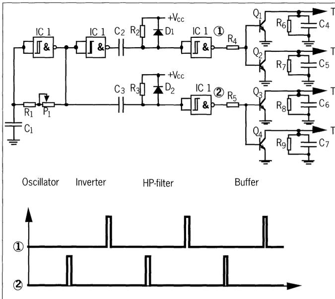
Figure 2. Oscillator circuitry used to synchronize current switching in the design in figure 3 and its output signals.
