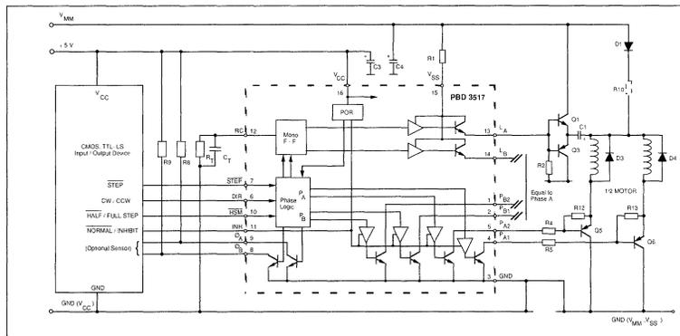
Figure 15. Voltage doubling with external transistors.
