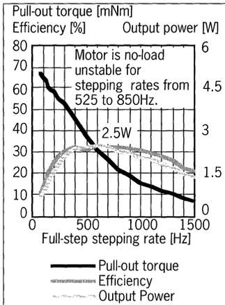
Figure 4. Performance curves for a 100ohm unipolar 57mm PM-motor driven by a 40/20V Bi-level constant-voltage driver (High-voltage-on time = 4ms).
