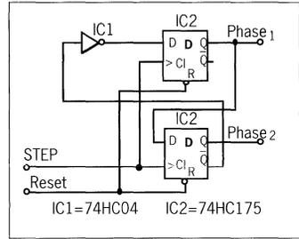
Figure 9. One direction TTL full step generator.
