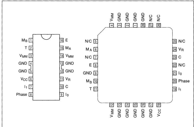
Figure 4. Pin configurations.
