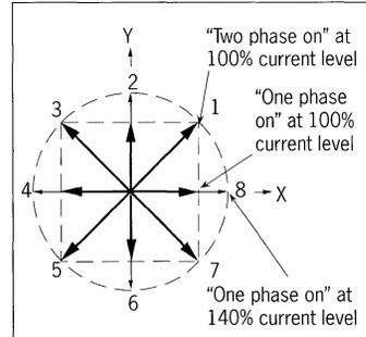
Figure 2. Direction and amplitude of the magnetic field.
