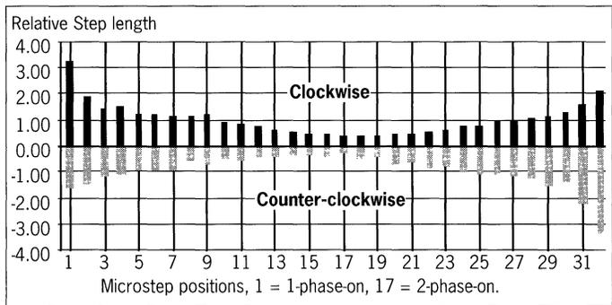
Figure 7. 57mm PM-stepper relative microstep lengths as function of stop position, 1/32-full-step mode.
