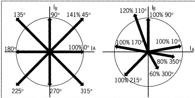
Figure 2. (A)—flux directions for normal half and full-step stop positions. Length is proportional to holding torque. (B)—microstepping flux directions. Direction and length are variable.
