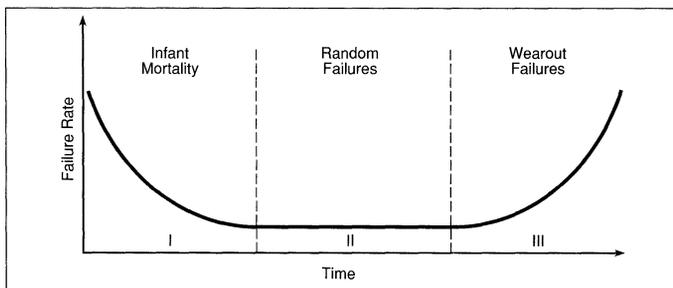
Figure 9. Failure rate distribution, "bathtub" curve.
