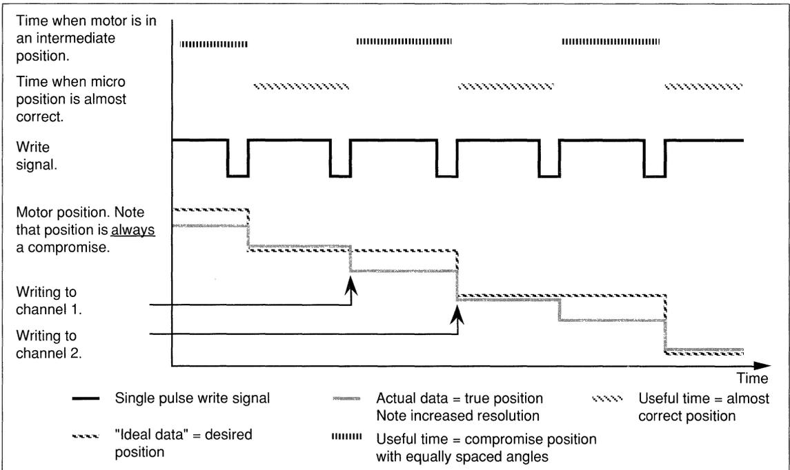
Figure 12. Single pulse programming, in- and output signals.
