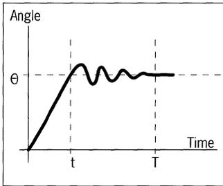
Figure 8. Single step response vs. time.
