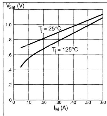
Figure 10. Typical sink saturation voltage vs. output current.
