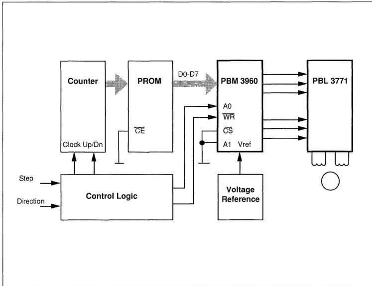
Figure 13. Typical block diagram of an application without a microprocessor. Available as testboard, TB 307i.
