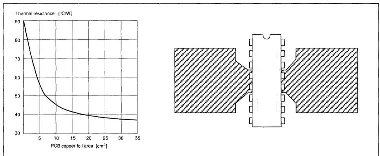
Figure 16. Copper foil used as a heatsink.
