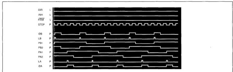
Figure 19. Half-step mode, reverse. 8-step sequence.
