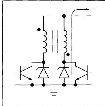
Figure 24. Power return turn-off circuit.
