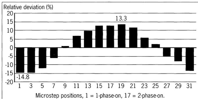
Figure 8. Microstepping holding torque ripple for a 57mm PM stepper. Ripple = 13.3 - -14.8 = 28.1%.
