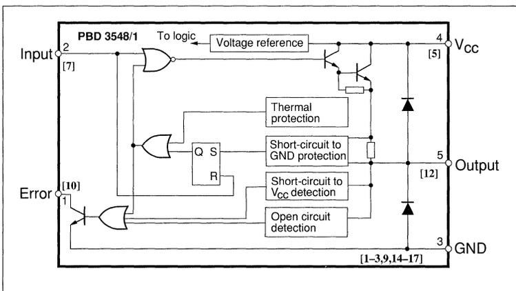
Figure 1. Block Diagram. Pin number in brackets refer to PLCC package.
