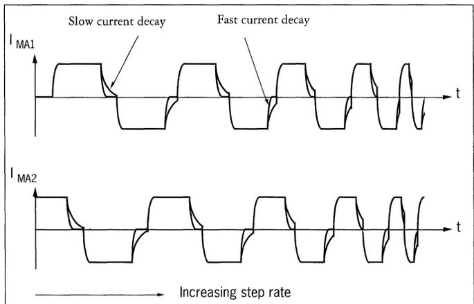
through the non-energized coil should be brought to zero as quickly as possible. Often fast current decay will result in a reduction of the vibrations and resonances. But the performance achieved is very much dependent on the application (mechanical damping, the lag between the rotor position and the magnetic field and so on). Fast current decay will “tighten up” the control of the magnetic field versus the input phase.
