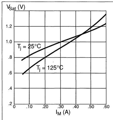
Figure 8. Typical source saturation voltage vs. output current.
