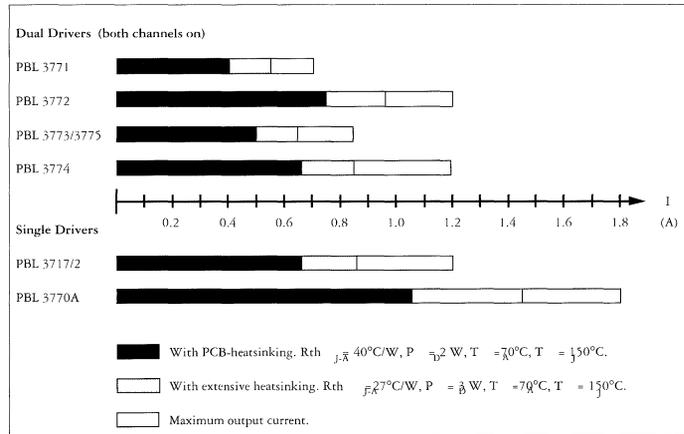
Figure 2. Output current capability for Ericsson's stepper motor driver ICs.
