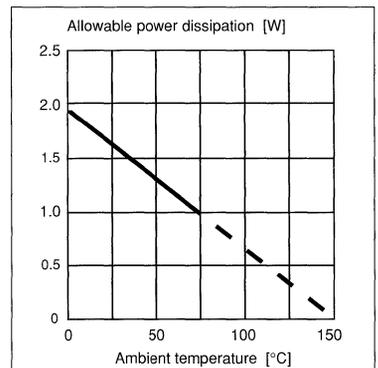
Figure 5. Typical  $P_D$  vs.  $T_a$ . Total power dissipation.
