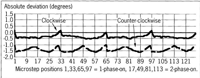
Figure 13. Sine/cosine CW compensated microstepping position ripple for 4 full-step cycles for a 57mm 7.5 degree PM stepper
