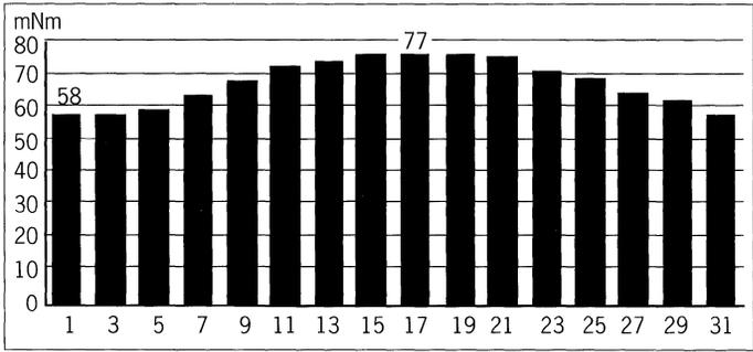
Figure 12. Microstepping holding torque for a 57mm PM stepper.
