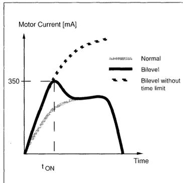
Figure 12. Motor current  $I_p$ .
