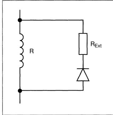
Figure 22. Resistance turn-off circuit.
