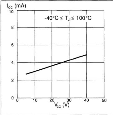
Figure 7. Current consumption vs. supply voltage at  $2\text{ V} \leq V_{in} \leq V_{cc}\text{ V}$ .
