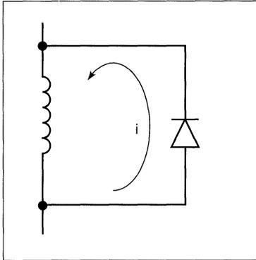
Figure 21. Diode turn-off circuit.
