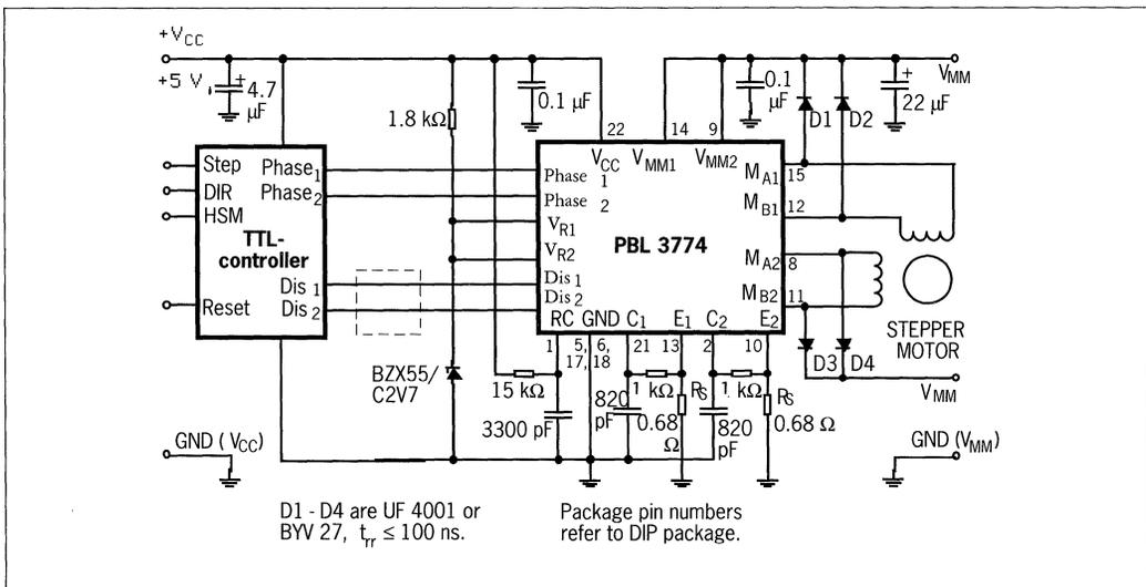
Figure 16. Typical application using a TTL controller and PBL 3774.
