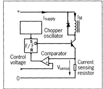
Figure 11. A simplified schematic shows the principle of constant current chopper regulation.
