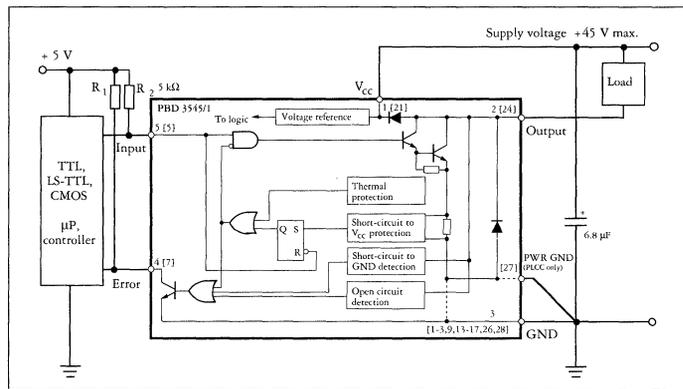
Figure 9. Block diagram and typical application of the PBD 3545/1 Sink Driver.
