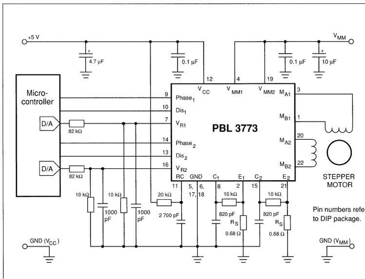
Figure 7. Microstepping system where a microcontroller including DACs provides analog current control voltages as well as digital signals to the PBL 3773.
