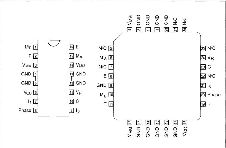
Figure 4. Pin configurations.
