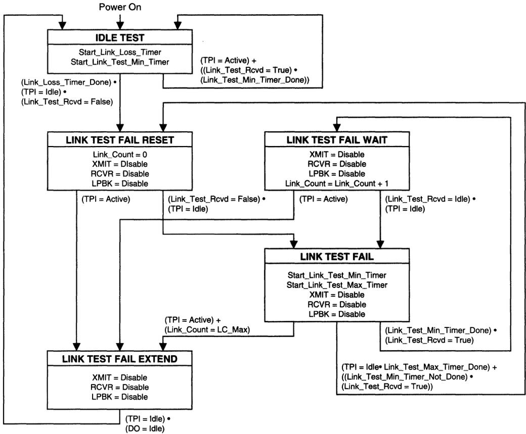
Figure 12. Link Integrity Test Function
