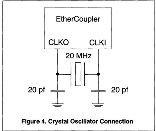
**Figure 4. Crystal Oscillator Connection**
