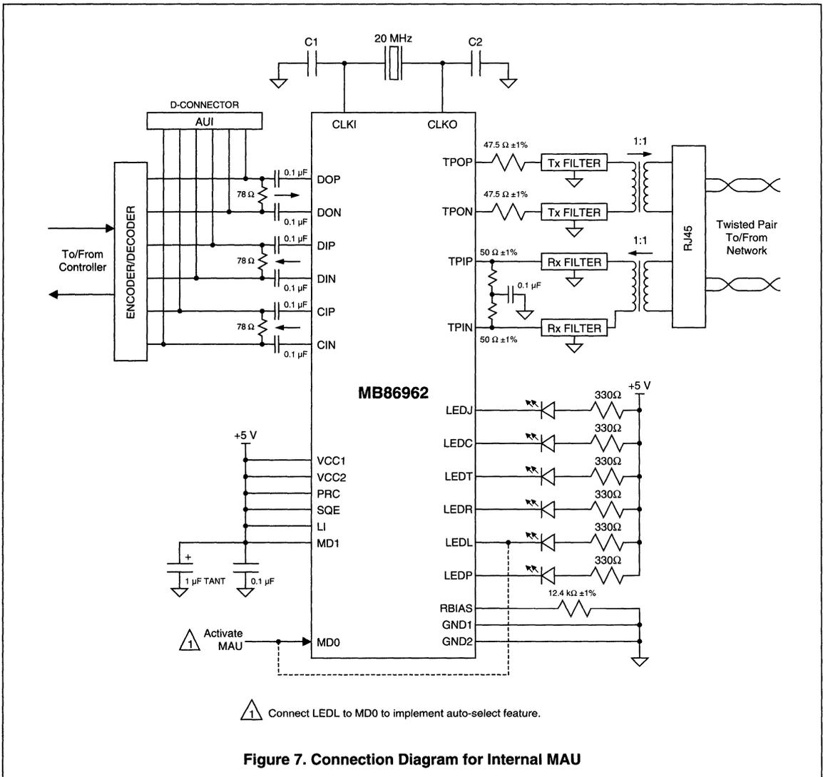
Figure 7. Connection Diagram for Internal MAU
