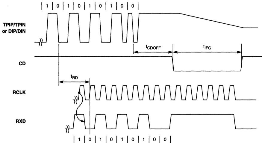
Note: RXD changes at the falling edge of RCLK. The controller is sampled at the rising edge.
