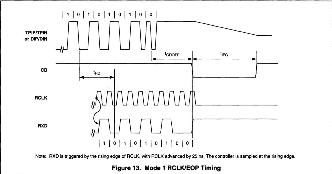
**Figure 13. Mode 1 RCLK/EOP Timing**
