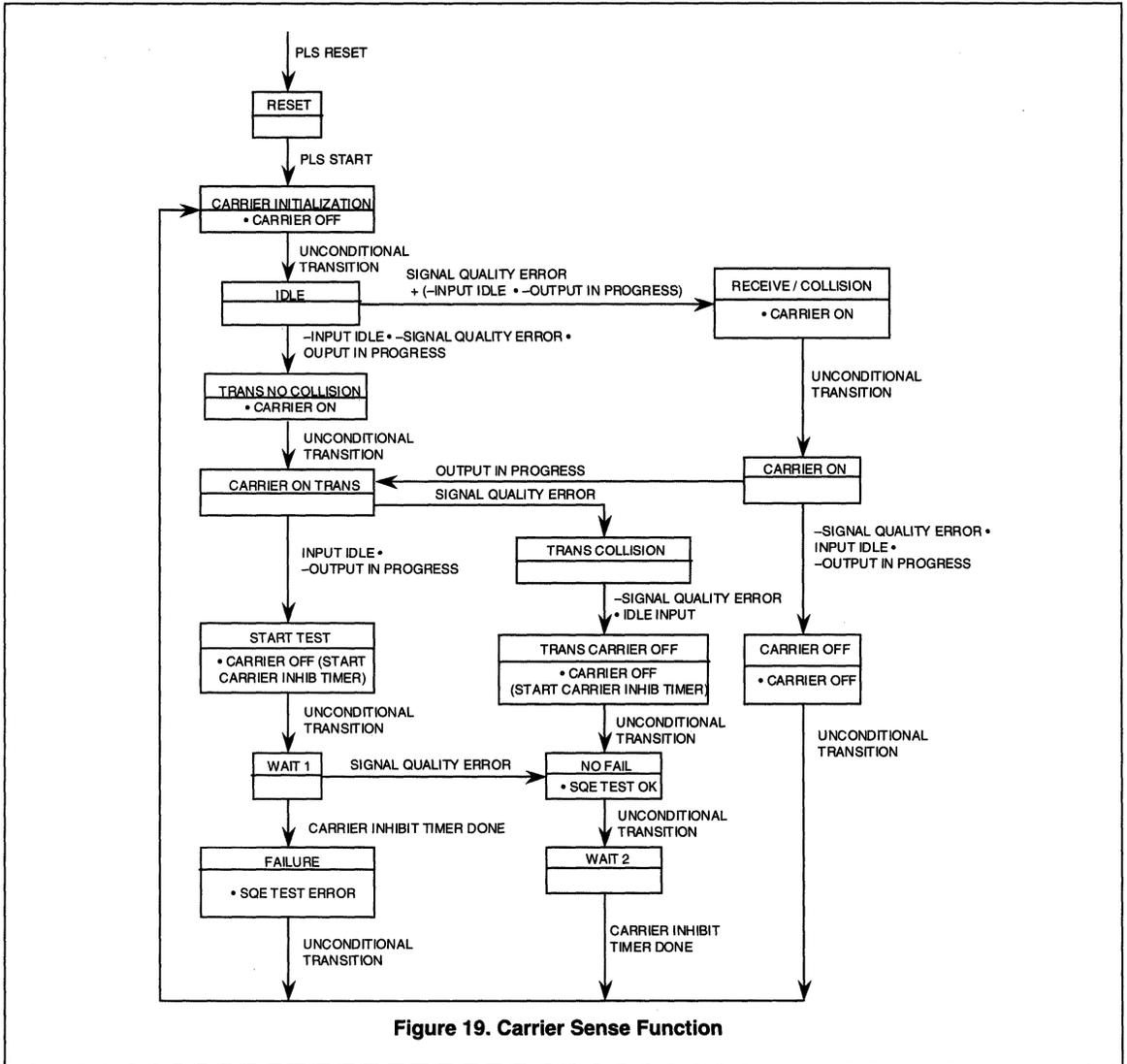
Figure 19. Carrier Sense Function
