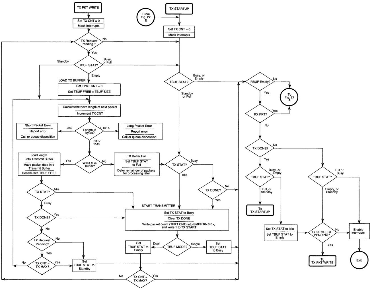
Figure 25. Transmit Packet Write Routine
