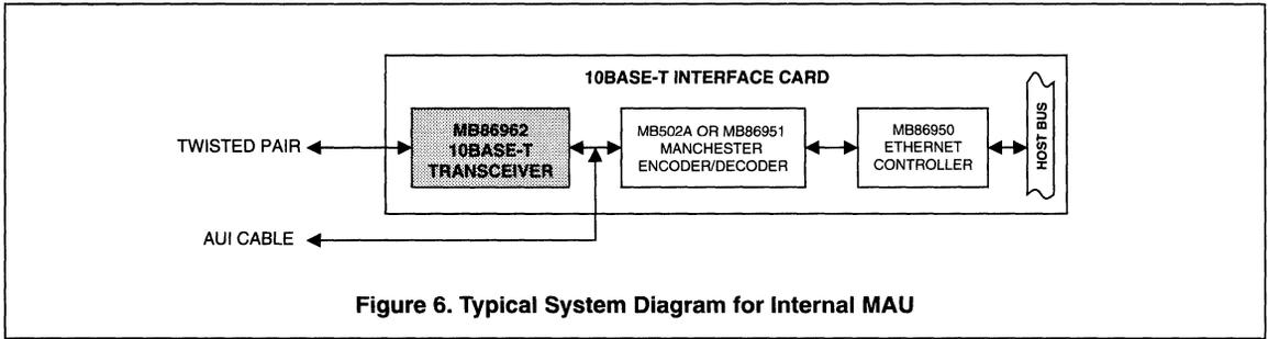
Figure 6. Typical System Diagram for Internal MAU
