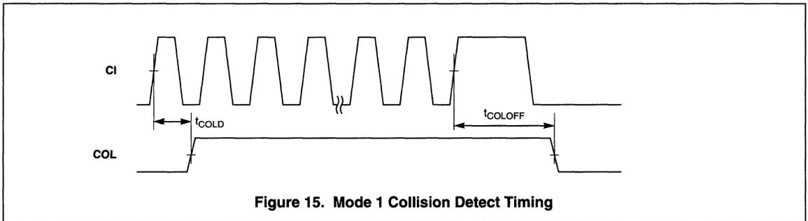
Figure 15. Mode 1 Collision Detect Timing
