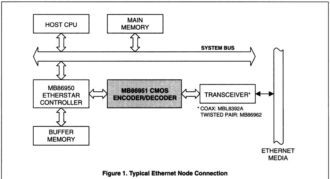
Figure 1. Typical Ethernet Node Connection
