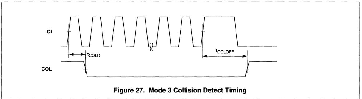
Figure 27. Mode 3 Collision Detect Timing
