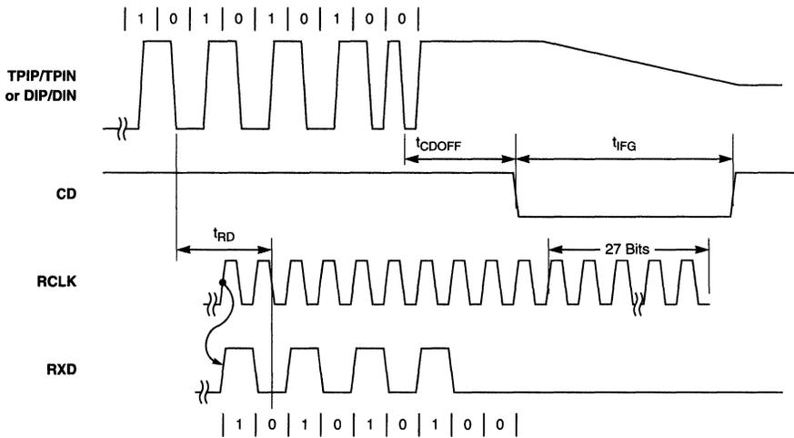
Note: RXD changes at the rising edge of RCLK. The controller is sampled at the falling edge.
