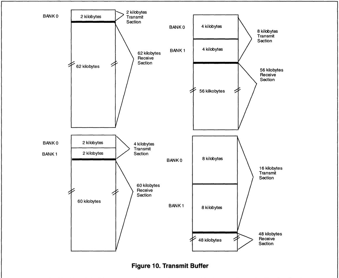
Figure 10. Transmit Buffer
