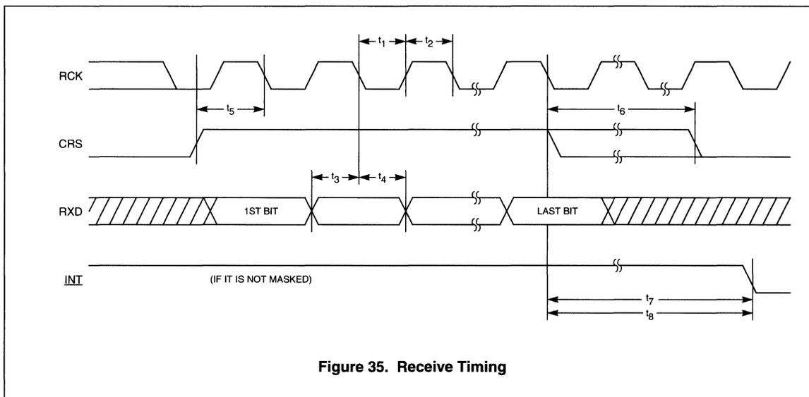
Figure 35. Receive Timing
