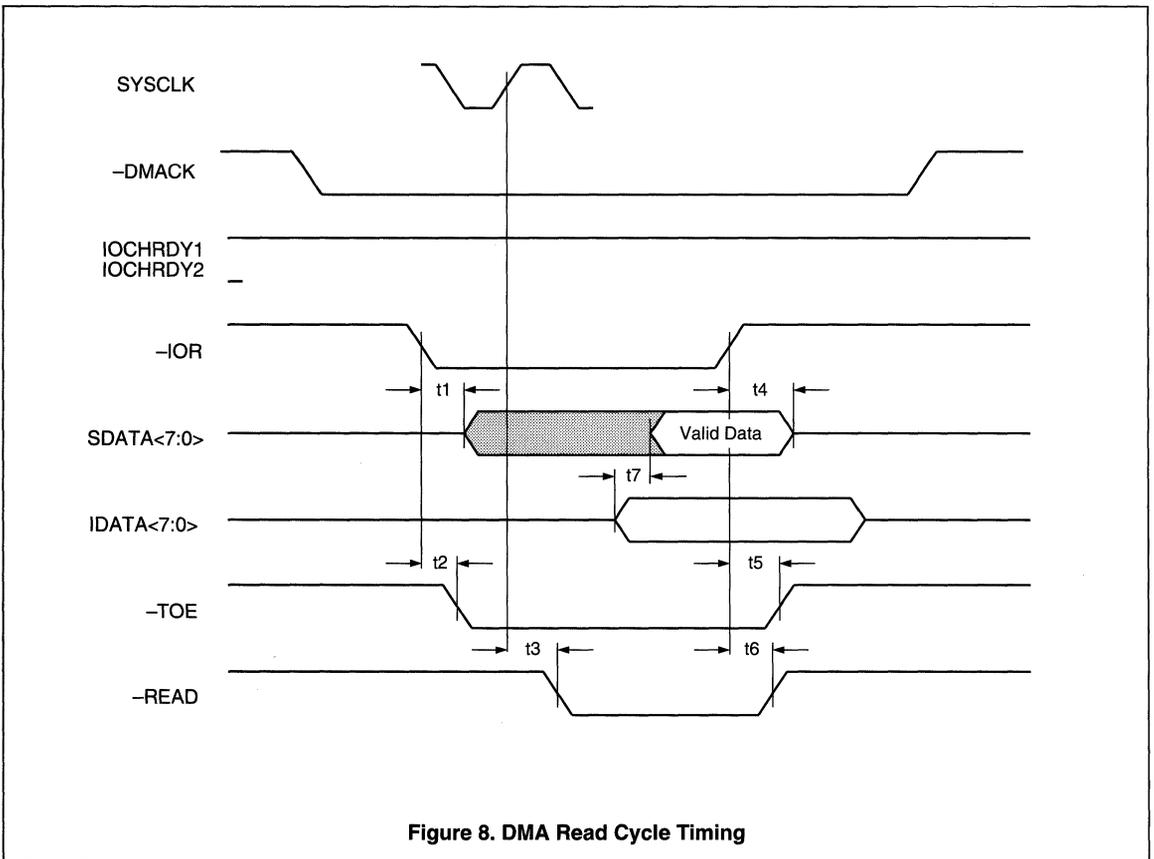
Figure 8. DMA Read Cycle Timing
