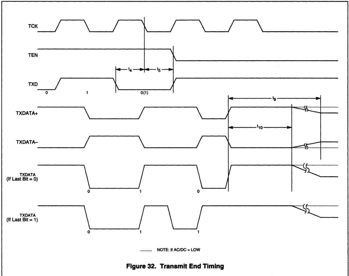
**Table 32. Transmit Start and End Timing: Figures 31-32 (for Encoder/Decoder Test mode)**
