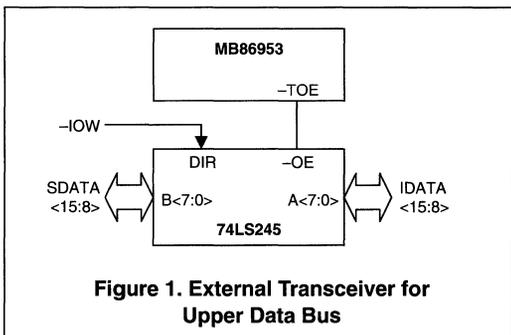
**Figure 1. External Transceiver for Upper Data Bus**
