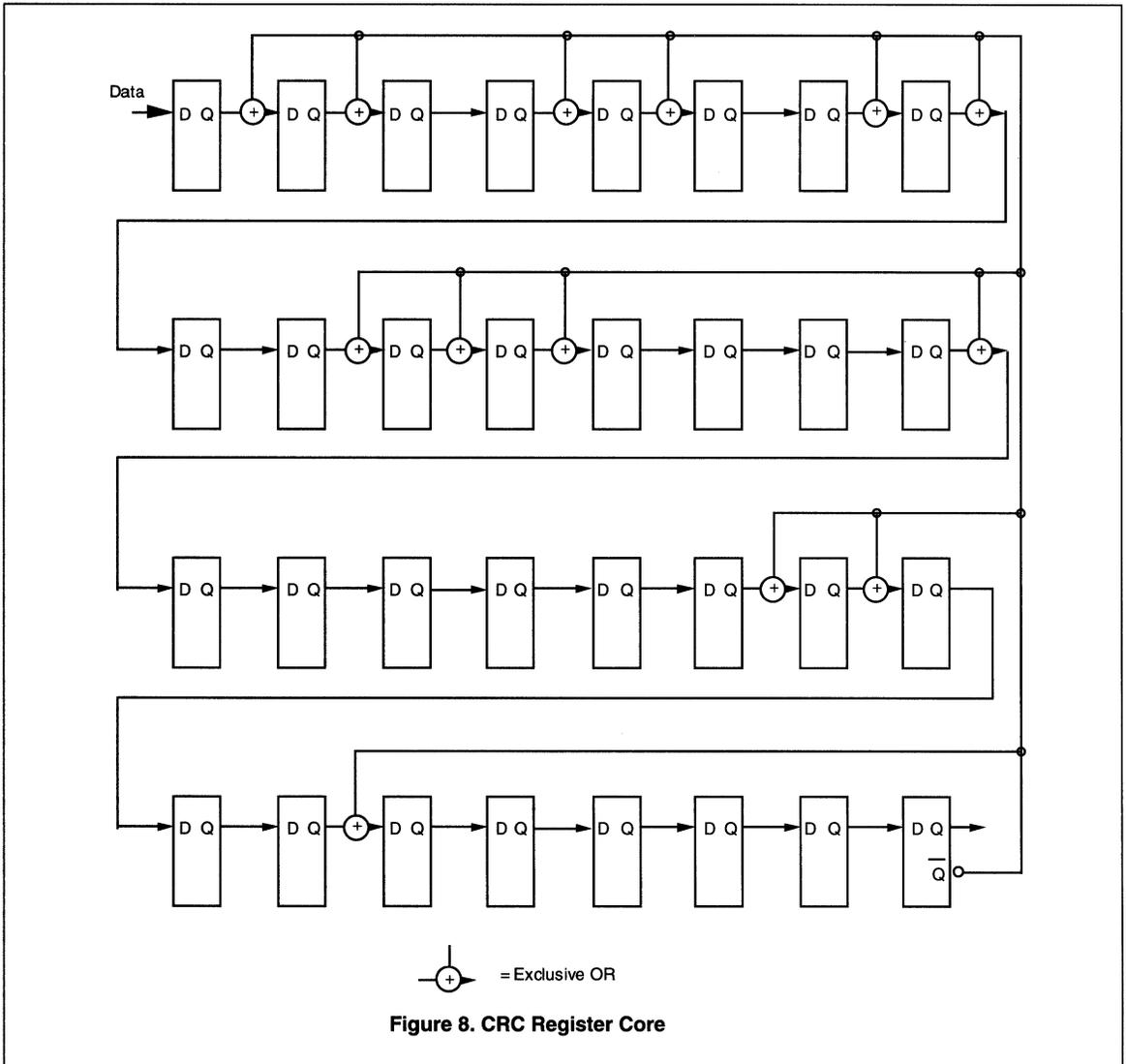
Figure 8 shows the Cyclical Redundancy Check (CRC) register core, which is a modified shift-right register used to generate and check CRCs. While some controllers share a single core between transmitter and receiver, EtherCoupler has one core for the generator and one core for the checker, thus allowing concurrent operation during self-receive.
