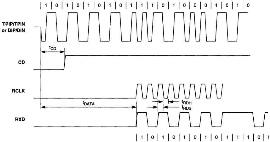
Note: RXD changes at the rising edge of RCLK. The controller is sampled at the falling edge.
