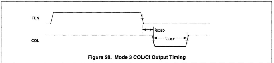
Figure 28. Mode 3 COL/CI Output Timing
