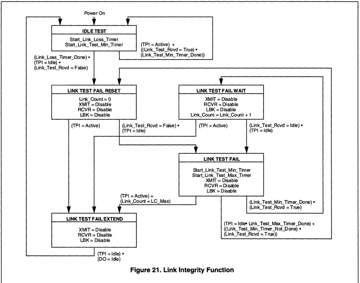
Figure 21. Link Integrity Function
