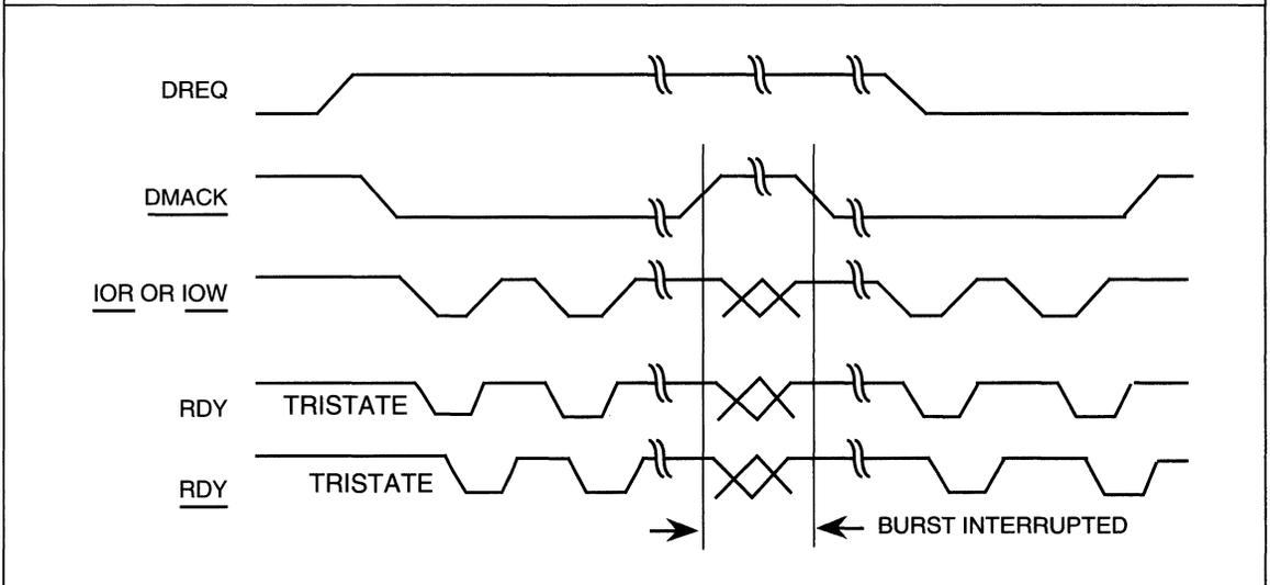
Burst can be interrupted by DMACK high-going pulse during the burst. Burst will resume when DMACK returns low. DREQ goes low during the next-to-last transfer of the burst
