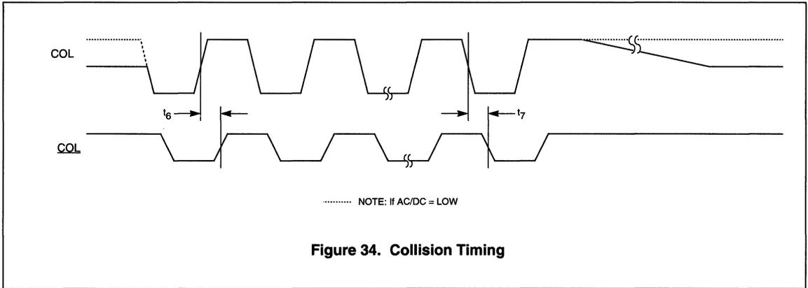
**Table 34. Collision Timing (for Encoder/Decoder Test mode)**
