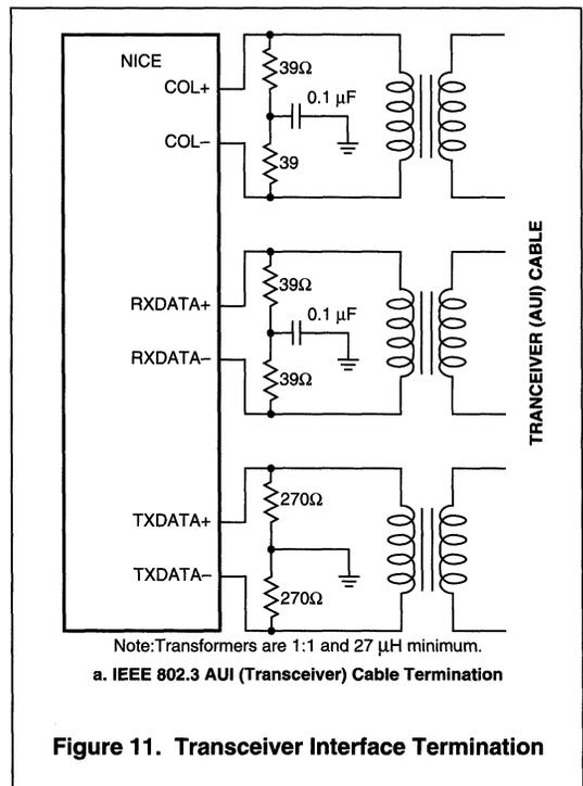
**Figure 11. Transceiver Interface Termination**
