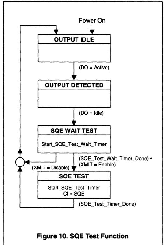
Figure 10. SQE Test Function
