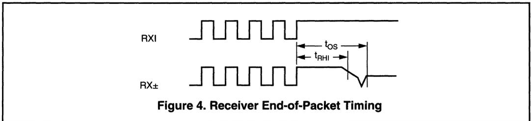
**Figure 4. Receiver End-of-Packet Timing**
