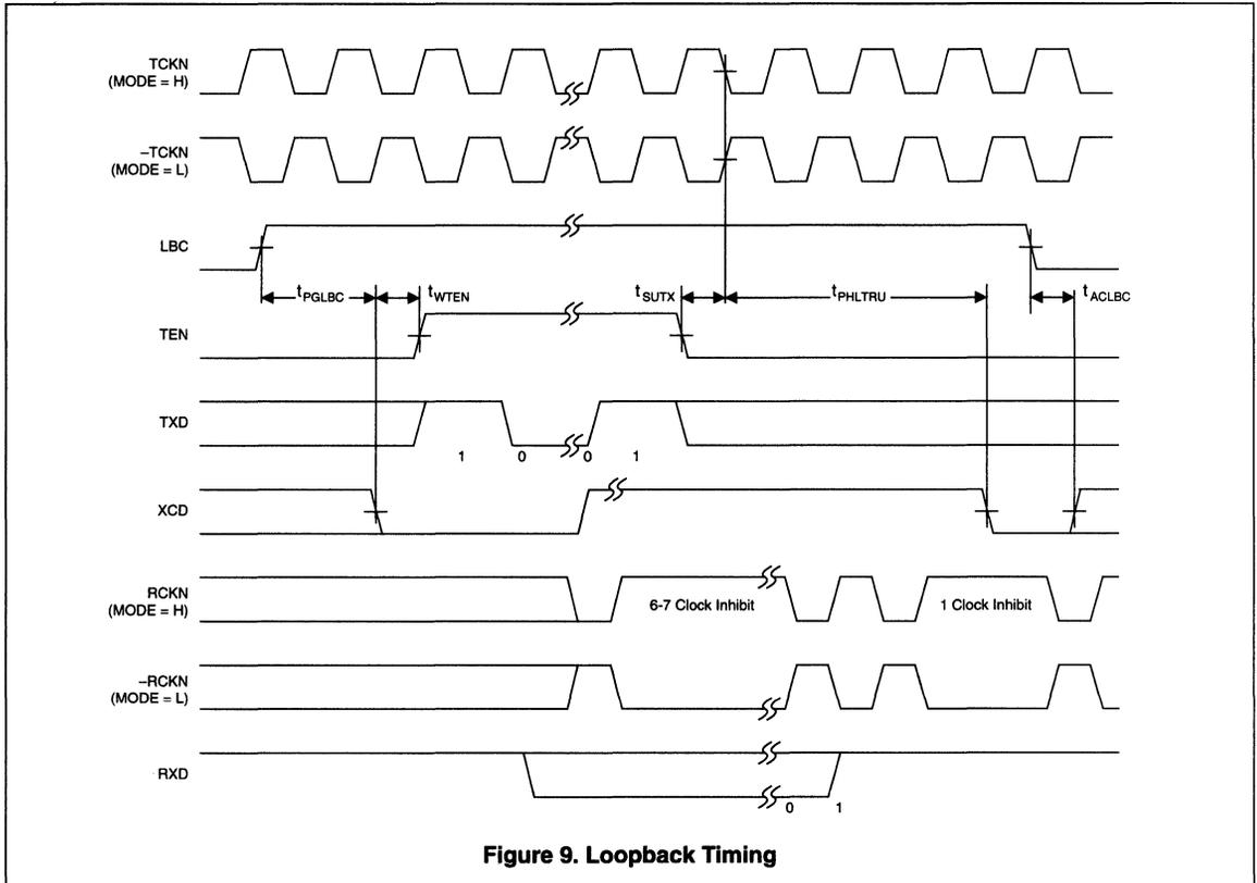
Figure 9. Loopback Timing
