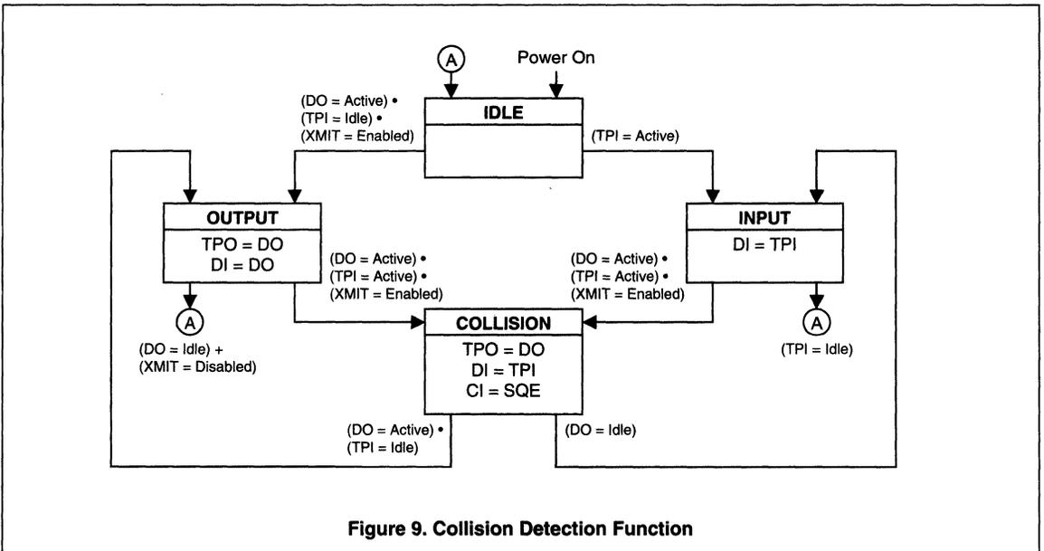
Figure 9. Collision Detection Function
