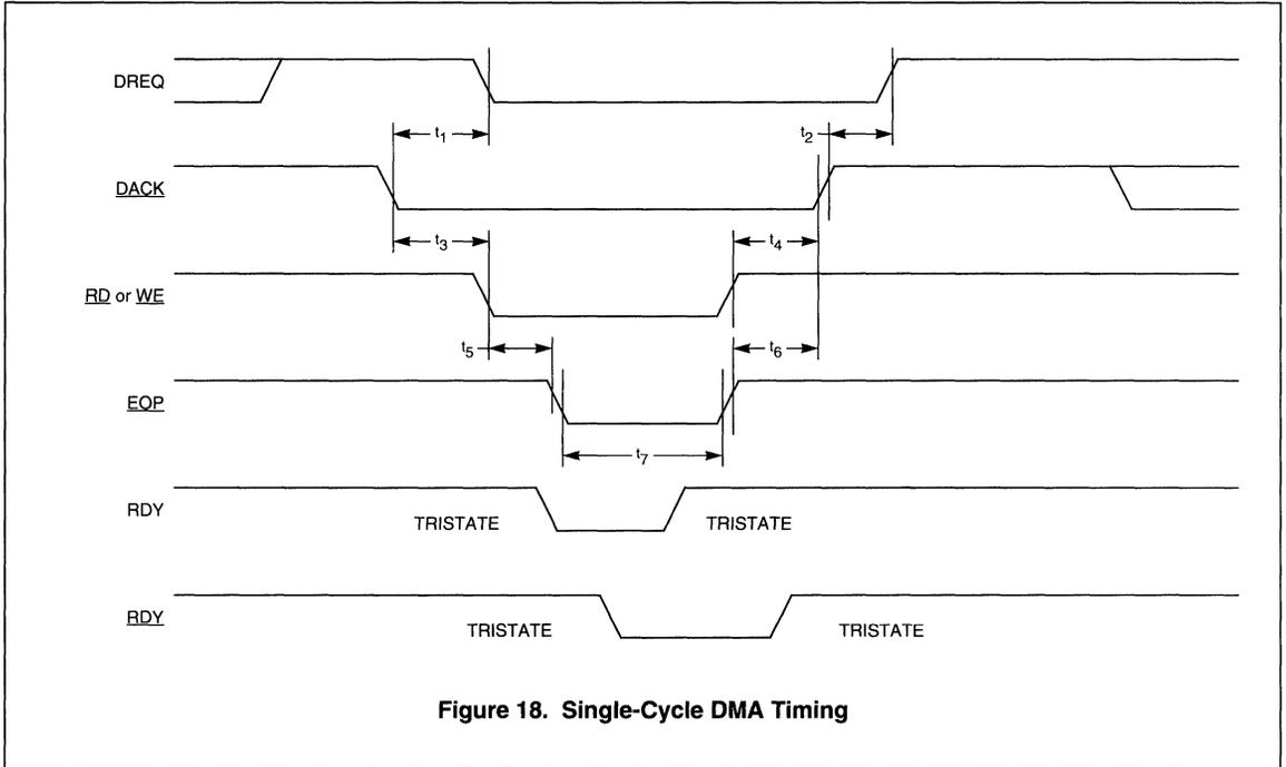
Figure 18. Single-Cycle DMA Timing
