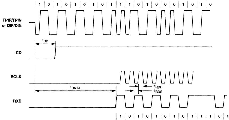
Note: RXD changes at the falling edge of RCLK. The controller is sampled at the rising edge.
