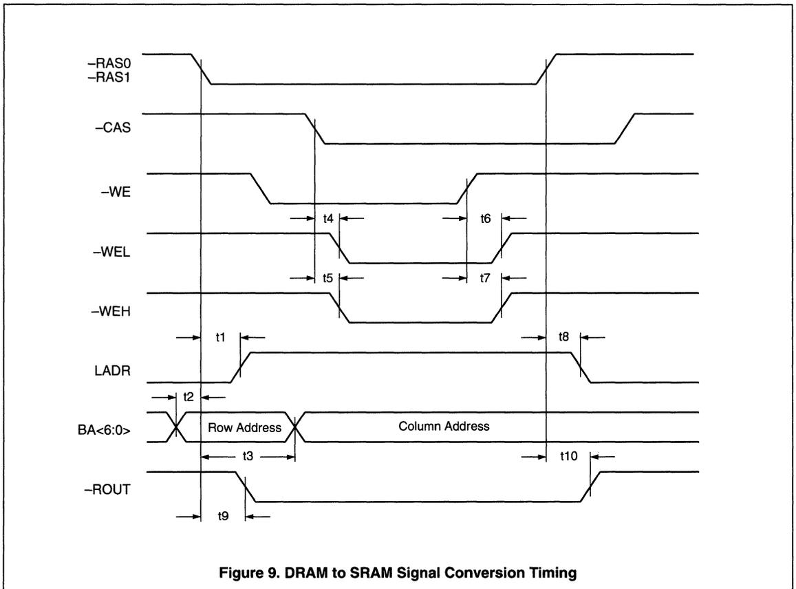
Figure 9. DRAM to SRAM Signal Conversion Timing
