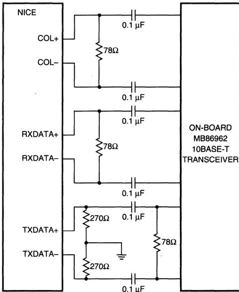
c. Simplified Termination for on-board 10BASE-T Transceiver
