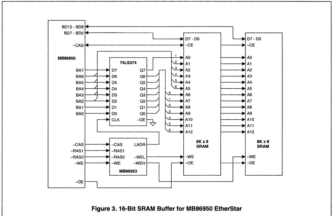
Figure 3. 16-Bit SRAM Buffer for MB86950 EtherStar
