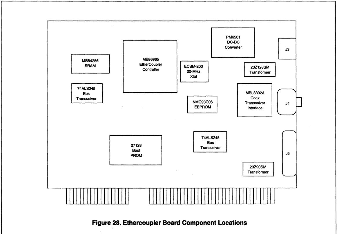
**Figure 28. Ethercoupler Board Component Locations**
