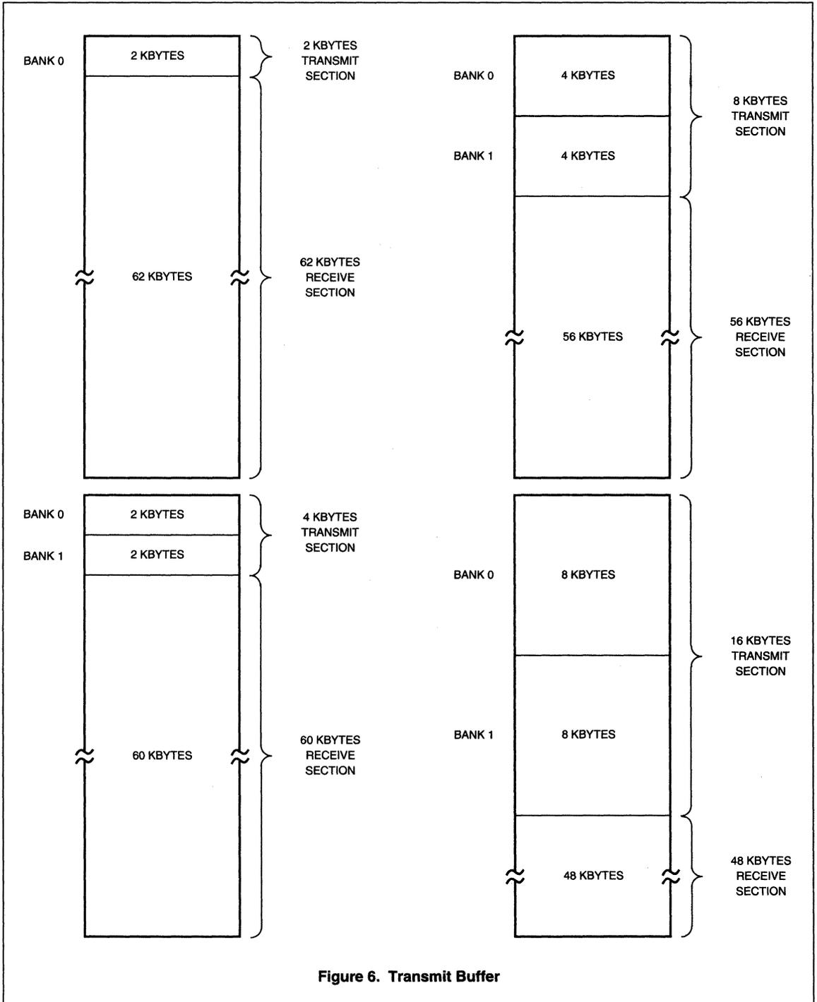
Figure 6. Transmit Buffer
