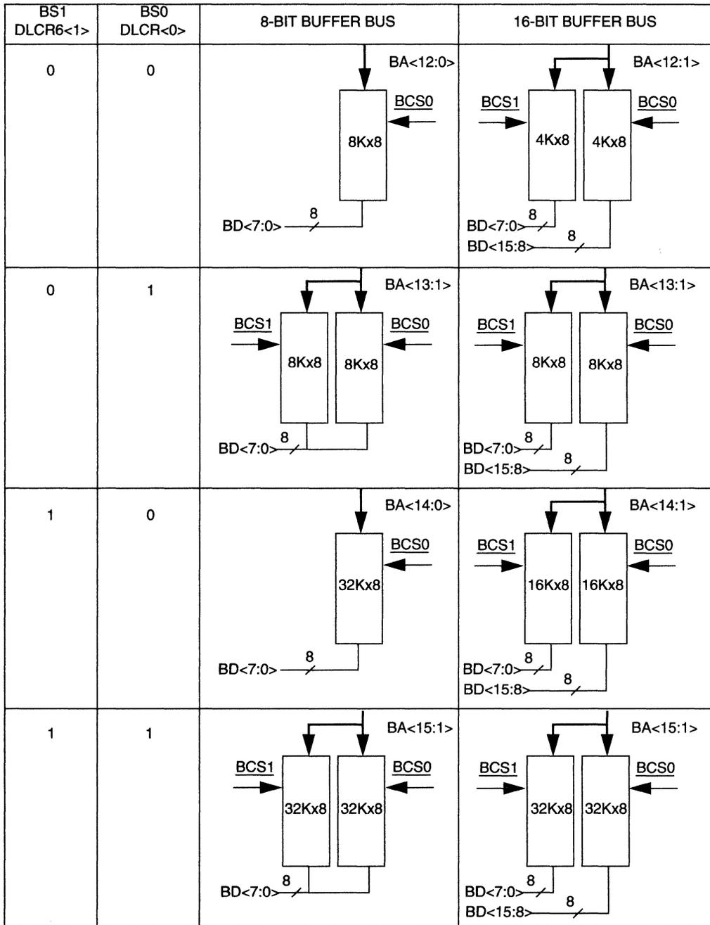
Figure 4. SRAM Configuration
