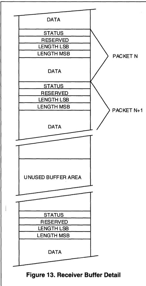
**Figure 13. Receiver Buffer Detail**
