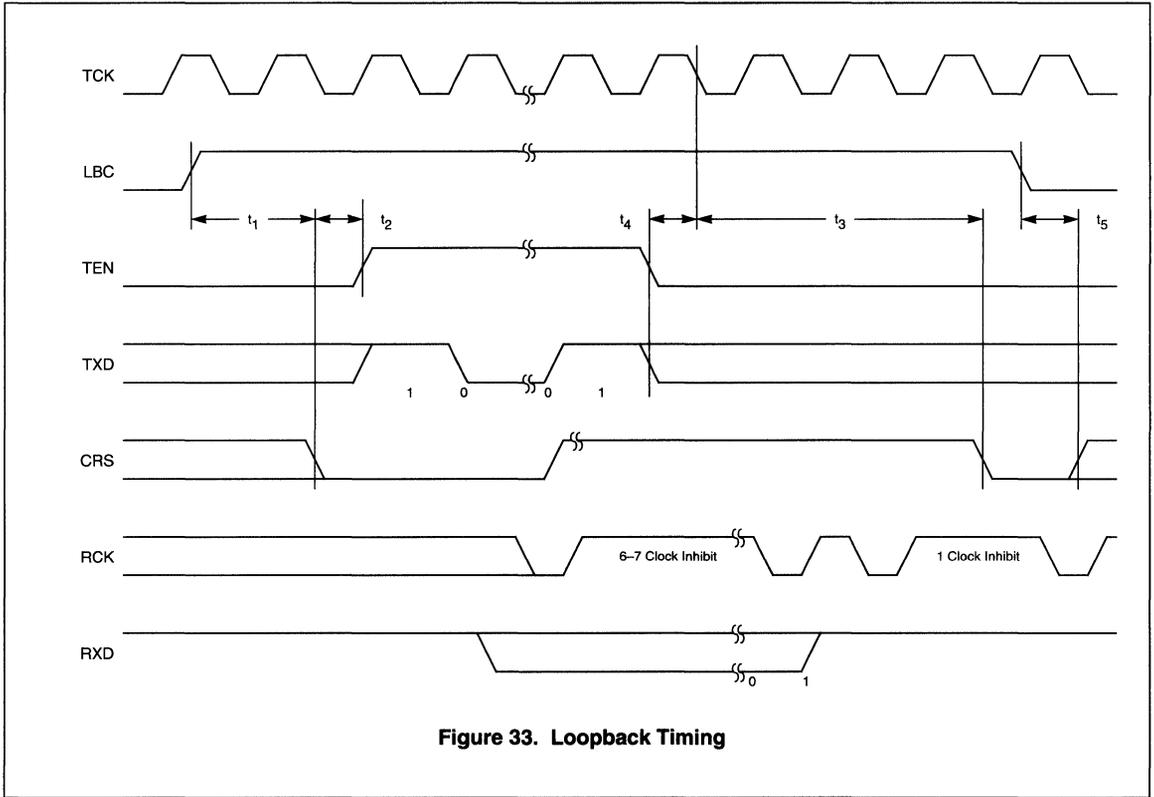
Figure 33. Loopback Timing
