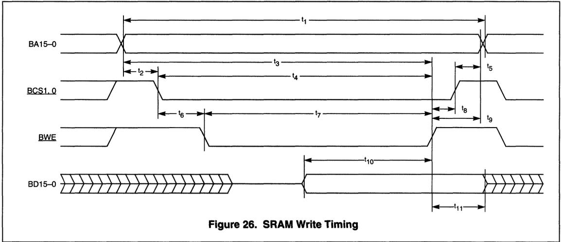
Figure 26. SRAM Write Timing
