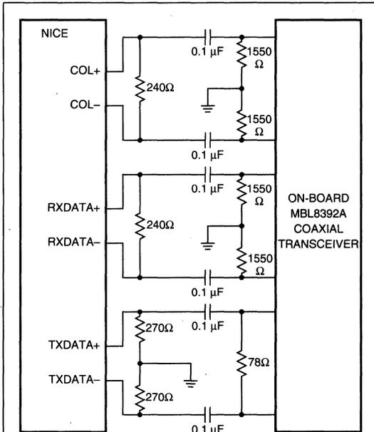
b. Simplified Termination for Coaxial Transceiver
