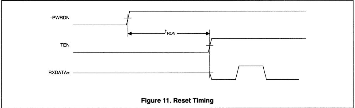
Figure 11. Reset Timing
