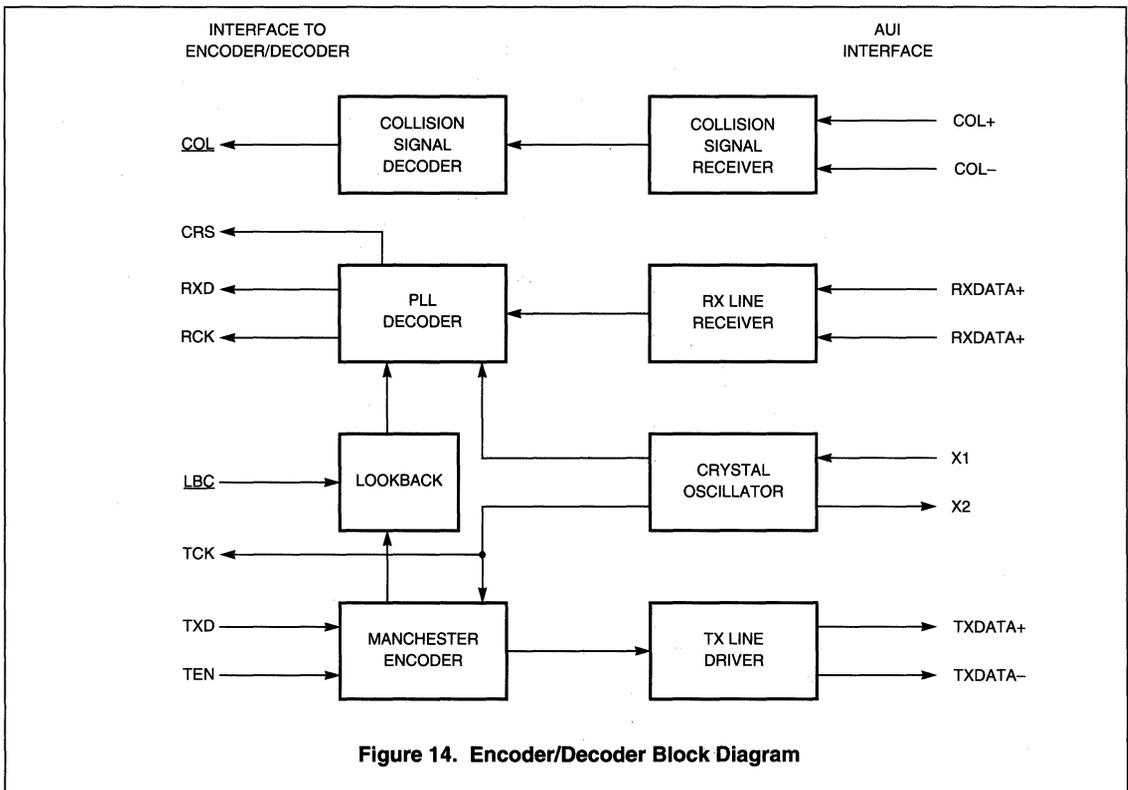
Figure 14. Encoder/Decoder Block Diagram
