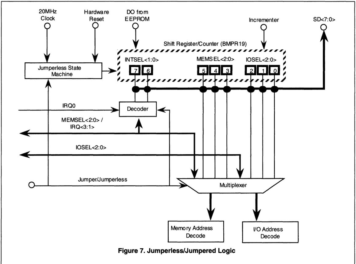
Figure 7. Jumperless/Jumpered Logic
