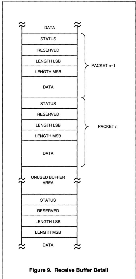
Figure 9. Receive Buffer Detail
