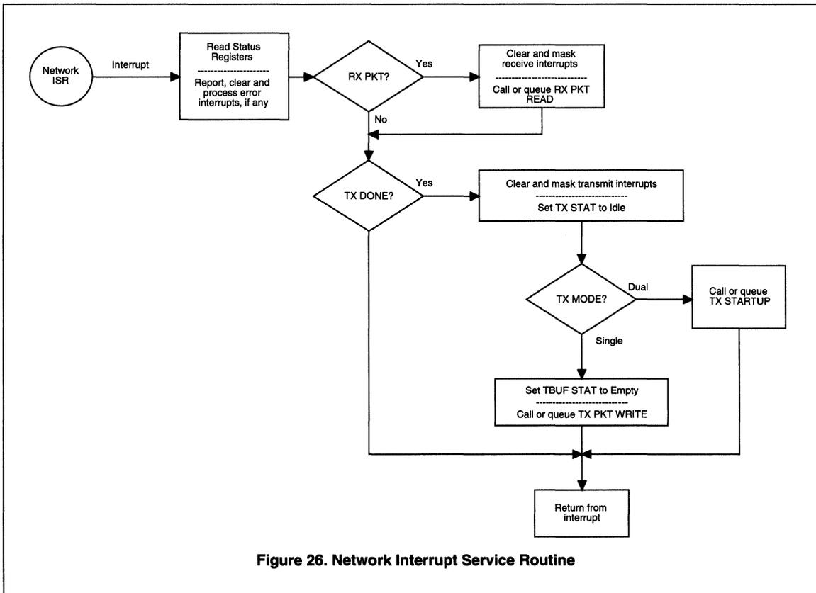
Figure 26. Network Interrupt Service Routine
