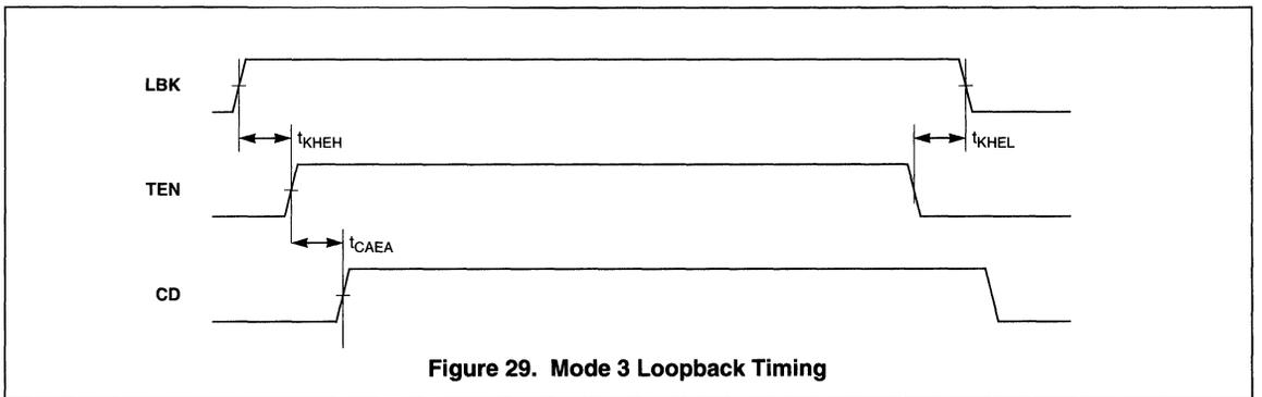
Figure 29. Mode 3 Loopback Timing
