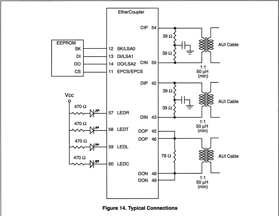
Figure 14. Typical Connections
