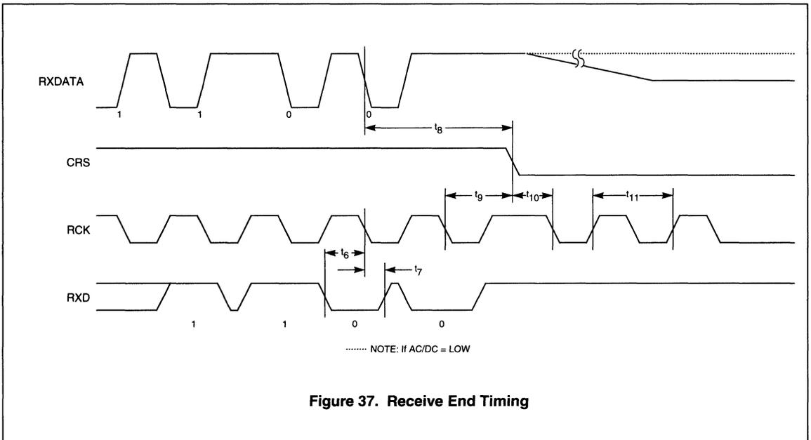
Figure 37. Receive End Timing
