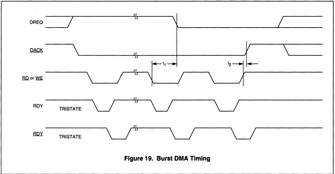
Figure 19. Burst DMA Timing
