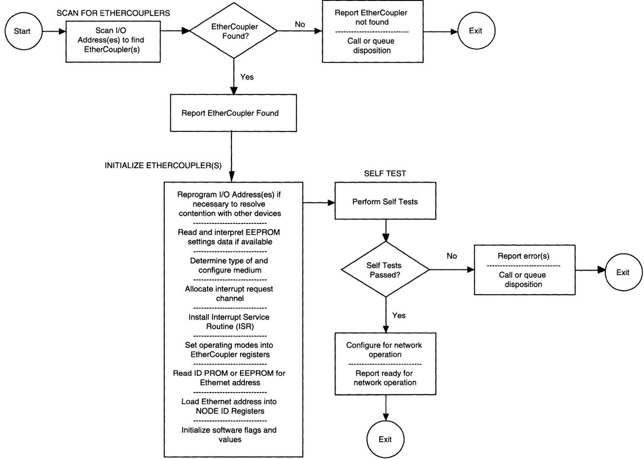
Figure 24. Start-up Testing
