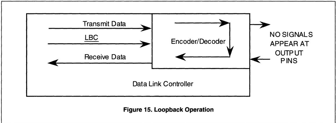
Figure 15. Loopback Operation
