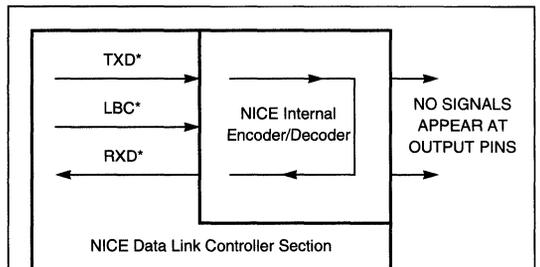
\* In "NICE" mode, these are internal signals and no signals appear on the corresponding pins.
