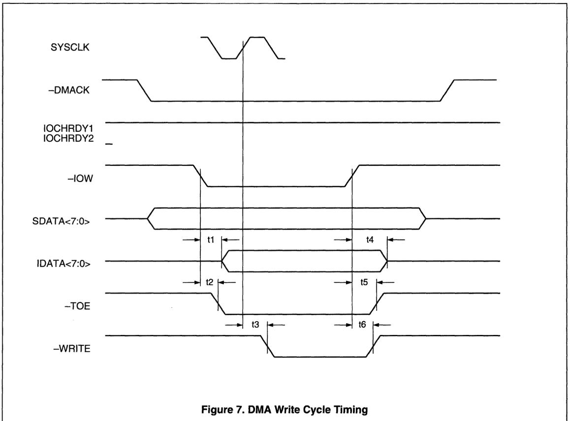
Figure 7. DMA Write Cycle Timing
