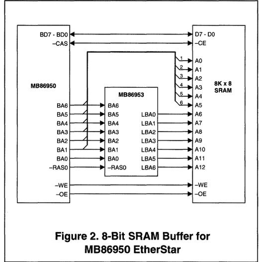
**Figure 2. 8-Bit SRAM Buffer for MB86950 EtherStar**
