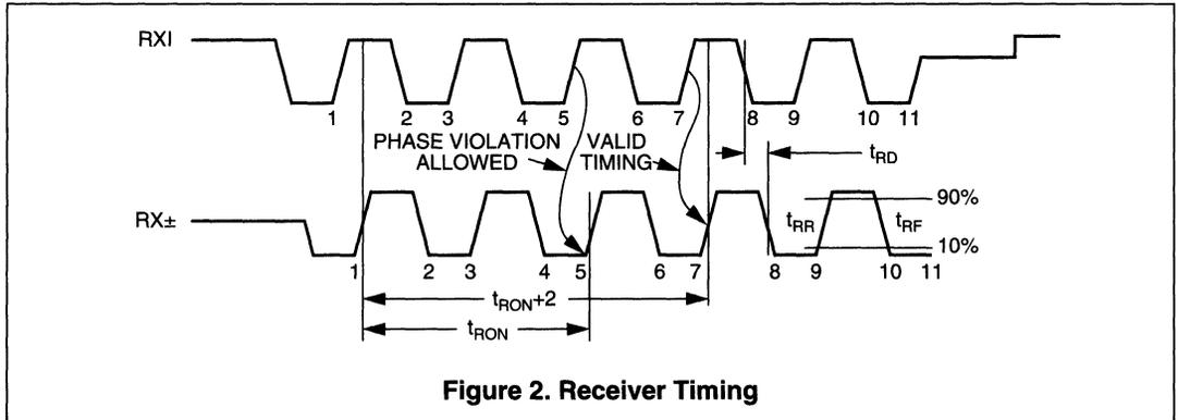
**Figure 2. Receiver Timing**
