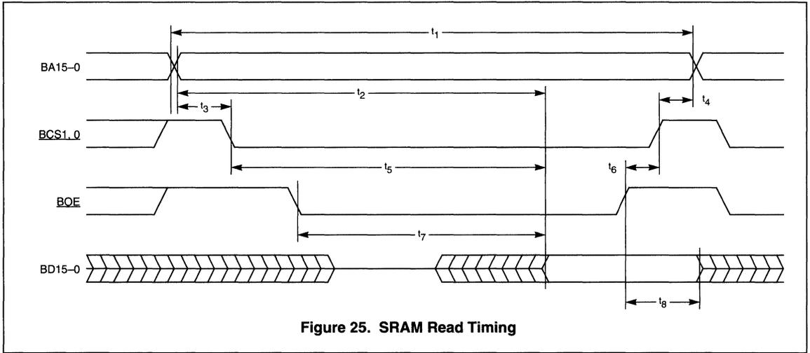
Figure 25. SRAM Read Timing
