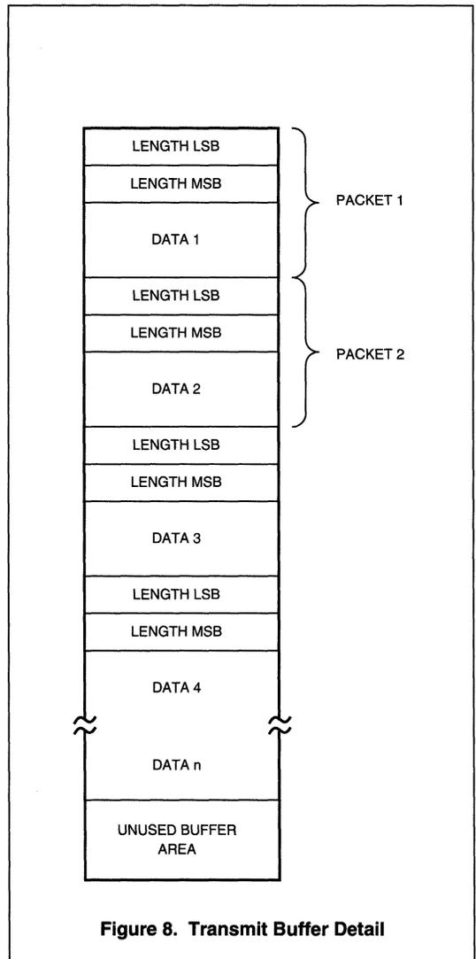
Figure 8. Transmit Buffer Detail
