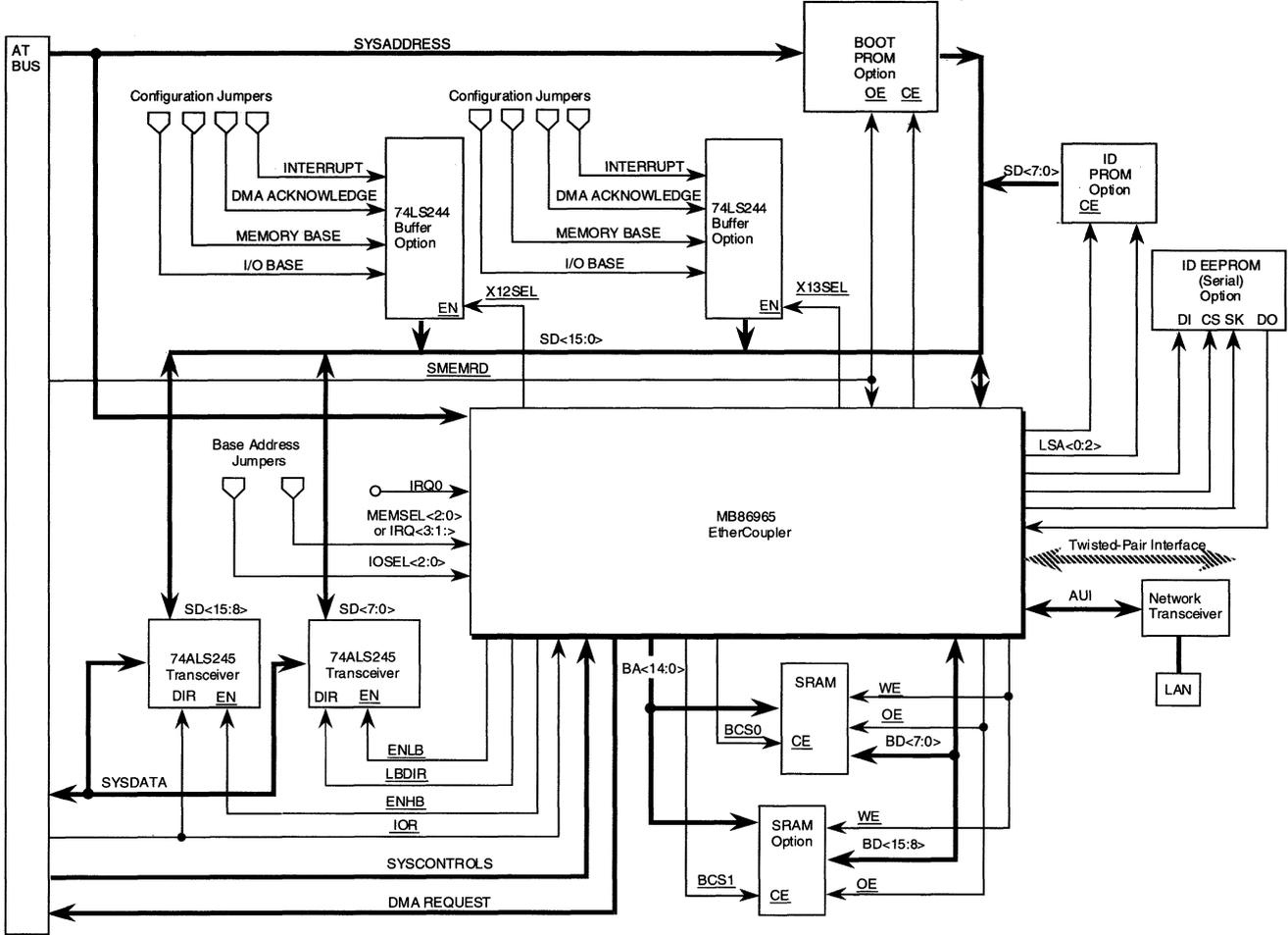
Figure 6. EtherCoupler Bus Operation Block Diagram
