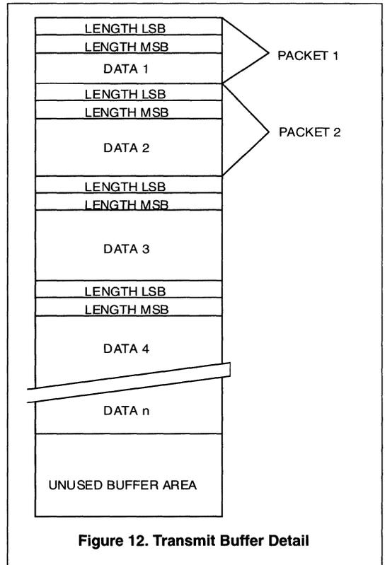
**Figure 12. Transmit Buffer Detail**
