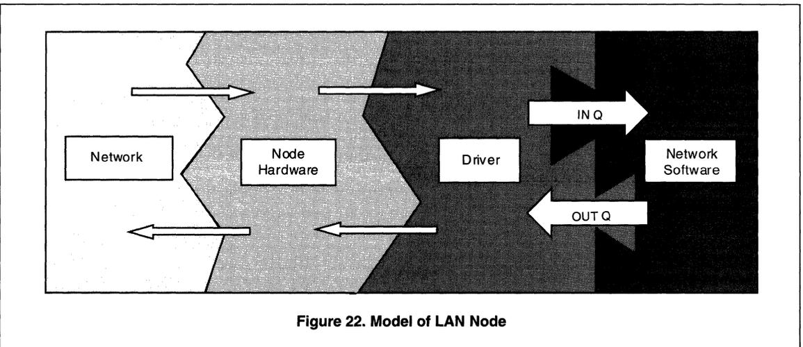
Figure 22. Model of LAN Node
