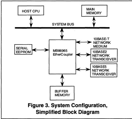
**Figure 3. System Configuration, Simplified Block Diagram**
