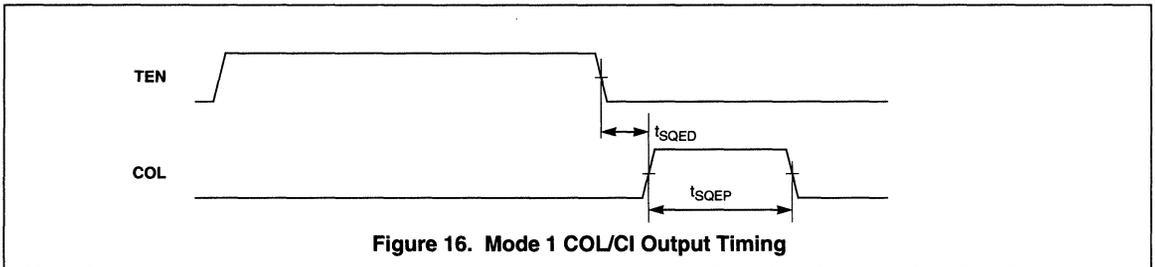
Figure 16. Mode 1 COL/CI Output Timing
