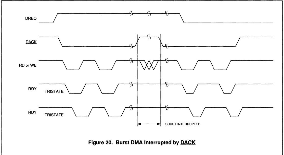
**Note:** Burst can be interrupted by DACK high-going pulse during the burst. Burst will resume when DACK returns low.
