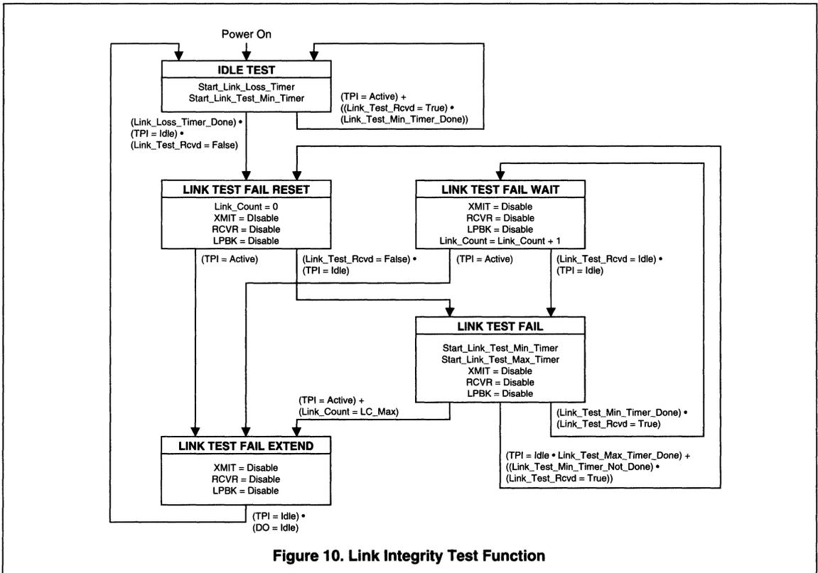
Figure 10. Link Integrity Test Function
