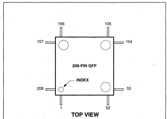
**PIN ASSIGNMENT — 208-LEAD QFP**
