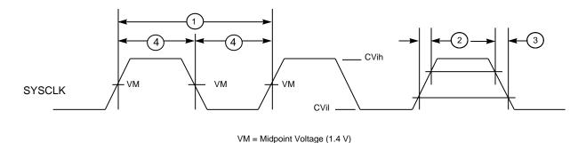
Figure 1. SYSCLK Input Timing Diagram
