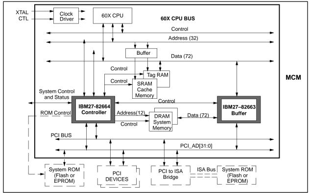
Figure 1-1. MCM Block Diagram
