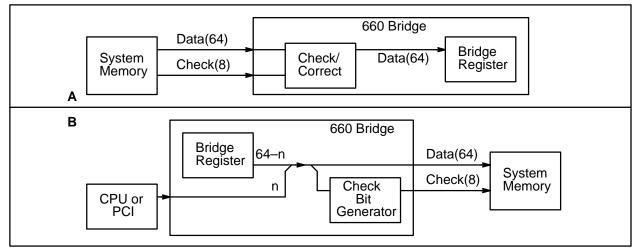
Figure 4-8. PCI or CPU Read-Modify-Write Data Flow
