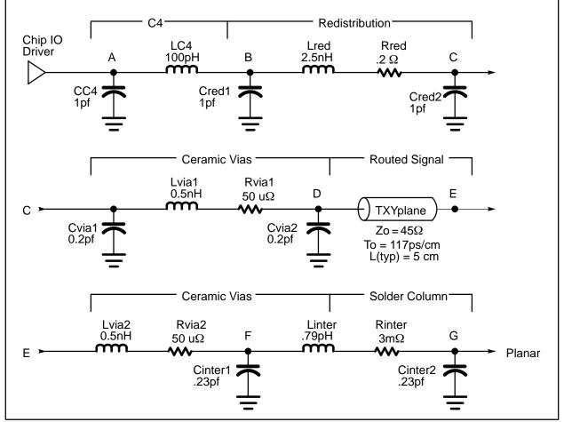
Figure 12-1. MCM Net Electrical Model
