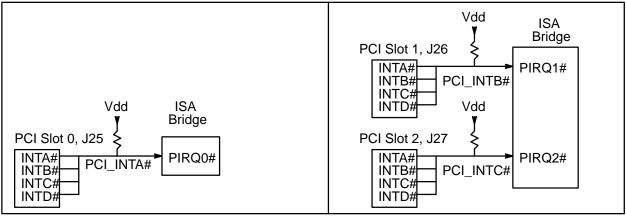
Figure 8-3. PCI Interrupt Connections
