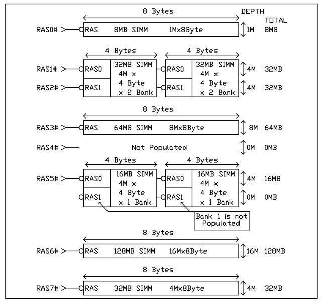
Figure 4-3. Example Memory Bank Configuration
