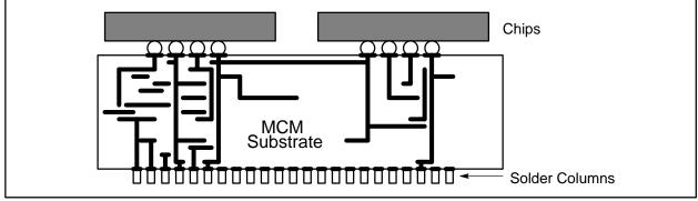
Figure 1-4. MCM Flip Chips and Internal Wiring
