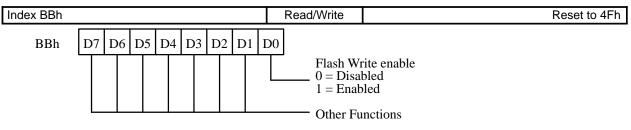
Bit 0 Flash write enable: When the ROM is remotely attached, this bit controls write access to the flash ROM address space (4G – 2M to 4G). When enabled, writes to this space are forwarded to the PCI memory space at the same address. When disabled, writes to this space are treated as noops and an error is signalled. After the bit is set to 0 (disabled), it cannot be reset to 1 (enabled).
