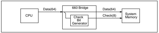
Figure 4-6. CPU 8-Byte Write Data Flow
