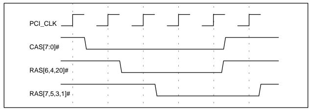
Figure 4-9. DRAM Refresh Timing Diagram
