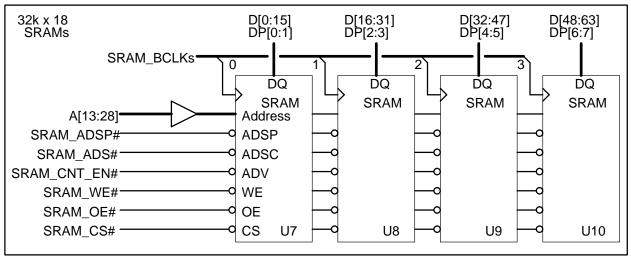
Figure 3-6. Synchronous SRAM, 512K L2
