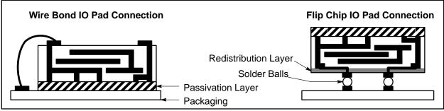
Figure 1-3. Chip Wire Bond and Flip Chip Connection
