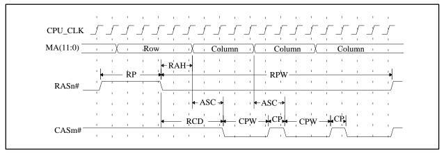
Figure 4-1. CPU to Memory Transfer Timing Parameters
