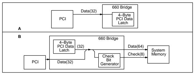
Figure 4-7. PCI 8-Byte Write Data Flow
