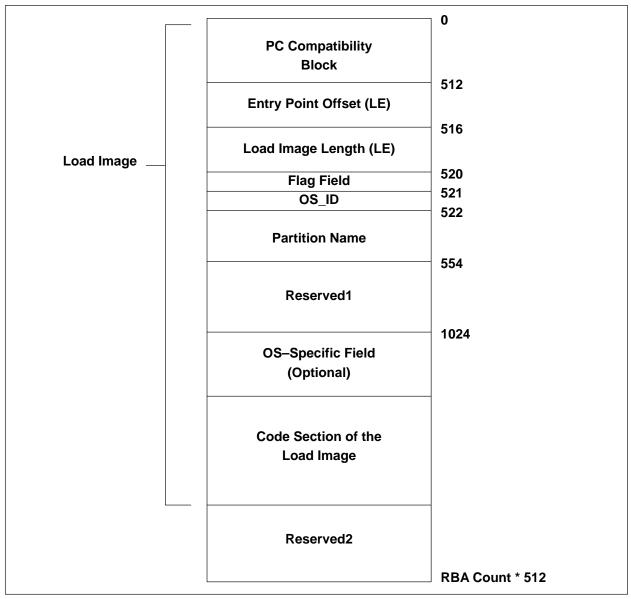
Figure 10-5. PowerPC Reference Platform Partition
