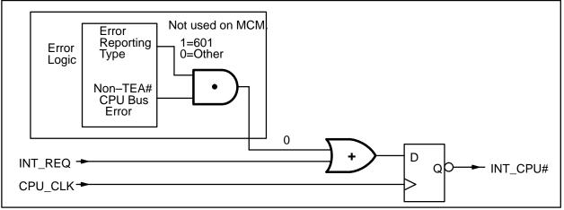
Figure 8-1. Conceptual Block Diagram of INT Logic
