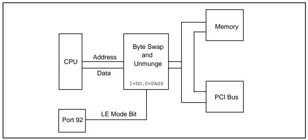
Figure 11-1. Endian Mode Block Diagram
