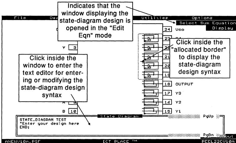
Figure 4-24, Entering design description for the state-diagram
