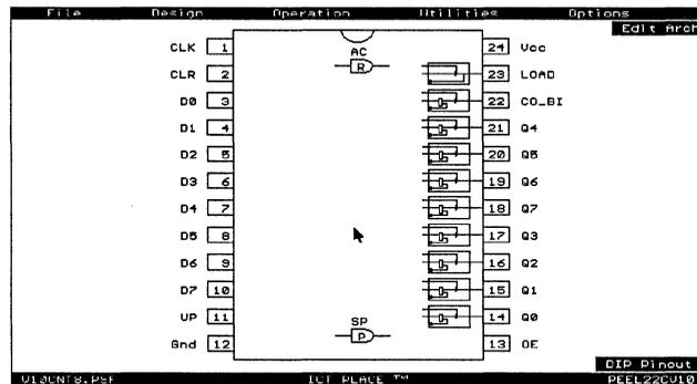
Figure 6-38, PLACE pin block diagram of V10CNT8.PSF
