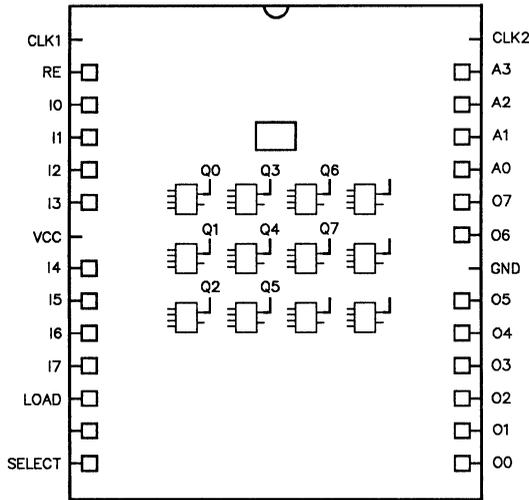
Figure 6-18, Pin block diagram of ST7128.PSF
