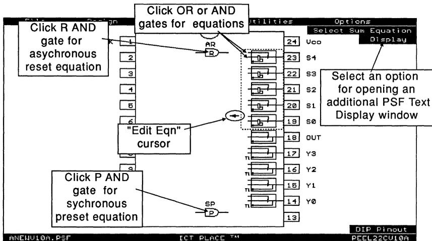
Figure 4-19, "Edit Eqn" mode of the PEEL22CV10A
