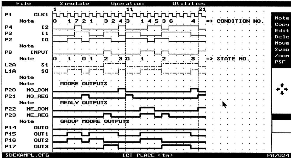
Figure 5-8 Simulate Waveforms for the SDEXAMPL Design Example
