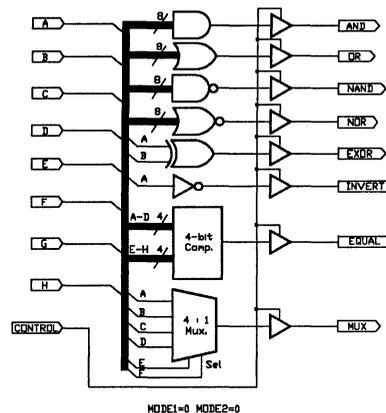
Figure 6-4, Logic schematic of GATES1.PSF
