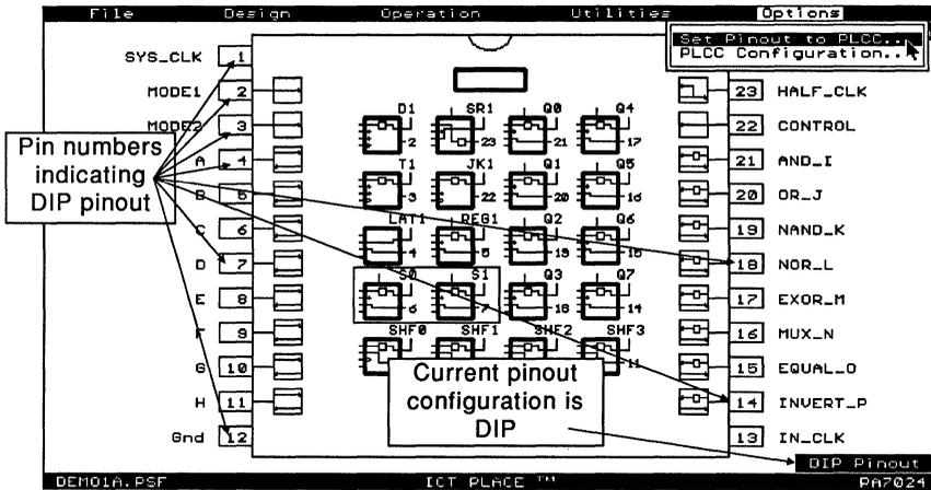
Figure 4-34, "Options" menu and DIP pinout for the PA7024
