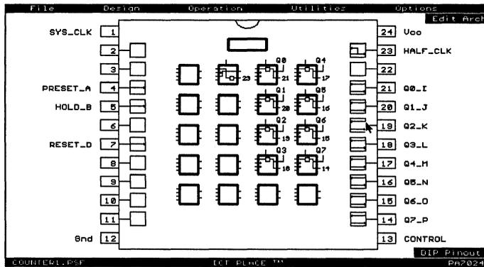
Figure 6-9, PLACE pin block diagram of COUNTER1.PSF
