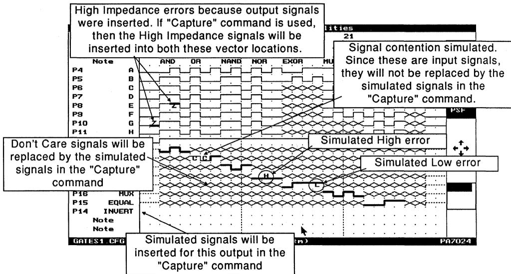
Figure 4-42, Vector simulate errors
