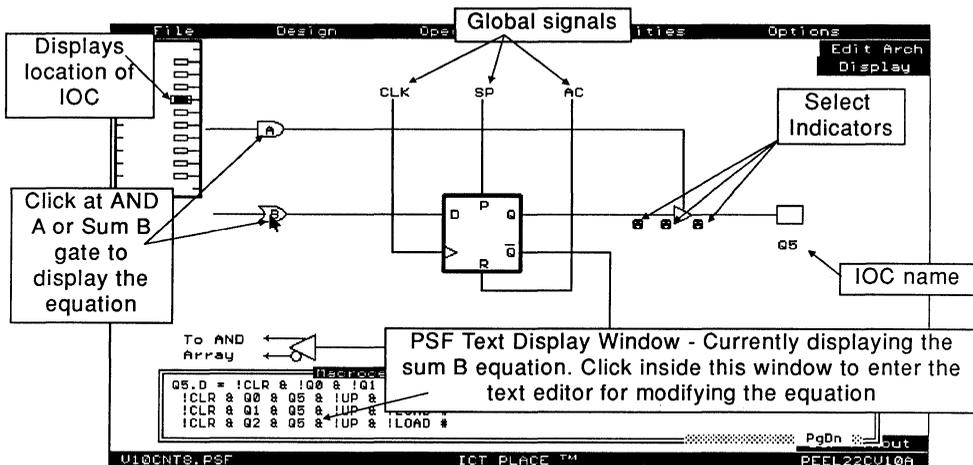
Figure 4-14, IOC screen of the PEEL22CV10A
