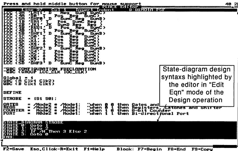
Figure 4-70, Automatic block selection by the editor in the Design operation
