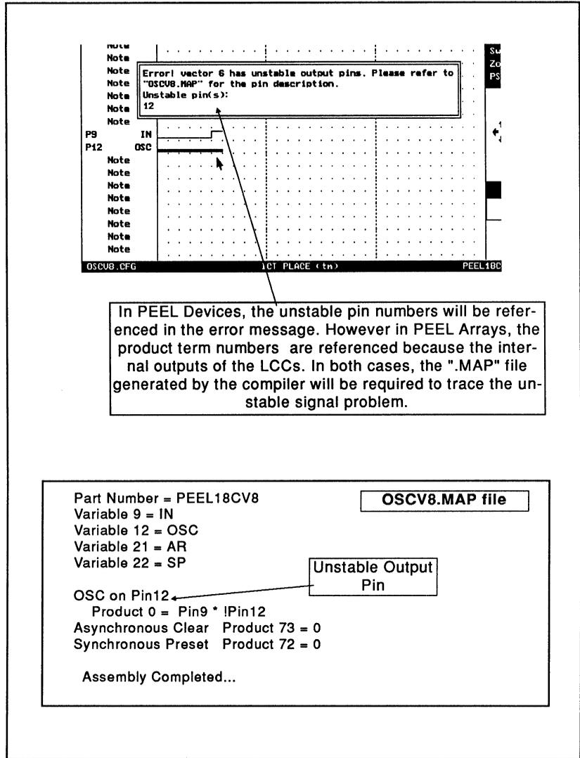
Figure 4-43, Unstable output simulation error example
