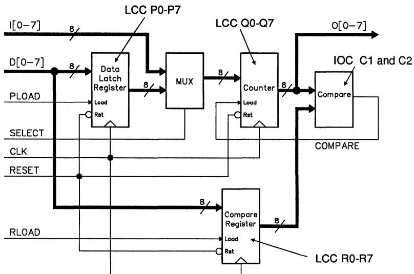
Figure 6-17, Logic block diagram of TC7140.PSF
