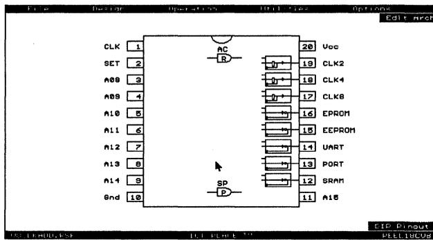
Figure 6-24, PLACE pin block diagram of V8CLKADD.PSF
