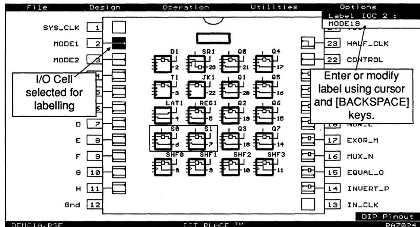
Figure 3-6, The "Label" command for Pin, INC, IOC and LCC
