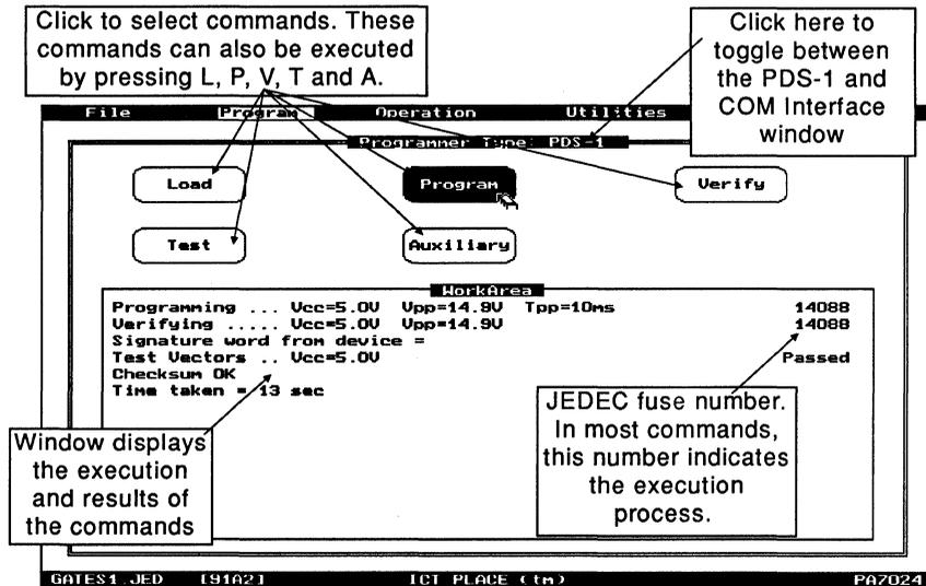
Figure 4-65, PDS-1 Interface window in the Program operation
