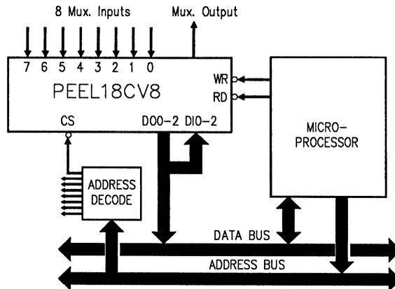
Figure 6-27, Logic schematic of V8BUSMUX.PSF
