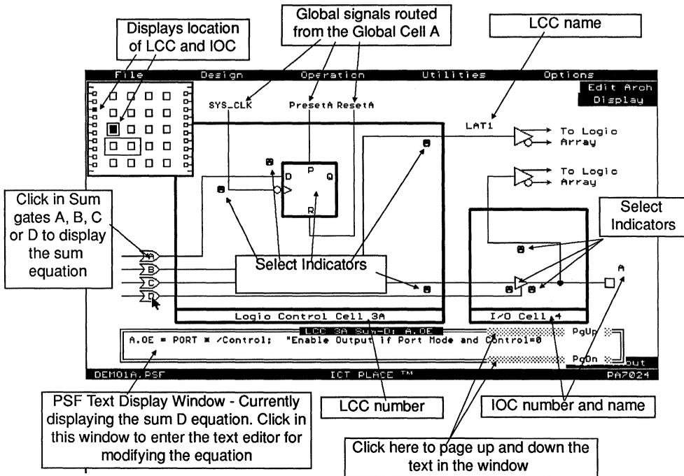
Figure 3-7, Configuring the LCC and IOC Architecture
