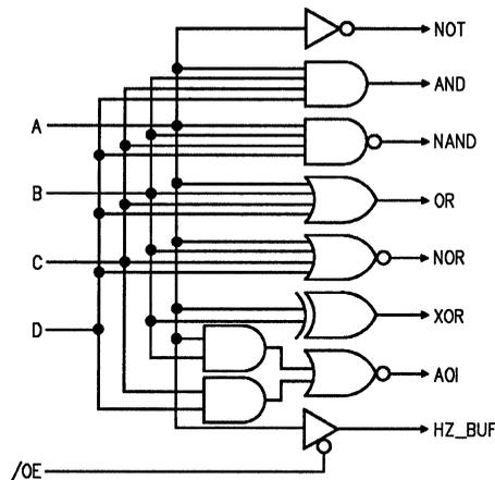
Figure 6-21, Logic schematic of V8GATES.PSF
