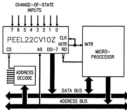
Figure 6-42, System interface block diagram of V10ZPORT.PSF
