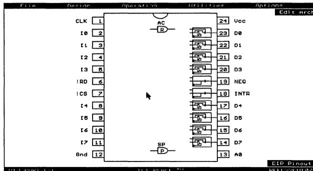
Figure 6-41, PLACE pin block diagram of V10ZPORT.PSF
