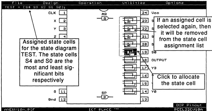
Figure 4-23, Allocating state cells for a state-diagram design
