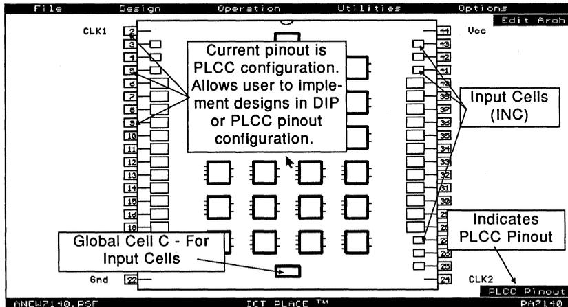
Figure 4-11, Pin Block Diagram of the PA7140
