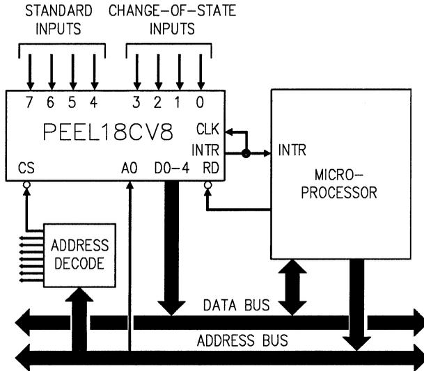
Figure 6-31, System interface block diagram of V8CPORT.PSF
