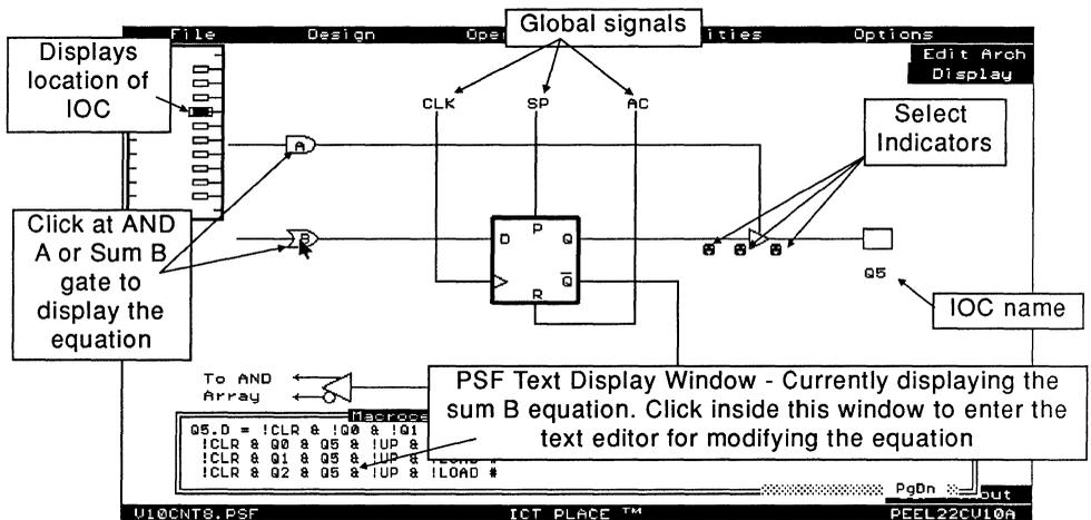
Figure 4-21, Editing equations in the IOC screen of the PEEL22CV10A
