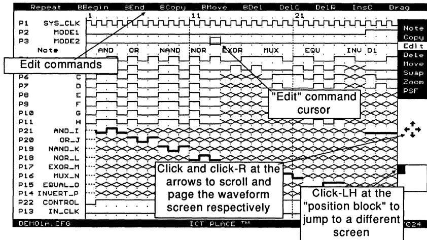
Figure 4-48, "Edit" command in the Simulate operation
