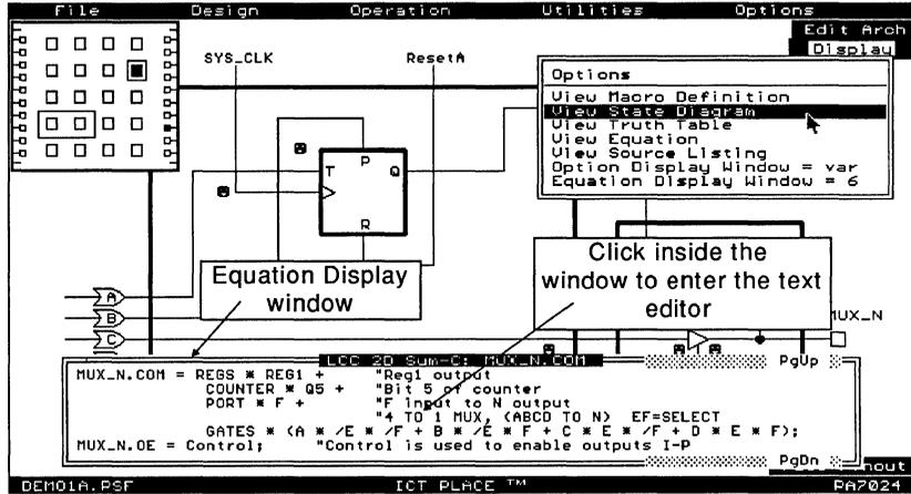
Figure 4-30, "Display" menu in the LCC/IOC screen
