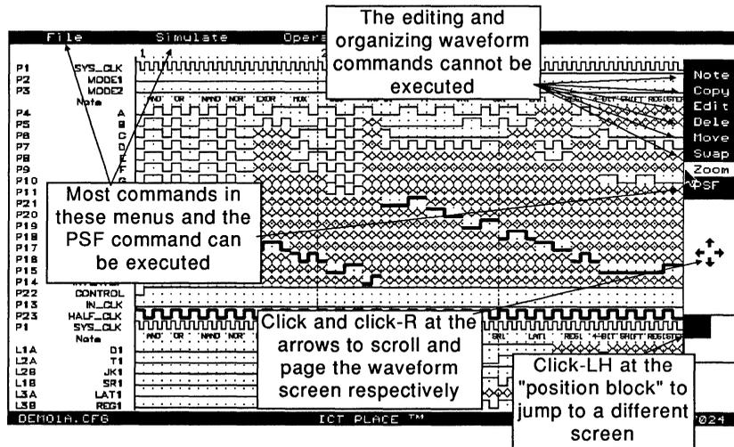
Figure 4-53, Mode A of the "Zoom" waveform screen
