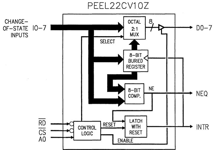
Figure 6-43, Logic schematic of V10ZPORT.PSF
