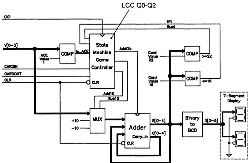
Figure 6-15, Logic block diagram of JACK7024.PSF
