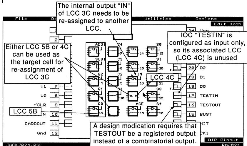
Figure 4-8, A typical example for re-assigning the LCC
