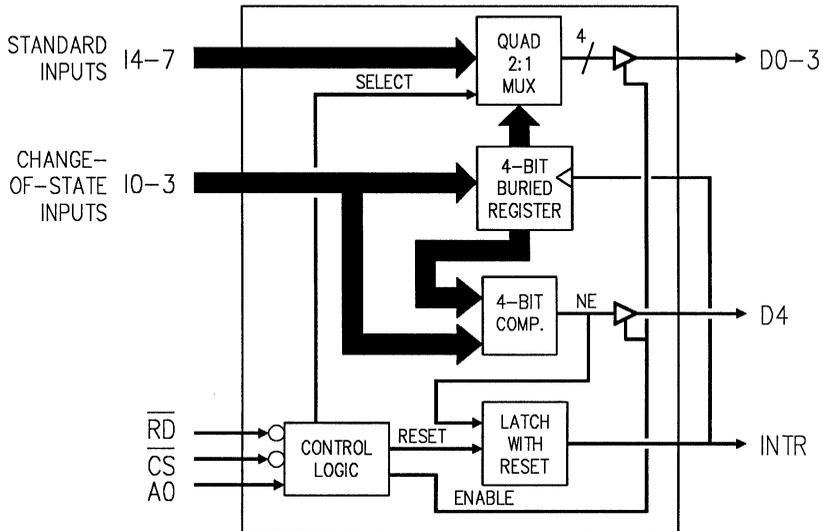
Figure 6-32, Logic schematic of V8CPORT.PSF
