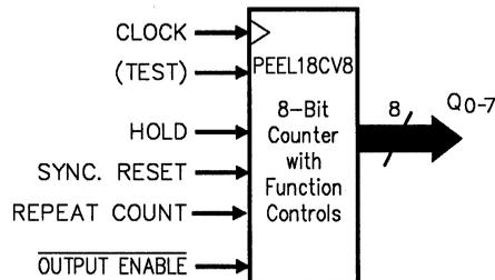
Figure 6-29, Block diagram of V8FCNTR.PSF
