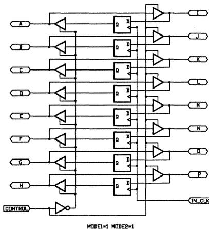
Figure 6-8, Logic schematic of BI\_PORT.PSF
