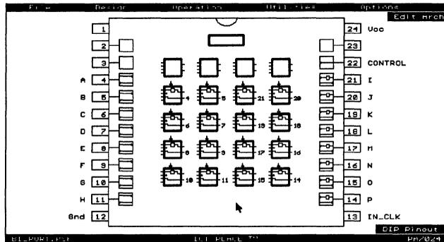
Figure 6-7, PLACE pin block diagram of BI\_PORT.PSF
