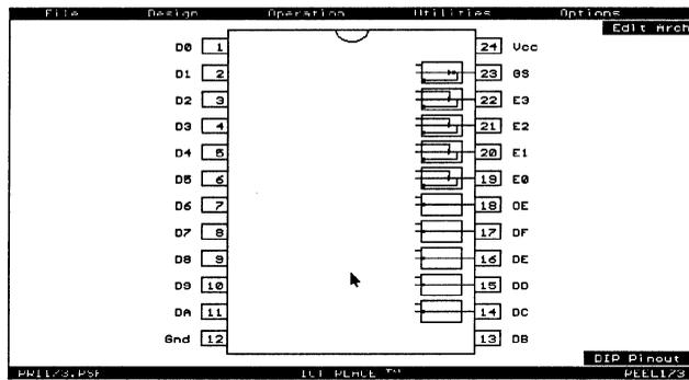
Figure 6-36, PLACE pin block diagram of PRI173.PSF
