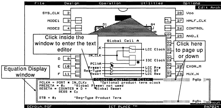
Figure 4-31, Equation Display window of the Global Cell A
