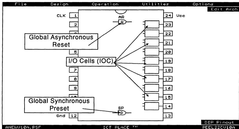
Figure 4-10, Pin Block Diagram of the PEEL22CV10A
