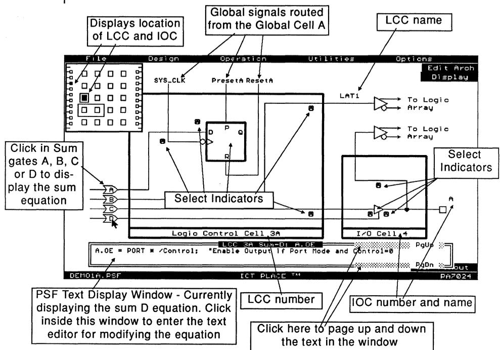
Figure 4-12, LCC and IOC screen of the PA7024
