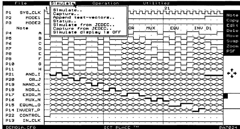
Figure 4-41, Simulate waveform screen
