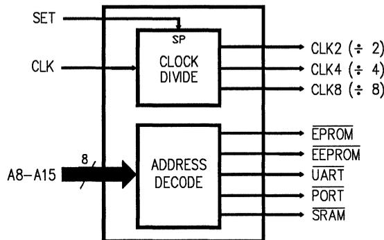
Figure 6-25, Block diagram of V8CLKADD.PSF
