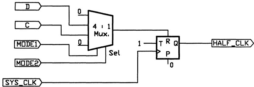
Figure 6-11, Logic schematic of a divide-by-2 clock design in COUNTER1.PSF
