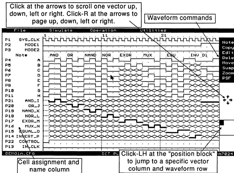
Figure 4-40, Simulate waveform screen
