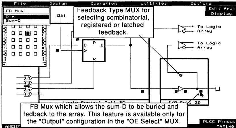
Figure 4-13, LCC and IOC screen of the PA7140
