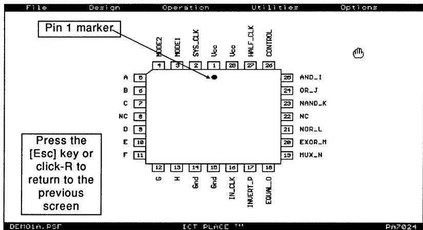
Figure 4-36, PLCC package configuration for the PA7024
