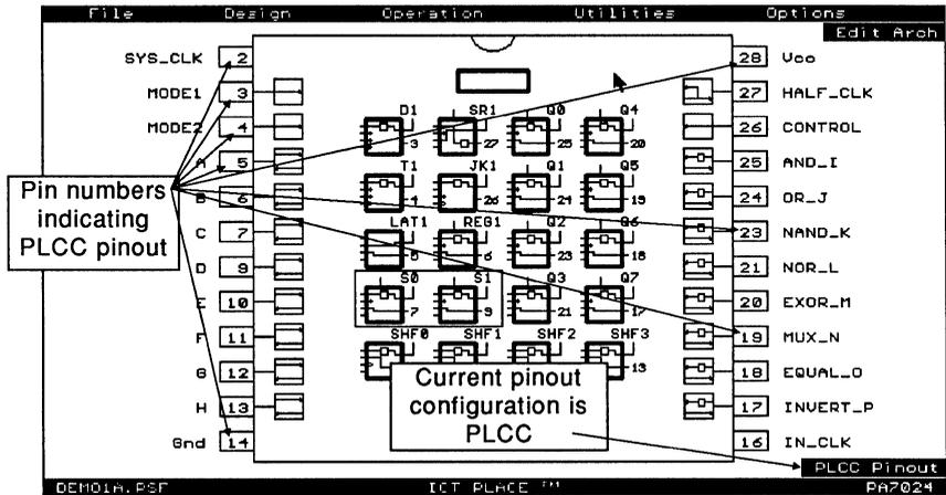
Figure 4-35, PLCC pinout for the PA7024
