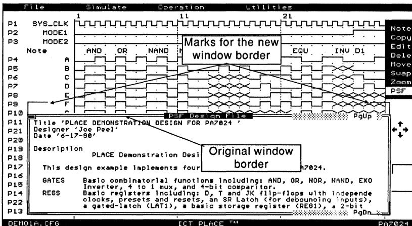
Figure 4-56, Sizing the PSF display window
