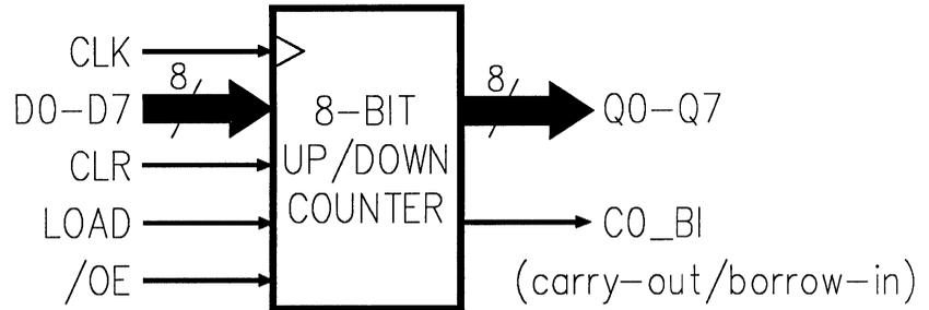
Figure 6-39, Block diagram of V10CNT8.PSF
