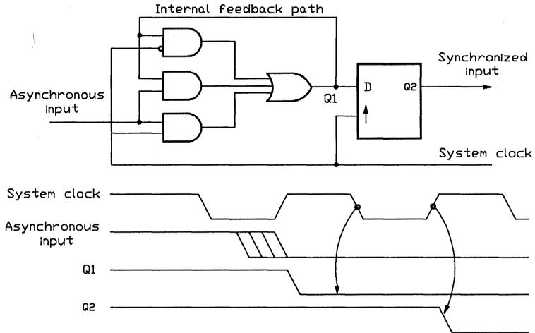
Figure 6-34, Synchronizer circuit in V8SYNC.PSF design
