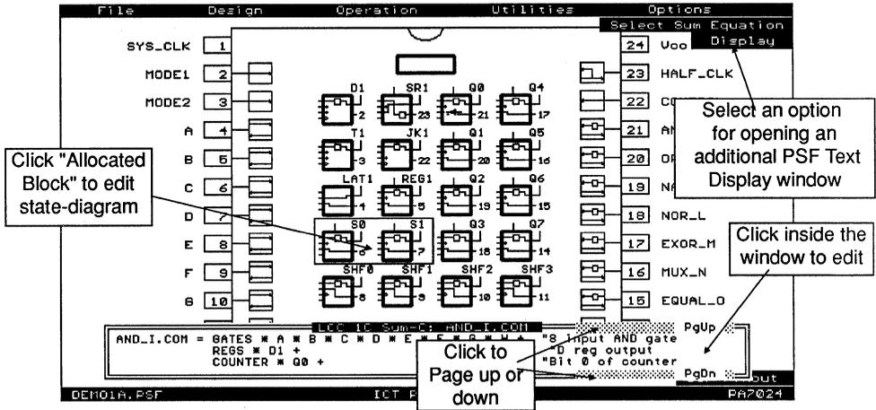
Figure 3-9, Selecting equations from the block diagram screen
