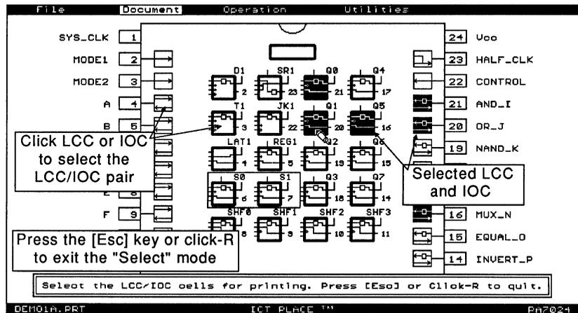
Figure 4-62, LCC/IOC "Select" screen for PA7024
