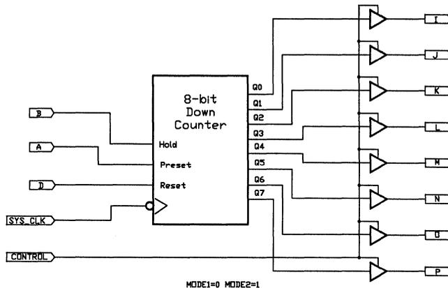
Figure 6-10, 8-bit counter logic schematic of COUNTER1.PSF
