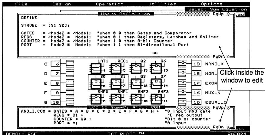
Figure 3-10, Selecting equations from the block diagram screen
