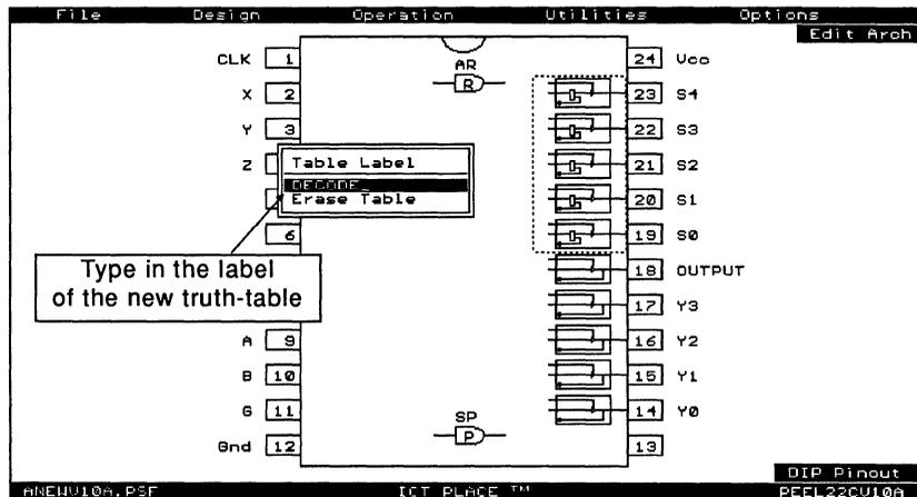
Figure 4-25, Entering the label for a new truth-table design
