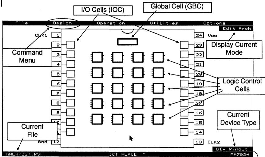
Figure 3-1, The PA7024 Pin Block Diagram screen in the Design Operation
