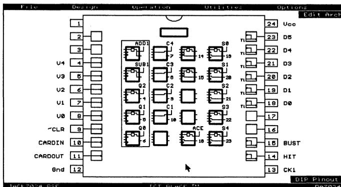
Figure 6-14, PLACE pin block diagram of JACK7024.PSF
