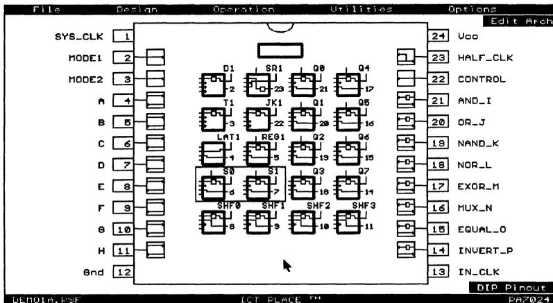
Figure 6-1, PLACE pin block diagram of DEMO1A.PSF
