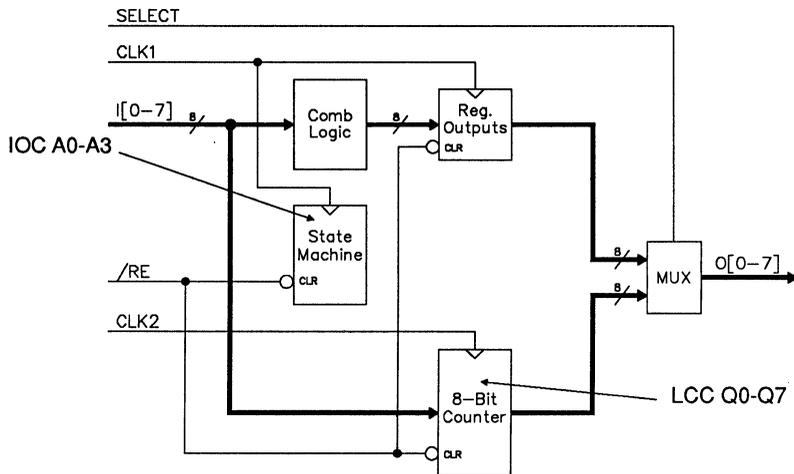
Figure 6-19, Logic block diagram of ST7128.PSF
