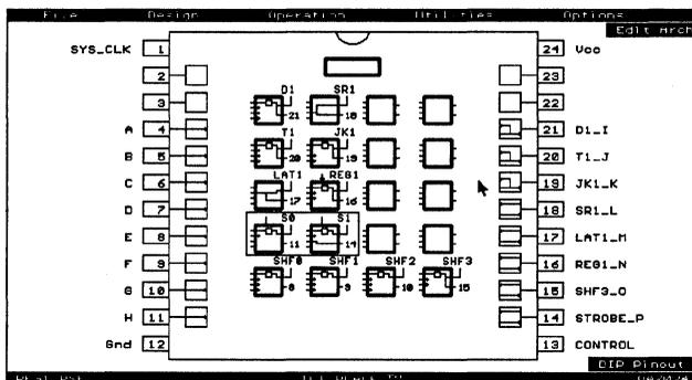
Figure 6-5, PLACE pin block diagram of REG1.PSF
