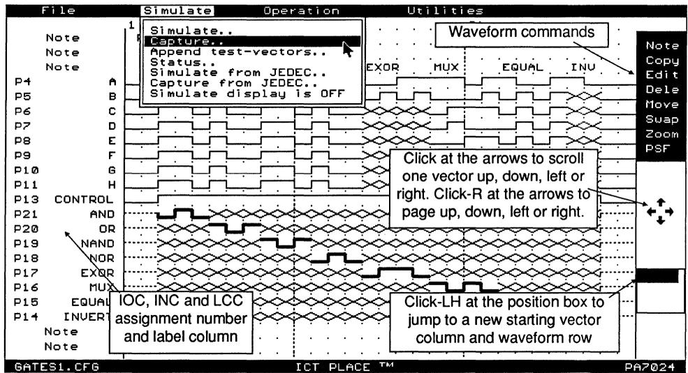
Figure 3-14, The Simulate Operation Main Screen
