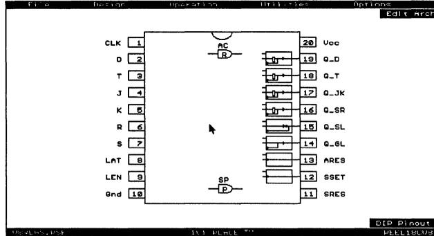
Figure 6-22, PLACE pin block diagram of V8REGS.PSF
