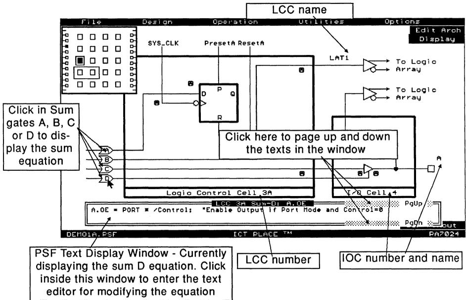
Figure 4-20, Editing equations in the LCC and IOC screen of the PA7024
