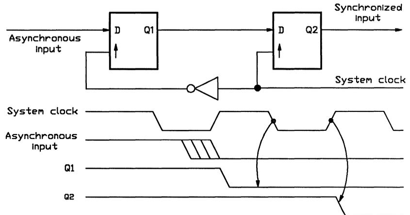
Figure 6-33, A common synchronizer circuit
