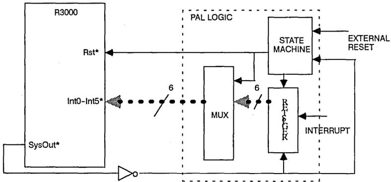
Figure 9: Block Diagram of Interrupt Controller on Reset
