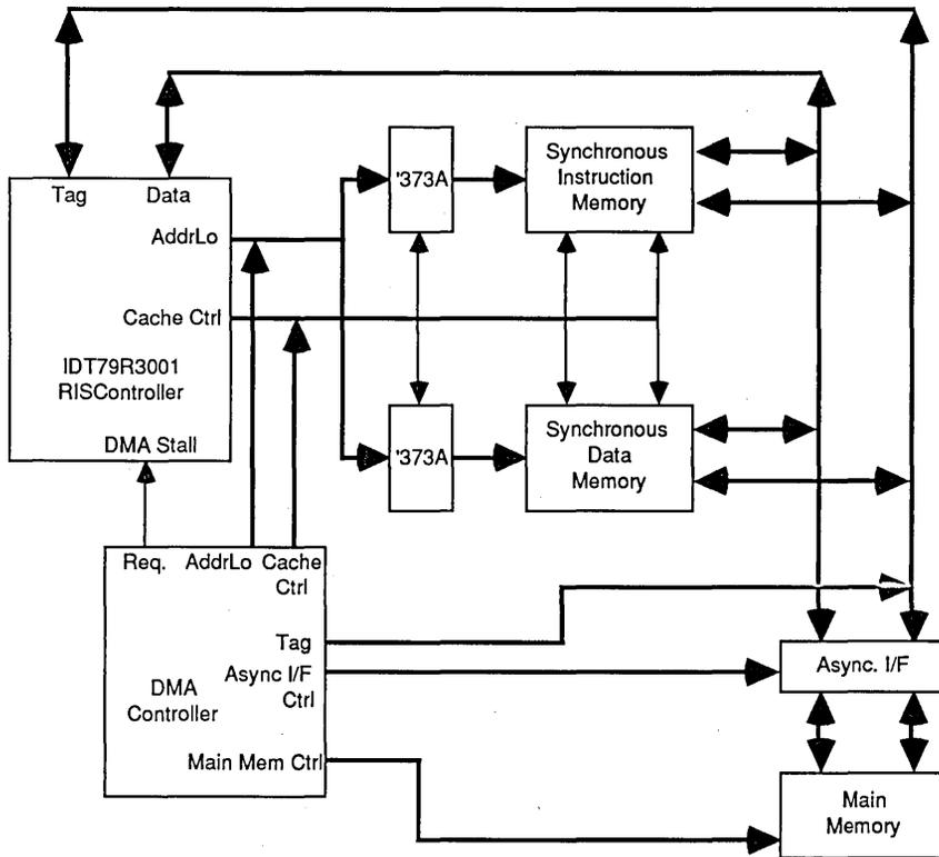
Figure 5. R3001 DMA Arbiter Interface
