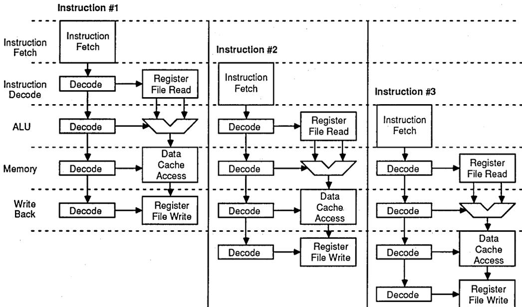
Figure 3. Pipeline Stages of the 79R3000
