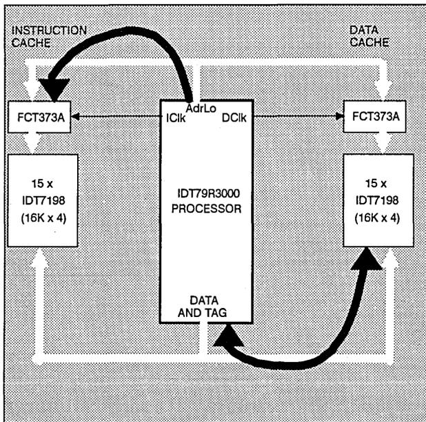
Figure 3b. Data and Instruction Caches During Phase 2
