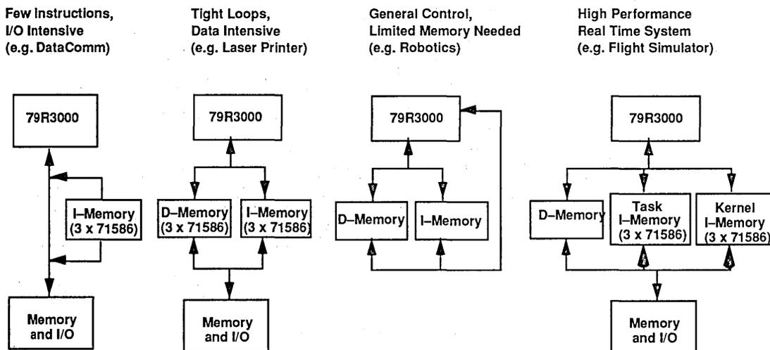
Figure 4. Typical 79R3000-based Systems
