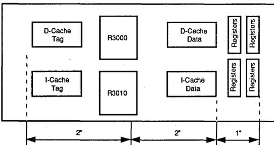
Figure 5.2. Surface Mount Board Layout of an R3001 System Using IDT71586 as Cache and Approximate Distances Between Devices
