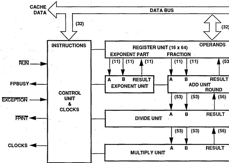
Figure 2. IDT79R3010 Floating-Point Accelerator
