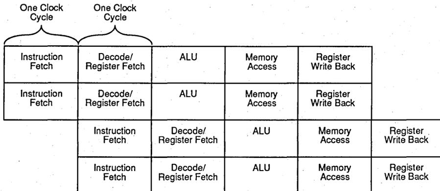
Figure 2. Superscalar RISC Pipeline
