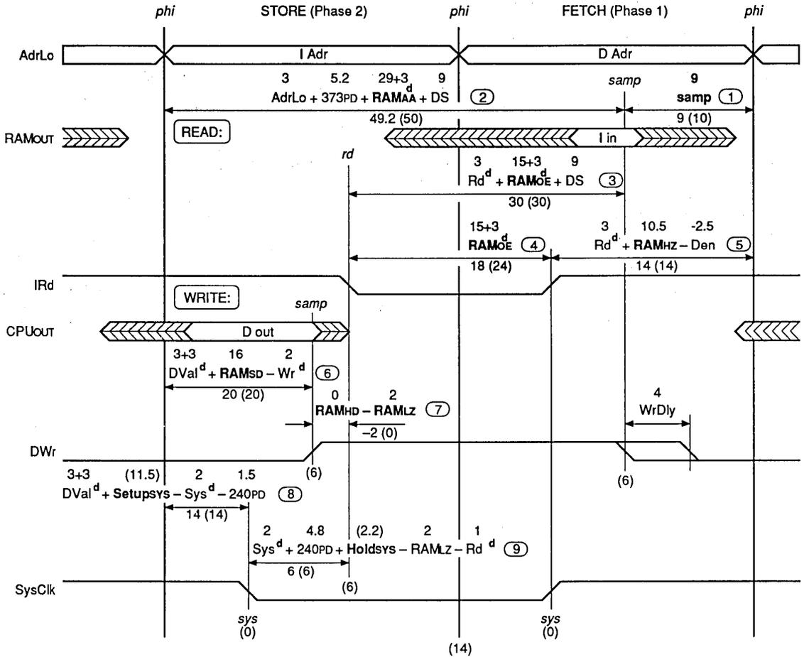
Figure 7. Cache Timing Diagram for a 16MHz IDT79R3000
