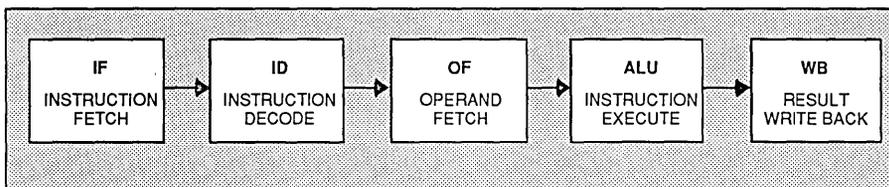
Figure 1. Stages of a Typical R3000 Instruction Pipeline
