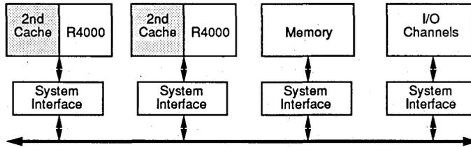
Figure 4. R4000-Based Multi-Processing System
