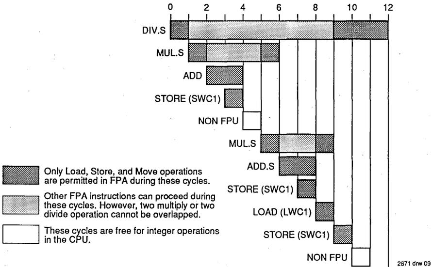
Figure 9. Examples of Overlapping Floating Point Operation
