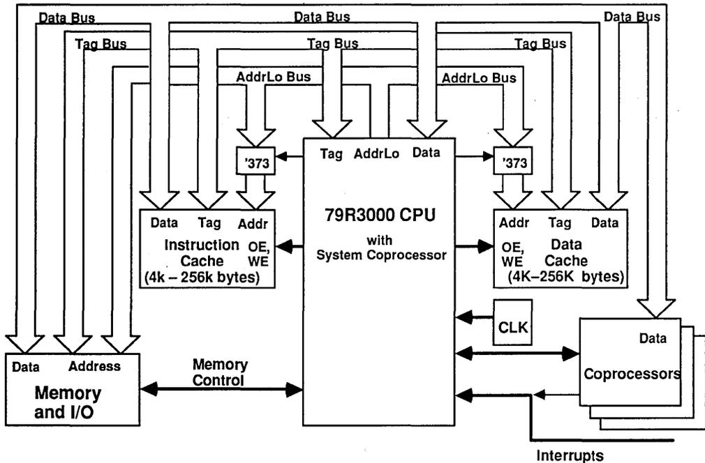
Figure 1. Typical 79R3000 Based System
