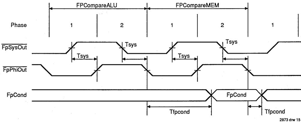
Figure 11. Floating Point Condition Timing
