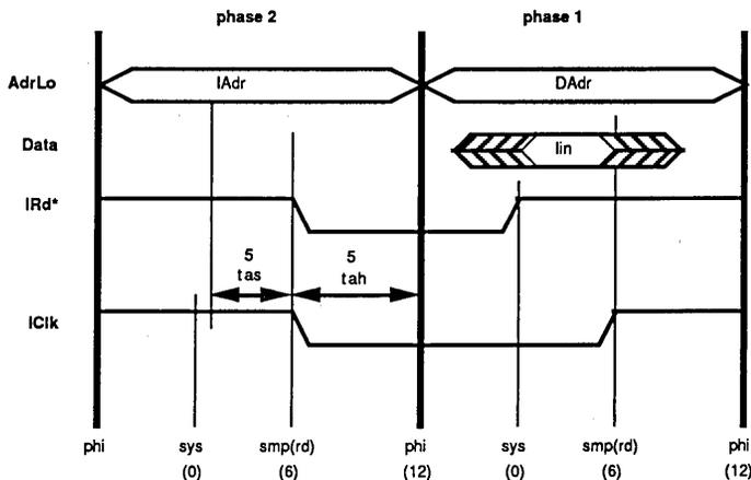
Figure 5.5. Address Setup and Hold Timing for a Latched RAM (25 MHz R3001)
