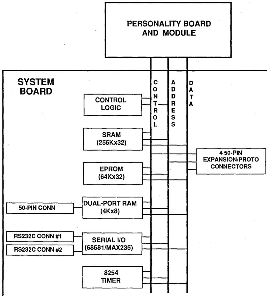
Block Diagram of the 7RS300 Series Prototyping Platforms
