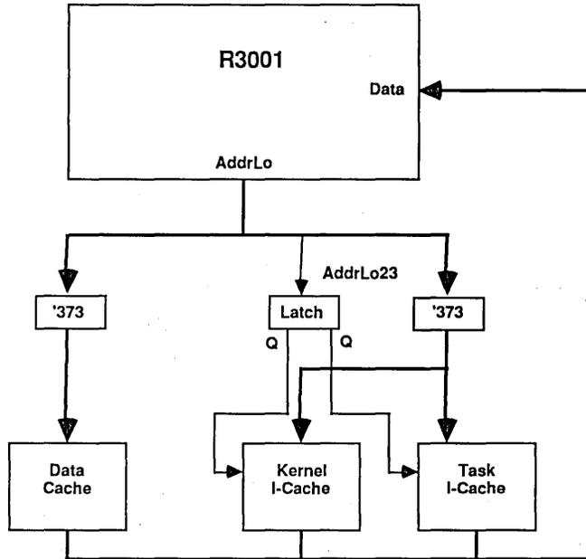
Figure 7. R3001 Real-Time, Cache Based System
