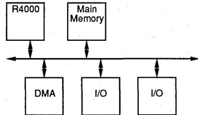
Figure 5. R4000-Based Embedded System
