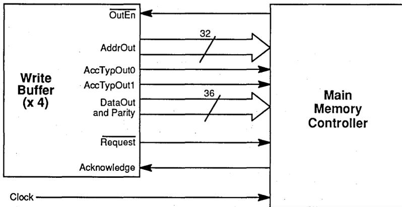
Figure 5. Write Buffer — Main Memory Interface
