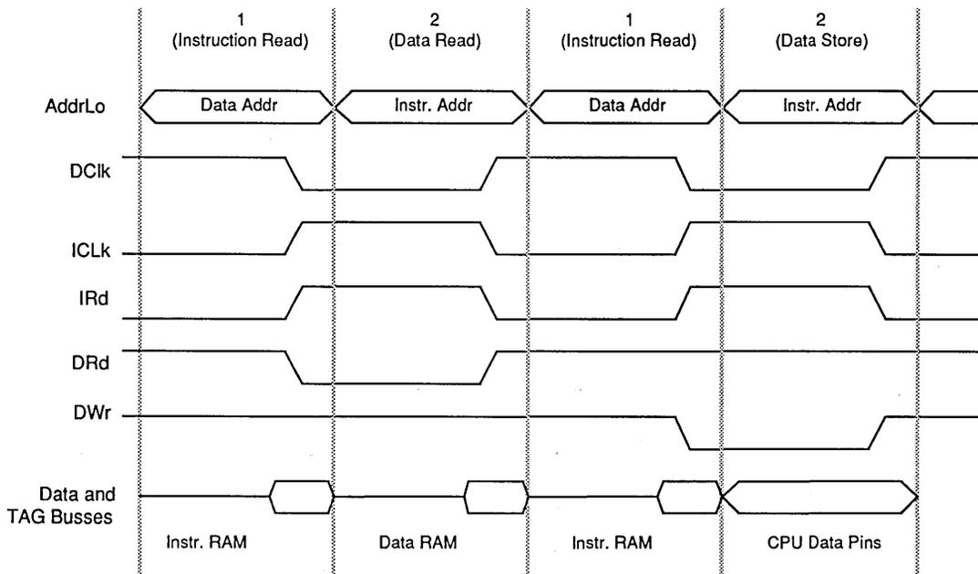
Figure 3. R3001 Synchronous Memory Interface Operation
