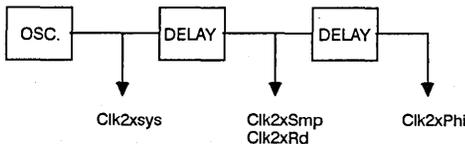
Figure 6. Tap Settings for the Clock Inputs
