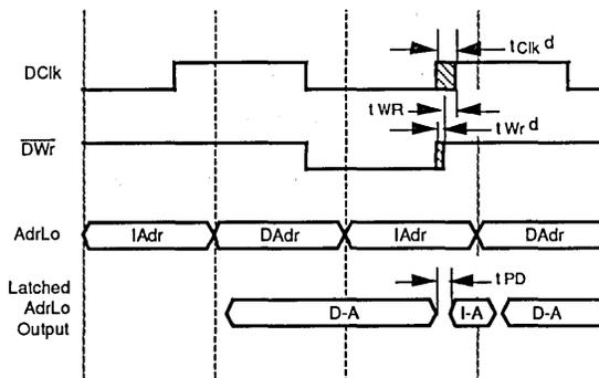
Figure 4.10b. Write Recovery Timing
