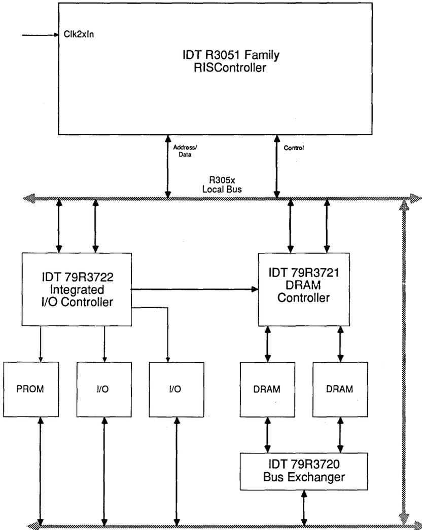
Figure 10. R3051 Family Chip Set Based System
