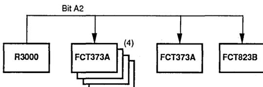
Figure 4.3. Block Diagram Showing Various Devices Connected to One Address Bit
