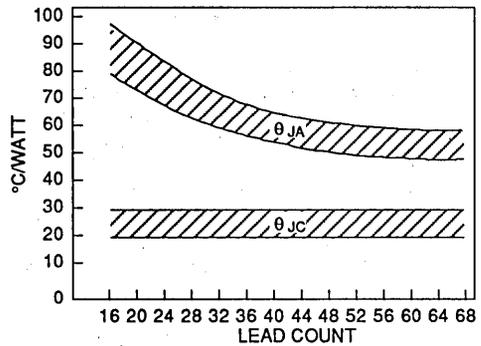
Thermal Resistance of PLCC/SOIC Packages
