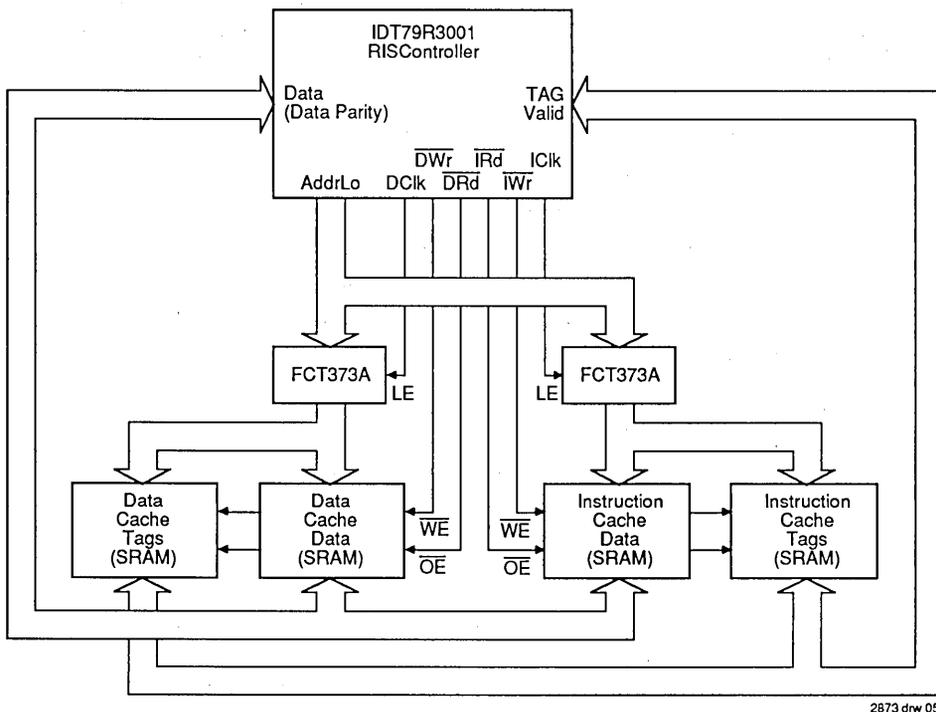
Figure 5. IDT79R3001 Synchronous Interface
