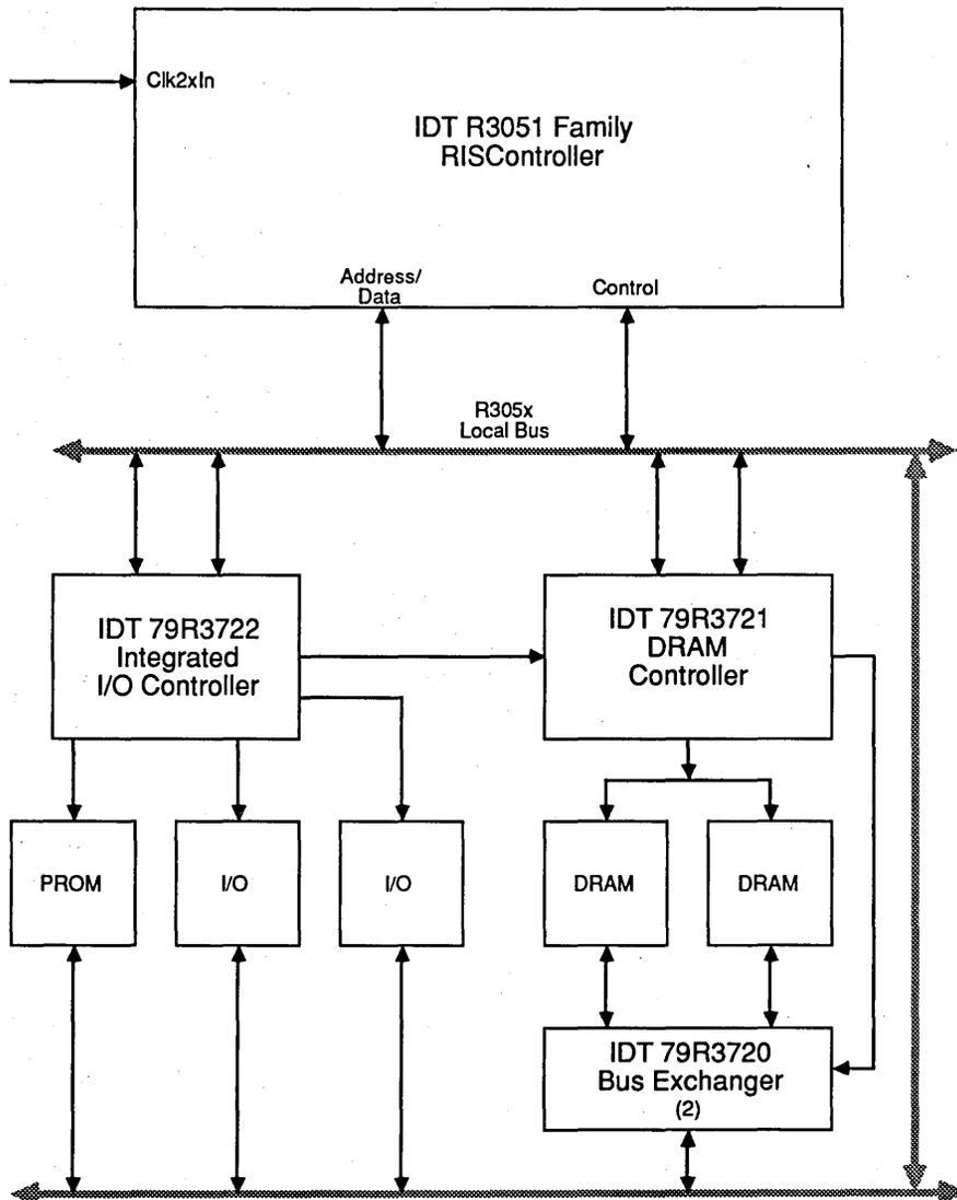
Figure 2. Bus Exchanger Used in R3051 Family System
