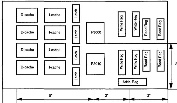
Figure 4.5. Board Layout for a Through-Hole Design of an R3001 Cache Subsystem
