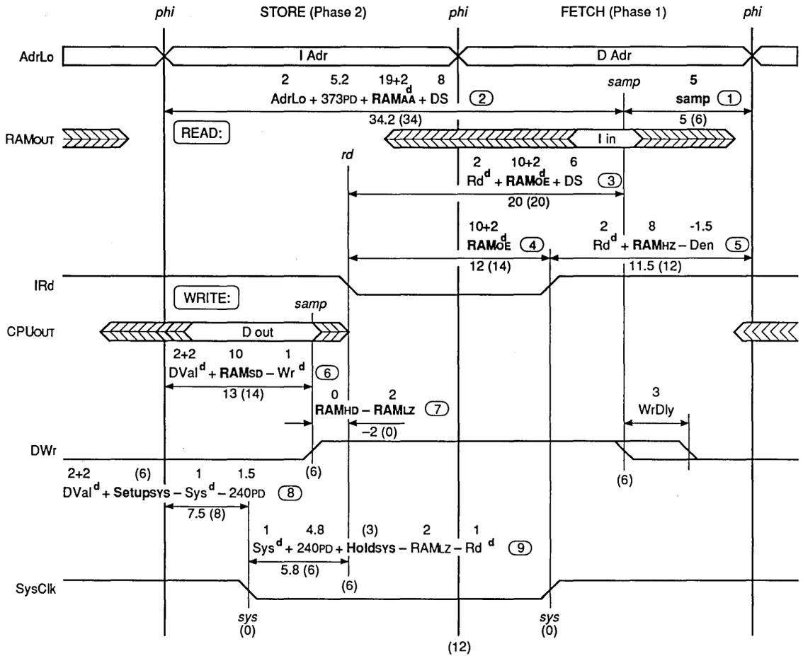
Figure 9. Cache Timing Diagram for a 25MHz IDT79R3000
