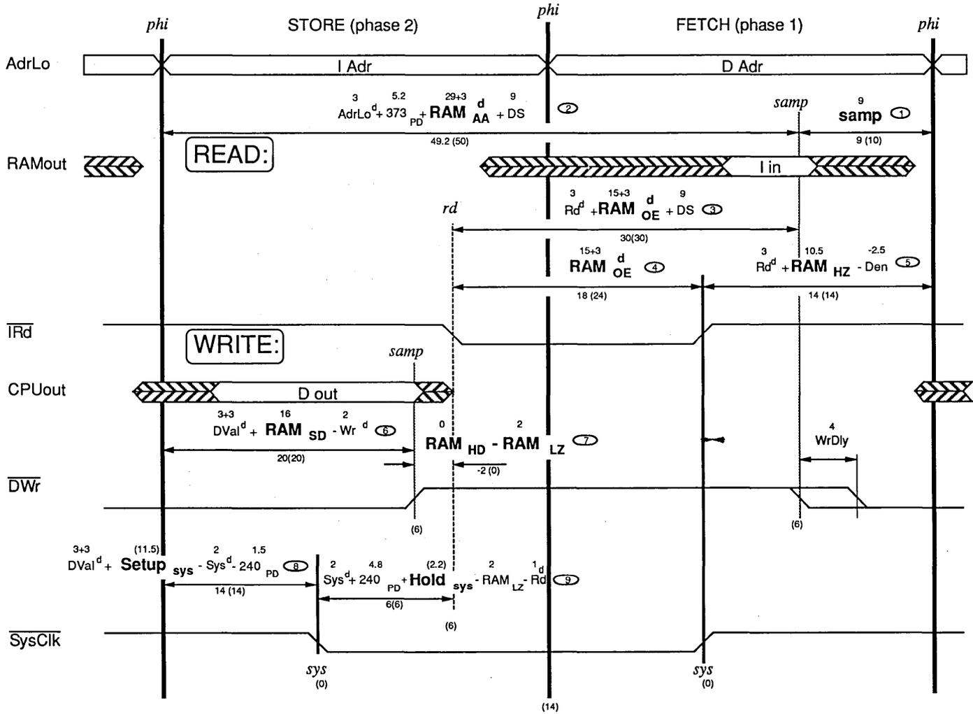
Figure 4.6. Cache Timing Diagram for a 16 MHz R3001
