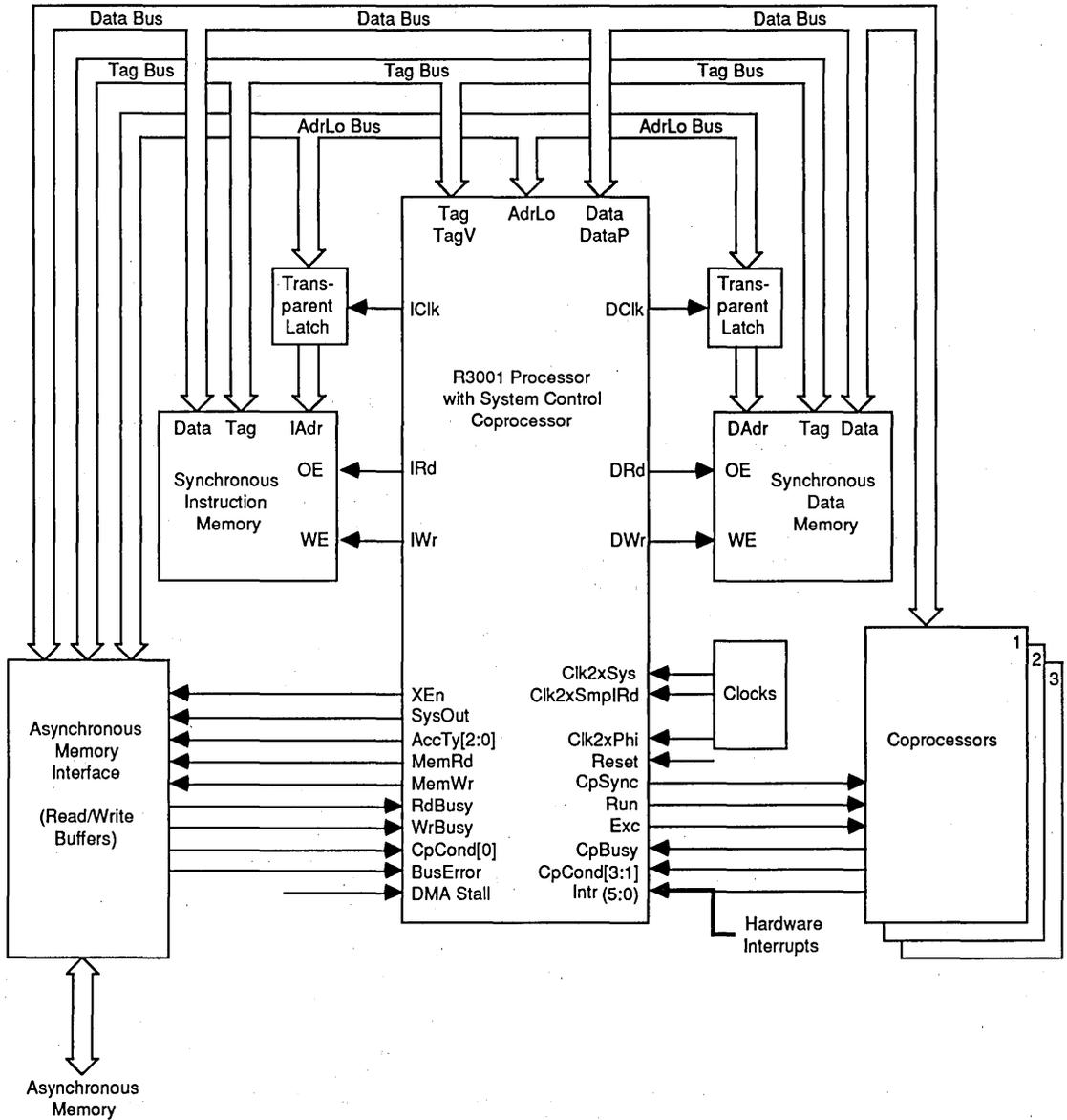
Figure 2. Memory Interfaces of IDT's R3001
