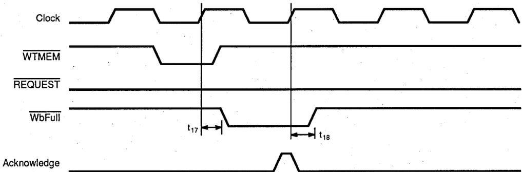
Figure 10.  $\overline{WbFull}$  Signal Timing Specifications
