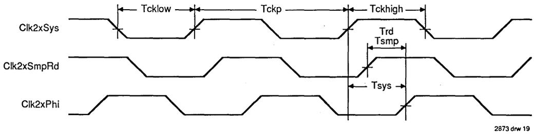
Figure 16. Input Clock Timing
