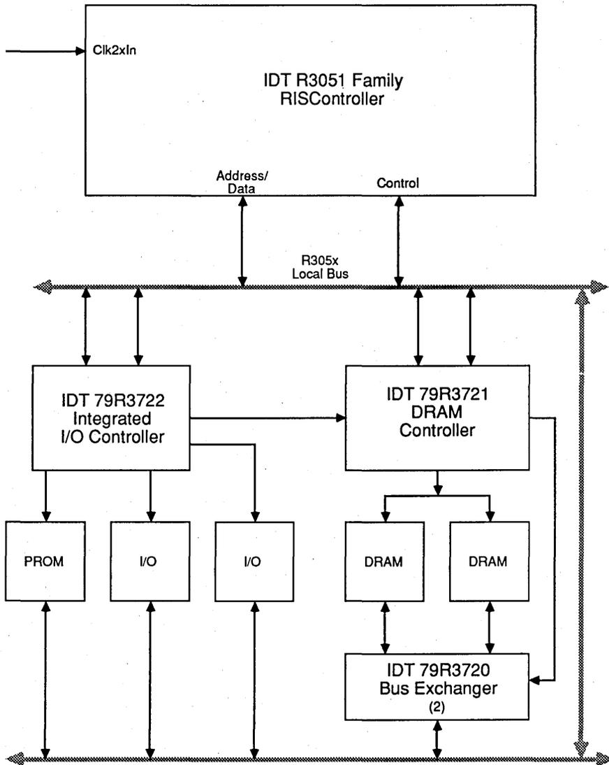
Figure 2. Use of R372x RISChipset in R3051 Family System
