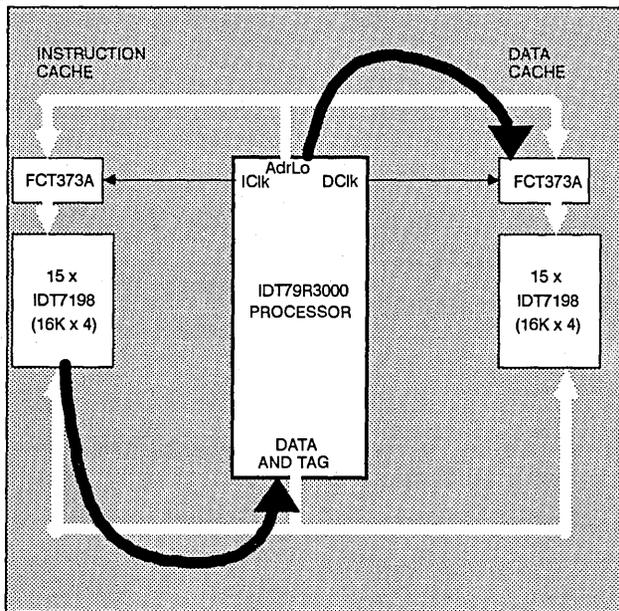
Figure 3a. Data and Instruction Caches During Phase 1
