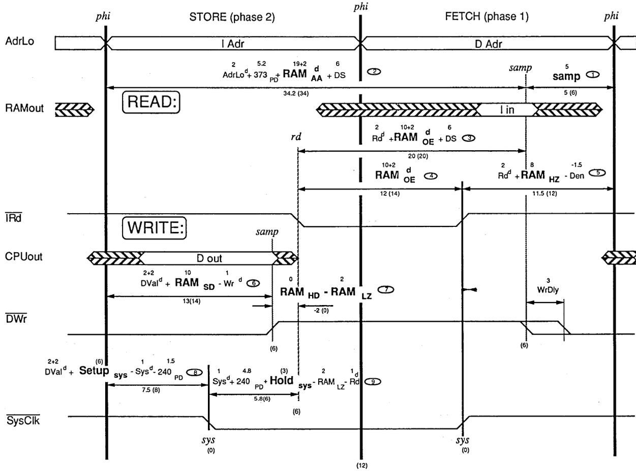
Figure 4.8. Cache Timing Diagram for a 25 MHz R3001
