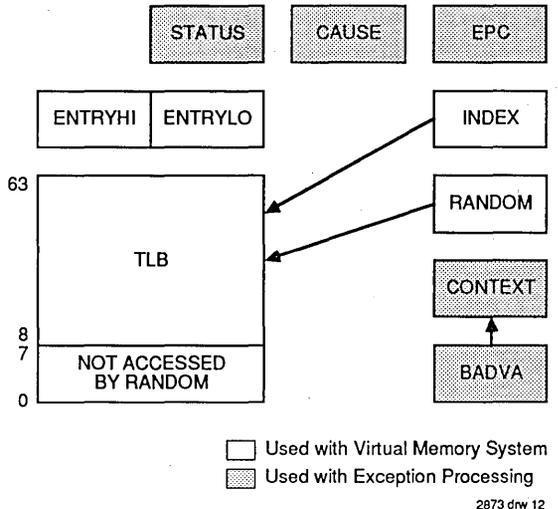
Figure 12. The System Control Co-processor (CP0) Registers
