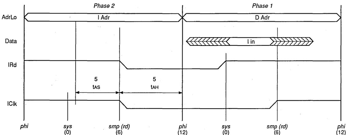
Figure 17. Address Setup and Hold Timing for a Latched RAM (25MHz IDT79R3000)
