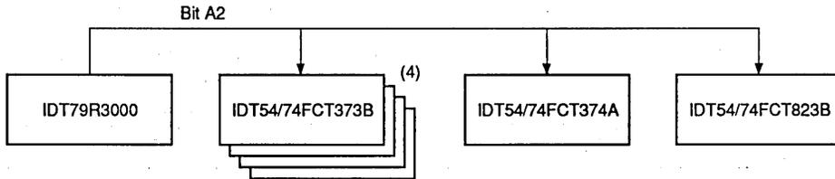
Figure 4. Block Diagram Showing Various Devices Connected to One Address Bit
