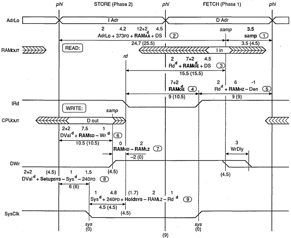
Figure 10. Cache Timing Diagram for a 33MHz IDT79R3000
