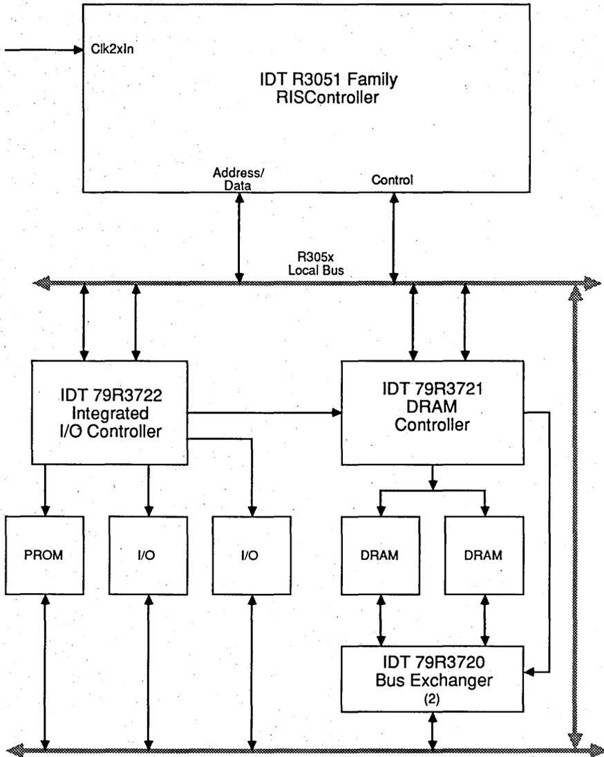
Figure 2. R3051 and RISChipset in an Embedded System
