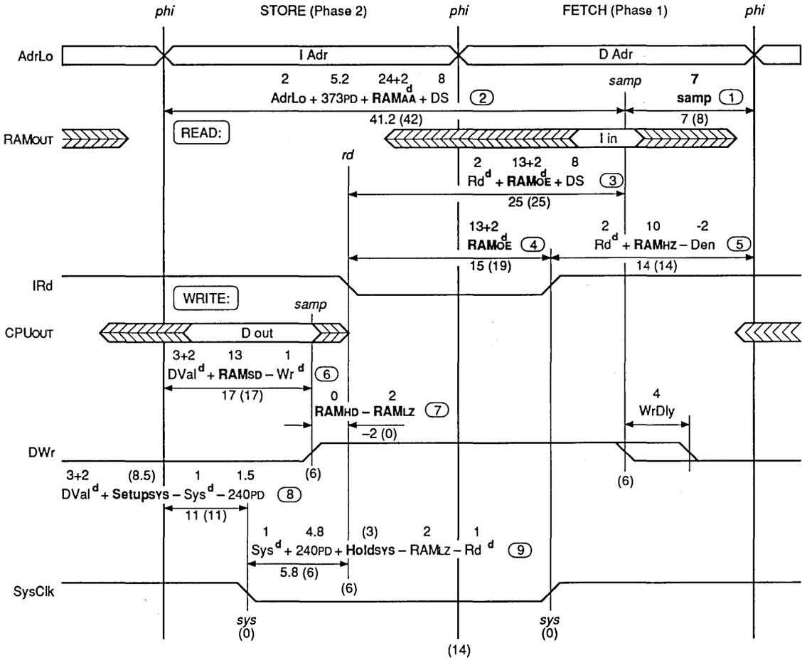
Figure 8. Cache Timing Diagram for a 20MHz IDT79R3000
