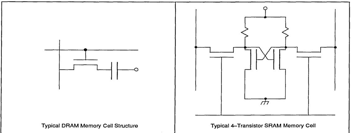
Figure 3. DRAM Memory Cell Structure and SRAM Memory Cell Structure
