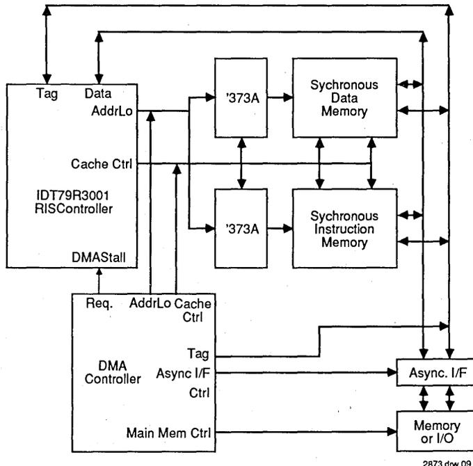
Figure 9. IDT79R3001 DMA Interface
