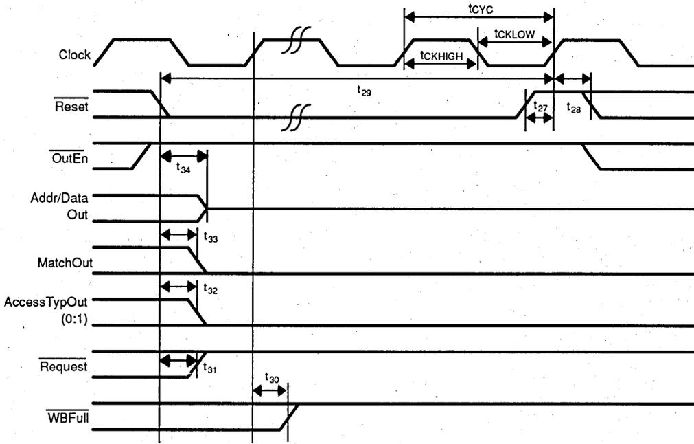
Figure 14. Reset Timing
