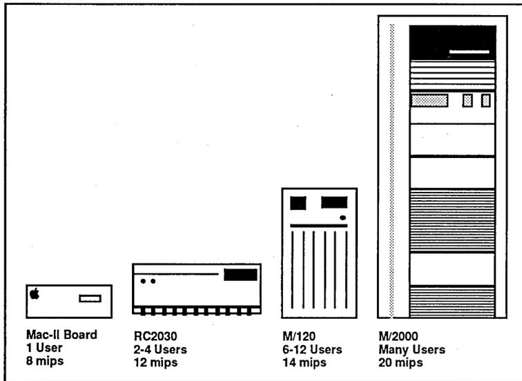
Figure 5. Range of SPP Host Development Systems for the IDT 79R3000
