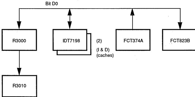
Figure 4.4. Block Diagram Showing Various Devices Connected to One Data Bit
