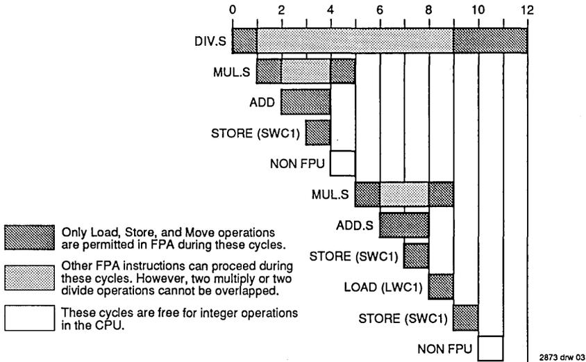
Figure 3. Examples of Overlapping Floating Point Operation
