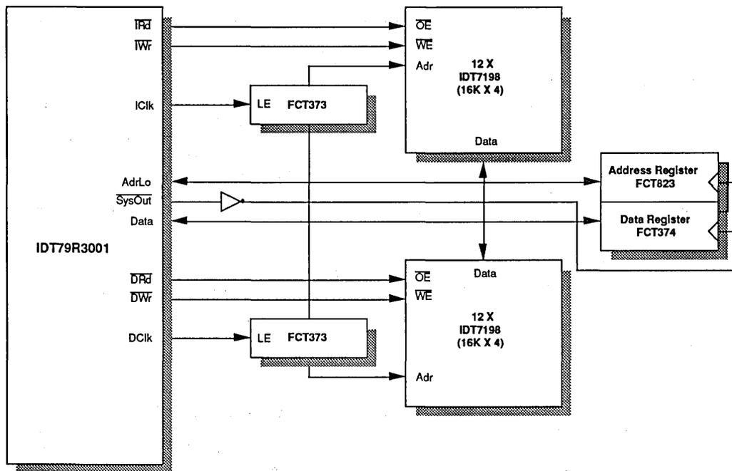
Figure 4.1. Block Level Diagram of a Cache Subsystem with the R3001 Using IDT7198 16K x 4 to Function as Cache (the R3010 is not shown in this figure)
