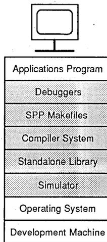
Figure 3. Using SPP to Develop Stand-Alone Applications on the Host System
