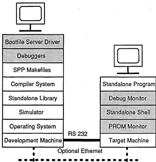
Figure 4. Using the SPP During Hardware/Software Integration
