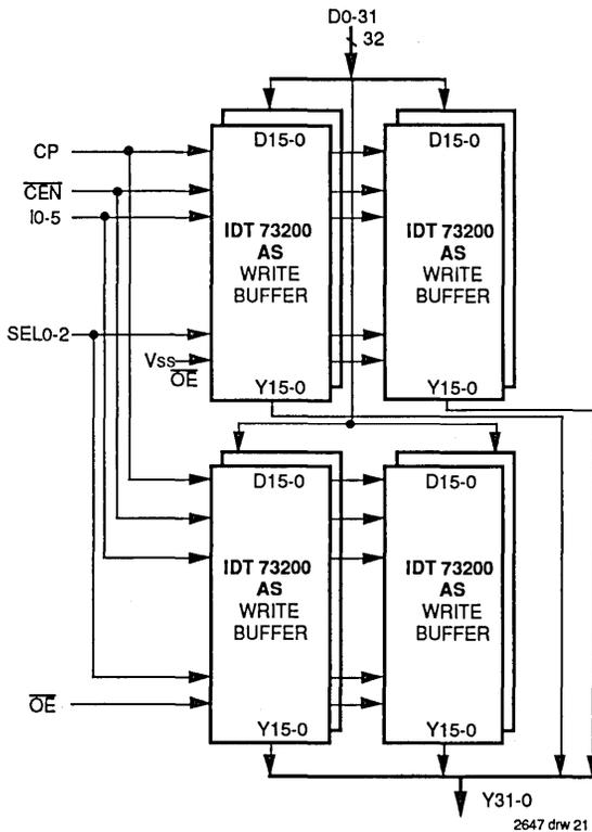
Figure 6. 16-Deep and 32-Wide Write Buffer Using IDT73200s
