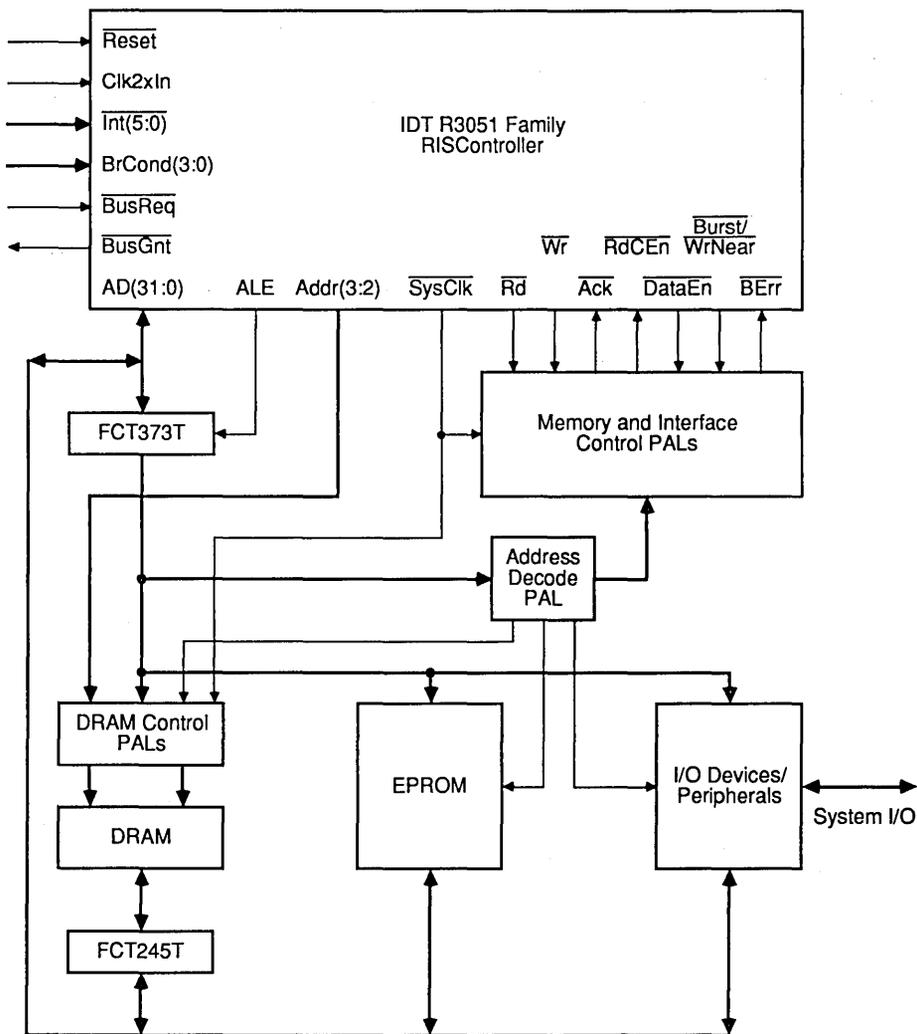
Figure 9. Typical R3051 Family Based System
