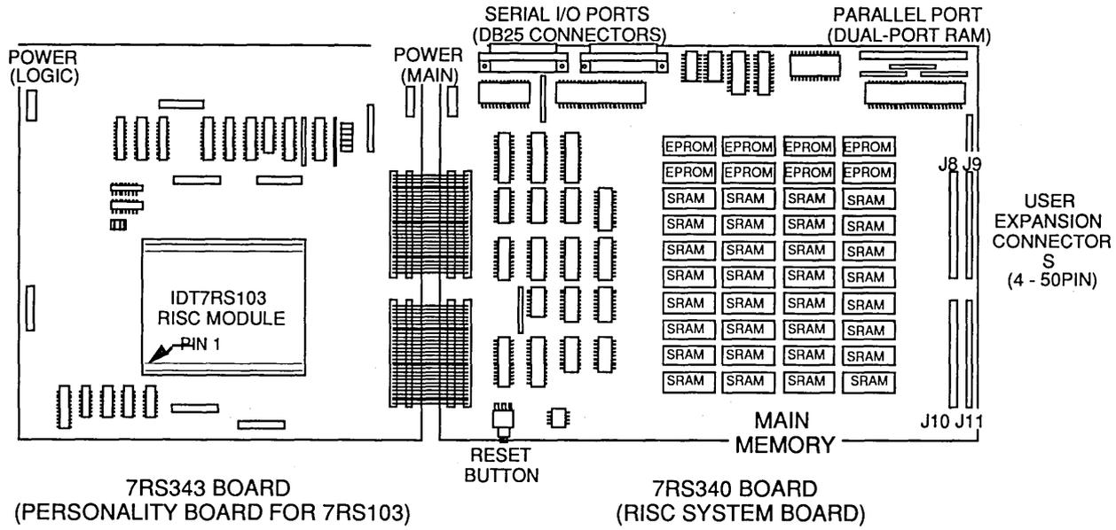
Layout of the series 300 Prototyping Platform.
