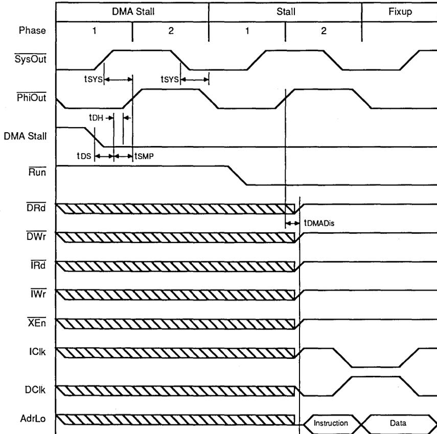
Figure 24. Entering DMA Stall
