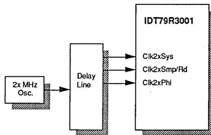
Figure 3.1. Three-Phase Clock Input to the R3001
