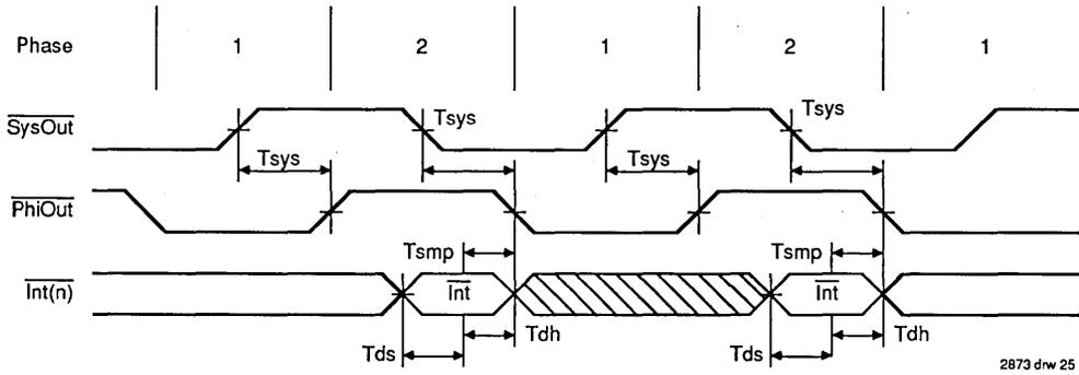
Figure 22. Interrupt Timing
