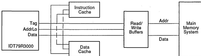
Figure 1. Typical Memory Subsystem IDT79R3000
