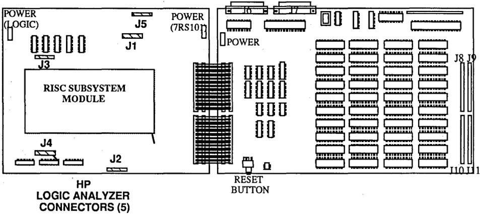
The 7RS301 Prototyping Platform for the 7RS101 Modules.
