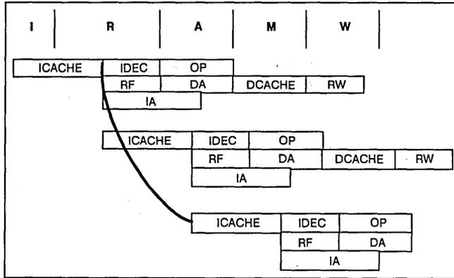
Figure 4. Pipeline Stages in the R3000
