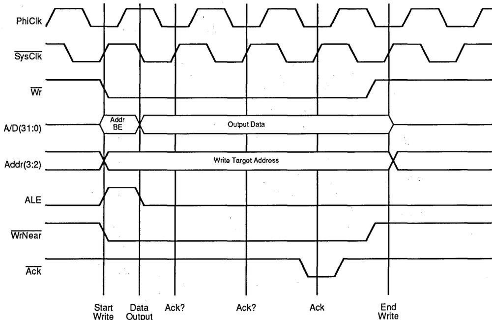
Figure 5. IDT R3051 Family Write Operation (Two Bus Wait Cycles)
