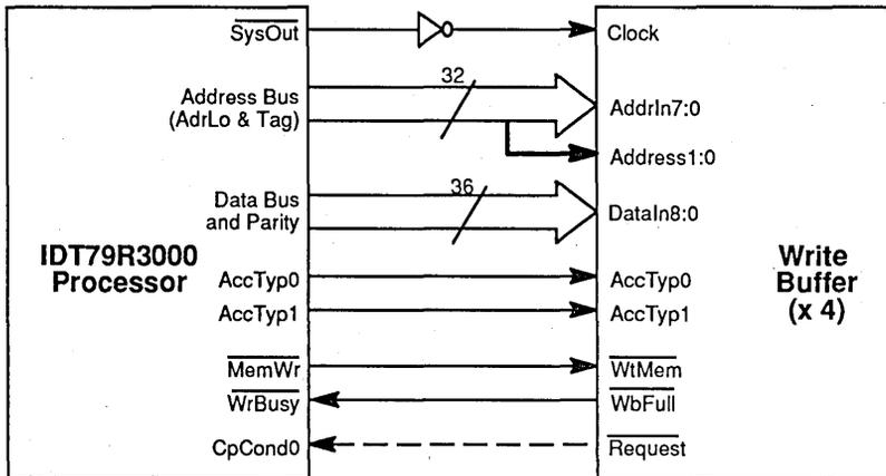
Figure 2. Write Buffer — IDT79R3000 Processor Interface
