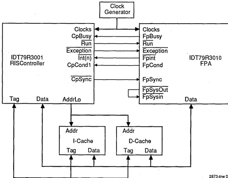
Figure 8. IDT79R3001 Interface to IDT79R3010 Floating Point Co-Processor
