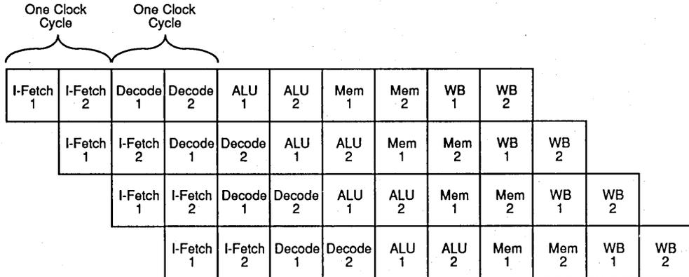
Figure 3. Superpipelined RISC Pipeline
