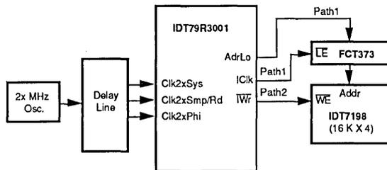
Figure 4.10a. Circuit Showing IWwr and ICik Signals to Latch and SRAM
