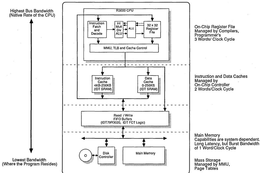
Figure 1. Hierarchies of Memory in an R3000-Based System
