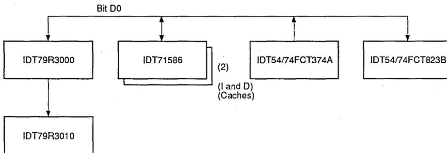
Figure 16. Devices Data Bus Connected to the IDT79R3000
