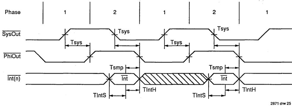
Figure 21. Interrupt Timing
