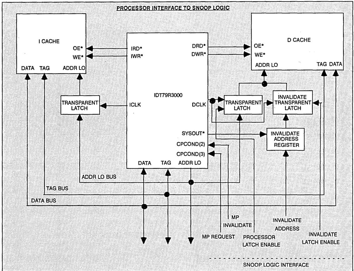
Figure 3. Processor Interface to the Snoop Control Logic
