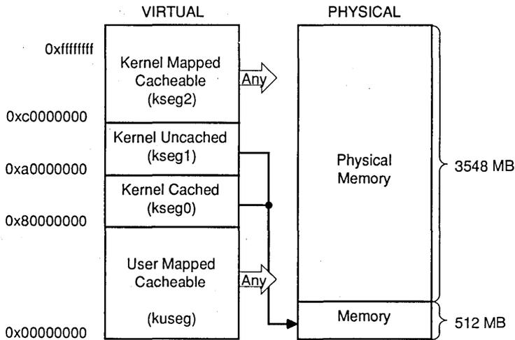
Figure 3. Virtual to Physical Mapping of Extended Architecture Versions
