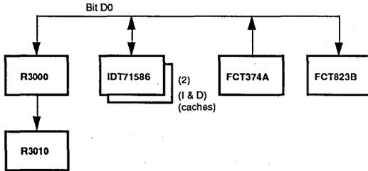
Figure 5.4. Devices Data Bus of the R3001 is Connected to
