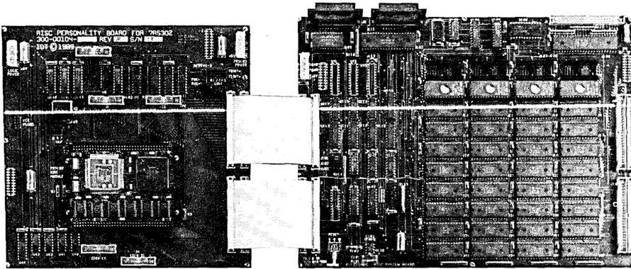
A Module Prototyping Platform.
