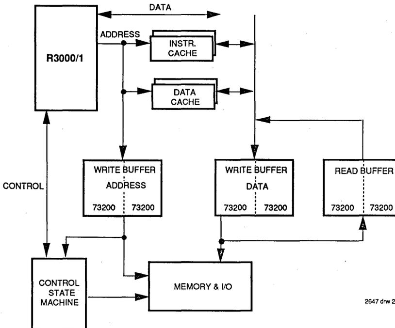
Figure 7. R3000/1 System with the Read-Write Buffers
