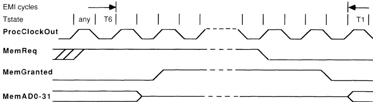
**Note :** MemReq is an asynchronous input signal and it is sampled internally. This sampling is effected by the current state of the external memory interface such that MemGranted will only be asserted at the end of any outstanding external memory cycle, including refresh.
