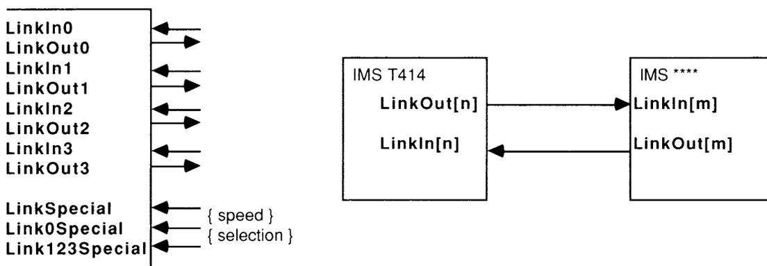
The T414 links wait until each full byte has been received before outputting the corresponding acknowledge packet. An acknowledge packet can be received at any time following the transmission of a data packet start bit.
