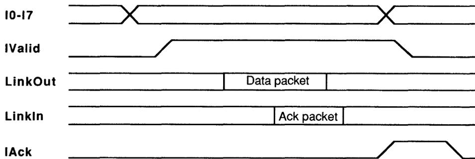
**IValid** and **IAck** provide a simple two wire handshake. Data is presented to the link adaptor on **I0-17**, and **IValid** is taken high to commence the handshake. The link adaptor transmits the data through the serial link, and acknowledges receipt of the data on **IAck** when it has received the acknowledgment from the serial link. **IValid** is then taken low, and the link adaptor completes the handshake by taking **IAck** low.
