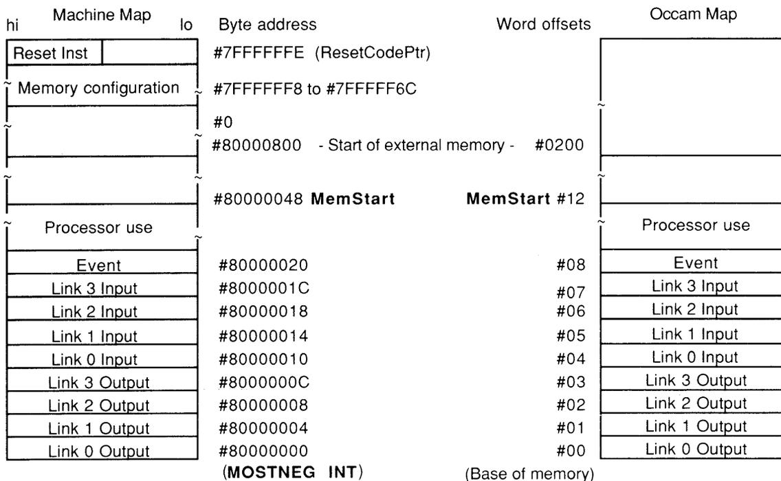
This schema for calculating addresses is used to provide word length independent code, as though memory were an array of type **INT** ([ ] **INT**). The link addresses will always be found within the lower bounds of the memory array space.
