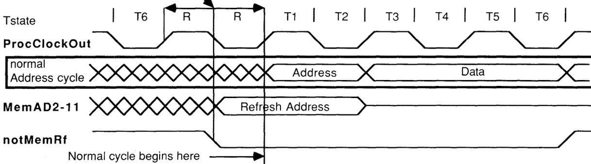
Refresh can be configured to be enabled or disabled. If Refresh is enabled, the interval between refresh cycles can be configured to be 18, 36, 54 or 72 periods of the input clock signal ClockIn.
