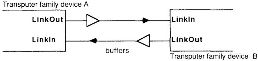
If buffers are used their overall propagation delay, TPD, should be stable within the skew tolerance.
