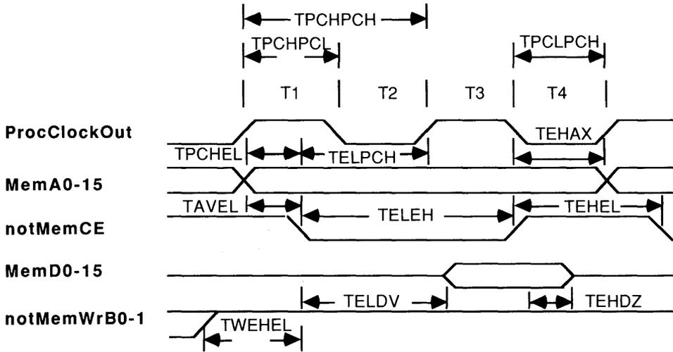
A.C timing for a single Wait State during a Write Cycle.
