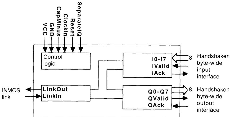
In mode 1 the link adaptor converts between an INMOS serial link and two independent fully handshaken byte-wide interfaces. One interface is for data coming from the serial link and one for data going to the serial link.
