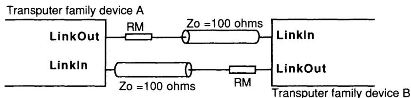
For long wires, approximately >30 cm, then a 100ohm transmission line should be used with series matching resistors.
