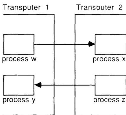
To provide synchronised communication, each message must be acknowledged. Consequently, a link requires at least one signal wire in each direction.
