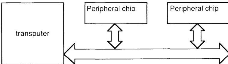
In all three methods, the peripheral driver interfaces to the rest of the application via occam channels. Consequently, a peripheral device can be simulated by an occam process. This enables testing of all aspects of a transputer system before the construction of hardware.
