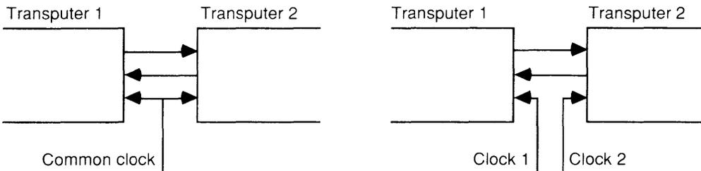
Link communication is not sensitive to clock phase. Thus, communication can be achieved between independently clocked systems as long as the communications frequency is the same.
