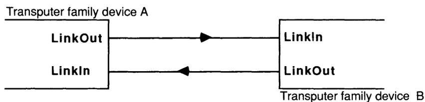
Direct connection is suitable for short distances on a printed circuit board.
