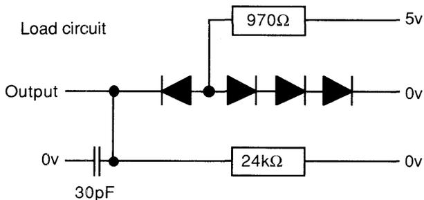
The load circuit approximates to two Schottky TTL loads, with total capacitance of 30 pF.
