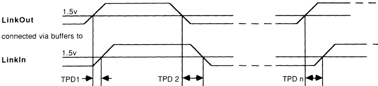
The absolute value of TPD is immaterial because data reception is asynchronous. However, TPD will vary from moment to moment because of ground noise, variation in the power supplies of buffers and the difference in the delay for rising and falling edges. This will vary the length of data bits reaching **LinkIn**. *Skew* is the difference between the maximum and minimum instantaneous values of TPD.
