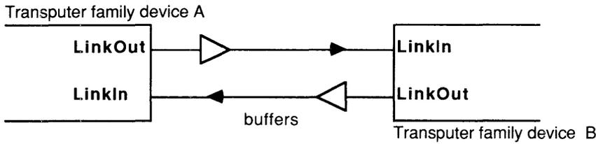
If buffers are used their overall propagation delay, TPD, should be stable within the skew tolerance.
