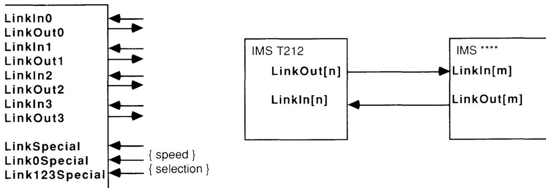
The T212 links wait until each full byte has been received before outputting the corresponding acknowledge packet. An acknowledge packet can be received at any time following the transmission of a data packet start bit.
