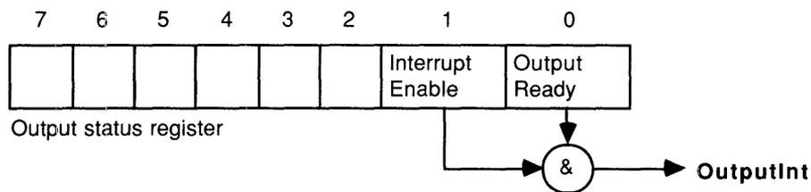
The output ready status bit indicates that the serial link is ready to send a byte of data. The bit is set high on reset, and when the link adaptor receives an acknowledgement from the serial link. It is reset low when a data byte is written to the output data register on the parallel interface. **OutputInt** is set high if both output ready and interrupt enable are set high. Output interrupt enable is set low on reset.
