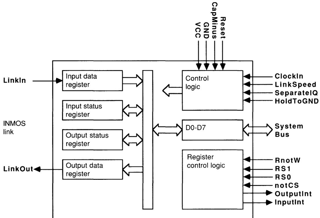
In mode 2 the link adaptor provides an interface between an INMOS serial link and a microprocessor system bus, via an 8-bit bi-directional interface.
