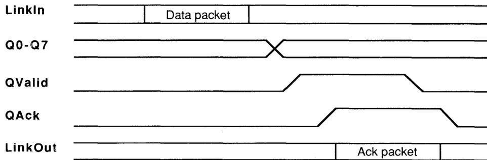
The link adaptor receives data from the serial link, presents it on **Q0-Q7**, and takes **QValid** high to commence the handshake. Receipt of the data is acknowledged on **QAck**, and the link adaptor then transmits an acknowledgement on the serial link. The link adaptor takes **QValid** low and the handshake is completed by taking **QAck** low.
