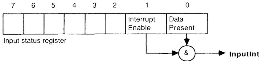
The data present status bit indicates that the serial link has received a byte of data. The bit is reset low when the data byte is read from the input data register on the parallel interface, this causes an acknowledgement to be transmitted on the serial link. **InputInt** is set high if both data present and interrupt enable are set high. Input interrupt enable and **data present** are both set low on reset.
