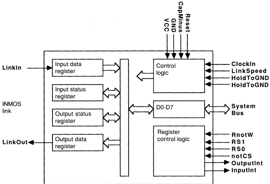
The C012 link adaptor provides an interface between an INMOS serial link and a microprocessor system bus, via an 8-bit bi-directional interface.
