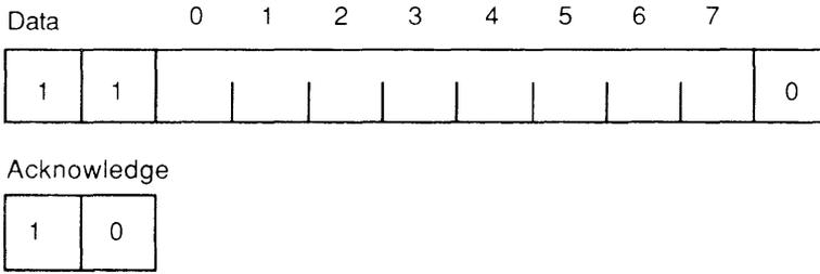
The links are designed to make the engineering of transputer systems straightforward. Board layout of two wire connections is easy to design and area efficient. All transputers will support a standard communications frequency of 10 Mbits/sec, regardless of processor performance. Thus transputers of different performance can be directly connected and future transputer systems will directly communicate with those of today.
