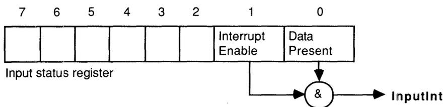
The data present status bit indicates that the serial link has received a byte of data. The bit is reset low when the data byte is read from the input data register on the parallel interface, this causes an acknowledgement to be transmitted on the serial link. **InputInt** is set high if both data present and interrupt enable are set high. Input interrupt enable and **data present** are both set low on reset.
