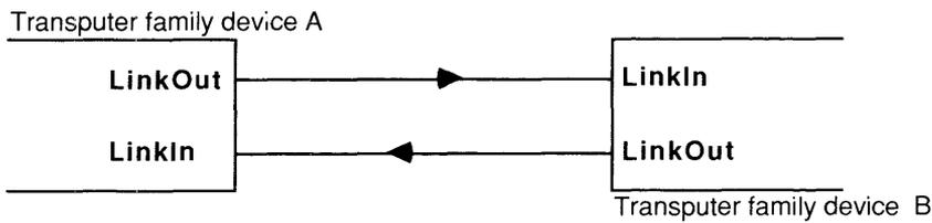
Direct connection is suitable for short distances on a printed circuit board.
