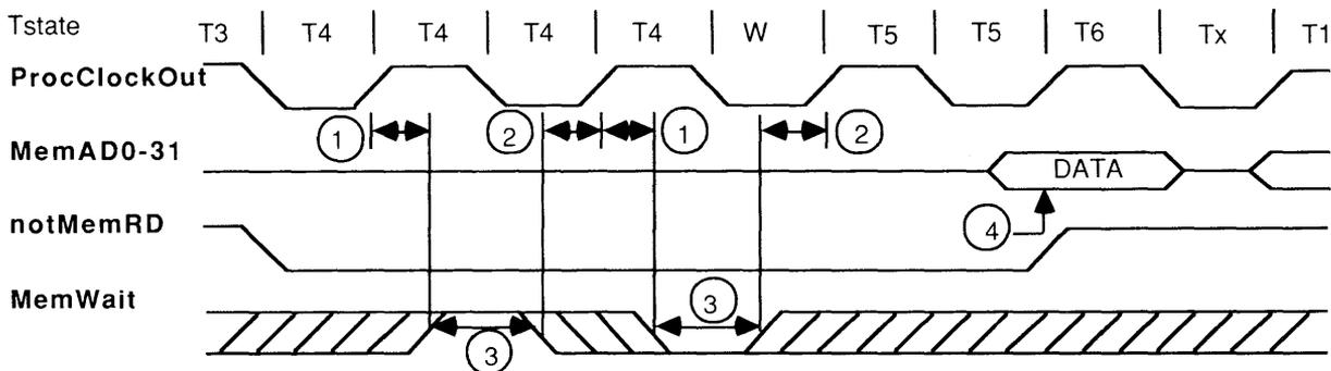
Cycle configured for long T4, with MemWait extending the cycle by two periods.
