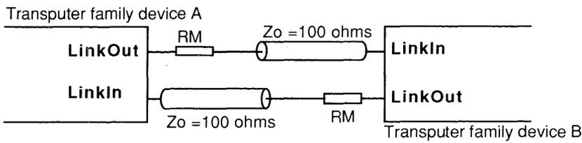
For long wires, approximately >30 cm, then a 100ohm transmission line should be used with series matching resistors.
