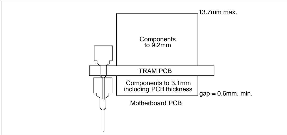
Figure 1.2 IMS B452 height specification
