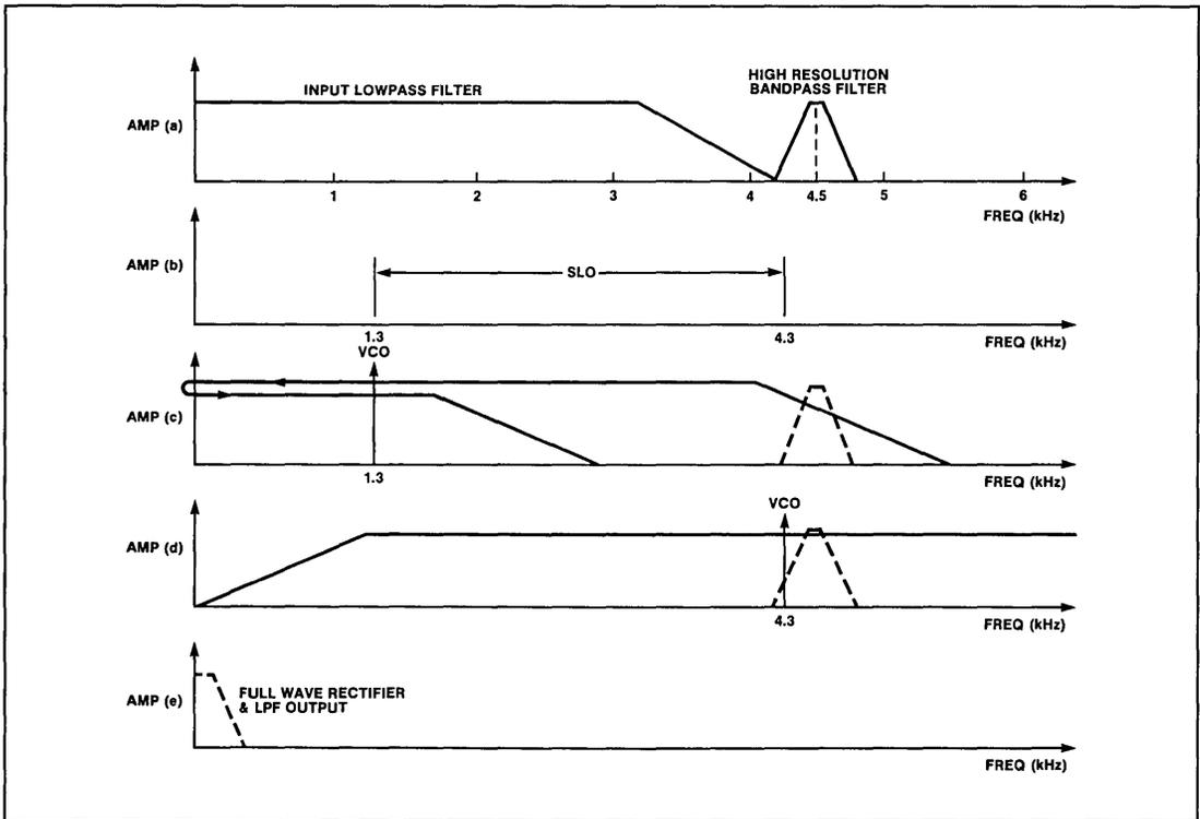
Figure 7-11. Spectrum Analyzer Design Frequency Domain Analysis
