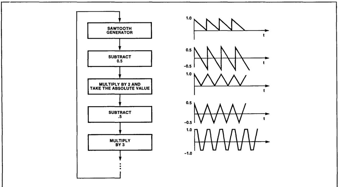
Figure 7-2. Waveform Shaper
