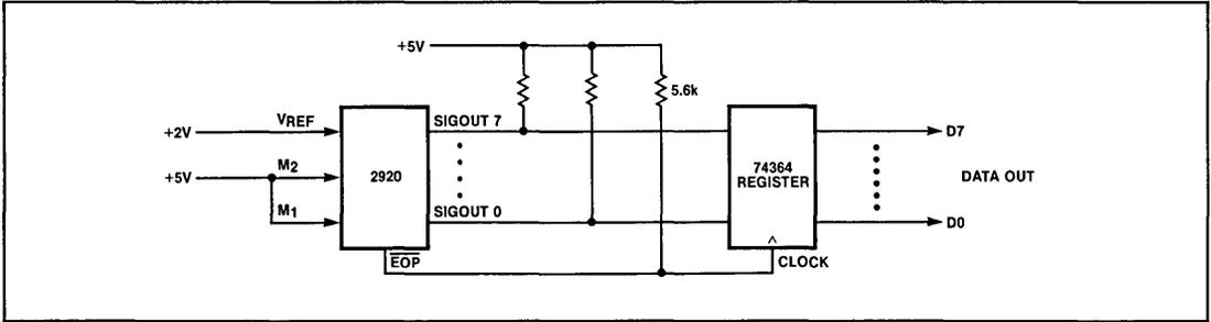
**Figure 6-4. Logic Diagram for Digital Output: Parallel**
