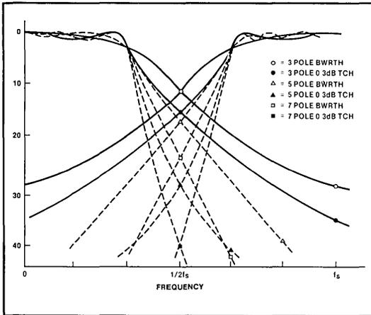
Figure 2-5. Effects of Filtering on Aliasing Noise
