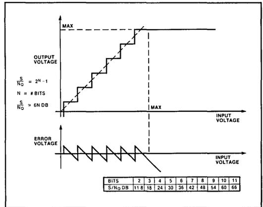
**Figure 2-9. Quantization Noise**
