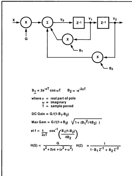
**Figure 5-12. Realization Of Complex Conjugate Pole Pair**
