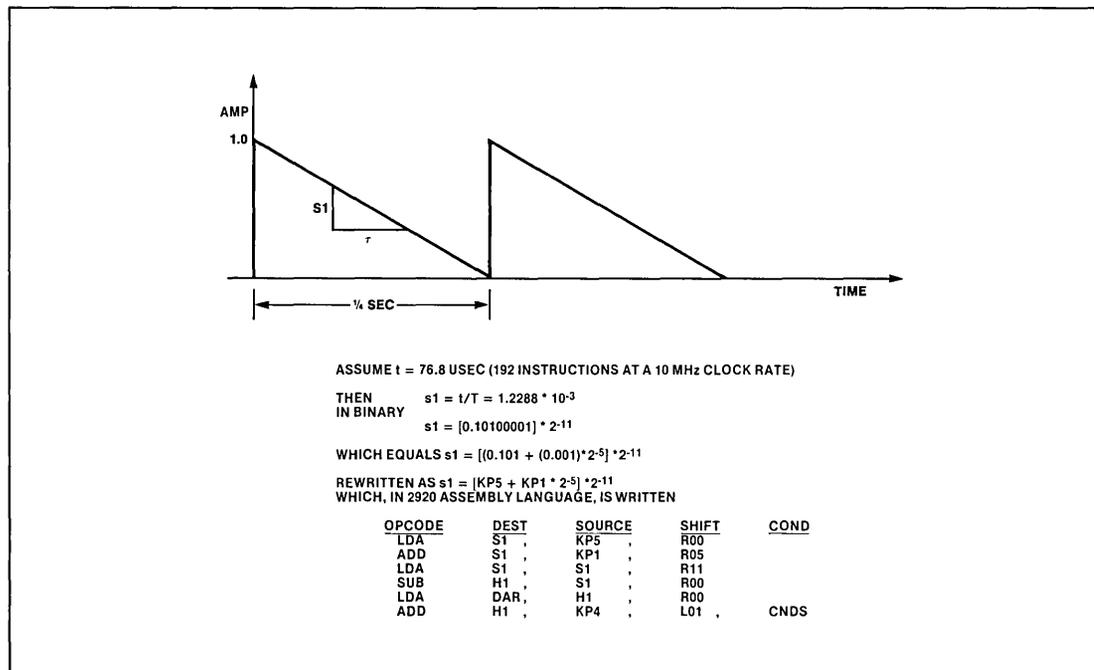
Figure 7-1. Sawtooth Sweep Rate Generator
