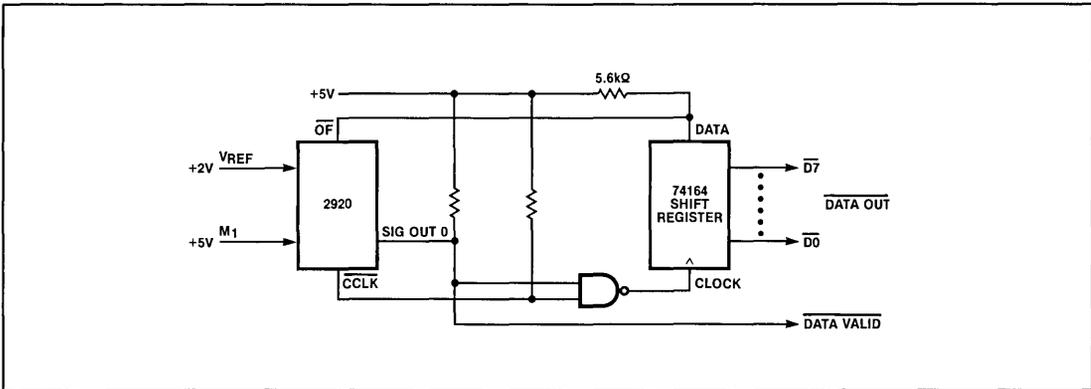
**Figure 6-5. Logic Diagram for Digital Output: Serial**
