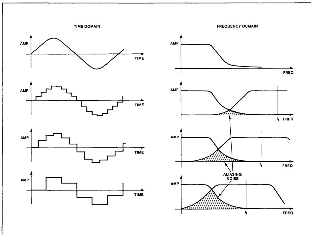
Figure 2-4. Effects of Sampling Rate on Aliasing Noise
