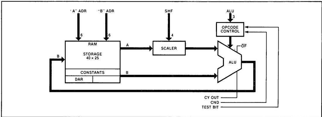
Figure 3-3. Arithmetic Unit and Memory
