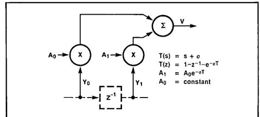
Figure 5-14. Realization Of A Single Real Zero
