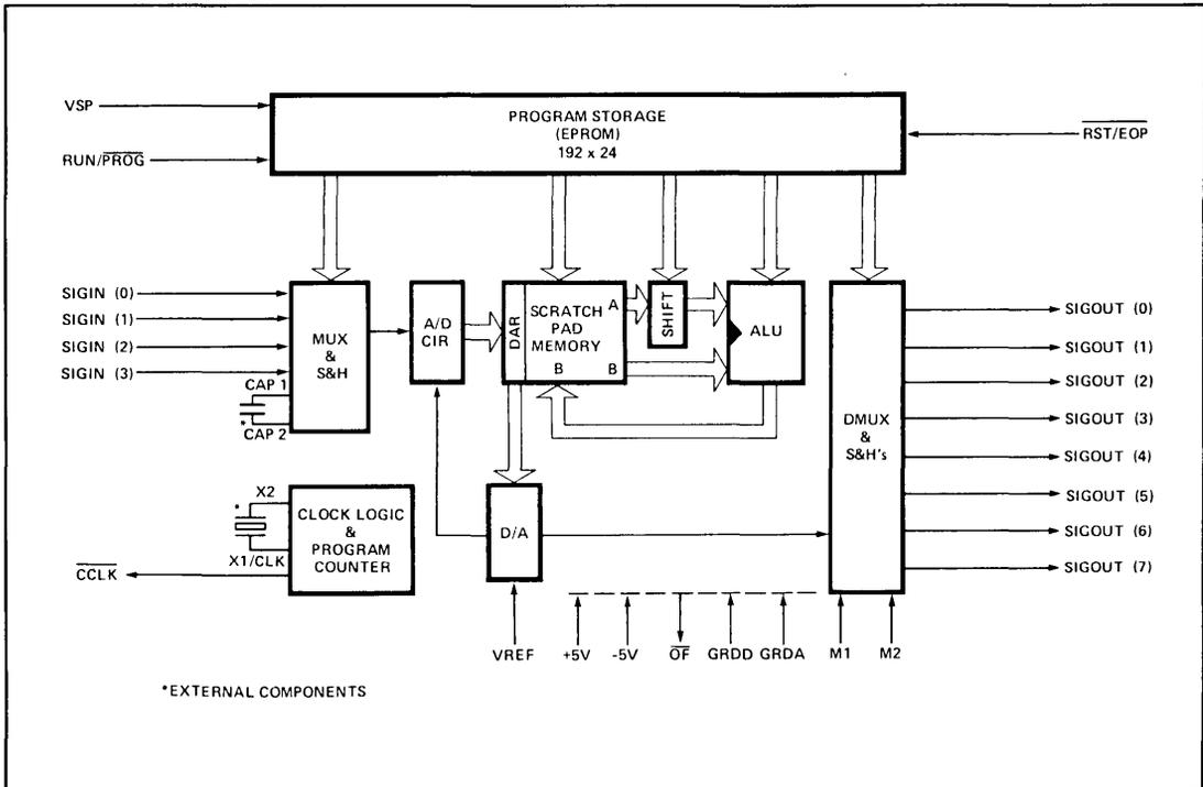
Figure 3-1. 2920 Block Diagram
