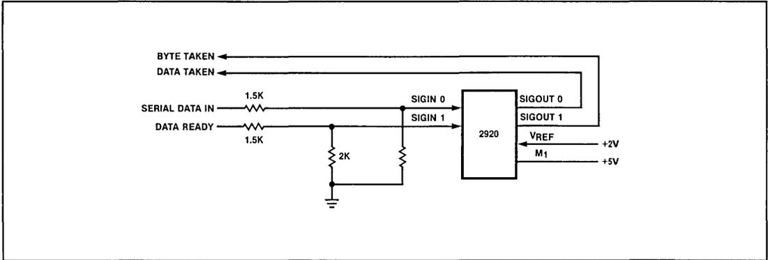
**Figure 6-9. Logic Diagram for Digital Input: Serial**
