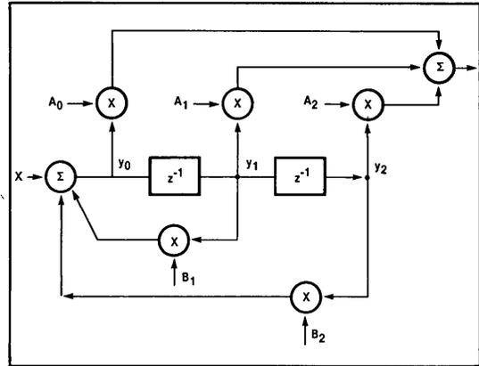
**Figure 5-7. Digital Filter Module (Second Order Section)**
