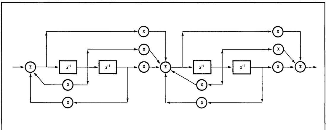
**Figure 5-19a. Cascade Structure for Complex Filter
