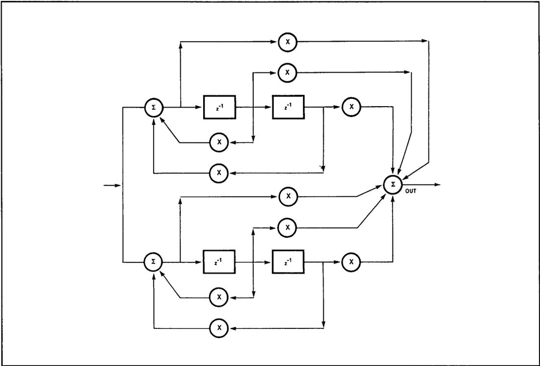
**Figure 5-19b. Parallel Structure for Complex Filters
