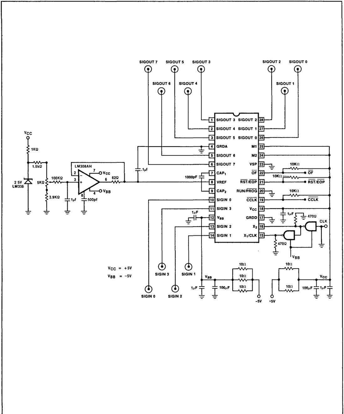
Figure 8-3. Schematic Diagram 2920 Application Breadboard
