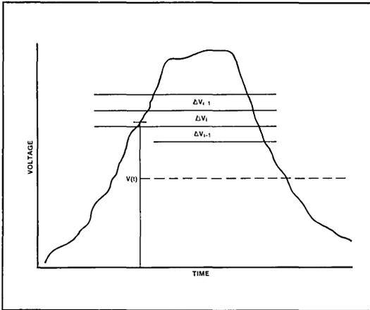
**Figure 2-10. Quantization Step**
