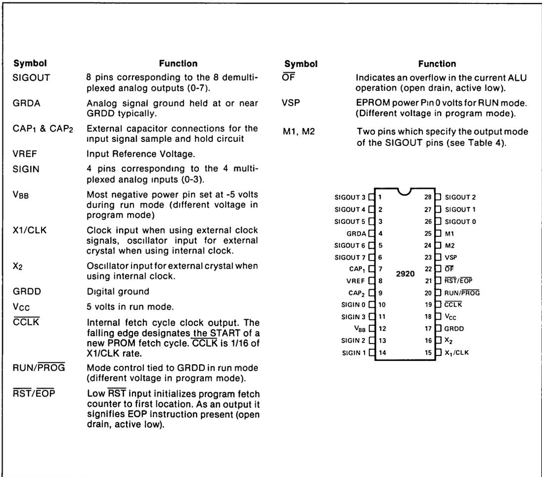
**Figure 8-2. 2920 Pinout**
