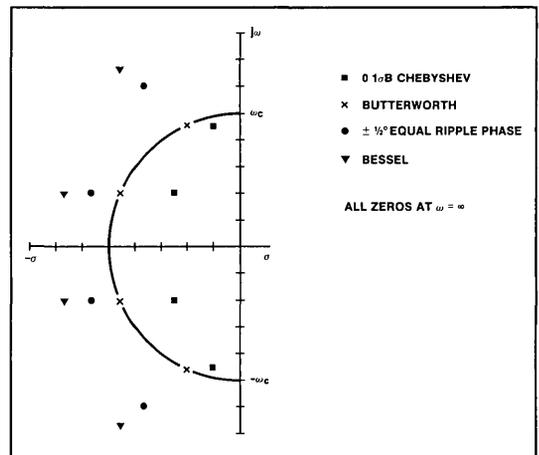
Figure 5-2. Pole-Zero Locations Of 4-Pole Lowpass Prototype Filters
