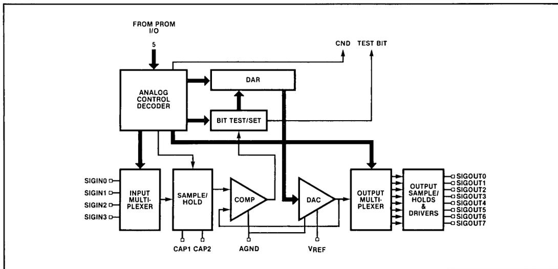
Figure 3-5. Analog Section Block Diagram
