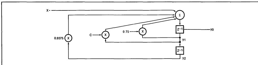
**Figure 6-3. Second Order Stage With Variable Center Frequency**
