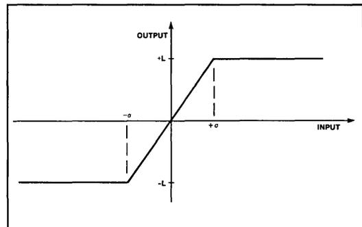
Figure 4-3. Limiter Transfer Characteristic
