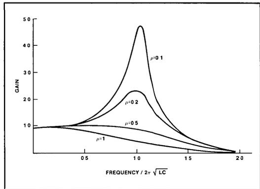
**Figure 5-13. Gain Of Complex Conjugate Pole Pair Section**
