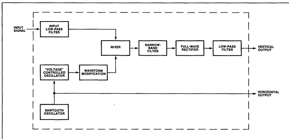
Figure 7-10. Block Diagram of a Spectrum Analyzer
