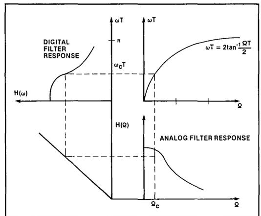
Figure 5-10. Transfer Function From  $\Omega$  to  $w$
