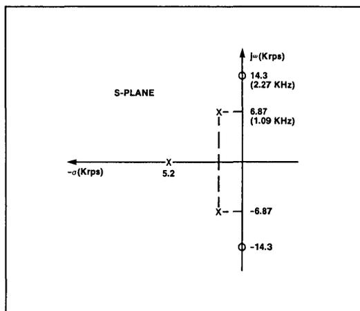
**Figure 7-7. Pole and Zero Plot in the S-Plane**
