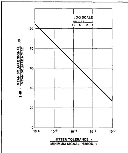
**Figure 2-8. Jitter SNR**
