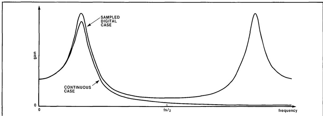
Figure 5-9. Comparison of Digital and Continuous Frequency Response
