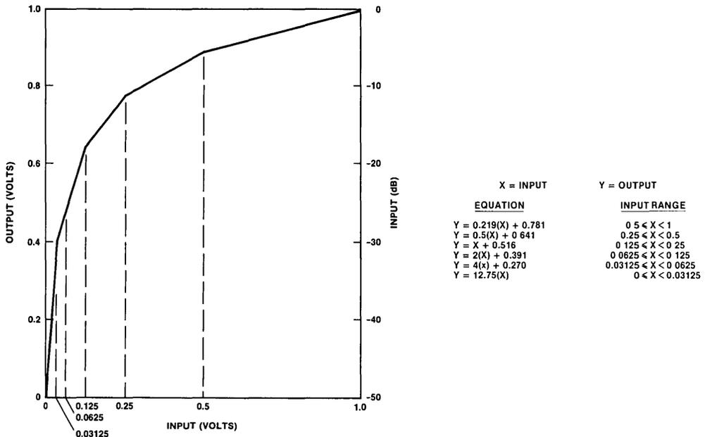
Figure 7-4. Log Amplifier Piecewise Linear Approximation Transfer Characteristics
