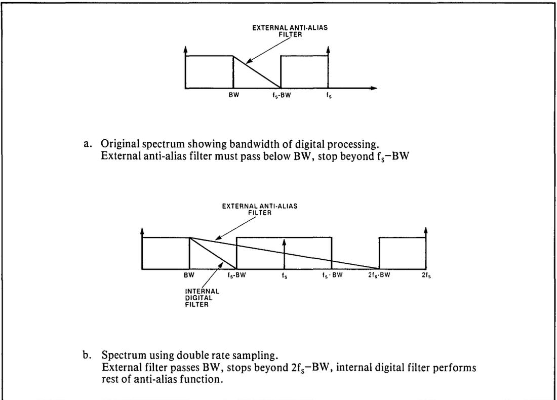
**Figure 5-18. Effects of Double Rate Input Sampling**
