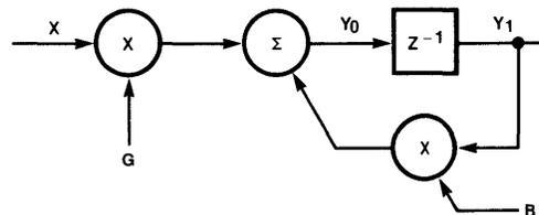
Figure 4-2. Sampled Realization of a Single Real Pole
