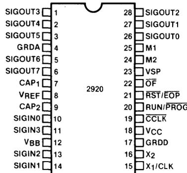
Figure 1-2. Run Mode Pin Configuration
