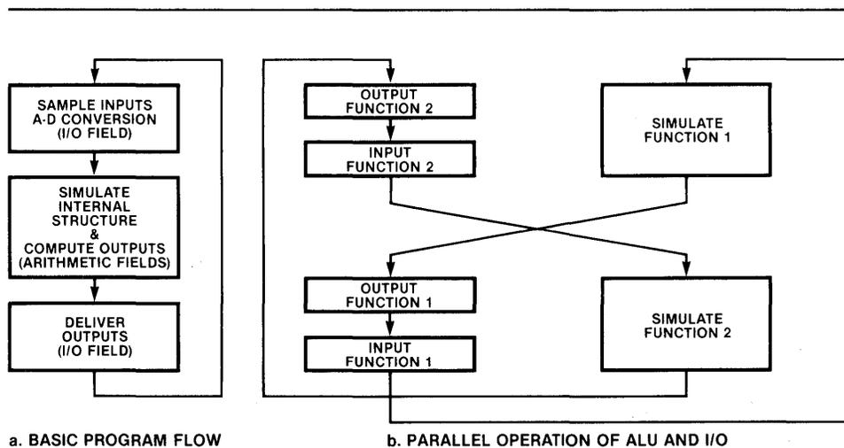
Figure 1-3. 2920 Program Flow Diagrams
