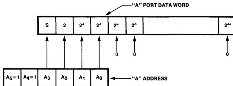
Figure 1-5. Address Mapping for Constants
