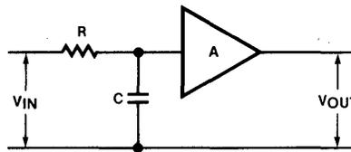
Figure 4-1. Continuous Realization of a Single Real Pole
