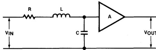
Figure 4-3. Continuous Realization of Complex Conjugate Pole Pair
