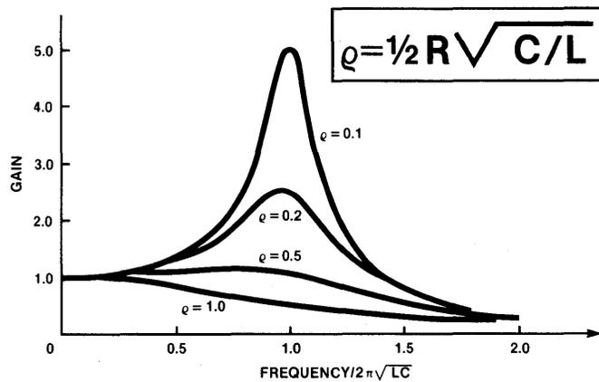
Figure 4-4. Gain of Complex Conjugate Pole Pair Section
