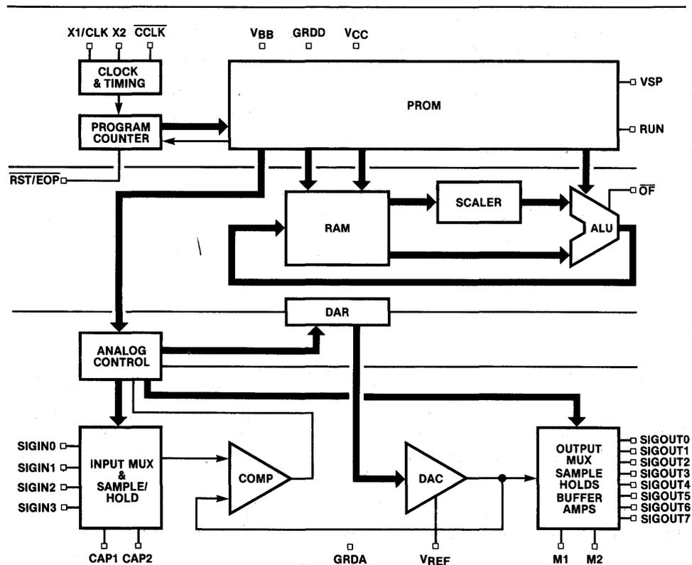
Figure 1-1. Block Diagram of 2920 Signal Processor
