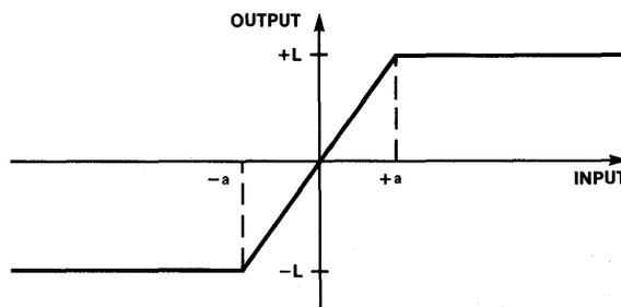
Figure 4-6. Limiter Transfer Characteristic
