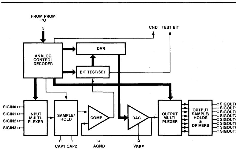
Figure 1-6. Analog Section Block Diagram
