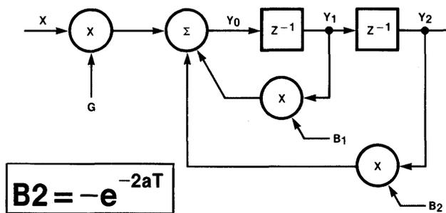
Figure 4-5. Sampled Realization of Complex Conjugate Pole Pair
