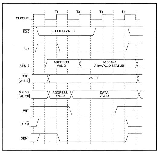
Figure 3.21. Typical Write Bus Cycle
