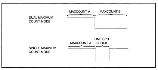
Figure 9.4. Timer/Counter Unit Output Modes
