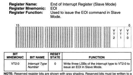
**NOTE:** Reserved register bits are shown with gray shading. Reserved bits must be written to a logic zero to insure compatibility with future Intel products.
