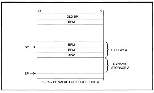
Figure A.4. Stack Frame for Procedure A at Level 2
