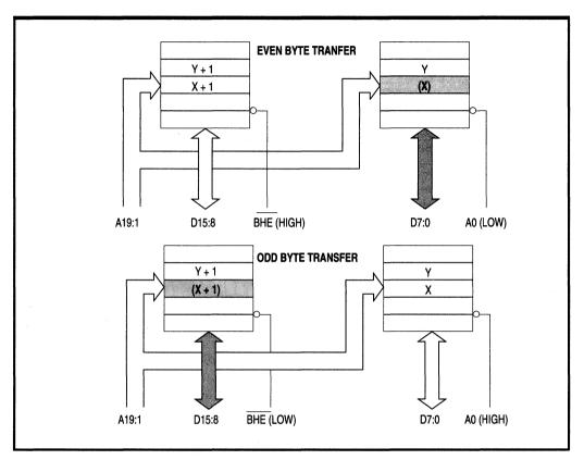
Figure 3.2. 16-Bit Data Bus Byte Transfers
