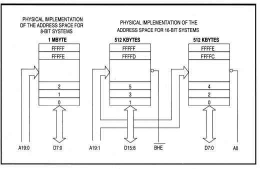
Figure 3.1. Physical Data Bus Models
