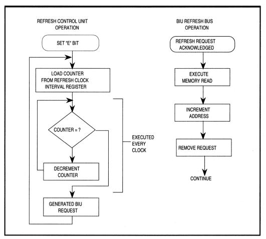
Figure 7.2. Refresh Control Unit Operation Flow Chart
