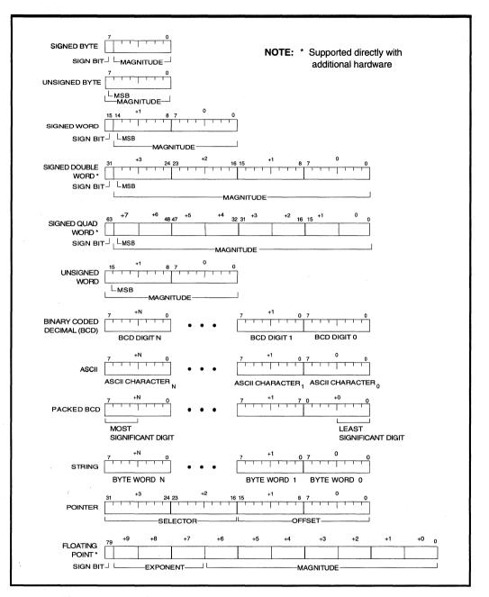
Figure 2.23. 80C186 Modular Core Family Supported Data Types
