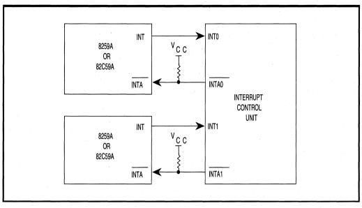
Figure 8.2. Using 8259As in Cascade Mode
