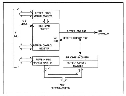
Figure 7.1. Refresh Control Unit Block Diagram
