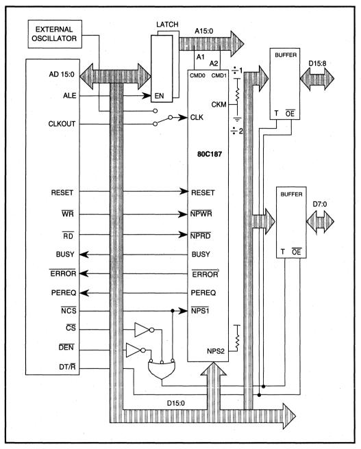
Figure 11.3. 80C187 Configuration with Partially Buffered Bus
