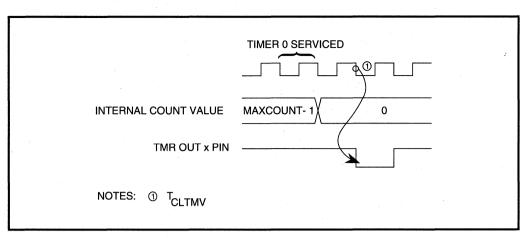
Figure 9.9. TxOUT Signal Timing
