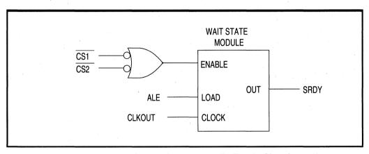
Figure 3.16. Generating a Normally Ready Signal
