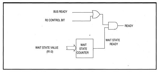
Figure 6.11. Wait State and Ready Control Functions
