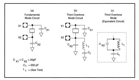
Figure 5.3. Crystal Connections to Microprocessor
