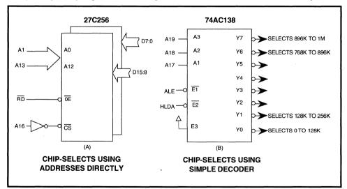
Figure 6.1. Common Chip-Select Generation Methods
