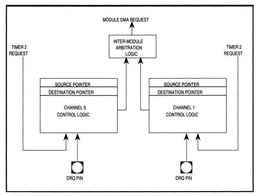
Figure 10.5. Two Channel DMA Unit
