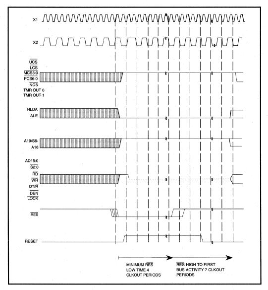
Figure 5.7. Warm Reset Waveform
