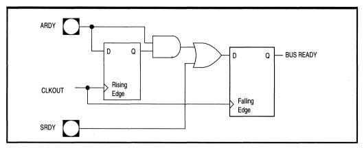
Figure 3.14. ARDY and SRDY Pin Block Diagram
