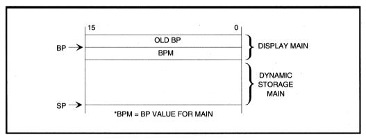
Figure A.3. Stack Frame for MAIN at Level 1
