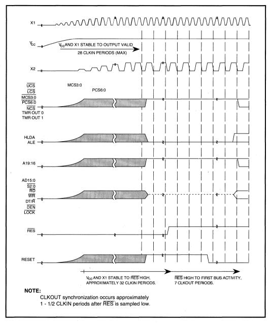
Figure 5.6. Cold Reset Waveform
