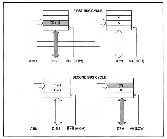
Figure 3.4. 16-Bit Data Bus Odd Word Transfers
