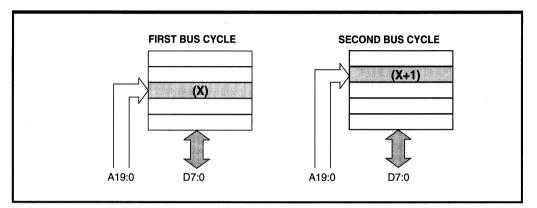
Figure 3.5. 8-Bit Data Bus Word Transfers
