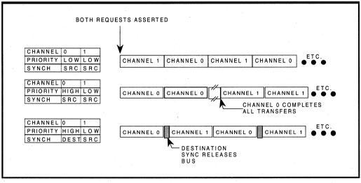
Figure 10.6. Examples of DMA Priority
