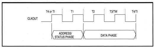
Figure 3.9. T-State and Bus Phases
