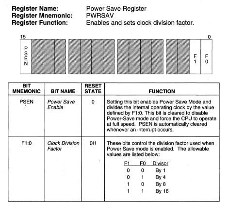
**NOTE:** Reserved register bits are shown with gray shading. Reserved bits must be written to a logic zero to insure compatibility with future Intel products.
