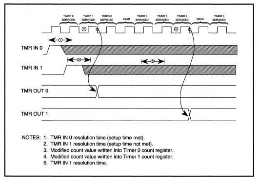
Figure 9.2. Counter Element Multiplexing and Timer Input Synchronization
