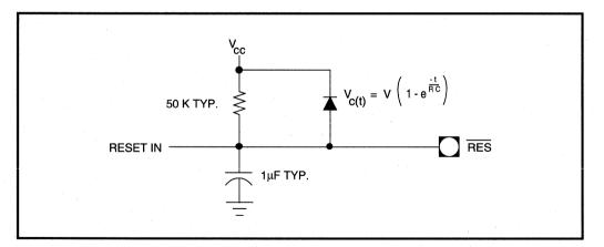
Figure 5.5. Simple RC Circuit for Powerup Reset
