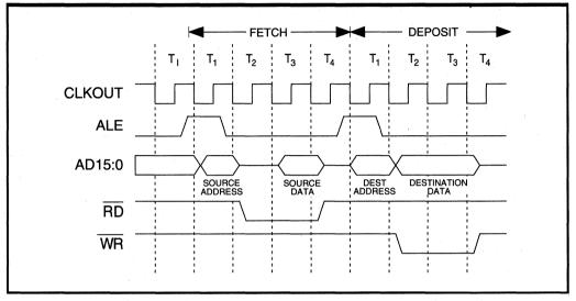
Figure 10.1. Typical DMA Transfer
