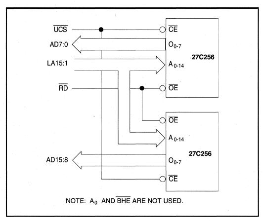
Figure 3.20. Read-Only Device Interface
