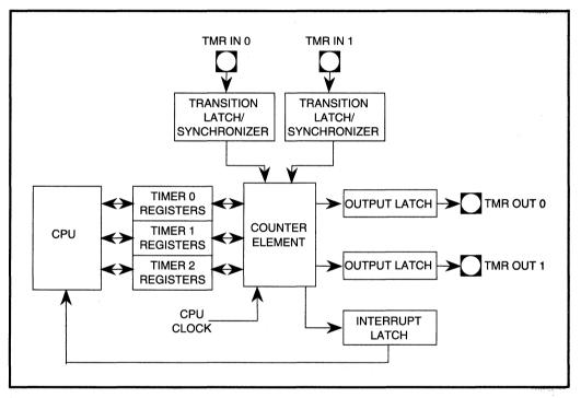
Figure 9.1. Timer/Counter Unit Block Diagram
