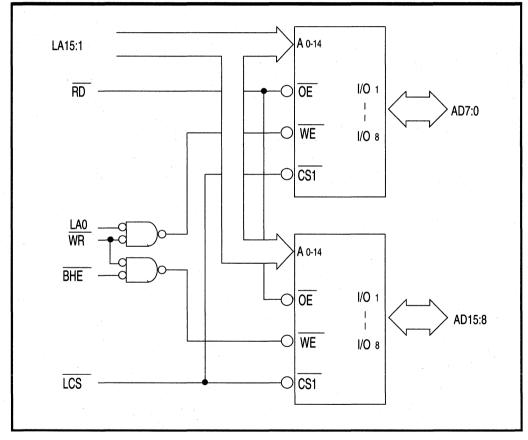
Figure 3.22. 16-Bit Bus Read/Write Device Interface
