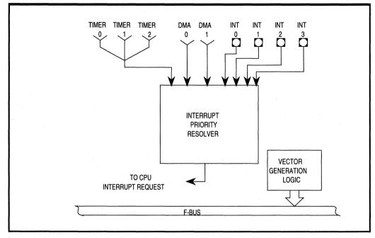
Figure 8.1. Interrupt Control Unit Block Diagram
