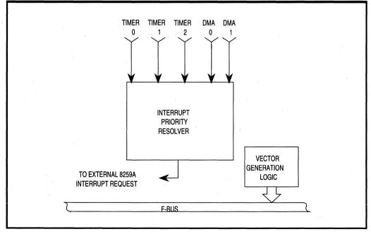
Figure 8.16. Interrupt Sources In Slave Mode
