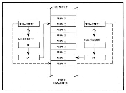
Figure 2.18. Accessing an Array with Indexed Addressing
