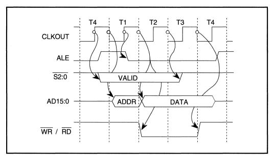
Figure 3.6. Typical Bus Cycle
