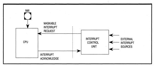
Figure 2.24. Interrupt Control Unit
