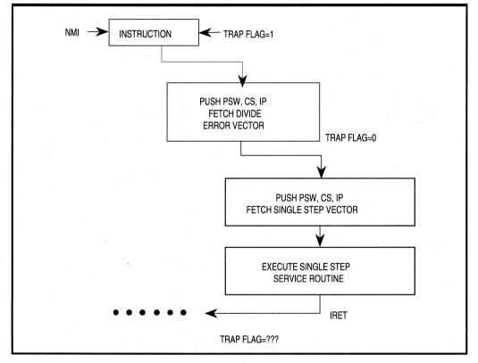
Figure 2.29. Simultaneous NMI and Single Step Interrupts
