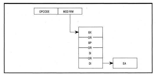
Figure 2.14. Register Indirect Addressing
