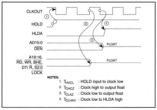
Figure 3.34. Timing Sequence Entering HOLD
