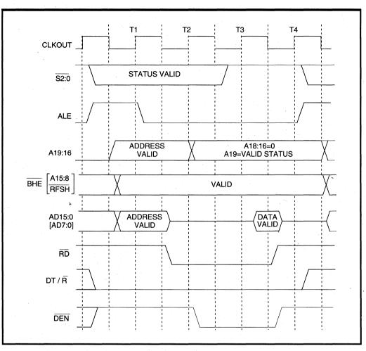
Figure 3.19. Typical Read Bus Cycle
