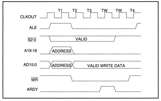
Figure 3.13. Typical Bus Cycle With Wait States
