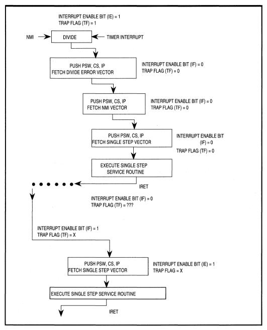
Figure 2.30. Simultaneous NMI, Single Step and Maskable Interrupt
