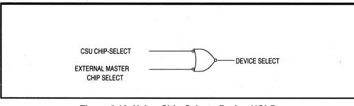
Figure 6.12. Using Chip-Selects During HOLD
