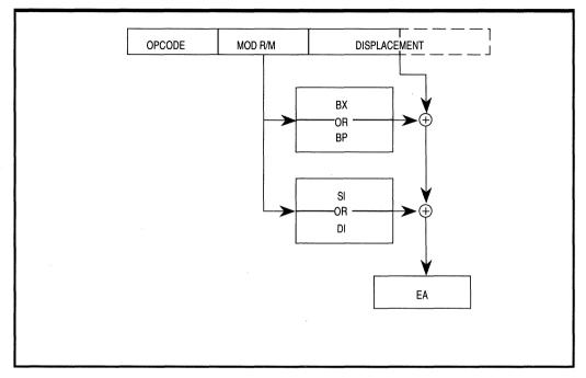
Figure 2.19. Based Index Addressing
