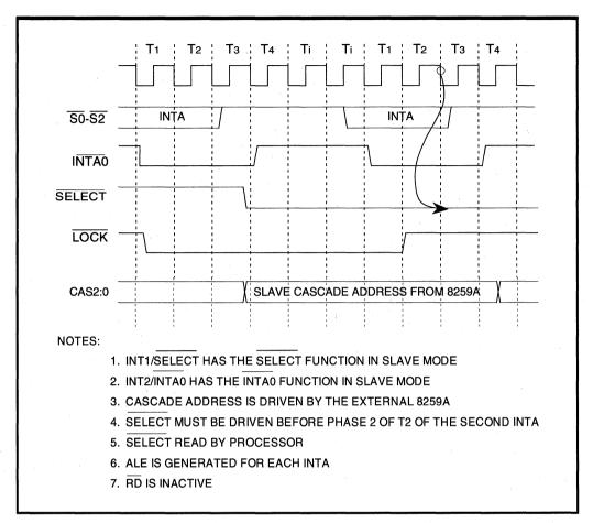
Figure 8.20. Interrupt Vectoring In Slave Mode
