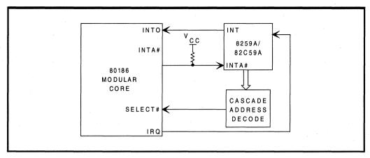
Figure 8.15. Interrupt Control Unit In Slave Mode
