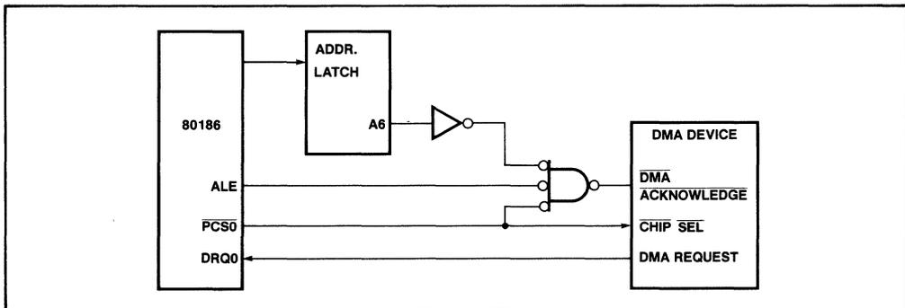
Figure 36. DMA Acknowledge Synthesis from the 80186
