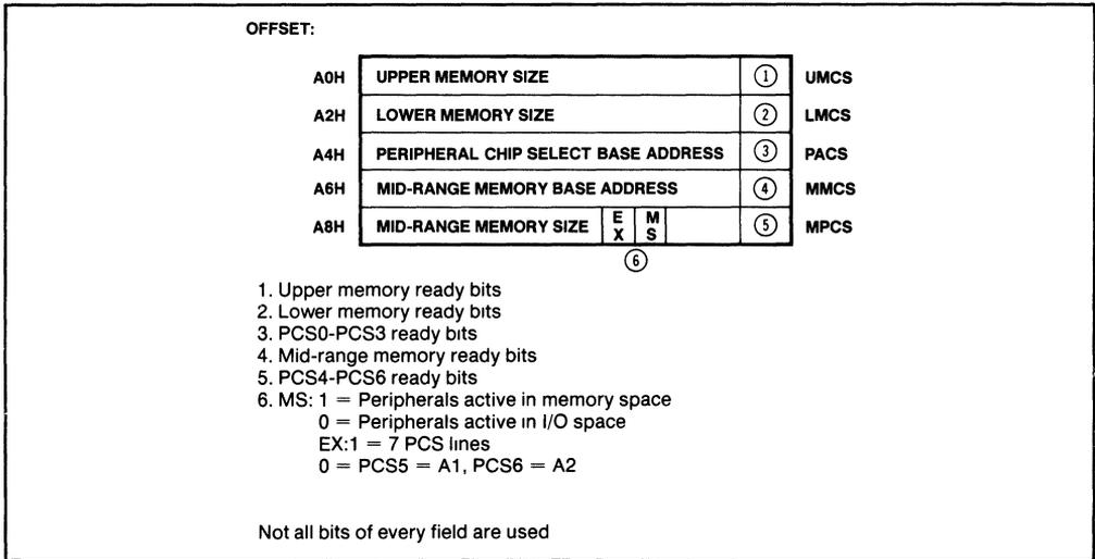
Figure 72. 80186 Chip Select Control Registers
