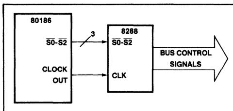
Figure 14. 80186/8288 Bus Controller Interconnection
