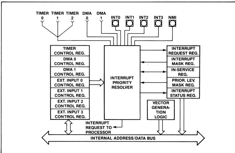
Figure 48. 80186 Interrupt Controller Block Diagram
