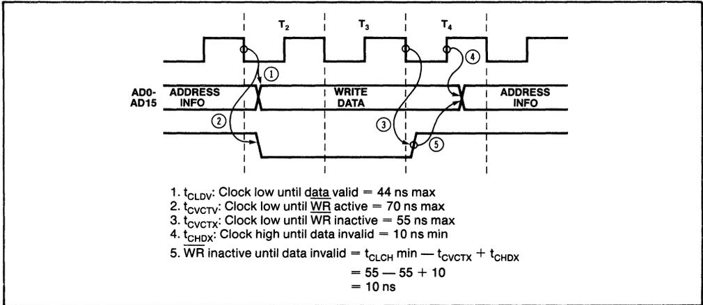
Figure 12. Write Cycle Timing of the 80186
