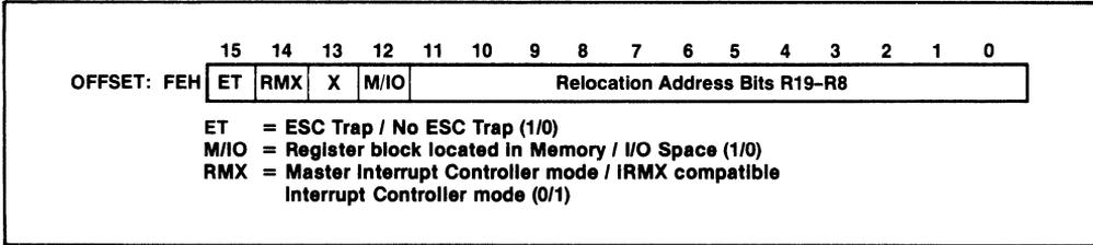
**Figure A-2. 80186 Relocation Register Layout**
