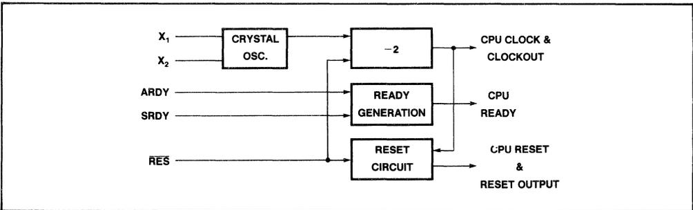
Figure 66. 80186 Clock Generator Block Diagram
