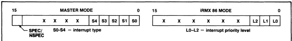
**Figure 54. 80186 End of Interrupt Register Format**
