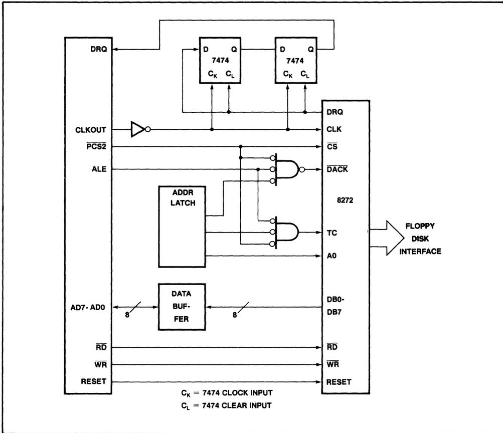
Figure 39. Example 8272/80186 DMA Interface
