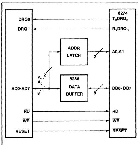
Figure 40. Example 8274/80186 DMA Interface
