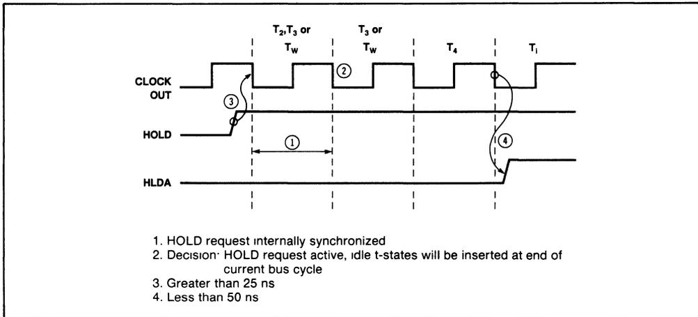
Figure 27A. HOLD/HLDA Timing in the 80186
