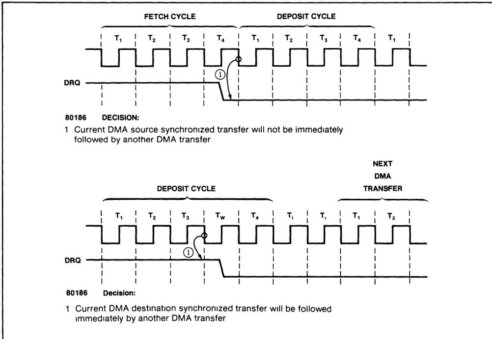
**Figure 37. Source & Destination Synchronized DMA Request Timing**
