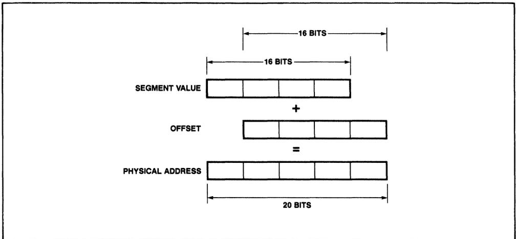
**Figure 2. Physical Address Generation in the 80186**
