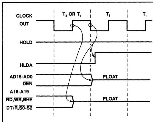
Figure 25. Signal Float/HLDA Timing of the 80186
