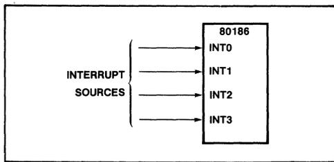
Figure 61. 80186 Non-Cascaded Interrupt Connection
