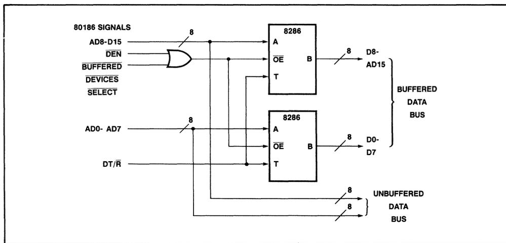
Figure 9. Example 80186 Buffered/Unbuffered Data Bus
