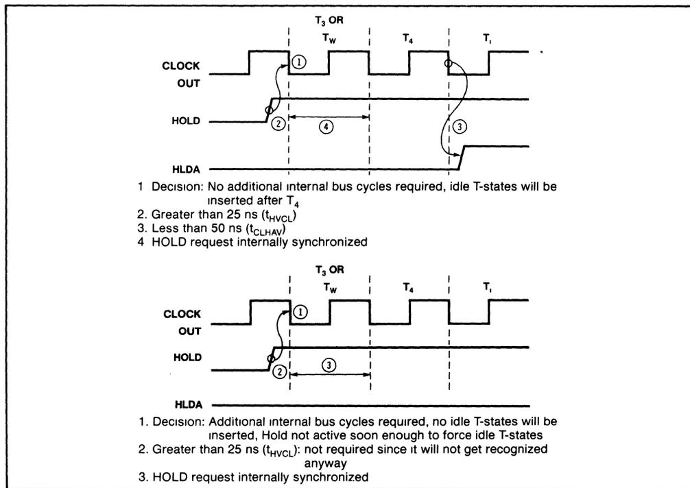
Figure 27. HOLD/HLDA Timing in the 80186
