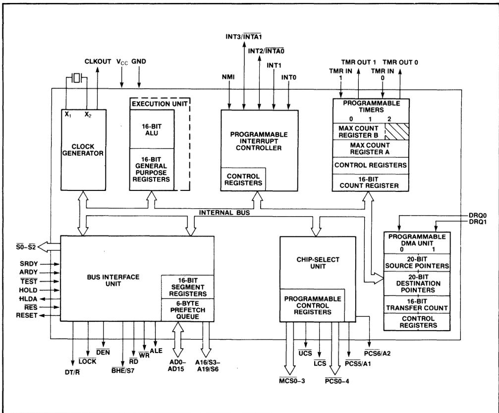
Figure 1. 80186 Block Diagram
