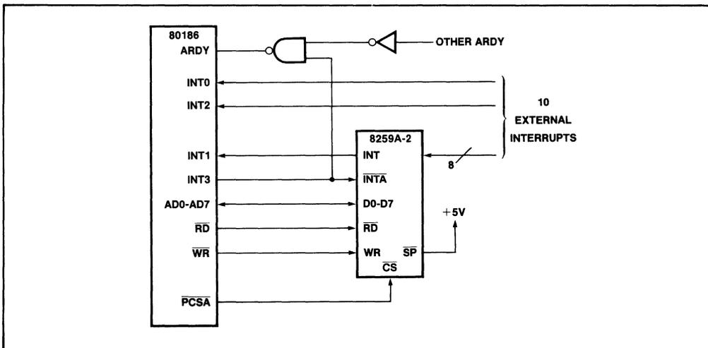
**Figure 64. 80186/8259A Interrupt Cascading**
