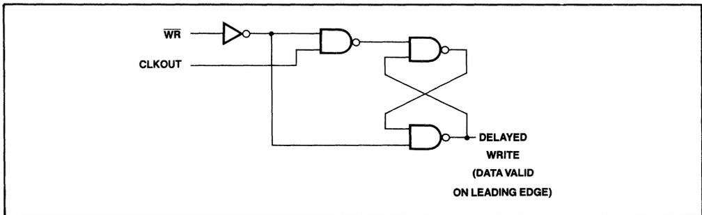
Figure 13. Synthesizing Delayed Write from the 80186
