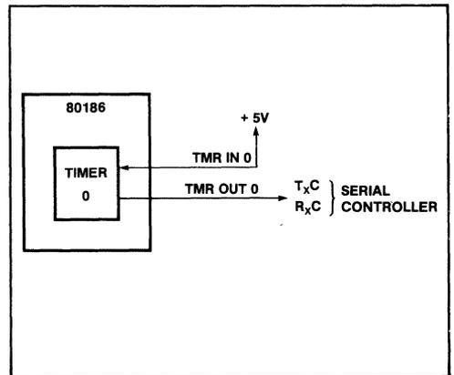
Figure 46. 80186 Baud Rate Generator
