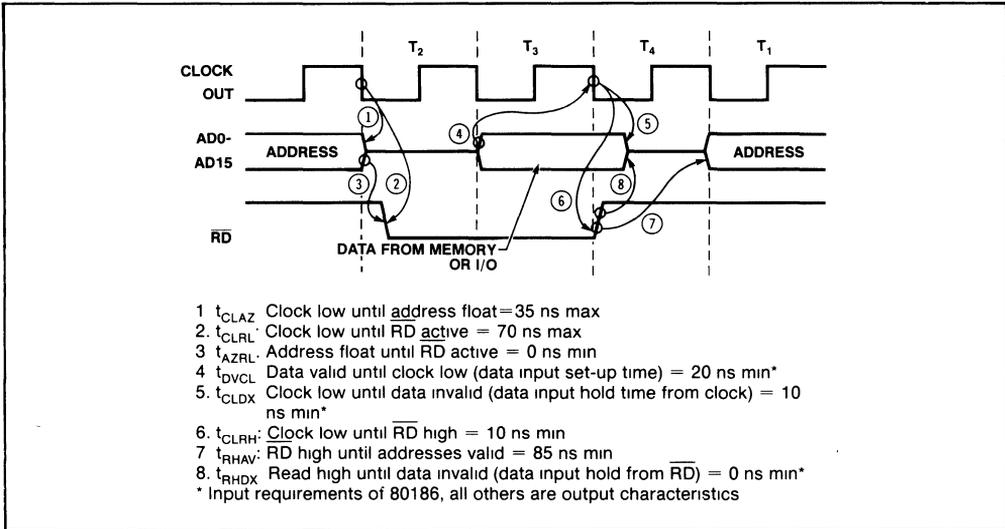
Figure 10. Read Cycle Timing of the 80186
