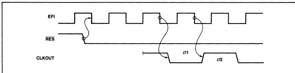
Figure 68. 80186 Clock Generator Reset
