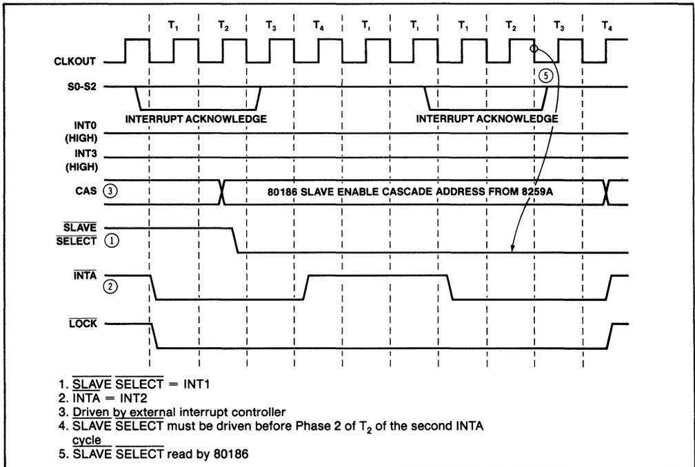
**Figure 59. 80186 iRMX-86 Mode Interrupt Acknowledge Timing**
