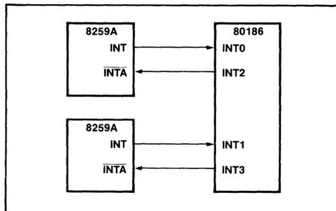
Figure 62. 80186 Cascade and Special Fully Nested Mode Interface
