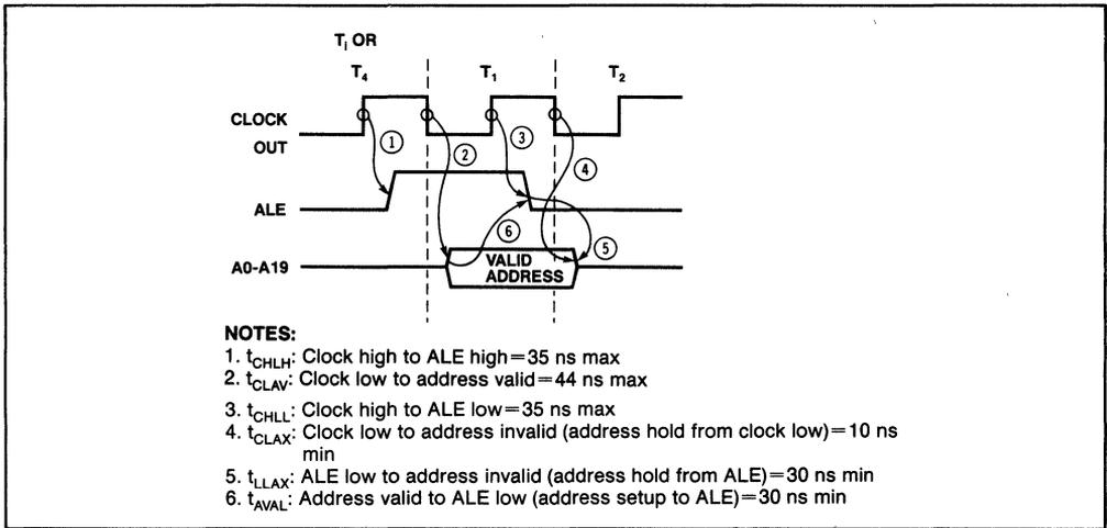
**Figure 6. Address Generation Timing of the 80186**
