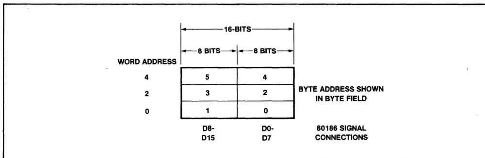
Figure 8. Physical Memory Byte/Word Addressing in the 80186
