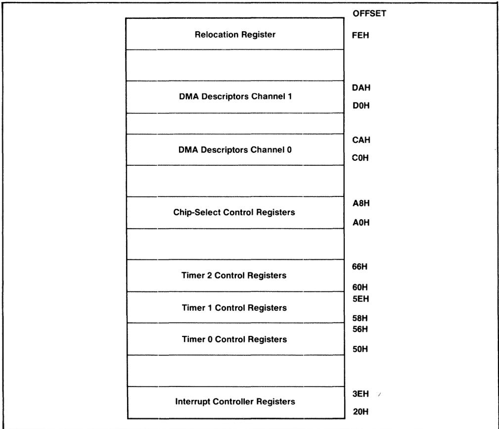
**Figure A-1. 80186 Integrated Peripheral Control Block**
