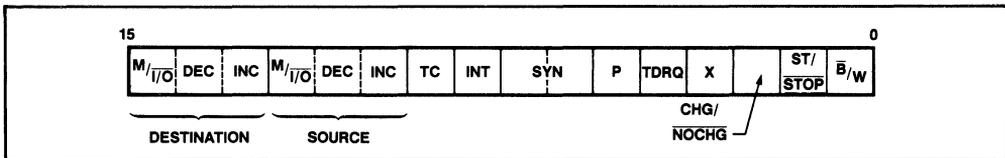
Figure 33. DMA Control Register
