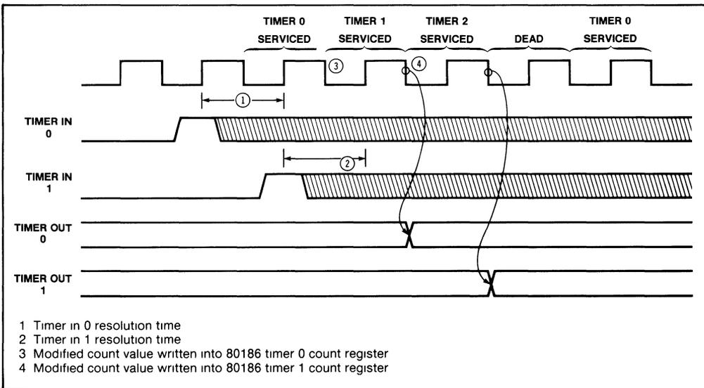
Figure 42. 80186 Counter Element Multiplexing and Timer Input Synchronization
