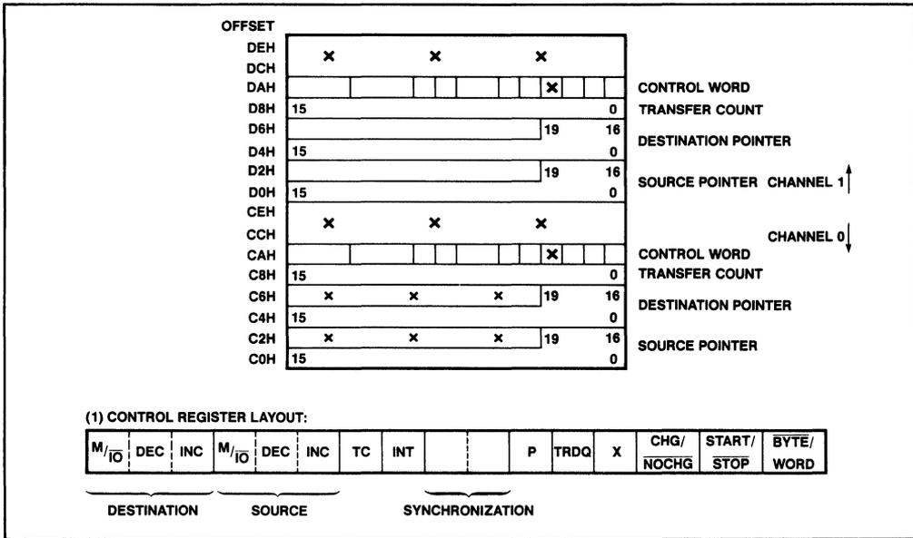
Figure 32. 80186 DMA Register Layout
