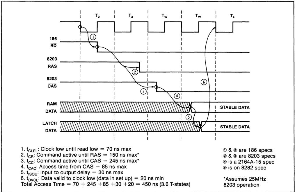
Figure 23. 8203/2164A-15 Access Time Calculation
