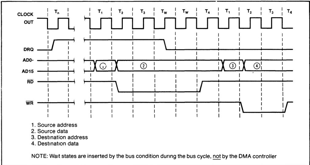
Figure 34. Example DMA Transfer Cycle on the 80186
