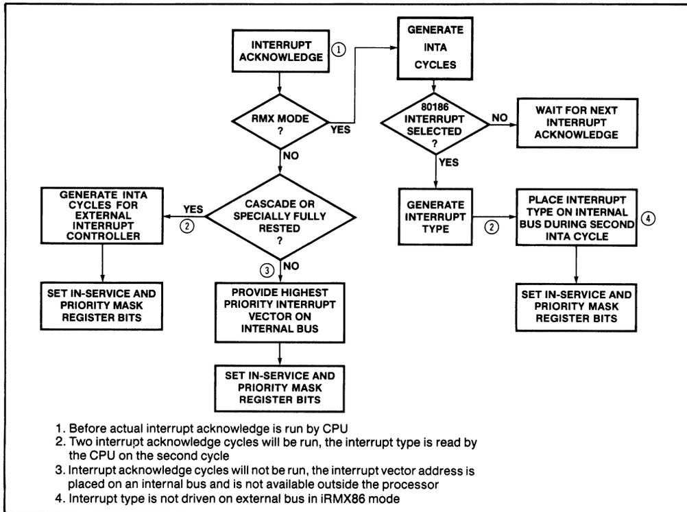
Figure 58. 80186 Interrupt Acknowledge Sequencing
