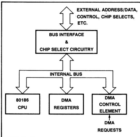
Figure 31. 80186 CPU/DMA Channel
