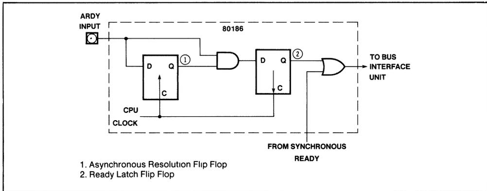
Figure 17. Asynchronous Ready Circuitry of the 80186
