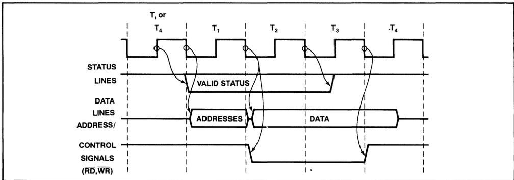
Figure 4. Example Bus Cycle of the 80186
