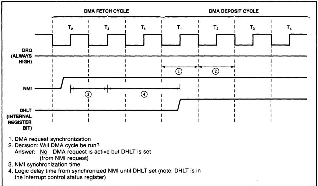
Figure 38. NMI and DMA Interaction
