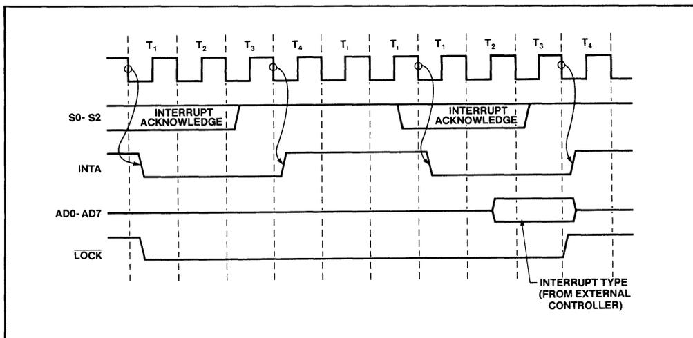
Figure 60. 80186 Cascaded Interrupt Acknowledge Timing
