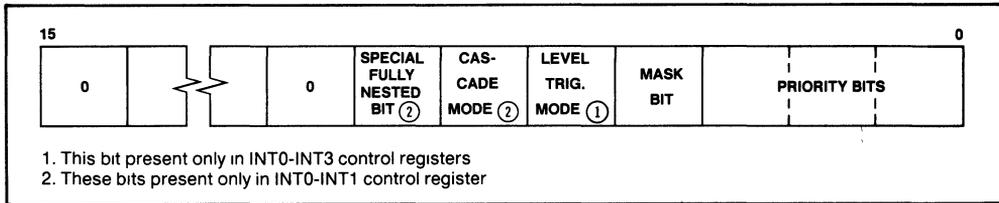
Figure 50. Interrupt Controller Control Register
