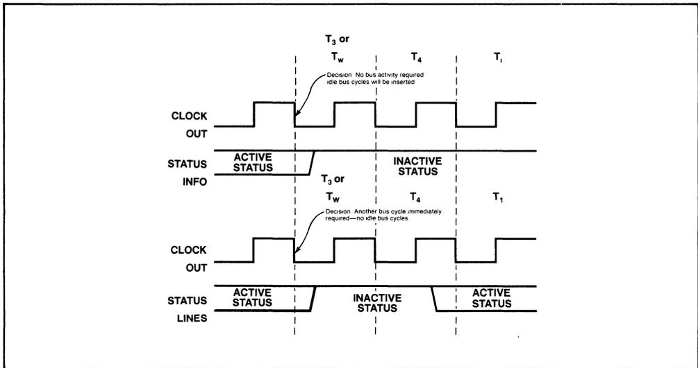
Figure 5. Active-Inactive Status Transitions in the 80186
