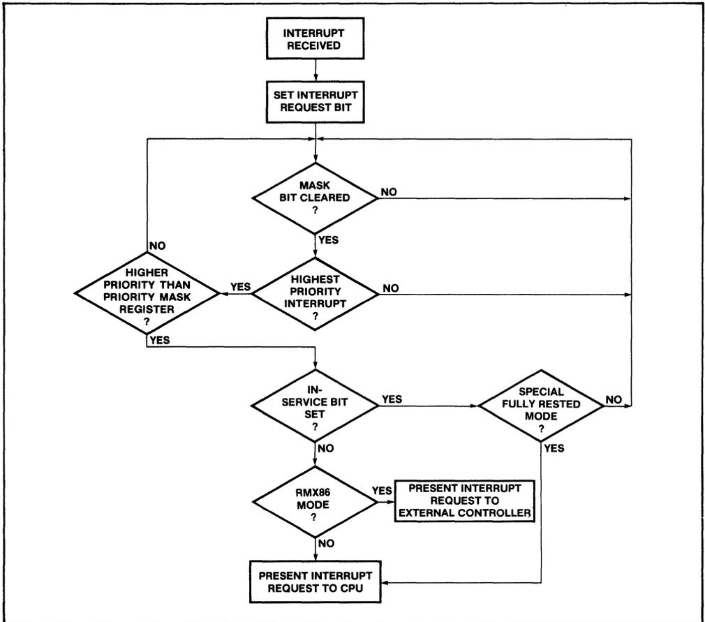
Figure 57. 80186 Interrupt Request Sequencing
