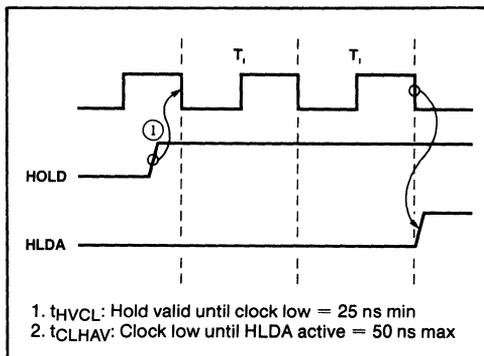
Figure 26. 80186 Idle Bus Hold/HLDA Timing
