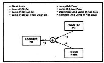
Figure 2.31. Unconditional Short Branch and Conditional Branch Operations
