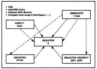
Figure 2.24. Internal Data Memory Arithmetic Operations
