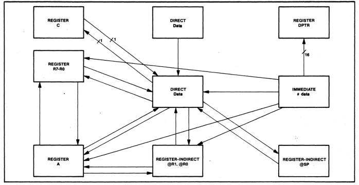
Figure 2.19. Internal Data Memory Move Operations
