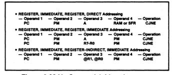
Figure 2.33.H. Operand Addressing Four-Operand Operations
