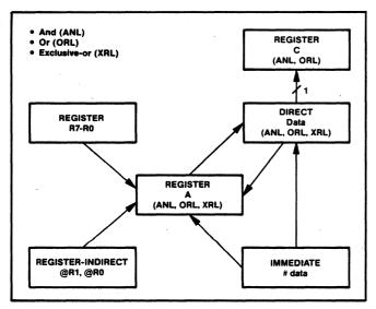
Figure 2.21. Internal Data Memory Logic Operations
