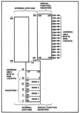
Figure 2.12. Internal Data Memory Address Space
