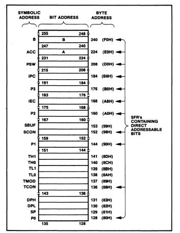
Figure 2.14. Mapping Of Special Function Registers
