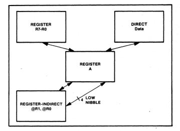
Figure 2.20. Internal Data Memory Exchange Operations
