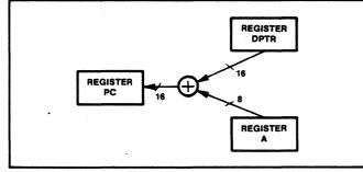
Figure 2.32. Unconditional Branch (Indirect) Operation
