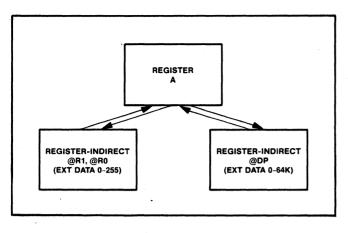
Figure 2.18. External Data Memory Move Operations
