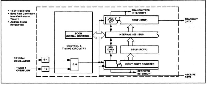
Figure 2.6. Serial Port—UART Modes 1, 2, and 3
