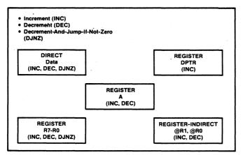
Figure 2.26. Internal Data Memory Arithmetic Operations
