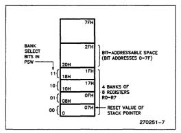
Figure 7. The Lower 128 Bytes of Internal RAM
