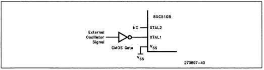
Figure 40. Driving the CHMOS Devices with an External Clock Sources
