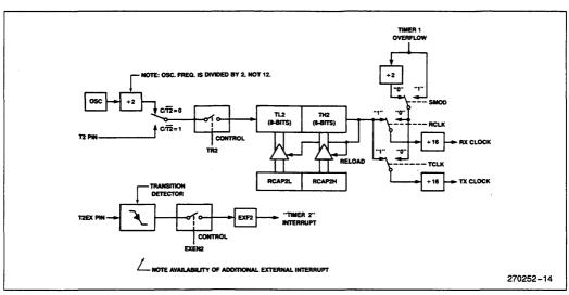
Figure 16. Timer 2 in Baud Rate Generator Mode
