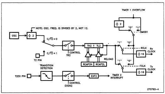
Figure 5. Timer 2 in Baud Rate Generator Mode
