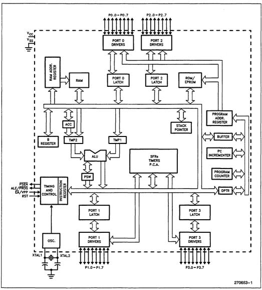
Figure 1. 8XC51FX Functional Block Diagram
