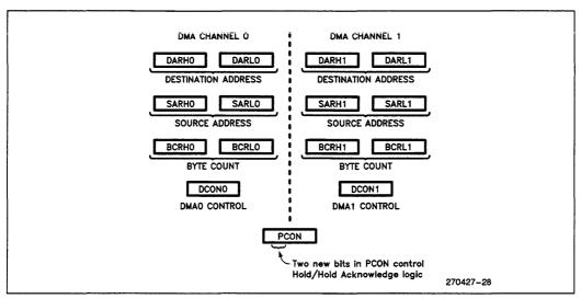
Figure 4.1. DMA Registers
