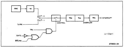
Figure 9. Timer/Counter 0 or 1 in Mode 1: 16-Bit Counter
