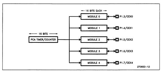
Figure 15a. Programmable Counter Array
