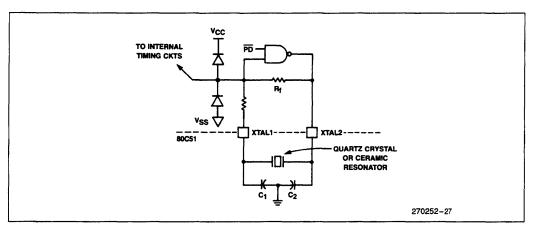
Figure 34. Using the CHMOS On-Chip Oscillator
