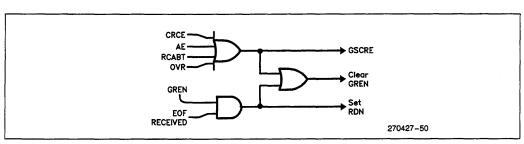
Figure 5.3. Receive Error Flag (Logic for Clearing GREN, setting RDN)
