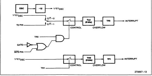
Figure 11. Timer/Counter 0 Mode 3: Two 8-Bit Counters 6-16
