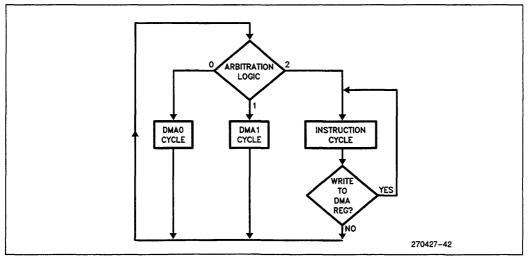
Figure 4.11. Internal Bus Usage
