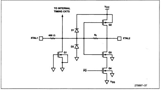
Figure 37. On-Chip Oscillator Circuitry
