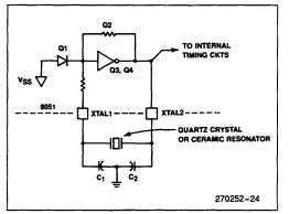
Figure 30. Using the HMOS On-Chip Oscillator
