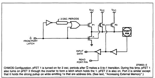
Figure 4. Ports 1 and 3 Internal Pullup Configurations
