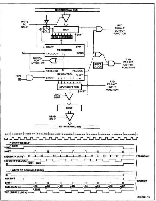
Figure 17. Serial Port Mode 0
