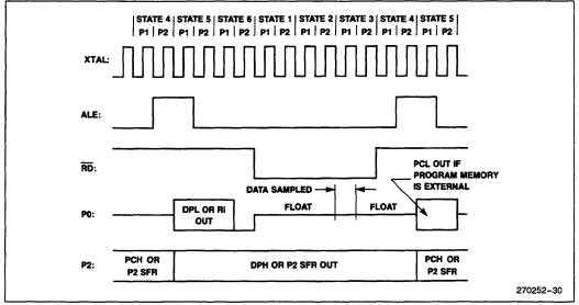
Figure 37. External Data Memory Read Cycle
