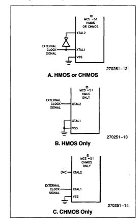
Figure 14. Using an External Clock
