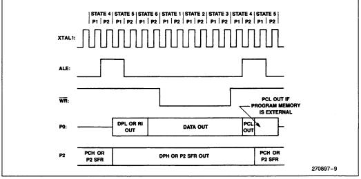
Figure 7. External Data Memory Write Cycle
