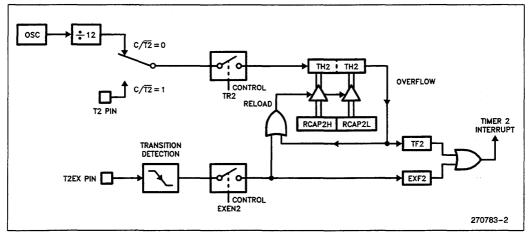
Figure 2. Timer 2 Auto Reload Mode (DCEN = 0)
