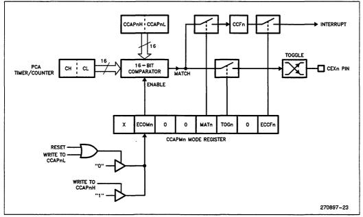
Figure 21. PCA 16-Bit Comparator Mode: High Speed Output
