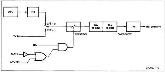
Figure 8. Timer/Counter 0 or 1 in Mode 0: 13-Bit Counter
