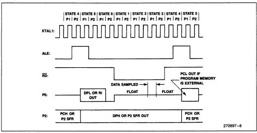
Figure 6. External Data Memory Read Cycle
