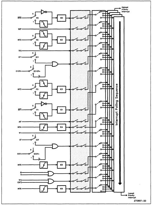
Figure 33. Interrupt Control System
