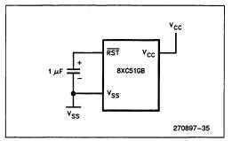
Figure 35. Power-On Reset Circuitry
