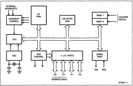
Figure 1. Block Diagram of the 8051 Core
