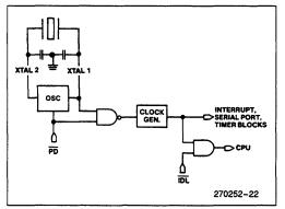
Figure 27. Idle and Power Down Hardware
