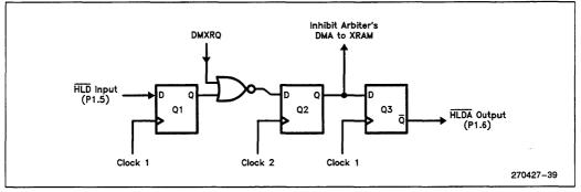
Figure 4.8. Internal Logic of the Arbiter
