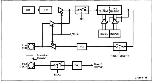
Figure 15. Timer 2 in Clock-Out Mode
