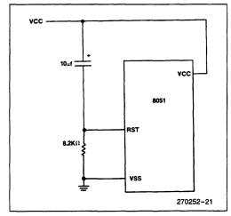
Figure 26. Power on Reset Circuit
