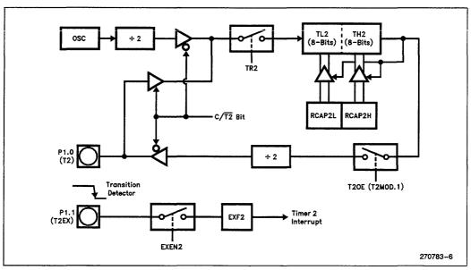
Figure 4. Timer 2 in Clock-Out Mode
