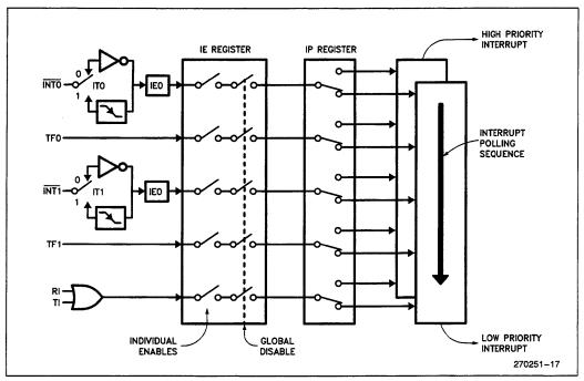
Figure 19. 8051 Interrupt Control System
