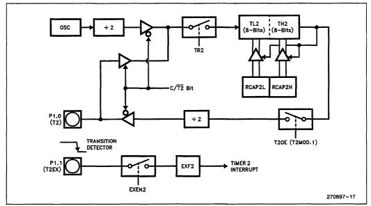
Figure 15. Timer 2 in Clock-Out Mode
