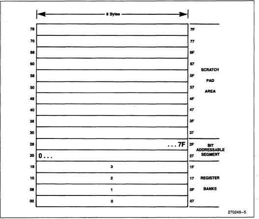
Figure 4. 128 Bytes of RAM Direct and Indirect Addressable
