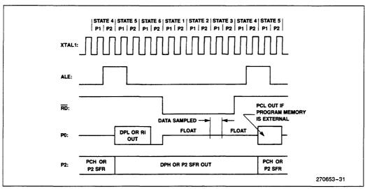
Figure 6. External Data Memory Read Cycle
