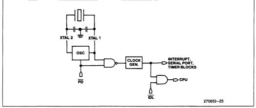
Figure 28. Idle and Power Down Hardware
