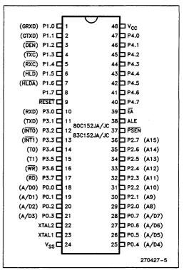
Figure 2.5A. DIP Pin Out
