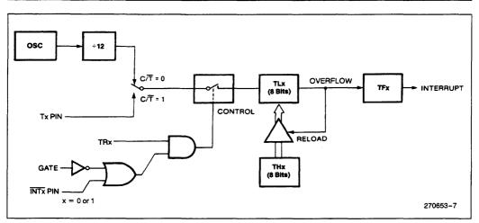
Figure 10. Timer/Counter 1 Mode 2: 8-Bit Auto-Reload
