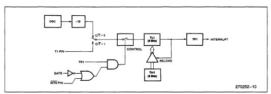
Figure 9. Timer/Counter 1 Mode 2: 8-Bit Auto-Reload
