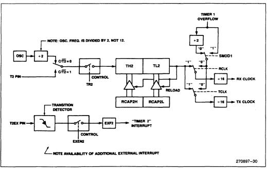
Figure 29. Timer 2 in Baud Rate Generator Mode
