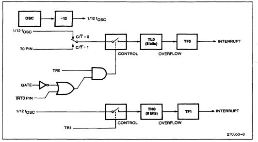
Figure 11. Timer/Counter 0 Mode 3: Two 8-Bit Counters
