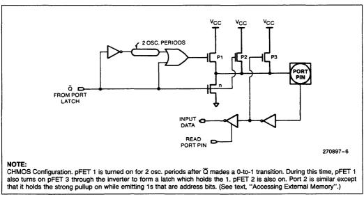
Figure 4. Ports 1, 3, 4, and 5 Internal Pullup Configuration
