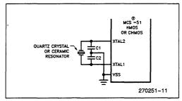
Figure 13. Using the On-Chip Oscillator
