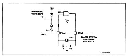
Figure 30. Using the CHMOS On-Chip Oscillator
