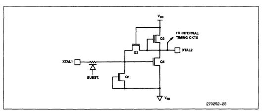
Figure 29. On-Chip Oscillator Circuitry in the HMOS Versions of the MCS®-51 Family
