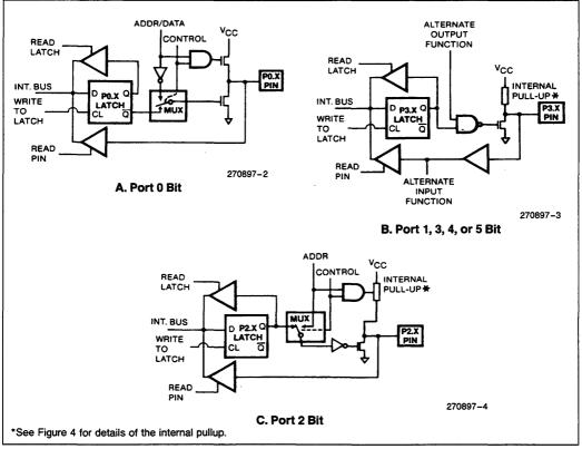
Figure 2. 8XC51GB Port Bit Latches and I/O Buffers
