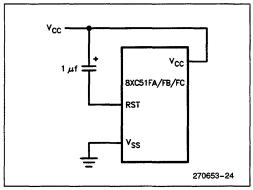
Figure 27. Power on Reset Circuitry
