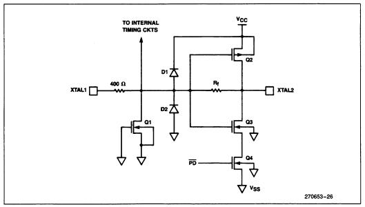
Figure 29. On-Chip Oscillator Circuitry
