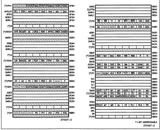
Figure 2.2. Special Function Registers
