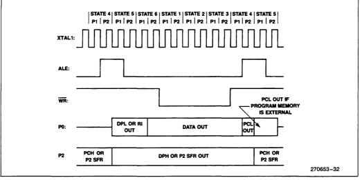
Figure 7. External Data Memory Write Cycle
