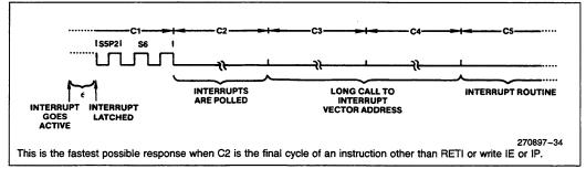
Figure 34. Interrupt Response Timing Diagram
