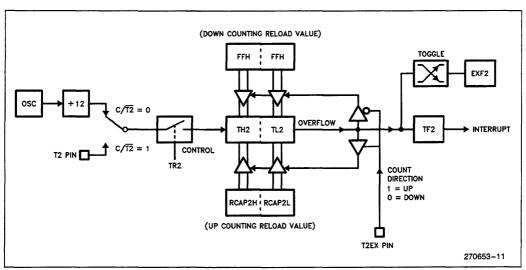
Figure 14. Timer 2 Auto Reload Mode (DCEN = 1)
