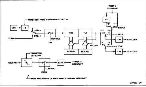
Figure 23. Timer 2 in Baud Rate Generator Mode
