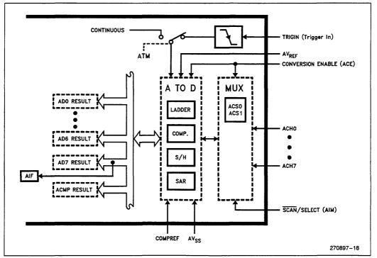
Figure 16. A/D Block Diagram
