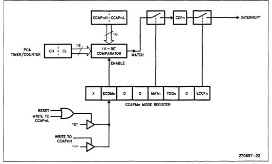
Figure 20. PCA 16-Bit Comparator Mode: Software Timer
