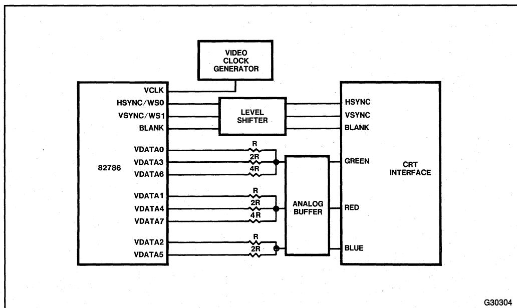
Figure 6-4. Resistor Ladder
