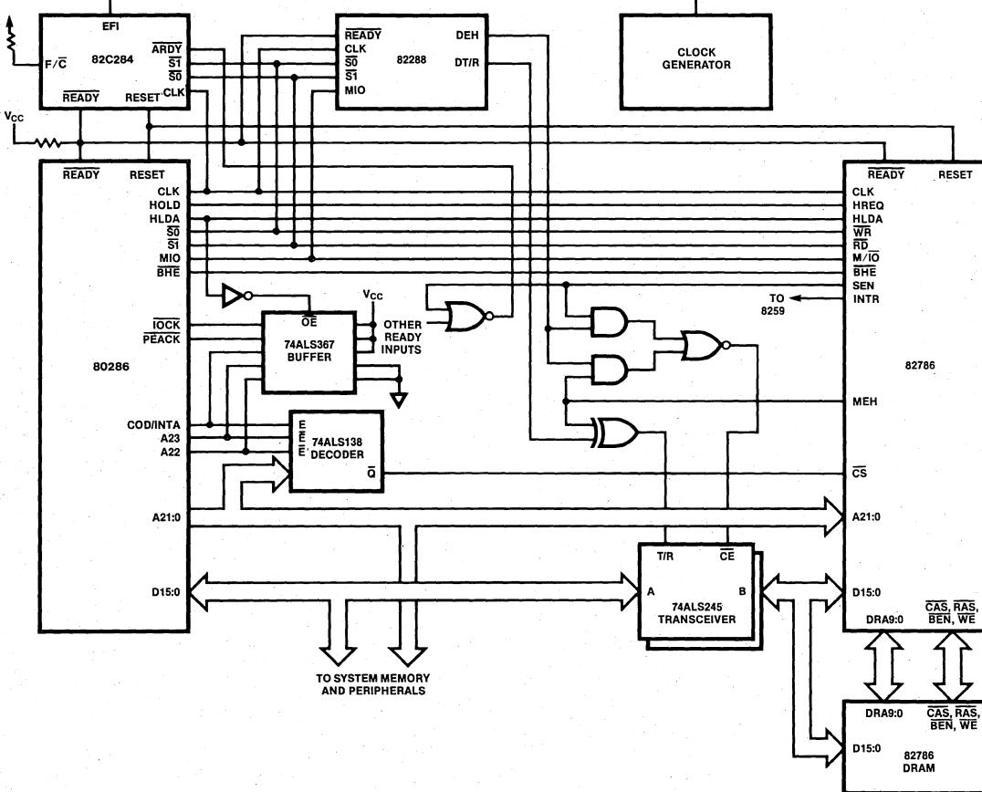
Figure 4-11. 82786 Synchronously Connected to an 80286
