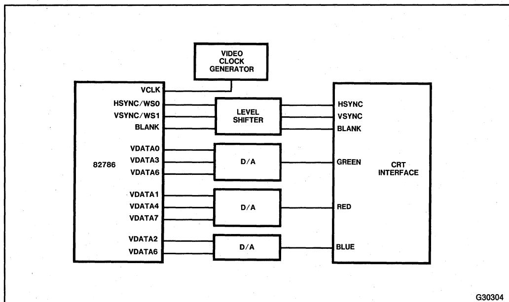
Figure 6-3. Analog CRT Interface Allows 256 Colors
