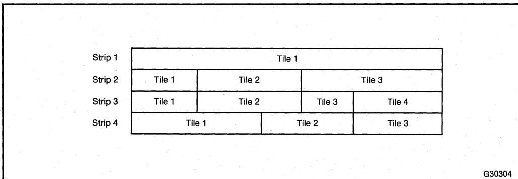
Figure 3-4. Screen Composition with Strips and Tiles
