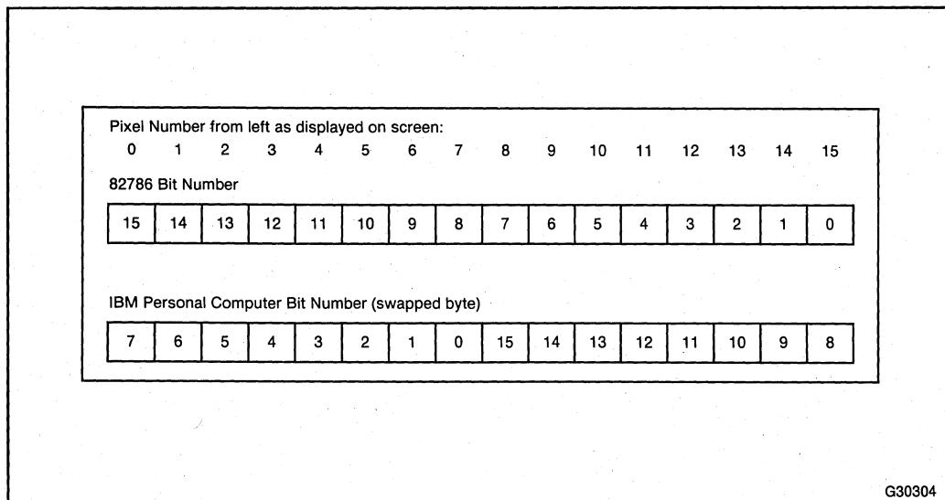
Figure 3-1. 82786 and IBM PC Swapped Byte Bitmap Formats
