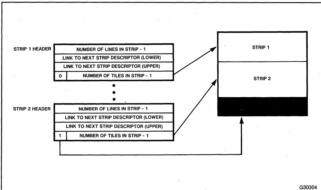
Figure 3-7. C Bit Can Indicate Final Strip Color
