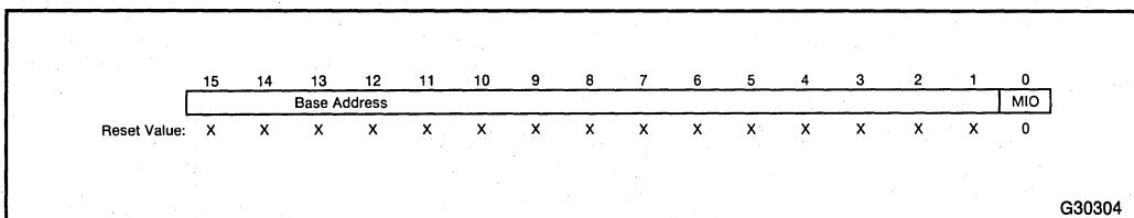
Figure 4-3. Relocation Register
