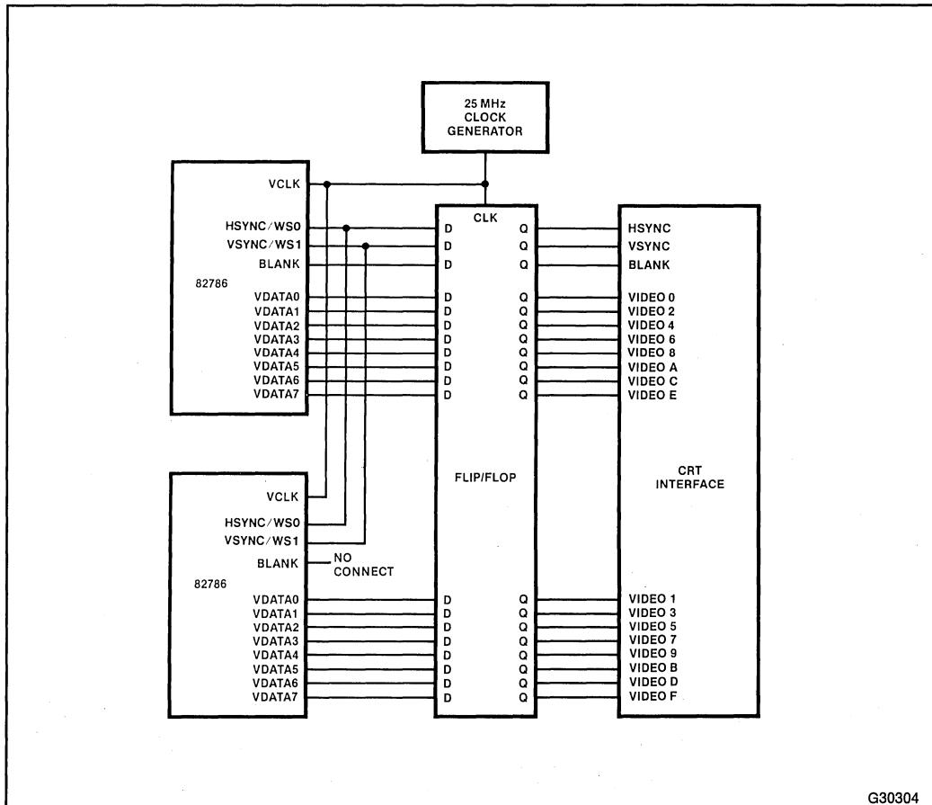
**Figure 6-14. Dual 82786s Generate 16 Bpp at 25 MHz**
