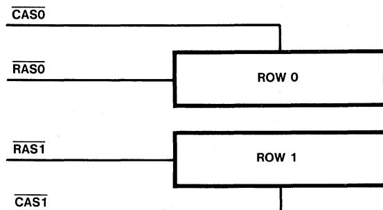
The third special case occurs with 1 M  $\times 1$  DRAMs. The 82786 multiplexes two mutually exclusive signals, DRA9 and RAS3, on the same pin. DRA9 is needed for 1M  $\times 1$  DRAMs only. Configuring more than two rows is impossible due to address space limitations, thus RAS3 is not needed. When 1 M height is programmed in the DRAM/VRAM Control Register (see Section 4.2.4), the DRA9/RAS3 pin functions as DRA9; otherwise, it functions as RAS3.
