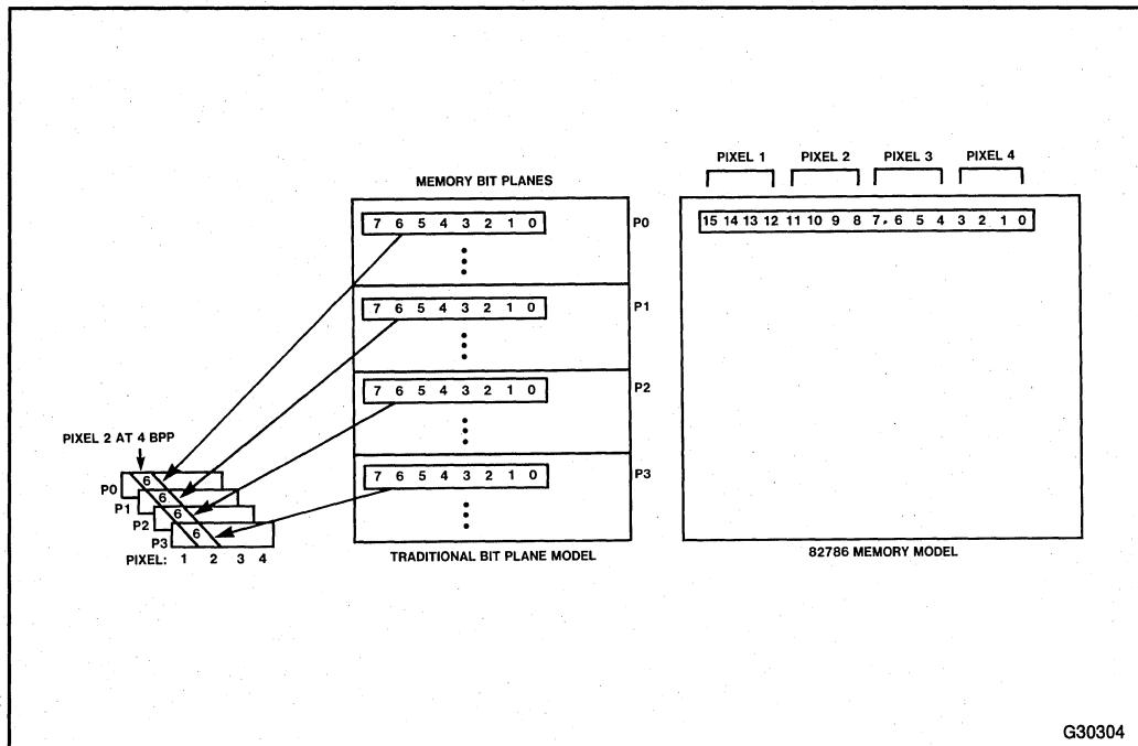
Figure 1-2. Sequential Ordering Replaces Traditional Bit Plane Model
