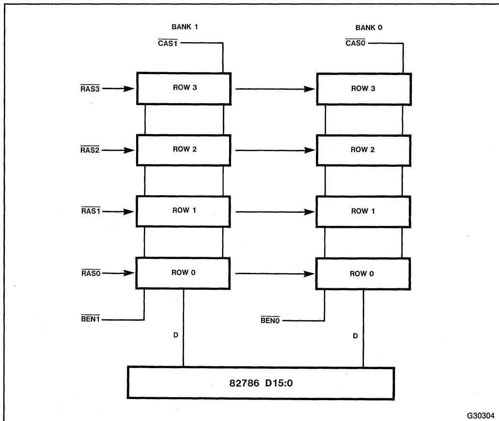
Figure 5-7. Data Line Connections  $\times 4$  and  $\times 8$
