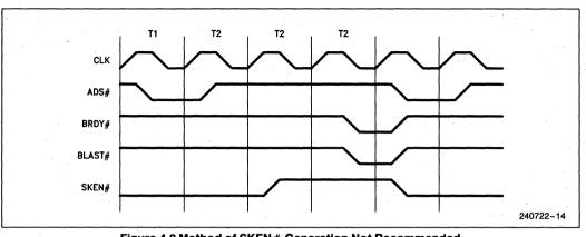
Figure 4.2 Method of SKEN# Generation Not Recommended
