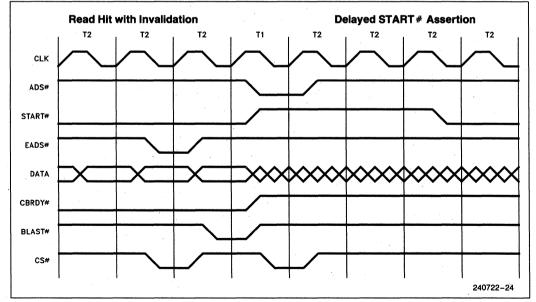
Figure 9.6. Invalidation Causing Delayed START#
