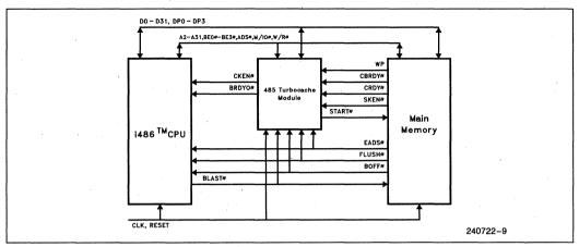
Figure 2.1. 485Turbocache Module Typical Configuration
