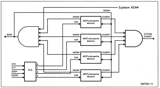
**Figure 3.2 Multiple Cache Configuration**
