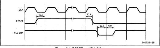
Figure 9.4. RESET and FLUSH #
