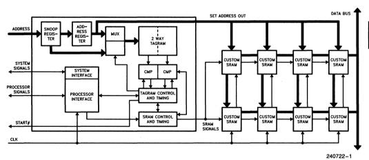
Figure 0.1. 485Turbocache Module Internal Block Diagram
