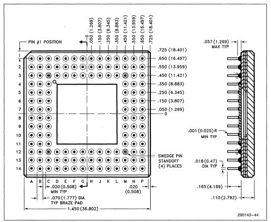
Figure 8-3.1. 132-Pin PGA Package Dimensions
