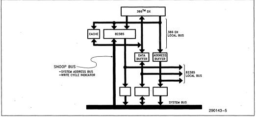
Figure 1-4. 82385 Bus Watching--Monitor System Bus Write Cycles
