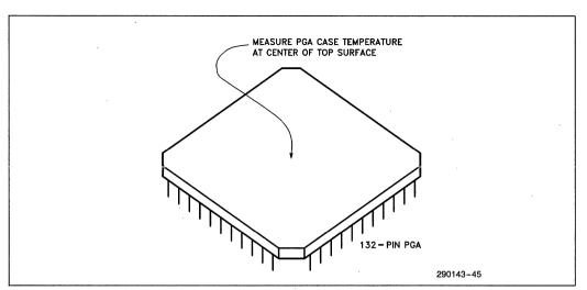
Figure 8-4. Measuring 82385 PGA Case Temperature
