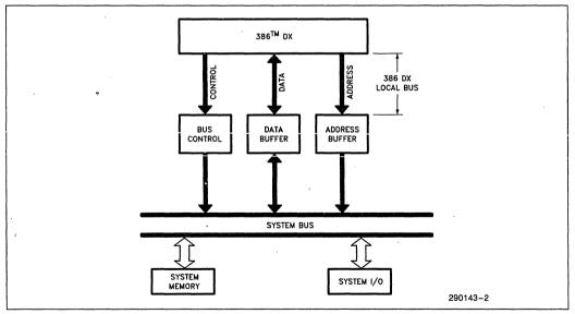
Figure 1-1. 386 DX System Bus Structure
