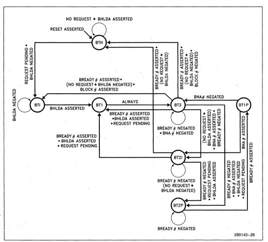
Figure 5-1B. 82385 Local Bus State Machine—Slave Mode
