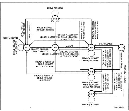
Figure 5-1A. 82385 Local Bus State Machine—Master Mode
