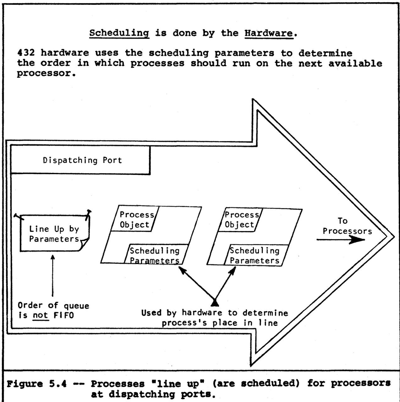
In summary, a process is scheduled as soon as it is sent to the dispatching port. The hardware compares its scheduling parameters with the scheduling parameters of the other processes already lined up at the port, and schedules the process by placing it in line at the appropriate position.
