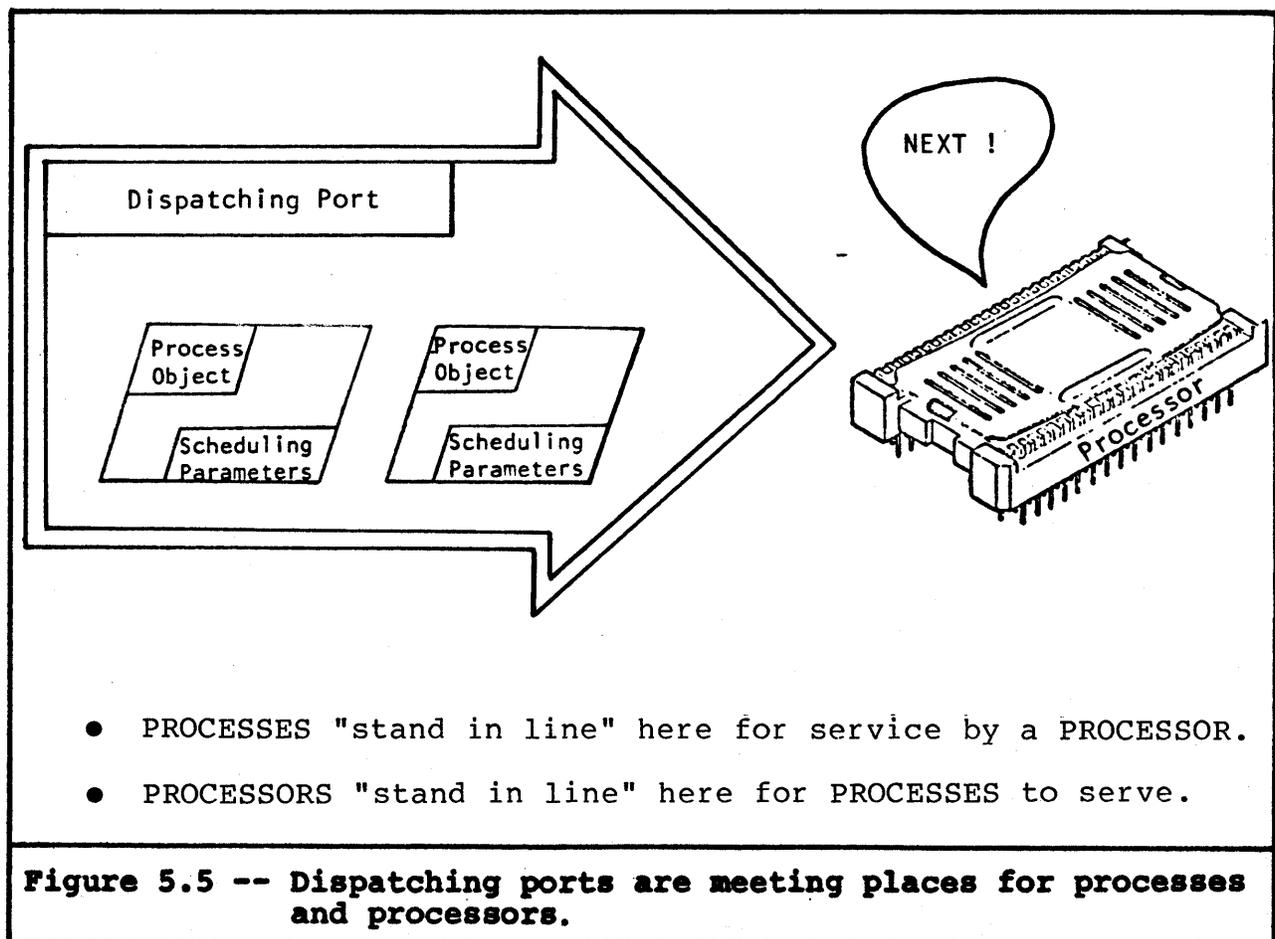
When a processor needs a process to execute, it simply removes the first process in line at its dispatching port and begins to execute it. If there are no processes waiting at the dispatching port, then the processor waits at the dispatching port until one is sent to the port (just like a process waits for a message at a communication port), see Figure 5.6.
