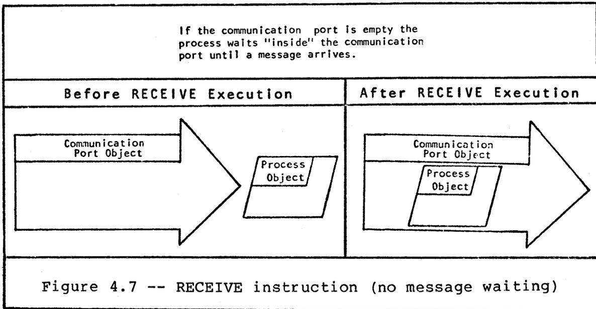
If a process executes a RECEIVE instruction and the communication port is empty, the process waits "inside" the communication port until a message is sent. Remember that messages are objects and that a process is just a special type of object. Therefore, processes can queue up waiting for messages just like messages can queue up waiting to be received by processes.
