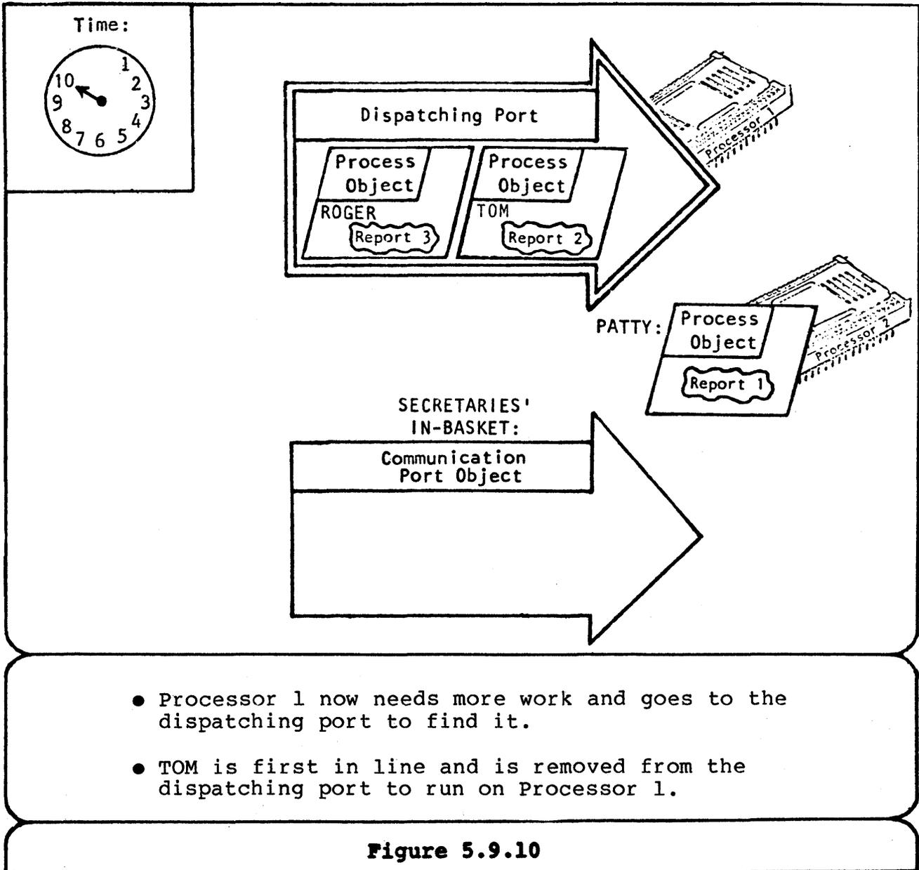
At Time 11 (Figure 5.9.11), there are two processes running. TOM is running on Processor 1 and PATTY is still running on Processor 2. ROGER is ready to run, and would be able to run if there were a third processor in the system. But, since there are only 2 processors in this example, ROGER must wait his turn at the dispatching port.
