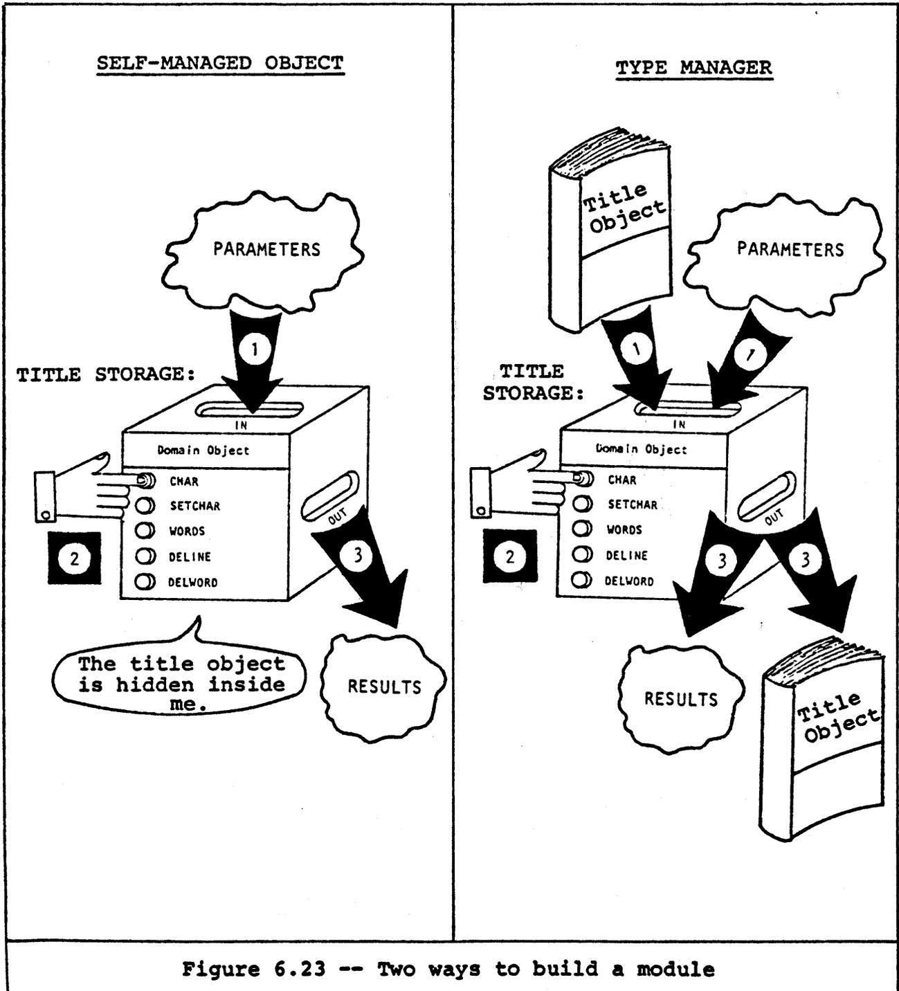
The major advantage of type managers is that a new instance of the module is not needed for each new instance of the object. One module can be used as the type manager for many instances of the object.
