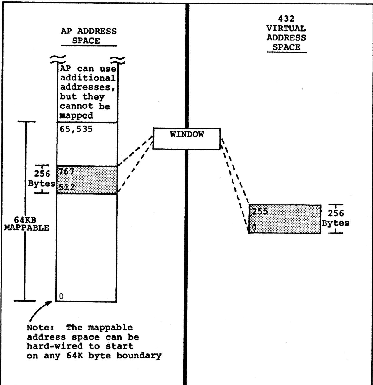
Figure 7.6 -- A window maps addresses from the AP address space to the 432 address space.
