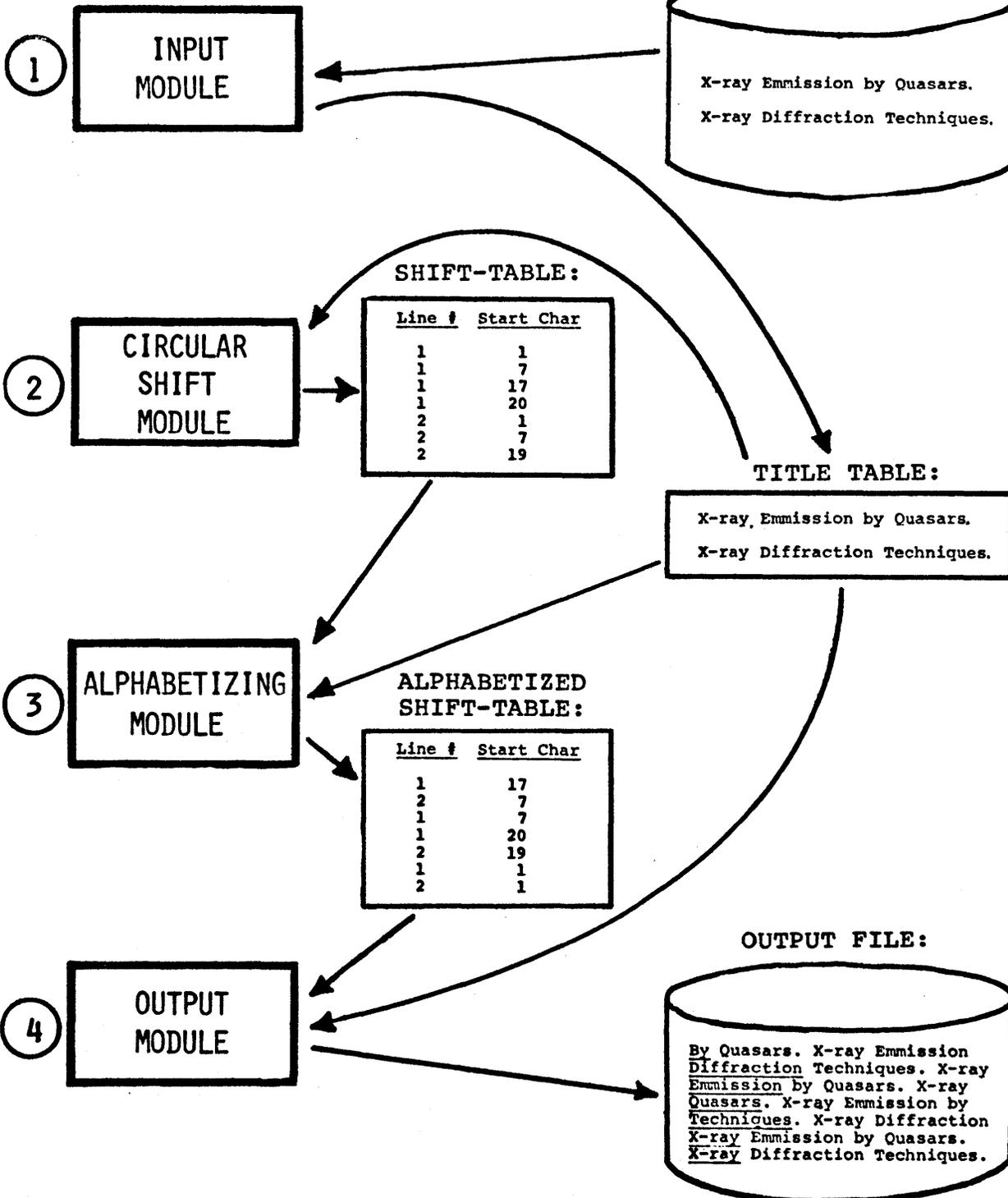
Figure 6.6 -- These modules directly manipulate shared data structures.
