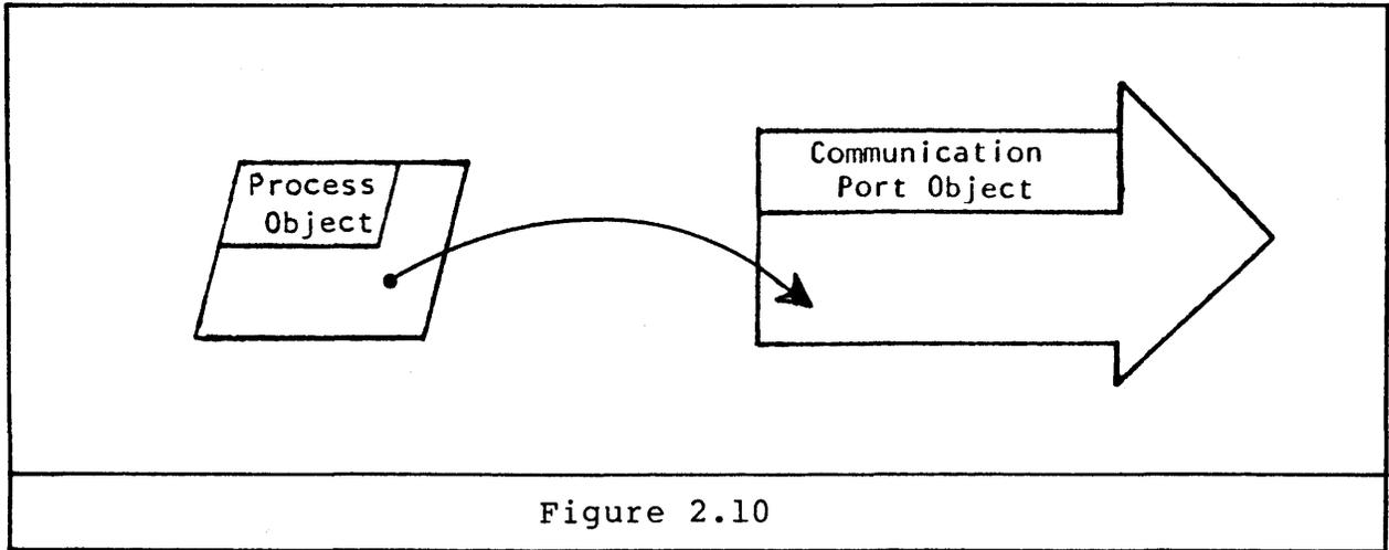
indicates that the process object can access the communication port object because it has a reference for it.
