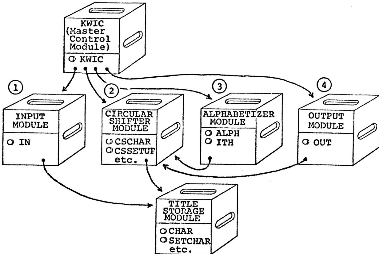
**Figure 6.17** -- These modules share information by using services (procedures) provided by other modules instead of directly manipulating shared data structures.
