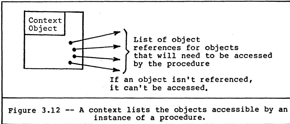
Figure 3.12 -- A context lists the objects accessible by an instance of a procedure.
