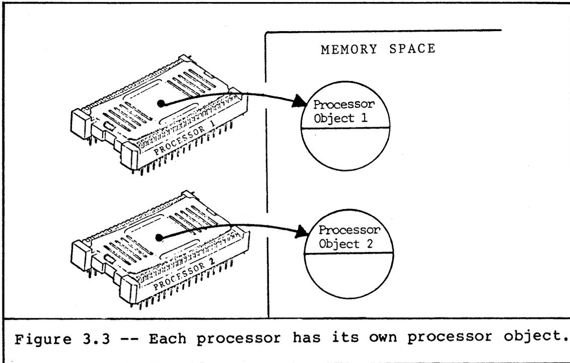
Figure 3.3 -- Each processor has its own processor object.
