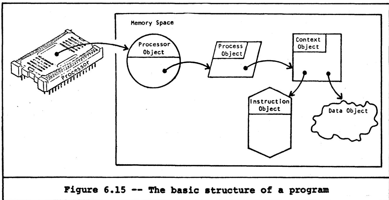
Figure 6.15 -- The basic structure of a program
