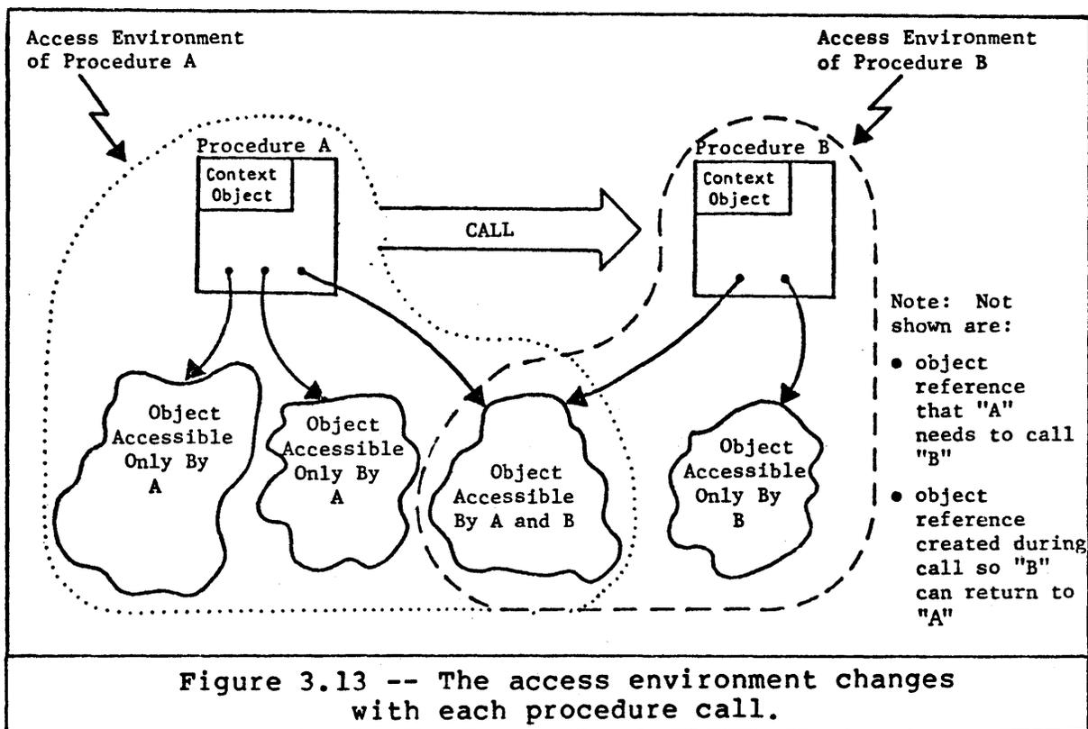
Note that this means that the 432 has a finer "protection granularity" than most machines. The protected access environment is at the procedure level, not at the process or job level as on most machines that have protection. We'll look at the advantages this provides in Chapter 6.
