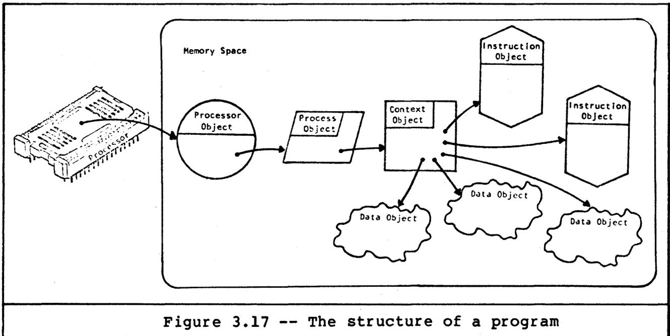
Figure 3.17 -- The structure of a program
