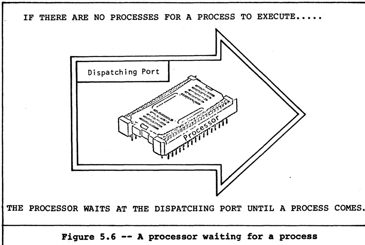
Figure 5.6 is a conceptual view of a processor waiting at a dispatching port. Figure 5.7 shows what really happens. An object reference for the waiting processor's processor object is queued at the dispatching port.
