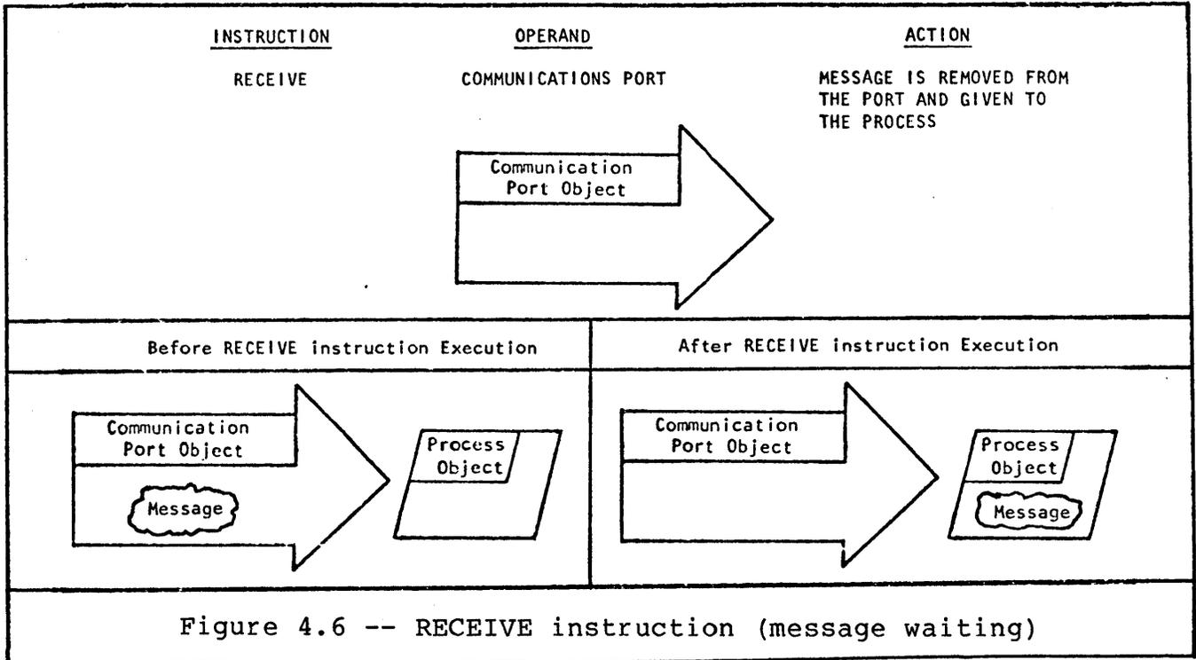
The RECEIVE instruction has one operand: the communication port where the message is to be received. Figure 4.6 summarizes the action of the instruction if there is a message waiting. Before RECEIVE is executed, there is a message waiting in the communication port (placed there earlier by a SEND instruction). After RECEIVE is executed, the message is moved from the port to the process executing the RECEIVE.
