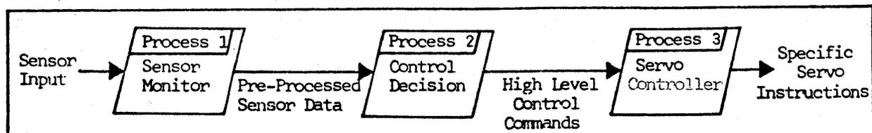
Figure 3.6 -- The structure of an example industrial control program
