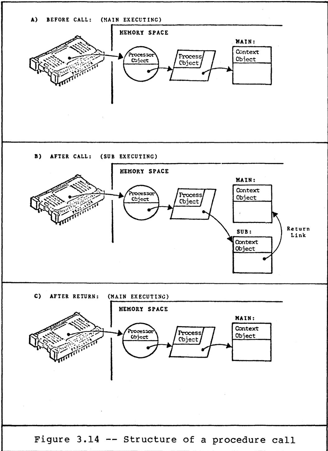
Figure 3.14 -- Structure of a procedure call
