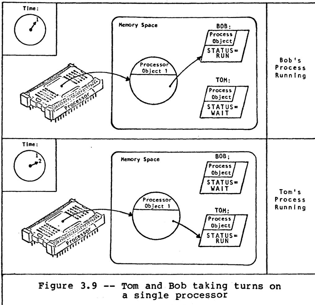
Note also that the process object contains the status information showing whether its process is running or waiting.
