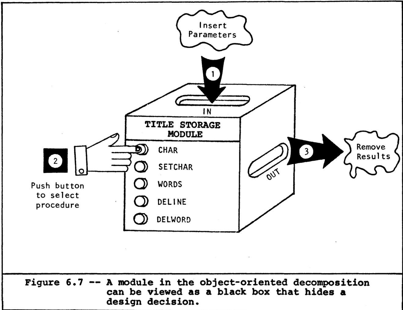
**Figure 6.7 -- A module in the object-oriented decomposition can be viewed as a black box that hides a design decision.**
