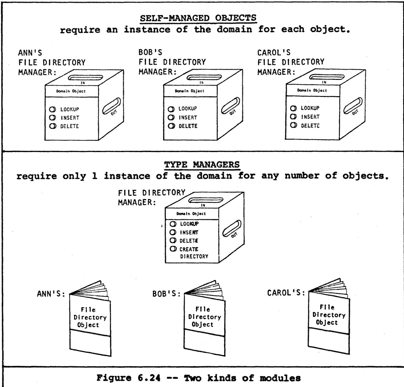
Note that with a type manager, the CREATE DIRECTORY procedure can be in the file directory manager along with the other procedures. This procedure is used to create a new directory object whenever a new user is added.
