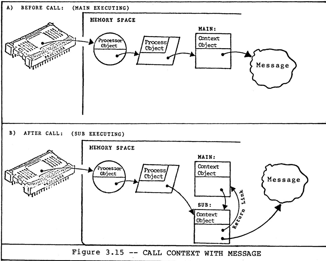
This is a powerful parameter-passing mechanism because it is general. Any object can be a message. For example, if the called procedure is sine of  $x$ , the message is simple -- it contains the value  $x$ . But, what if the called procedure is the part of the operating system that schedules processes? The message might be a process object that needs to be scheduled.
