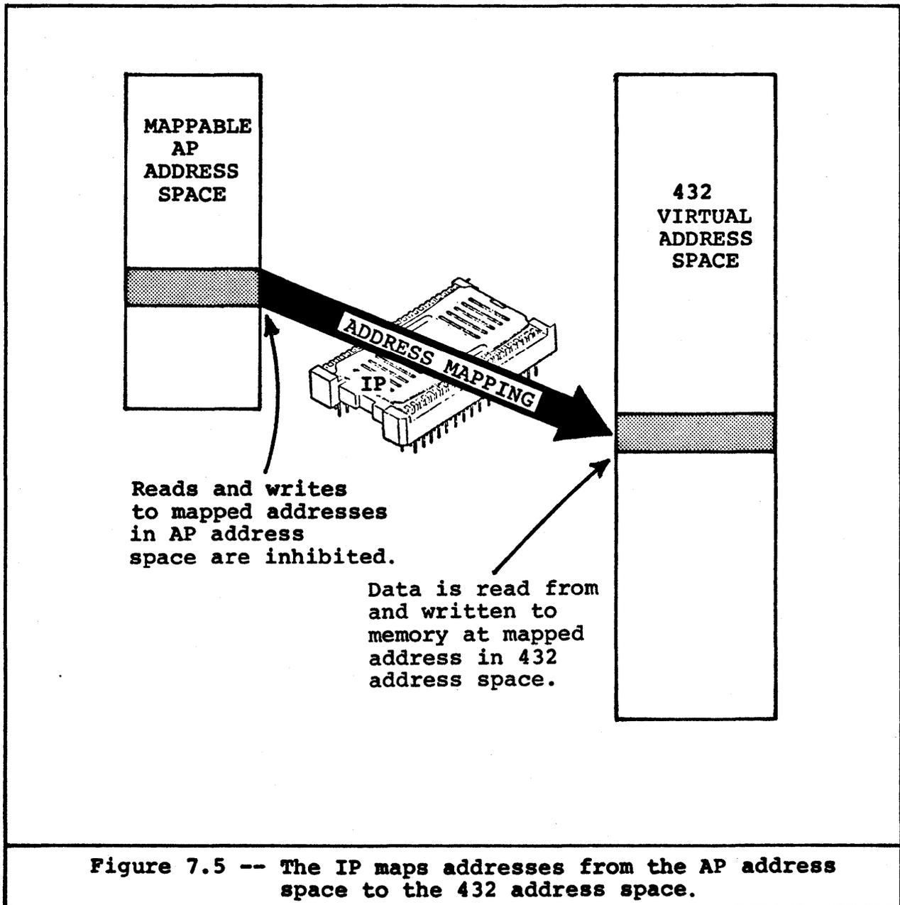
Here is a simple example with one window. Locations 512 through 767 (decimal) in the AP address space are mapped to a 256 byte segment in the 432 address space (i.e., byte 512 in the AP address space maps to byte 0 in the 432 segment, byte 513 maps to byte 1, etc. -- see Figure 7.6).
