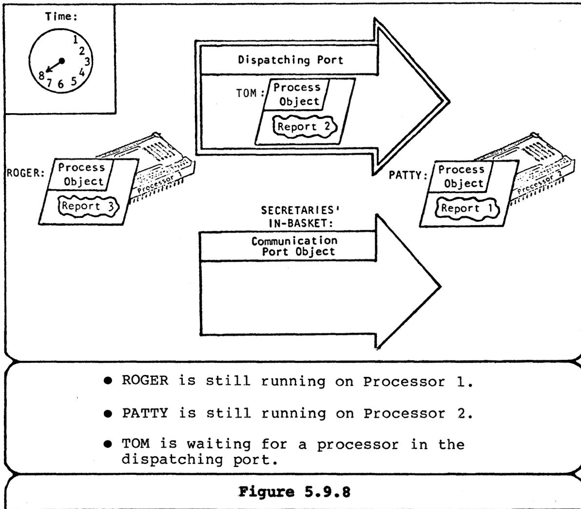
There have been two examples of what happens when a process is sent to a dispatching port. Either a processor is waiting at the port and starts executing the process immediately, or a processor is not waiting at the port and the process lines up to wait for a processor.
