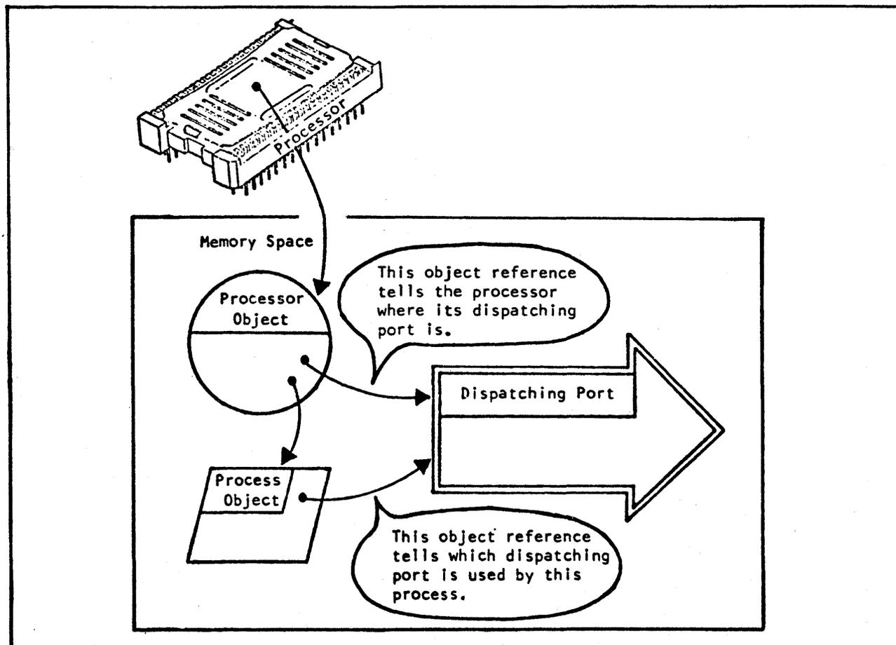
**Figure 5.10 -- Each processor object and each process object has a reference for a dispatching port.**
