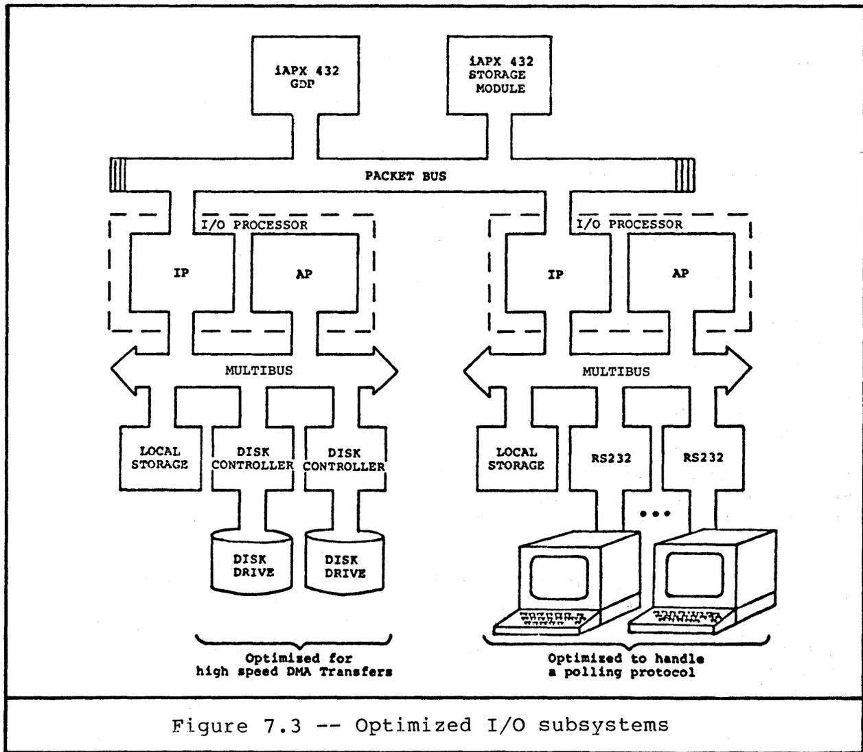
Figure 7.3 -- Optimized I/O subsystems
