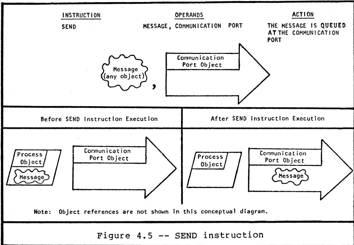
The SEND instruction has 2 operands: the message being sent and the communication port it is being sent to. Figure 4.5 summarizes the action of the instruction. Before SEND is executed, the process has a message it wants to send. After SEND is executed, the message has been sent to the specified communication port (the message is not actually copied; only an object reference is copied).
