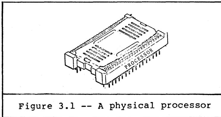
This symbol (Figure 3.1) represents a physical processor. The physical processor is not an object (it is not a data structure), although, as you'll see in the next section, there is an object called a processor object. The physical processor, however, is made of silicon, sits inside a package on a printed circuit board, and fetches and executes instructions.
