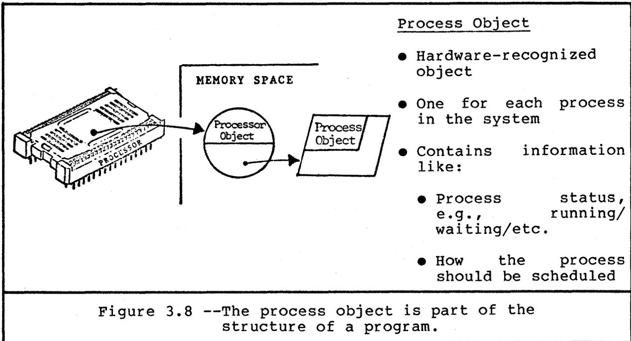
Figure 3.8 shows that the processor object contains an object reference for the process object currently running on the processor. This is important because the 432's object-oriented addressing and protection mechanism does not allow a processor to access an object unless it has an object reference for it.
