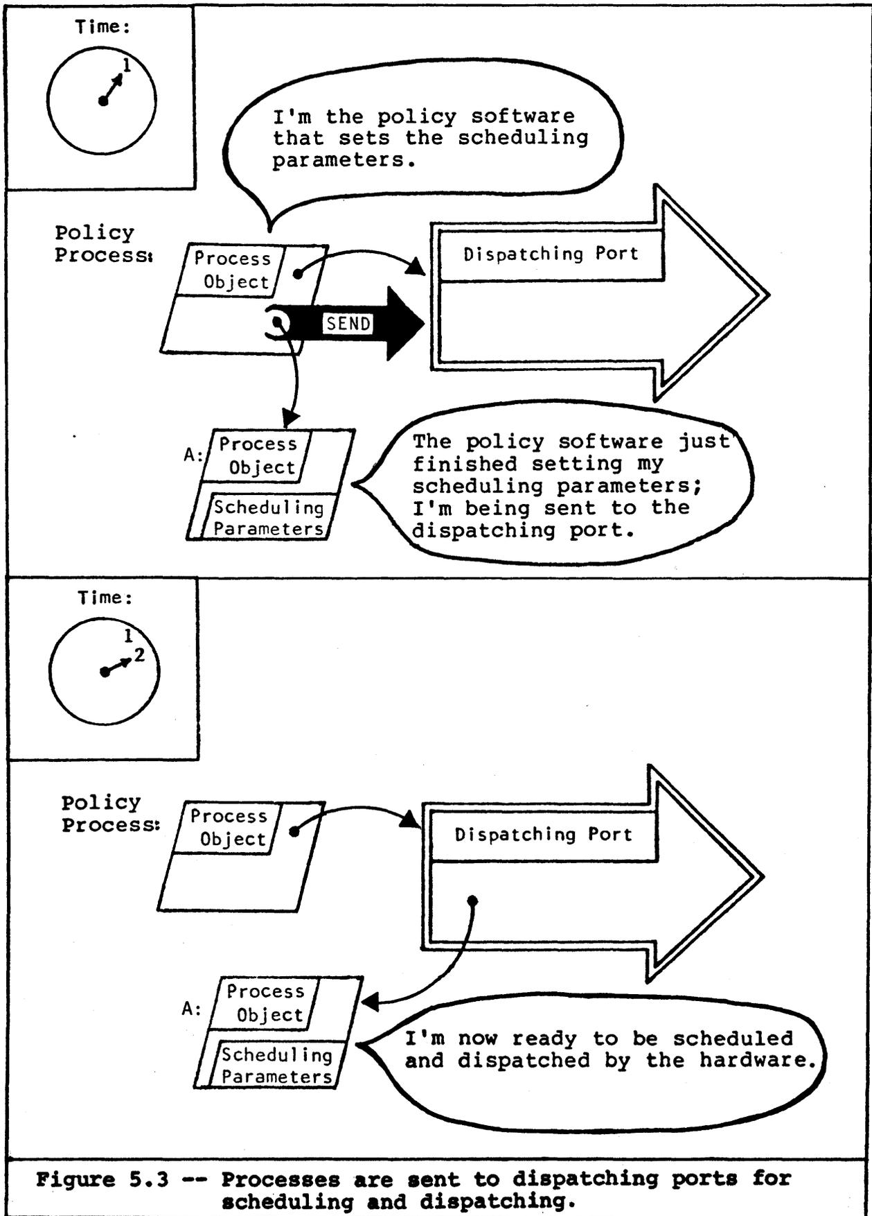
Dispatching ports are where processes "line up" (are scheduled) for execution on a processor. The first process in line is the first process that will be assigned to a processor.
