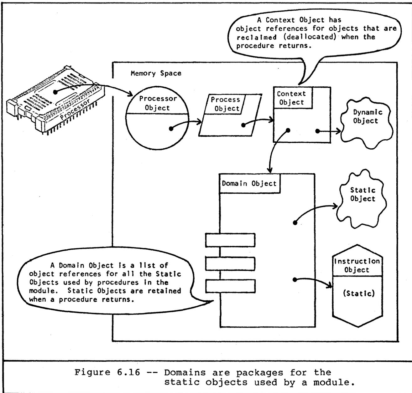
Figure 6.16 -- Domains are packages for the static objects used by a module.
