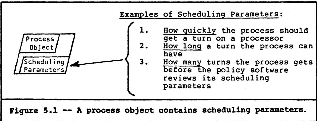
**Figure 5.1 -- A process object contains scheduling parameters.**
