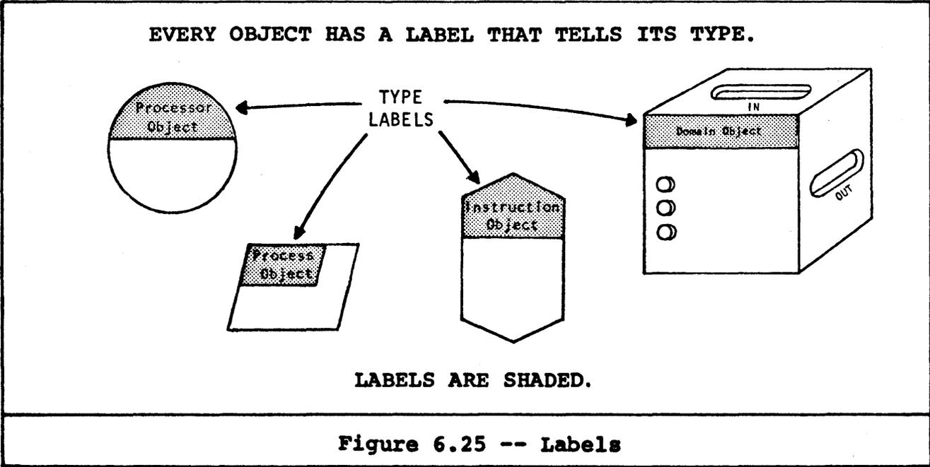
These labels are used to solve the first problem discussed in the last section -- insuring that the object to be manipulated is of the proper type.
