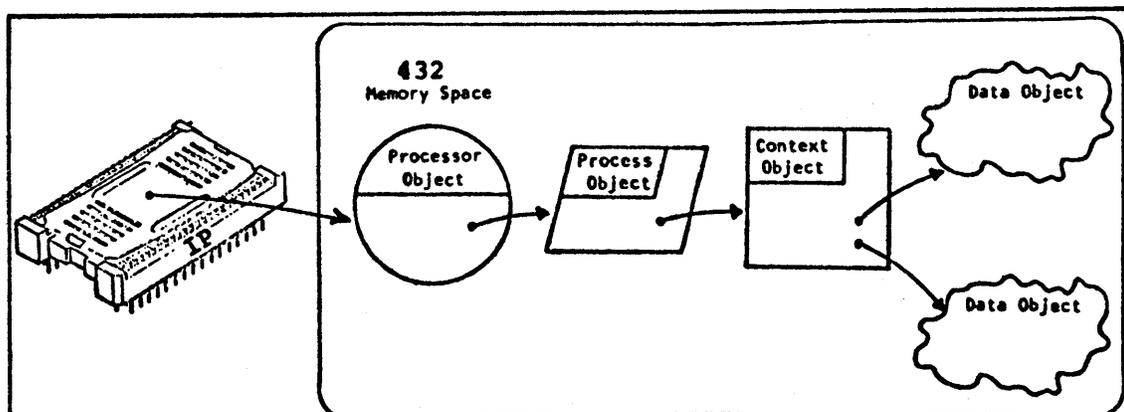
Figure 7.4 -- The structure of an IP "program"
