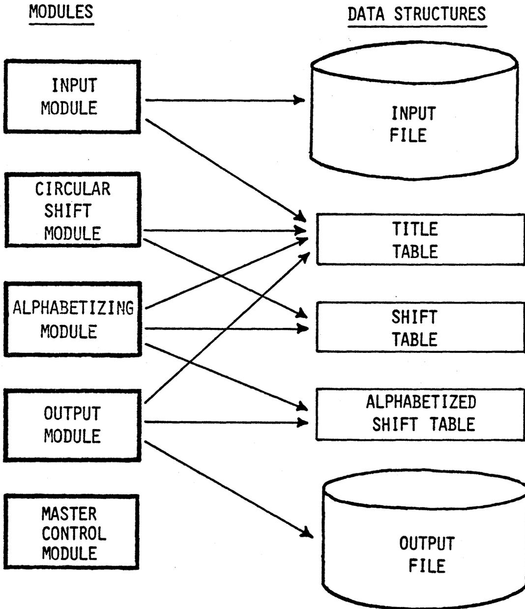
ARROWS POINT TO ALL THE DATA STRUCTURES THAT ARE DIRECTLY MANIPULATED BY A MODULE.
