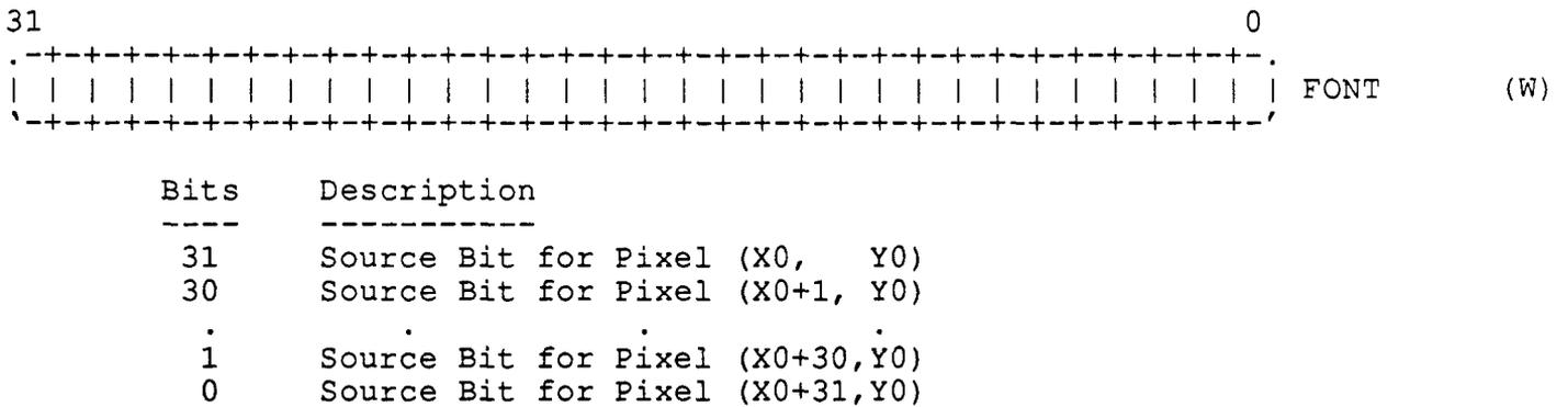
Figure 7-3 FONT Register Format (COLOR1 mode & 68020/SPARC mode)
