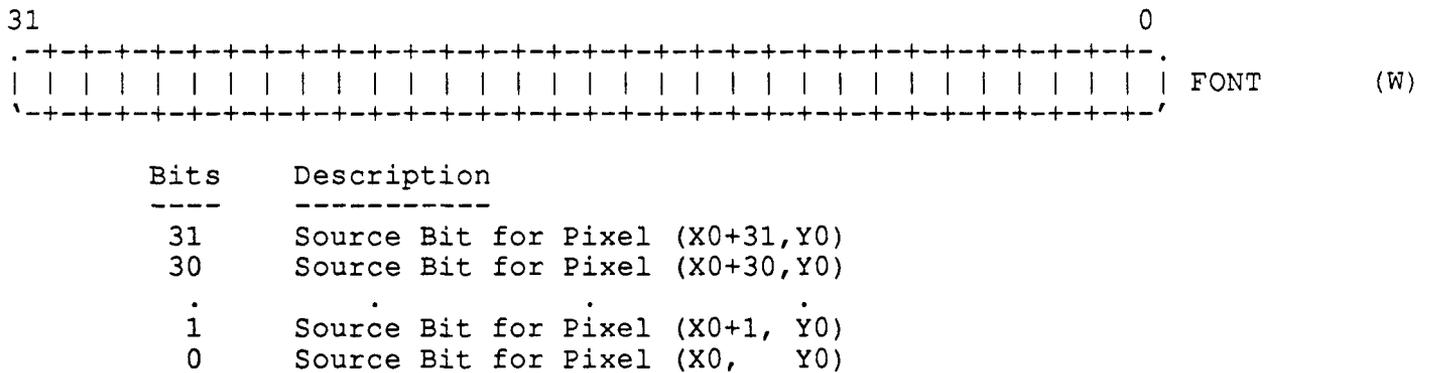
Figure 7-4 FONT Register Format (COLOR1 mode & 80386 mode)
