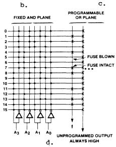
FIGURE 8. Exclusive-OR gates can be implemented in PLEs very efficiently. A 4-input XOR gate (a) maps into a checkerboard pattern in a Karnaugh Map (b) and requires eight products terms (c). The PLE implementation is shown in (d). An 8-input XOR gate requires sixteen product terms.
