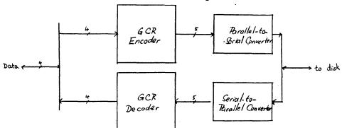
FIGURE 7. GCR encoder/decoder block diagram.
