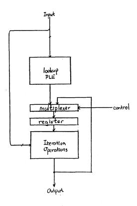
FIGURE 9. PLE look-up tables and iteration loops can be used to generate very accurate trigonometric and arithmetic functions. An approximation to the function is stored in a PLE and additional accuracy is gained using iteration operations.
