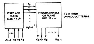
FIGURE 3. Block diagram of a PROM viewed as a PLE. Notice that the PLE provides many (2<sup>n</sup> where n is the number of inputs) product terms. A by-product of this is programmable output polarity; either Active High or Active Low output polarity is available.
