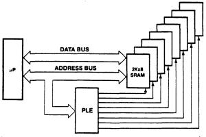
FIGURE 4. PLE address decoding application. The PLE select one of eight 2Kx8 Static RAMs by decoding several microprocessor address lines.
