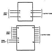
FIGURE 5. Two examples of PLE code converters. The second example illustrates how to use two inputs as code select lines so that four converters can be provided in one PLE.
