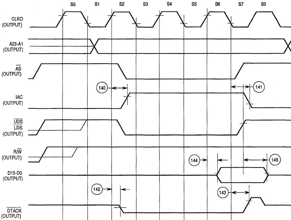
Figure 6-11. Internal Master Internal Read Cycle Timing Diagram
