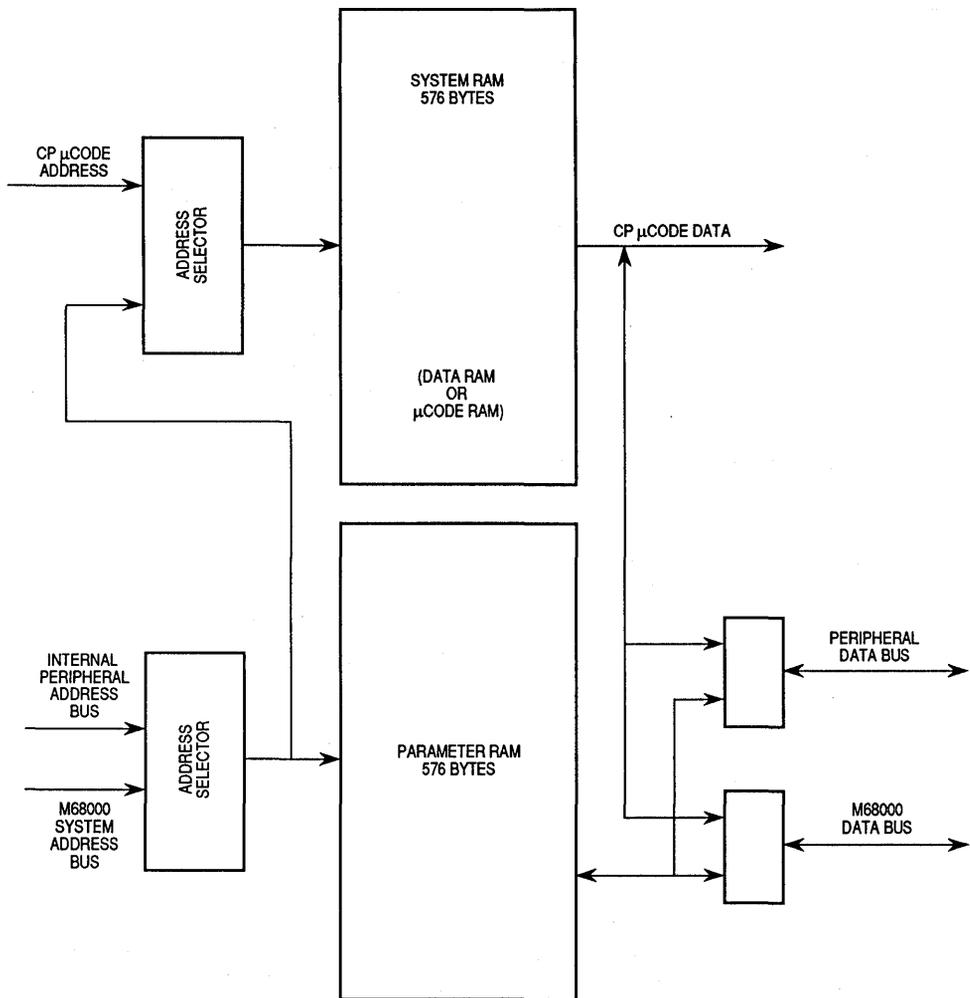
Figure 3-4. RAM Block Diagram
