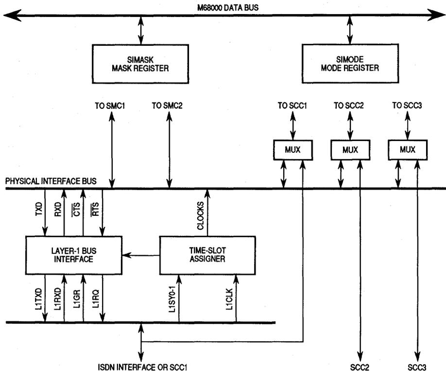
**Figure 4-1. Serial Channels Physical Interface Block Diagram**
