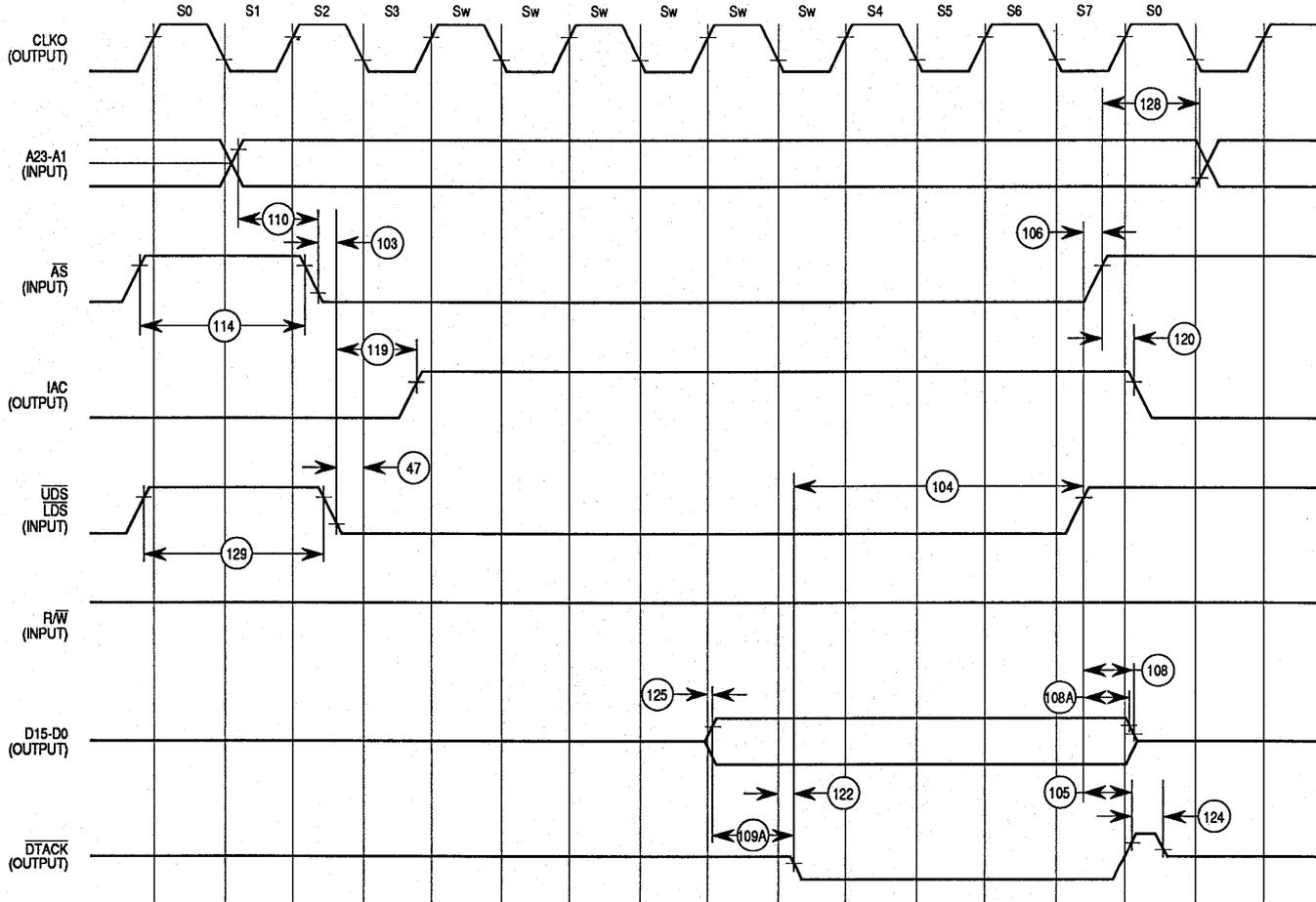
Figure 6-6. External Master Internal Asynchronous Read Cycle Timing Diagram
