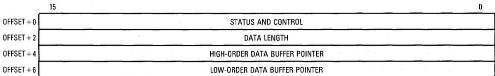
**Figure 4-8. SCC Buffer Descriptor Format**
