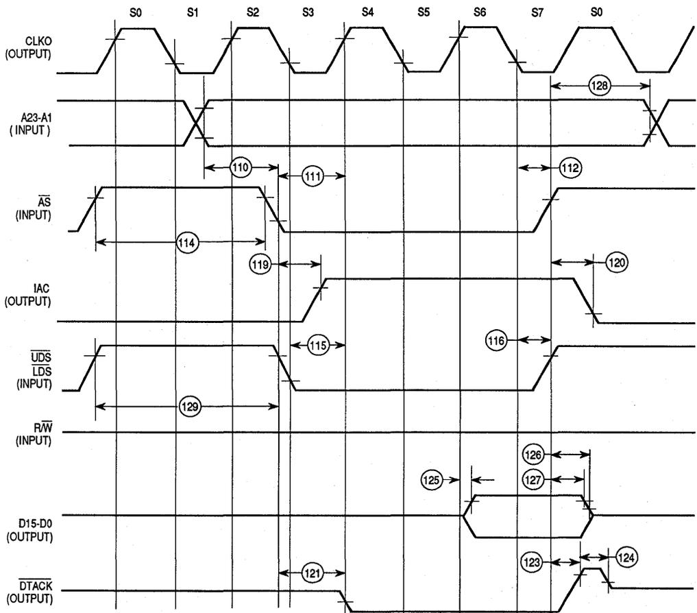
**Figure 6-8. External Master Internal Synchronous Read Cycle Timing Diagram**
