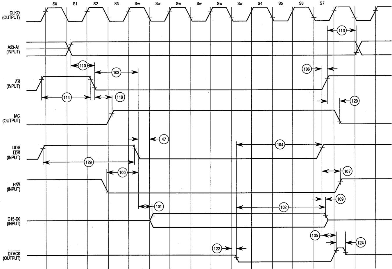
Figure 6-7. External Master Internal Asynchronous Write Cycle Timing Diagram
