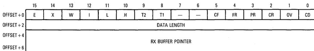
**Figure 4-21. DDCMP Receive Buffer Descriptor**
