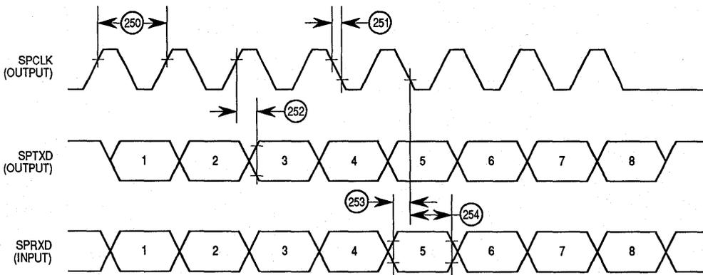
Figure 6-17. Serial Communication Port Timing Diagram
