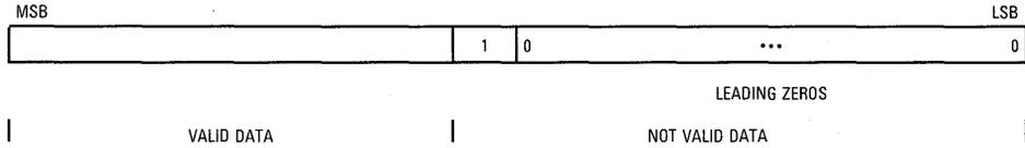
5. CRC Error. When this error occurs, the channel writes the received CRC to the data buffer, closes the buffer, sets the CR bit in the BD, and generates the RXF interrupt (if enabled). The channel also increments the CRC error counter (CRCEC). After receiving a frame with a CRC error, the receiver enters hunt mode. (An immediately following back-to-back frame will be received.) CRC checking cannot be disabled, but the CRC error may be ignored if checking is not required.
