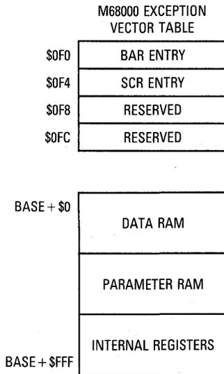
**Figure 2-5. MC68302 IMP Configuration Control**
