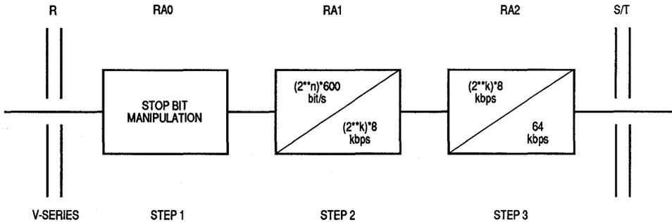
**Figure 4-24. Three-Step Asynchronous Bit Rate Adaption**
