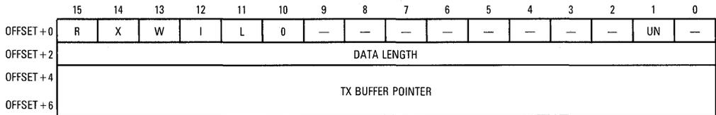
**Figure 4-26. V.110 Transmit Buffer Descriptor**
