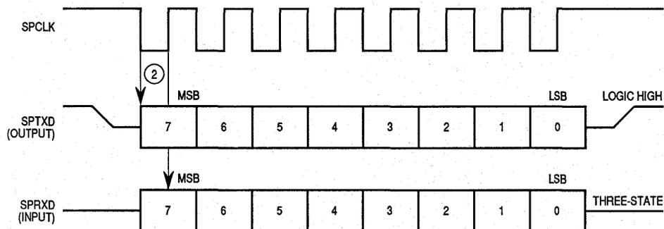
NOTE: Transmitted data bits shift on falling edges; received bits are sampled on rising edges.
