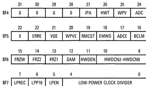
Figure 3-8. System Control Register
