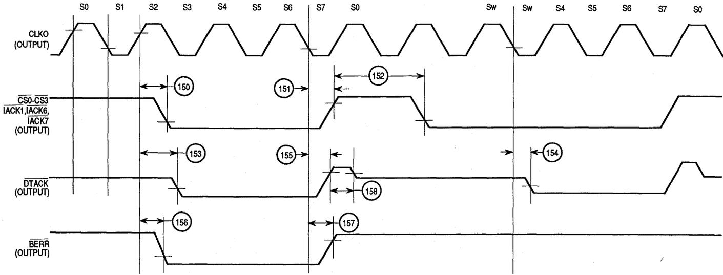
Figure 6-12. Internal Master Chip-Select Timing Diagram
