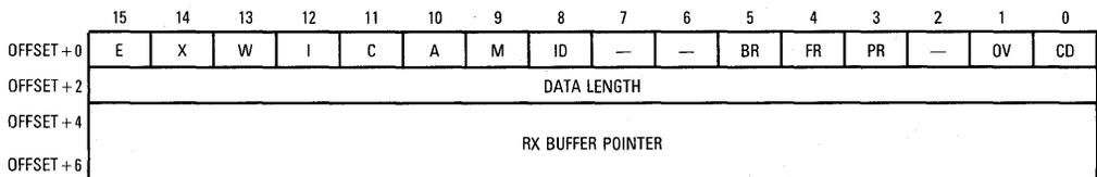
**Figure 4-11. UART Receive Buffer Descriptor**
