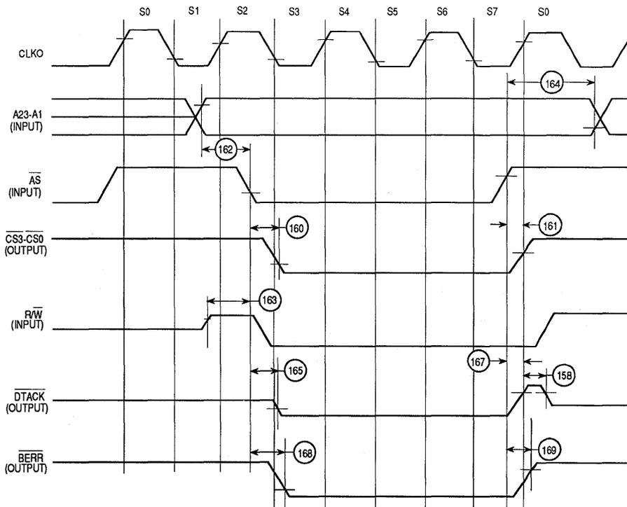
Figure 6-13. External Master Chip-Select Timing Diagram
