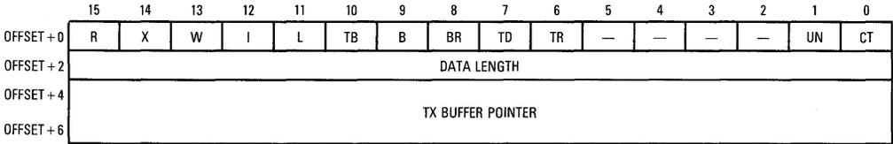
**Figure 4-19. BISYNC Transmit Buffer Descriptor**
