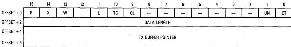
**Figure 4-22. DDCMP Transmit Buffer Descriptor**
