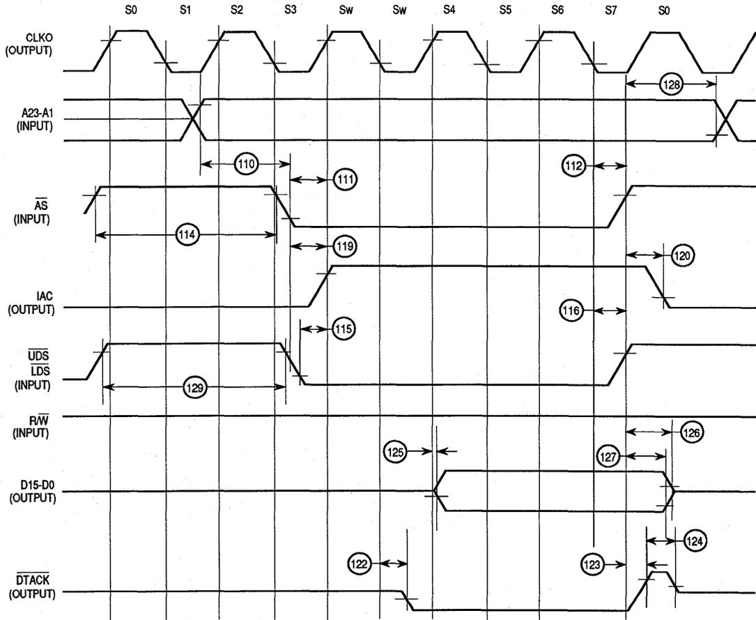
Figure 6-9. External Master Internal Synchronous Read Cycle Timing Diagram (One Wait State)
