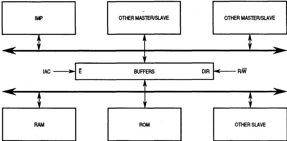
**Figure 5-2. External Address/Data Buffer**
