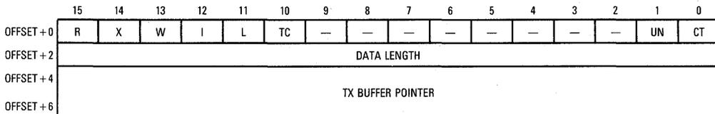
**Figure 4-15. HDLC Transmit Buffer Descriptor**
