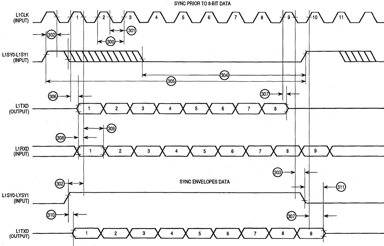
Figure 6-20. PCM Timing Diagram
