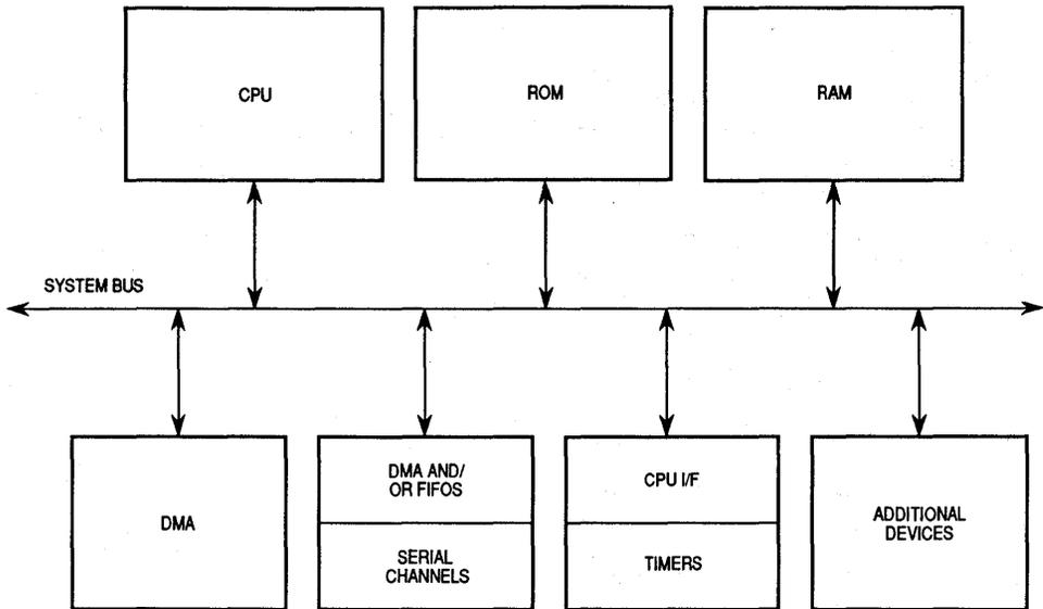
**Figure 1-2. General-Purpose Microprocessor System Design**
