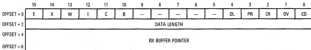
**Figure 4-18. BISYNC Receive Buffer Descriptor**
