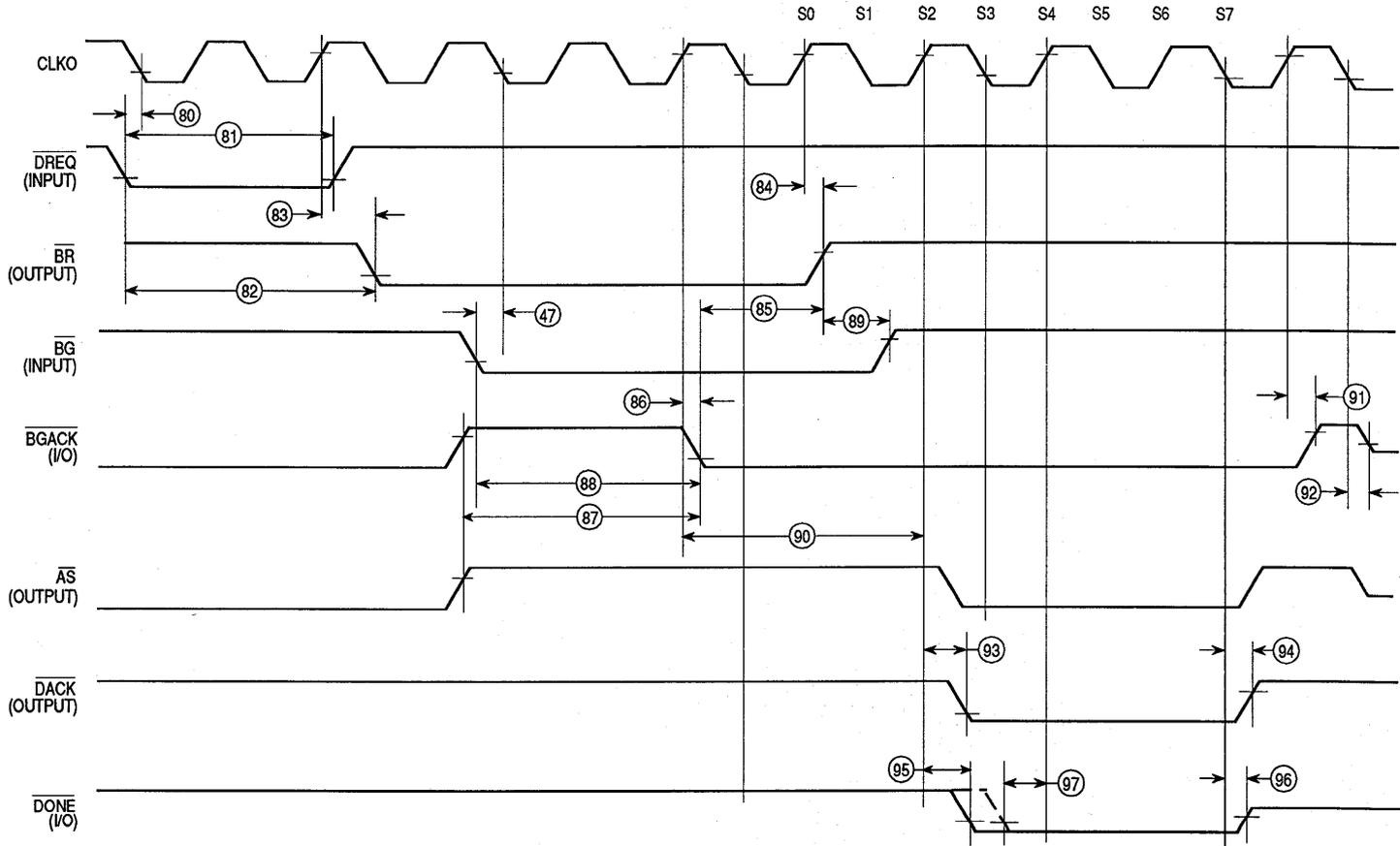
Figure 6-5. DMA Timing Diagram
