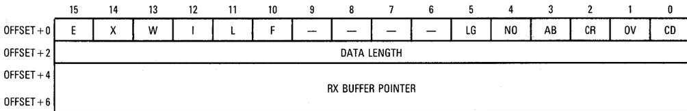
**Figure 4-14. HDLC Receive Buffer Descriptor**
