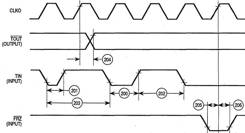
Figure 6-16. Timers Timing Diagram
