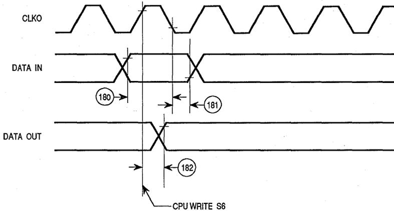
Figure 6-14. Parallel I/O Data In/Data Out Timing Diagram
