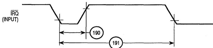
Figure 6-15. Interrupts Timing Diagram
