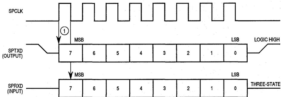
NOTE: Transmitted data bits shift on rising edges; received bits are sampled on falling edges.
