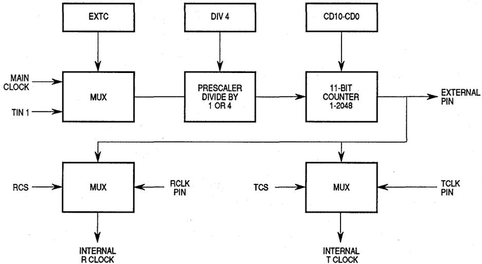
Figure 4-6. SCC Baud Rate Generator
