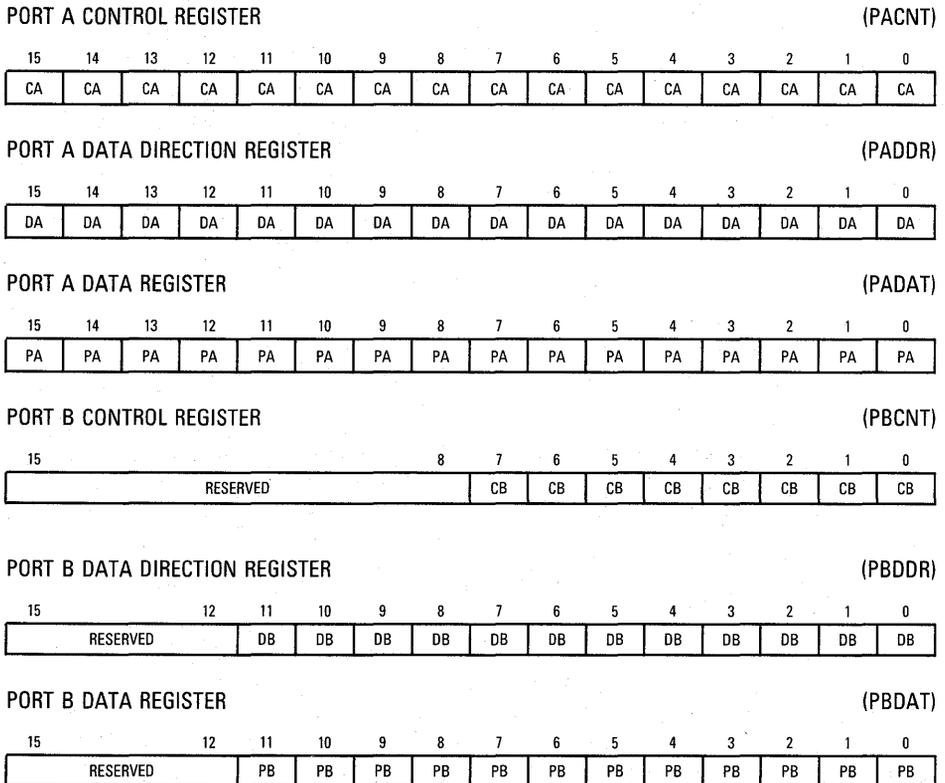
**Figure 3-3. Parallel I/O Port Registers**
