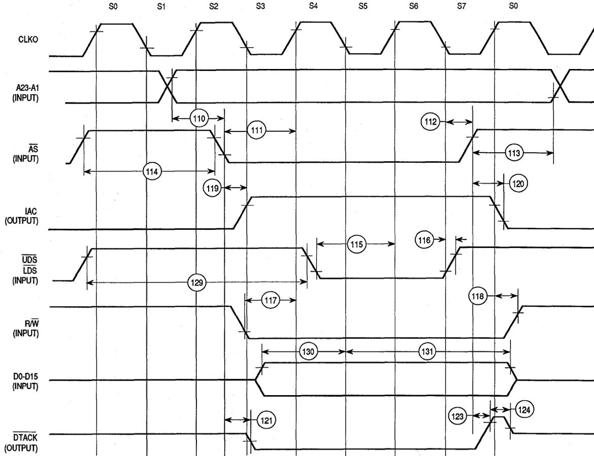
Figure 6-10. External Master Internal Synchronous Write Cycle Timing Diagram
