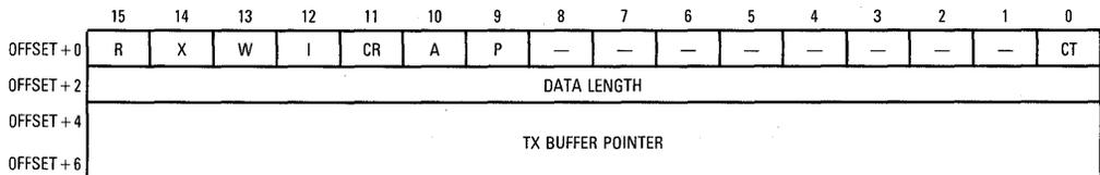
**Figure 4-12. UART Transmit Buffer Descriptor**
