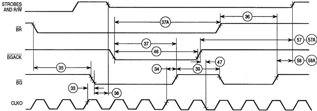
NOTE: Setup time to the clock (#47) for the asynchronous inputs  $\overline{BERR}$ ,  $\overline{BGACK}$ ,  $\overline{BR}$ ,  $\overline{DTACK}$ , and  $\overline{IPL2-IPL0}$  guarantees their recognition at the next falling edge of the clock.
