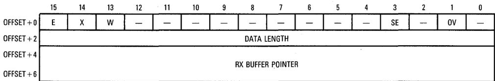
**Figure 4-25. V.110 Receive Buffer Descriptor**
