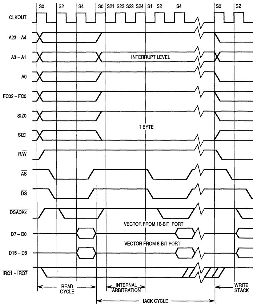
Figure 3-23. Interrupt Acknowledge Cycle Timing
