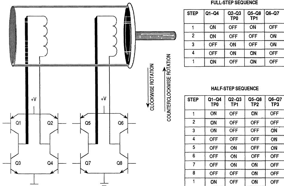
**Figure 8-6. Two-Phase Stepper Motor with H-Bridge Drive and Step Sequences**
