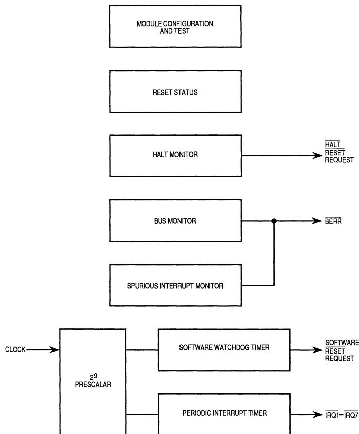
**Figure 4-3. System Configuration and Protection Submodule**
