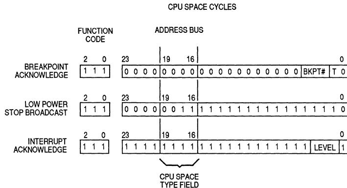
**Figure 3-17. CPU Space Address Encoding**
