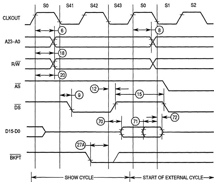
NOTE: All timing with respect to 20% and 70% V<sub>DD</sub>
