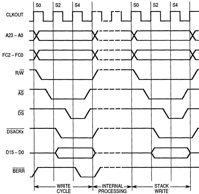
Figure 3-26. Late Bus Error with DSACK<sub>x</sub>
