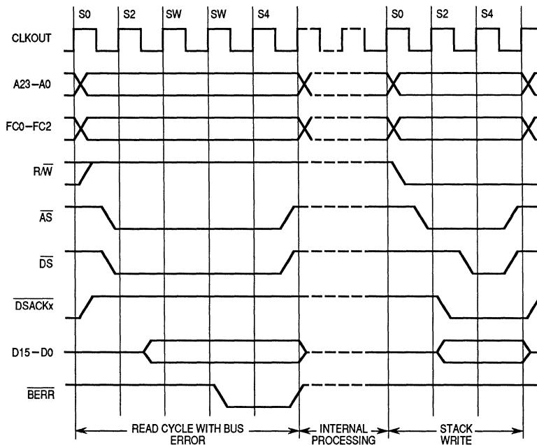
Figure 3-25. Bus Error without DSACK<sub>x</sub>
