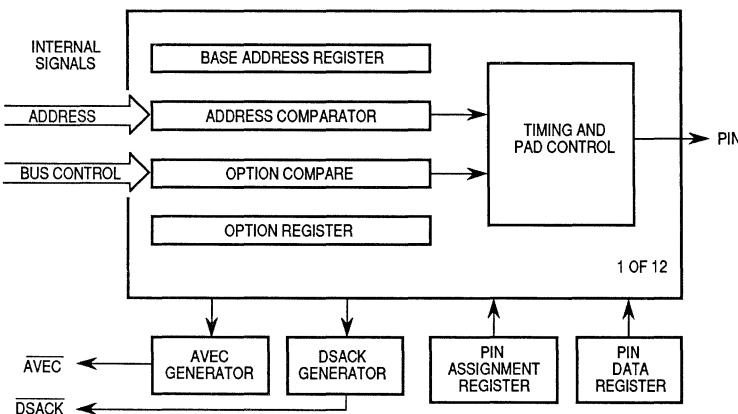
**Figure 4-14. Chip-Select Circuit Block Diagram**
