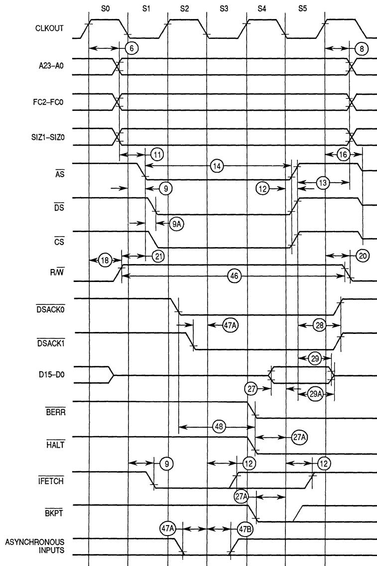
NOTE: All timing is shown with respect to 20% and 70% V<sub>DD</sub>
