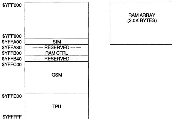
Y = M111, where M is the modmap signal state on the IMB, which reflects the state of the modmap bit in the module configuration register of the system integration module (Y= \$7 or \$F).
