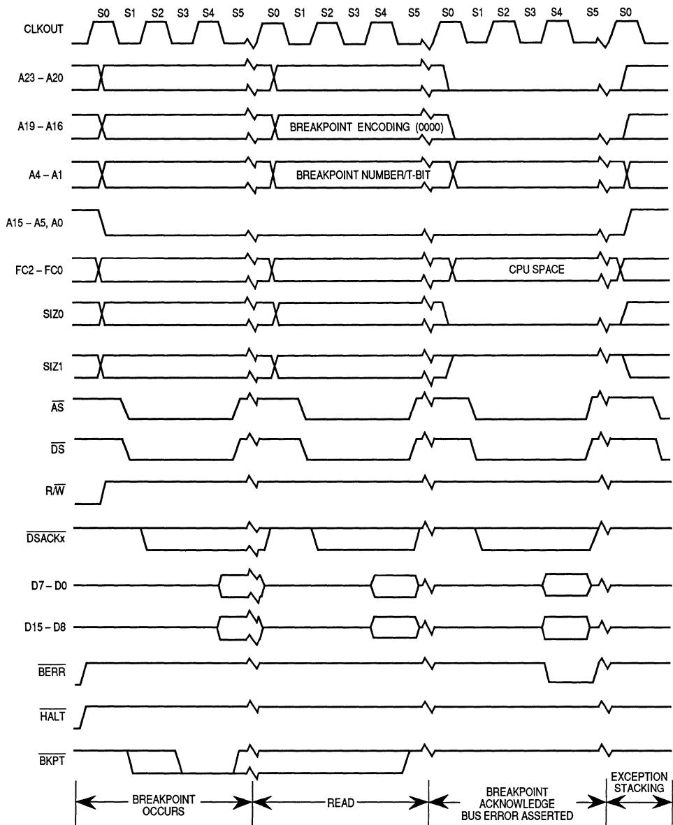
**Figure 3-21. Breakpoint Acknowledge Cycle Timing
