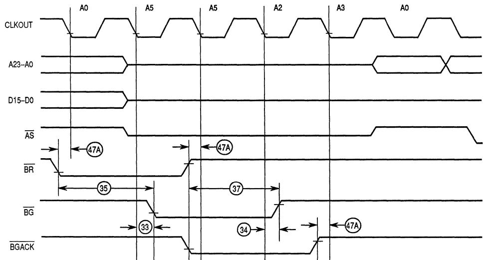
NOTE: All timing with respect to 20% and 70% V<sub>DD</sub>
