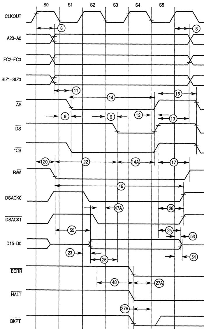
NOTE: All timing with respect to 20% and 70% V<sub>DD</sub>
