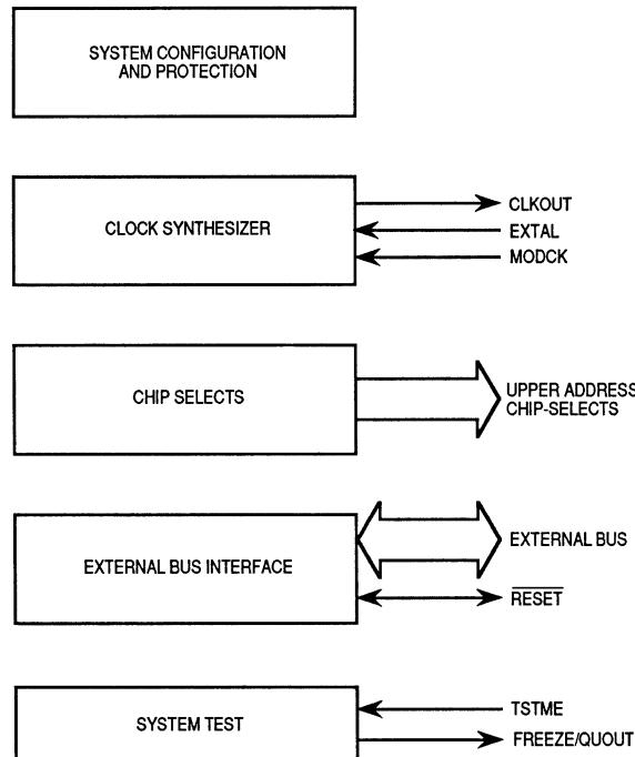
Figure 4-1. System Integration Module Block Diagram
