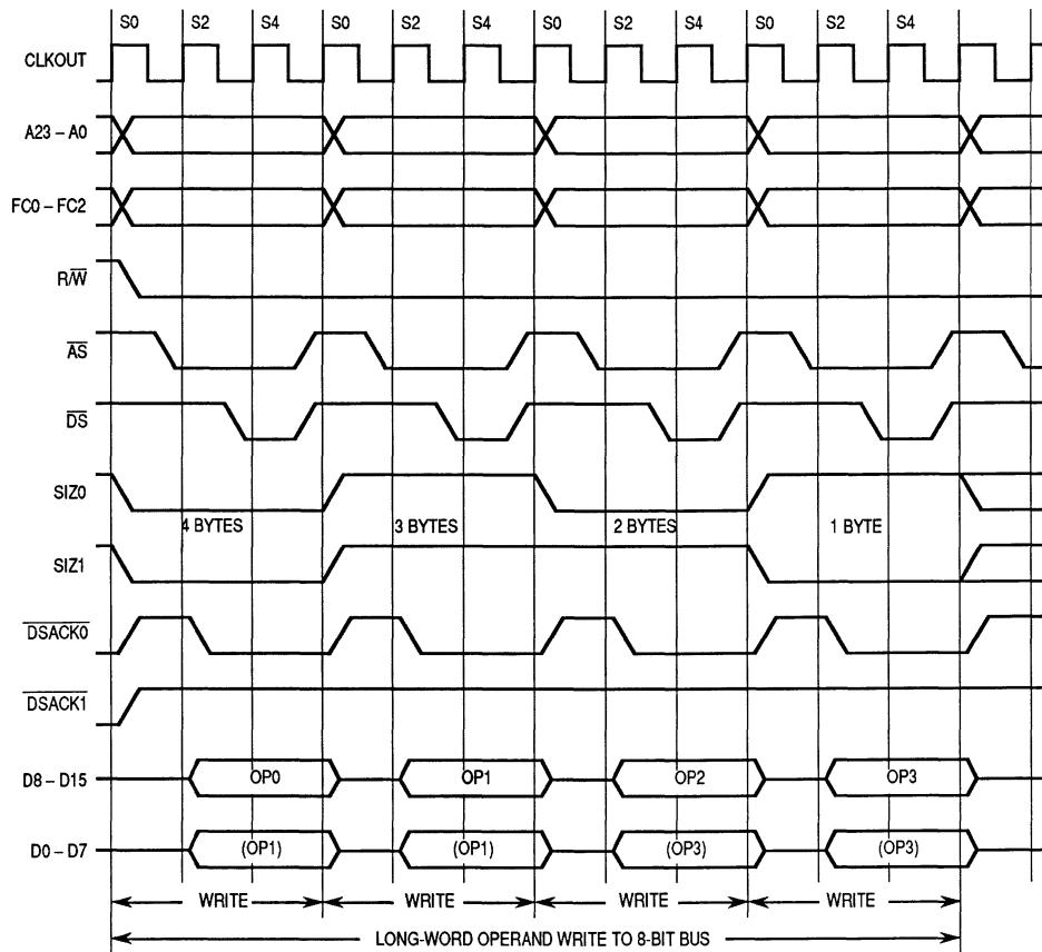
Figure 3-10. Long-Word Operand Write Timing to 8-Bit Port
