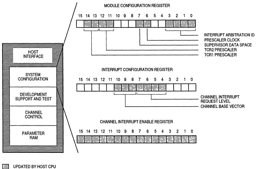
**Figure 8-4. TPU Module Configuration**
