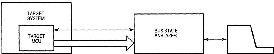
**Figure 7-11. Bus State Analyzer Configuration**
