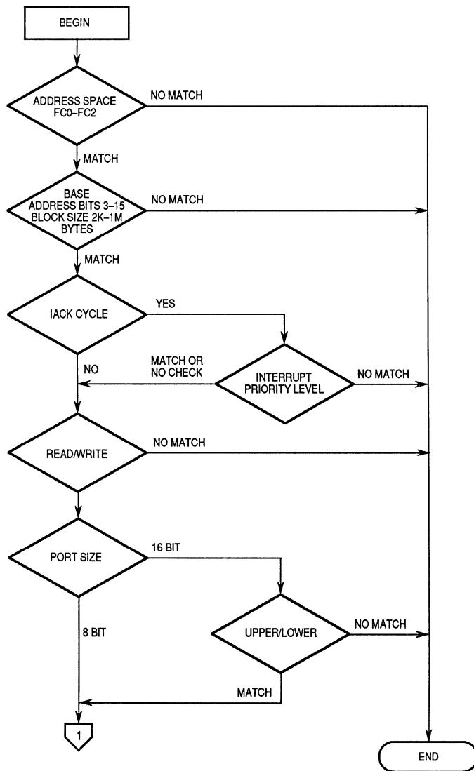
Figure 4-15. Flow Diagram for Chip Select (Sheet 1 of 3)
