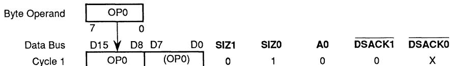
**Figure 3-4. Byte Operand to 16-Bit Port, Even (A0 = 0)**
