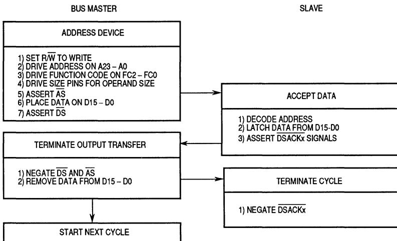
**Figure 3-15. Write Cycle Flowchart**
