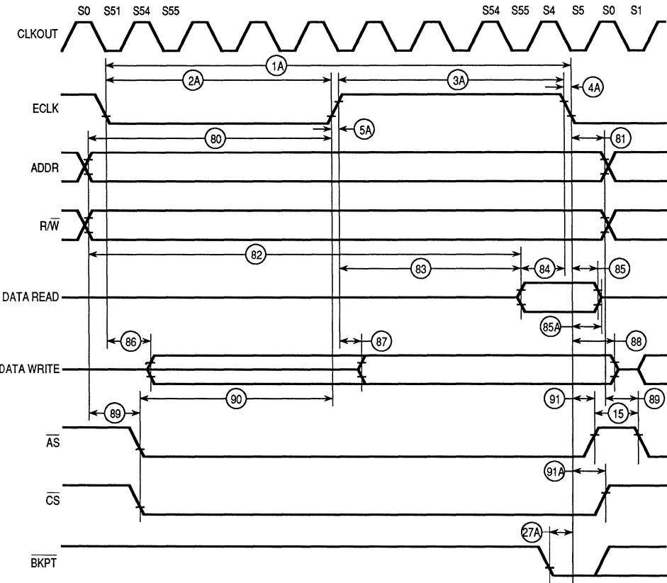
NOTE: All timing is shown with respect to 20% and 70%  $V_{DD}$ .
