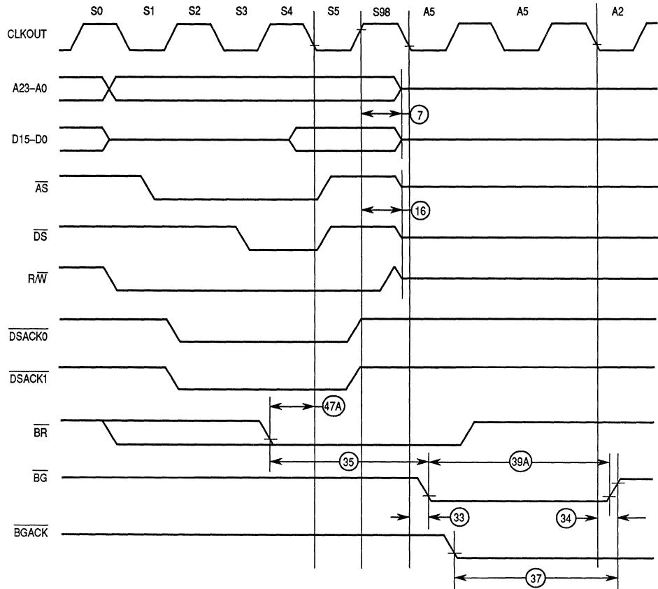
NOTE: All timing with respect to 20% and 70% V<sub>DD</sub>
