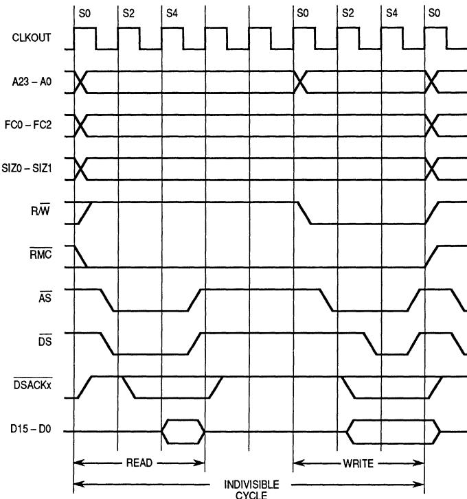
Figure 3-16. Read-Modify-Write Cycle Timing
