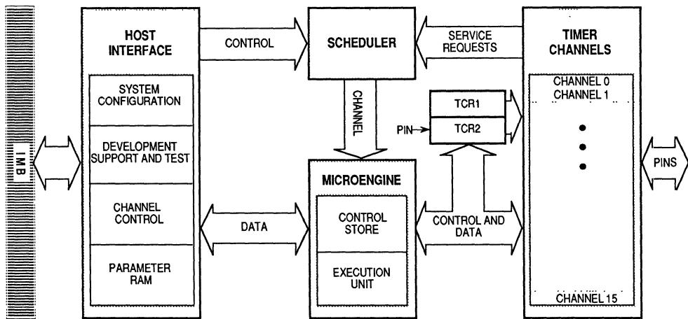
**Figure 8-1. TPU Simplified Block Diagram**
