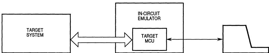
**Figure 7-10. Traditional In-Circuit Emulator Diagram**
