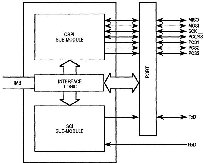
**Figure 5-1. QSM Block Diagram**
