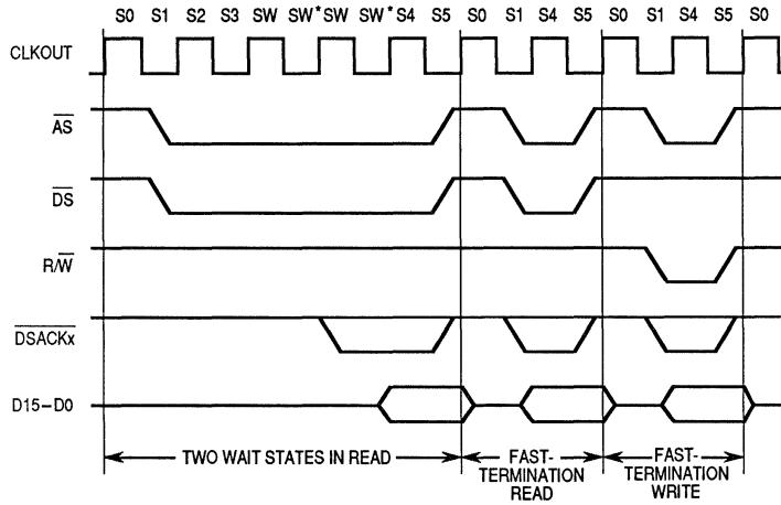
\* DSACK<sub>x</sub> only internally asserted for fast-termination cycles
