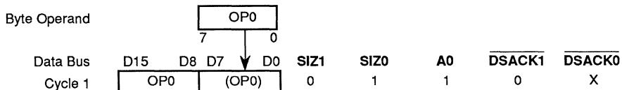
**Figure 3-5. Byte Operand to 16-Bit Port, Odd (A0 = 1)**
