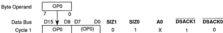
Figure 3-3. Byte Operand to 8-Bit Port, Even (A0 = 0)
