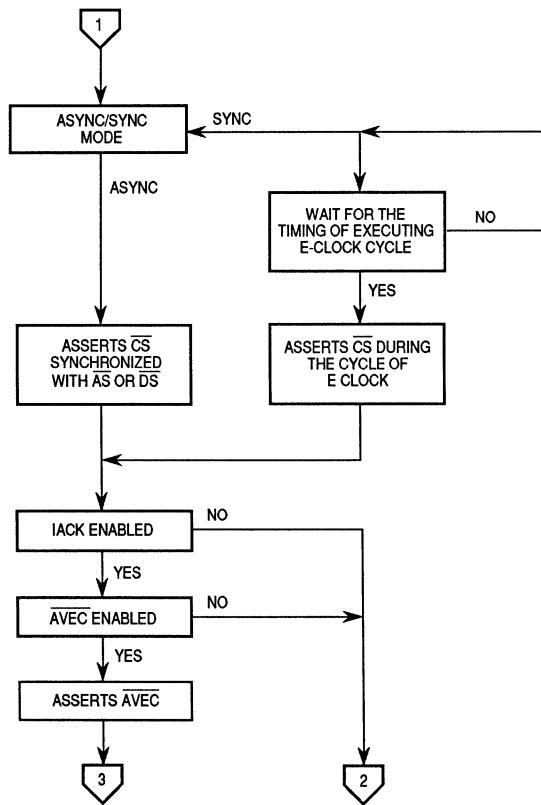
Figure 4-15. Flow Diagram for Chip Select (Sheet 2 of 3)
