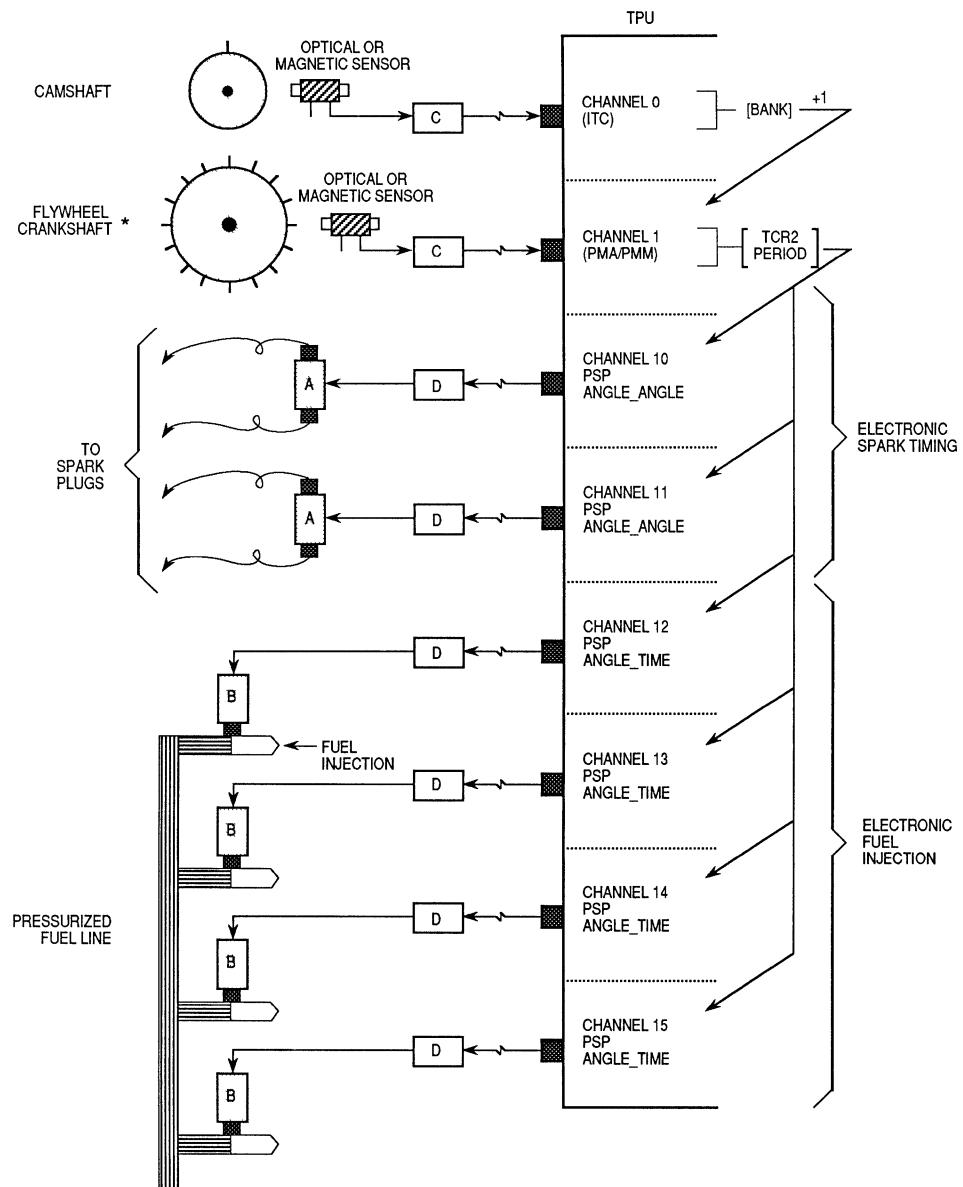
\* Flywheel crankshaft will have either a missing tooth or an additional tooth.
