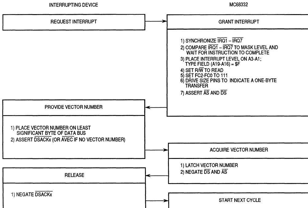
**Figure 3-22. Interrupt Acknowledge Cycle Flowchart**
