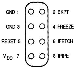
**Figure 9.4. Berg Connector Pinout**
