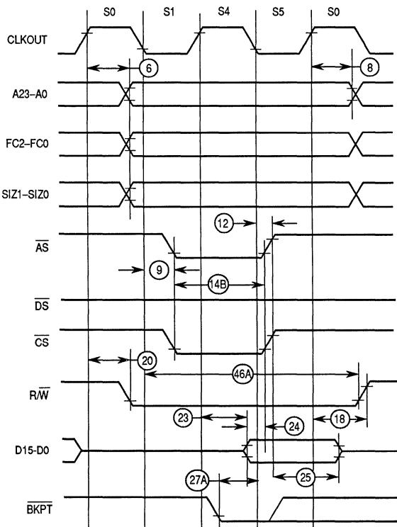
NOTE: All timing with respect to 20% and 70% V<sub>DD</sub>
