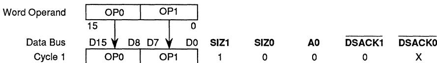
Figure 3-7. Word Operand to 16-Bit Port, Aligned
