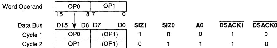
Figure 3-6. Word Operand to 8-Bit Port, Aligned
