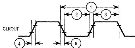
NOTE: All timing shown with respect to 20% and 70%  $V_{DD}$
