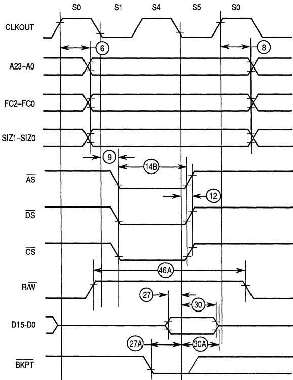
NOTE: All timing with respect to 20% and 70% V<sub>DD</sub>
