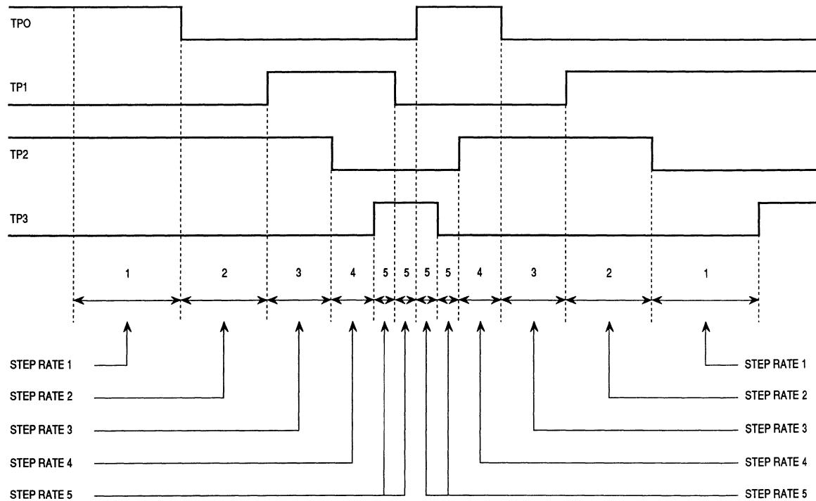
**Figure 8-10. Half-Stepping Waveforms, Counterclockwise Rotation**
