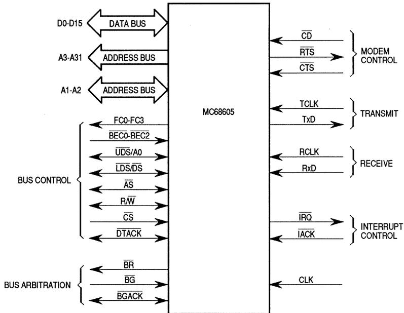
**Figure 7-1. Input and Output Signals**
