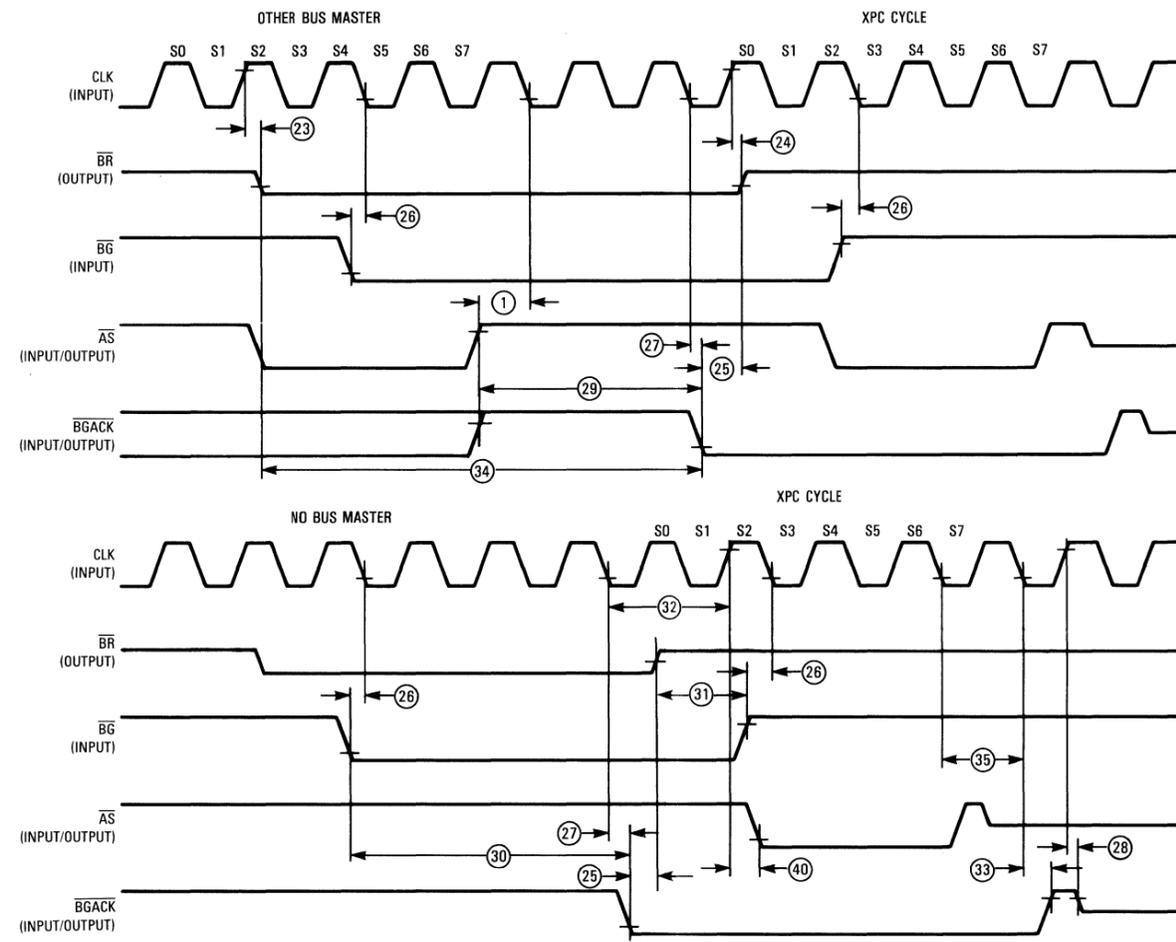
Figure 10-4. Bus Arbitration Timing Diagram
