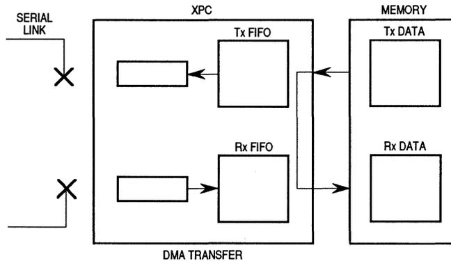
**Figure 6-1. DMA Configuration**
