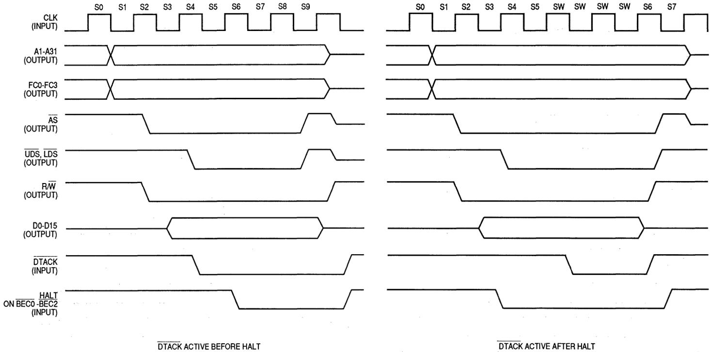
Figure 8-7. Write Cycle with Halt
