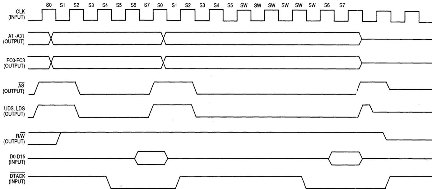
Figure 8-4. Read Cycle and Slow Read Cycle
