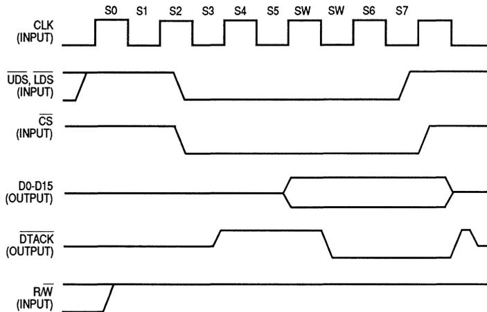
**Figure 8-1. Host Processor Read Cycle**
