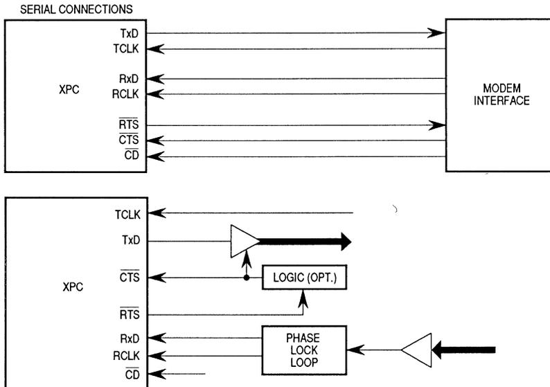
**Figure 9-3. Serial Interface Examples**
