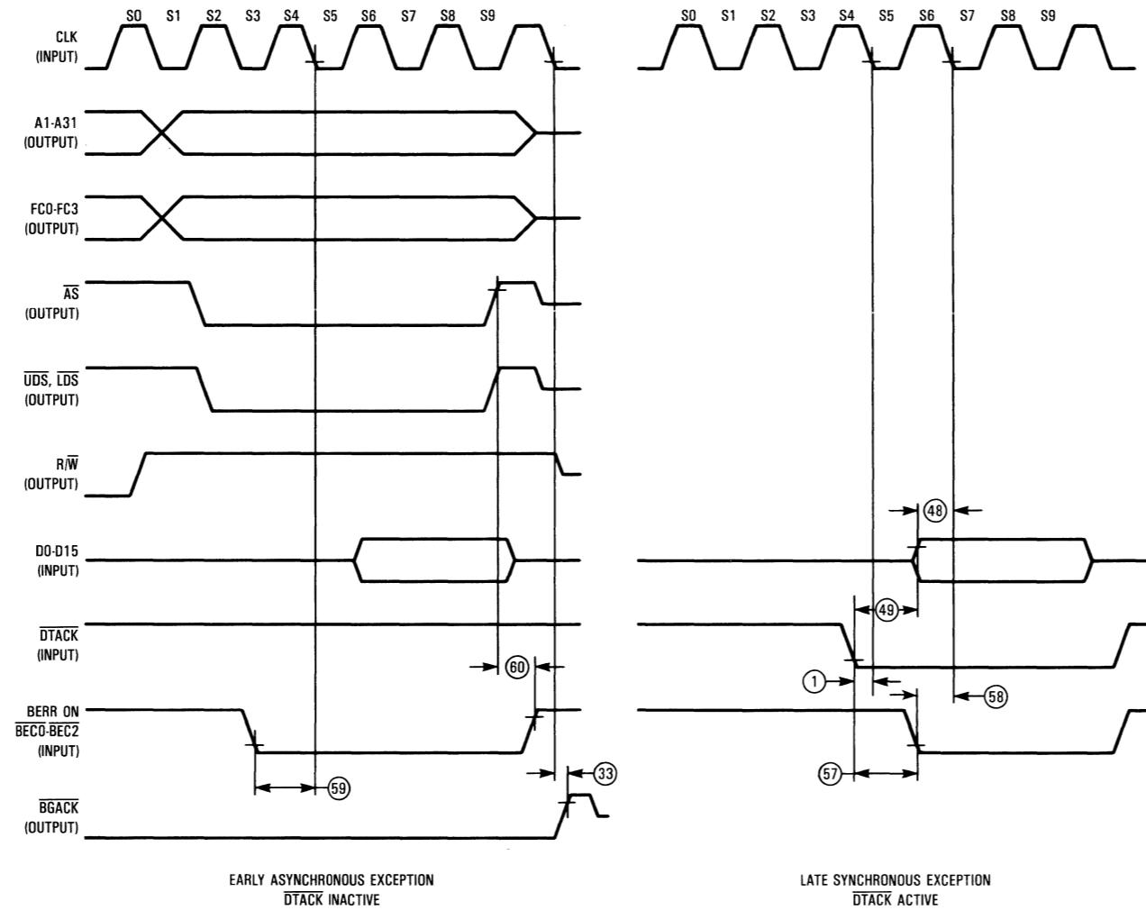
Figure 10-8. Read Cycle with Bus Error Timing Diagram
