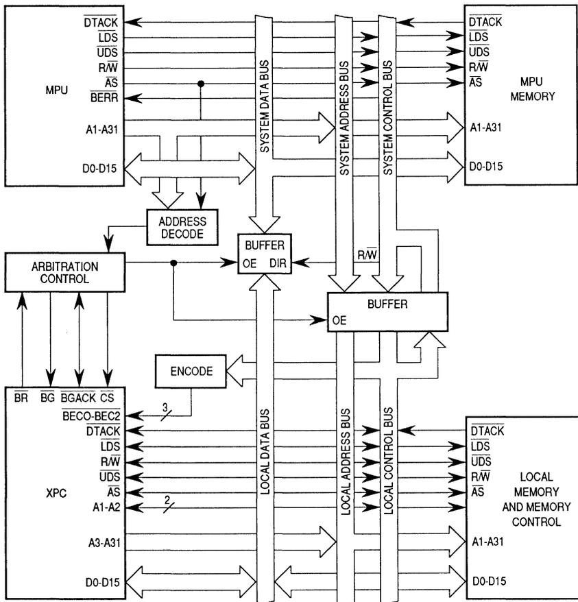
Figure 9-1. XPC-to-Host-Processor Interface
