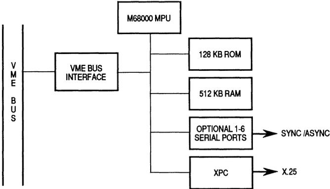
Figure 1-1. XPC System Configuration
