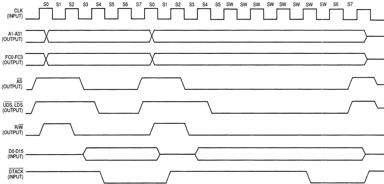
Figure 8-5. Write Cycle and Slow Write Cycle
