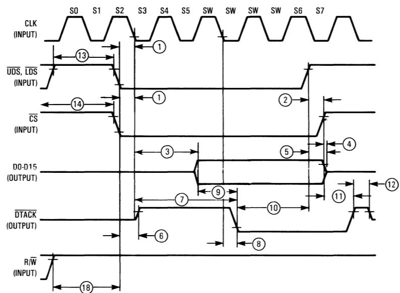
Figure 10-1. Host Processor Read Cycle Timing Diagram
