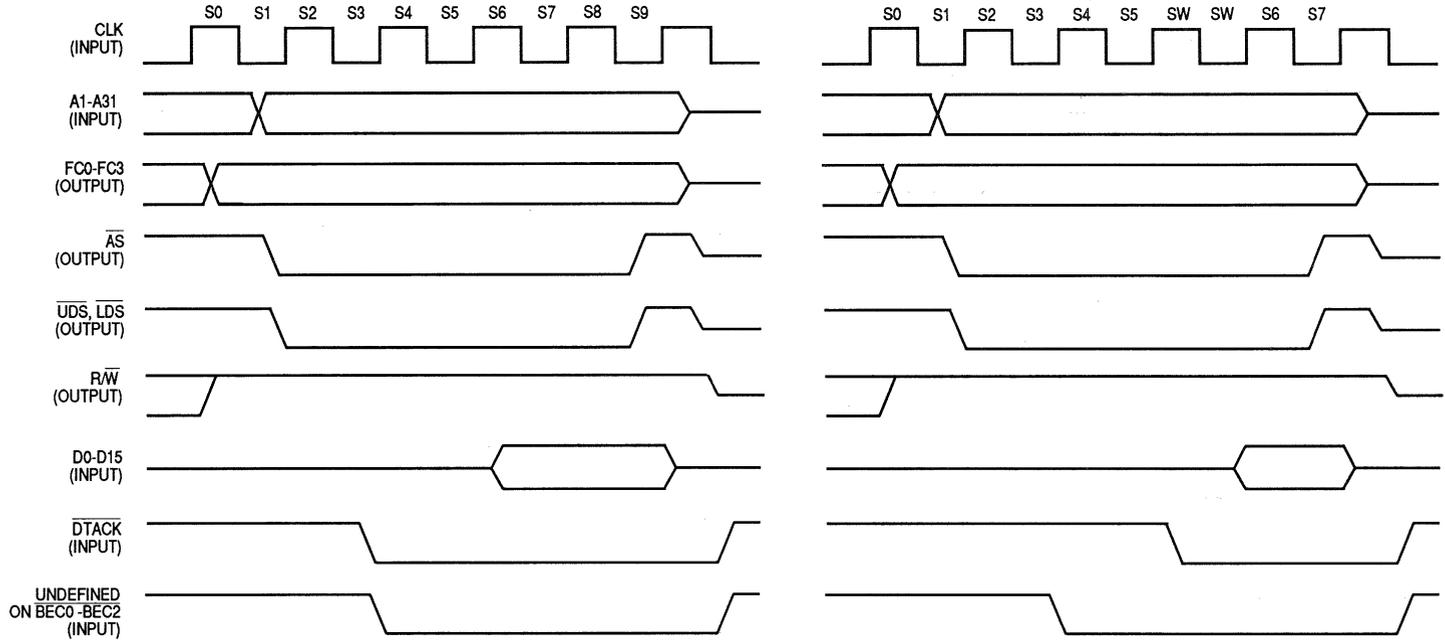
Figure 8-12. Read Cycle with Undefined  $\overline{\text{BEC0}}-\overline{\text{BEC2}}$
