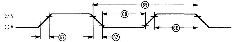
Figure 10-11. Clock (CLK) Timing Diagram
