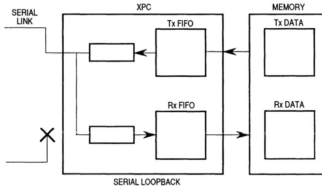
**Figure 6-2. Serial Loopback Configuration**
