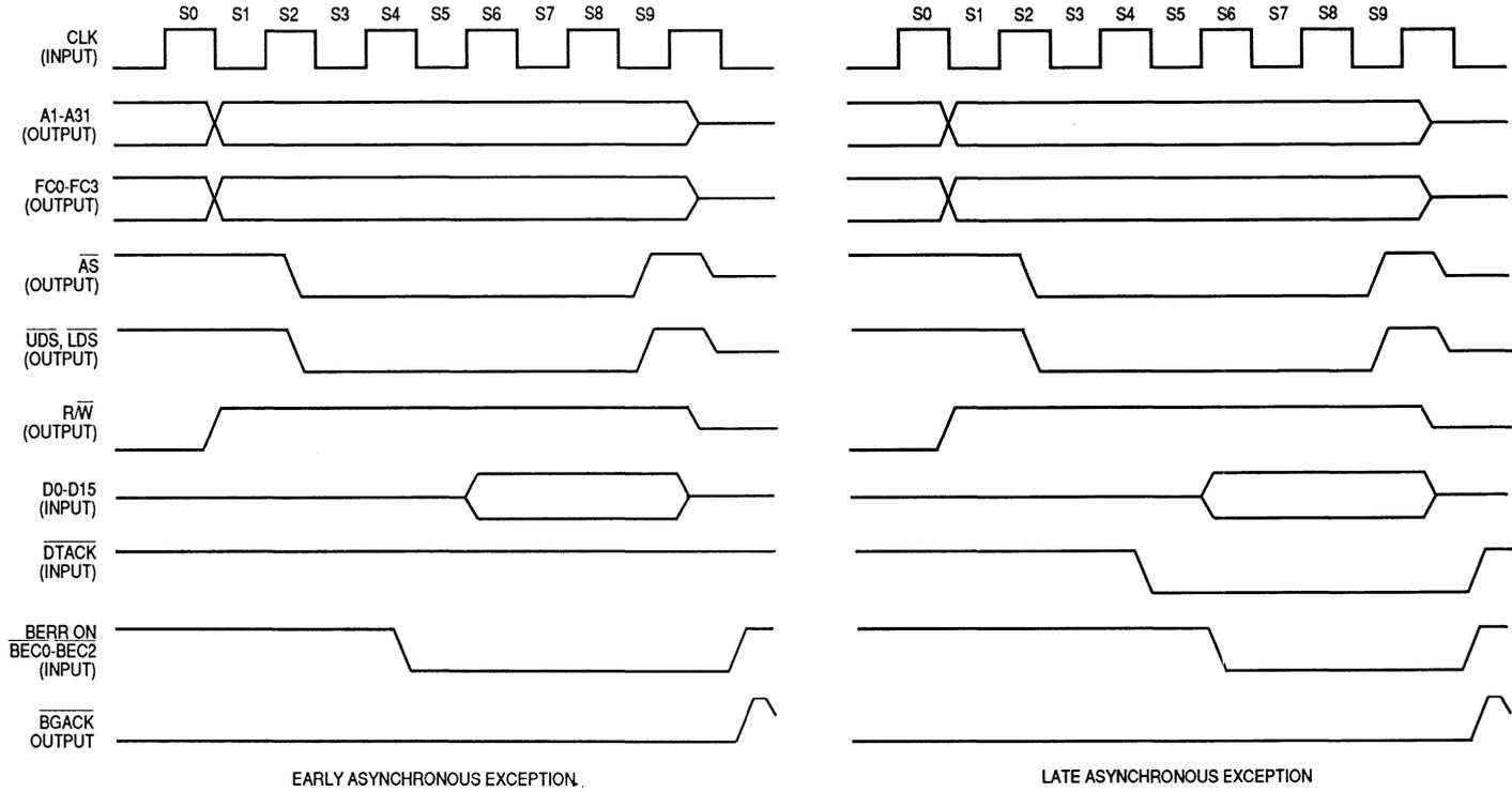
Figure 8-8. Read Cycle with Bus Error
