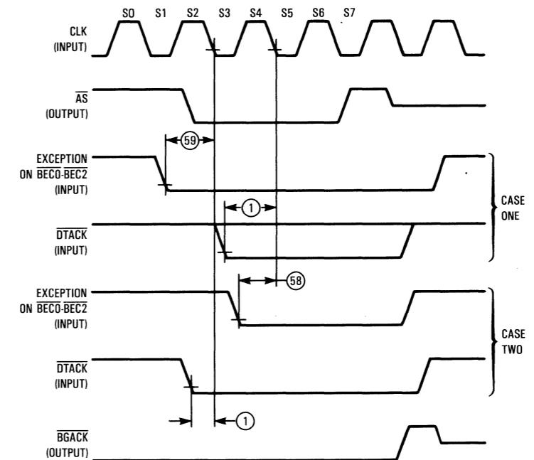
Two alternatives of  $\overline{DTACK}$  and exception. Case one has  $\overline{DTACK}$  occur after exception and case two has exception occur after  $\overline{DTACK}$ . Note that a HALT cycle can be terminated only by  $\overline{DTACK}$ .
