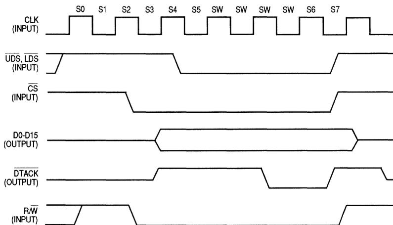
Figure 8-2. Host Processor Write Cycle
