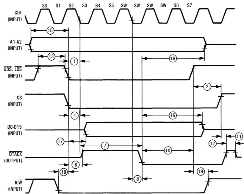
Figure 10-2. Host Processor Write Cycle Timing Diagram
