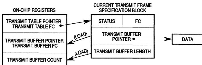
Figure 4-2. Transmit Registers
