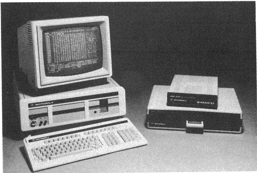
Figure 4.7. VME/10 Central development computer with HDS-200 hardware development station
