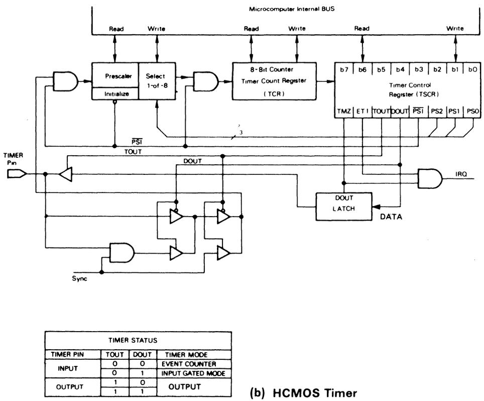
Figure 2.9. M6804 Timer Block Diagrams. Note that HMOS Devices differ from HCMOS
