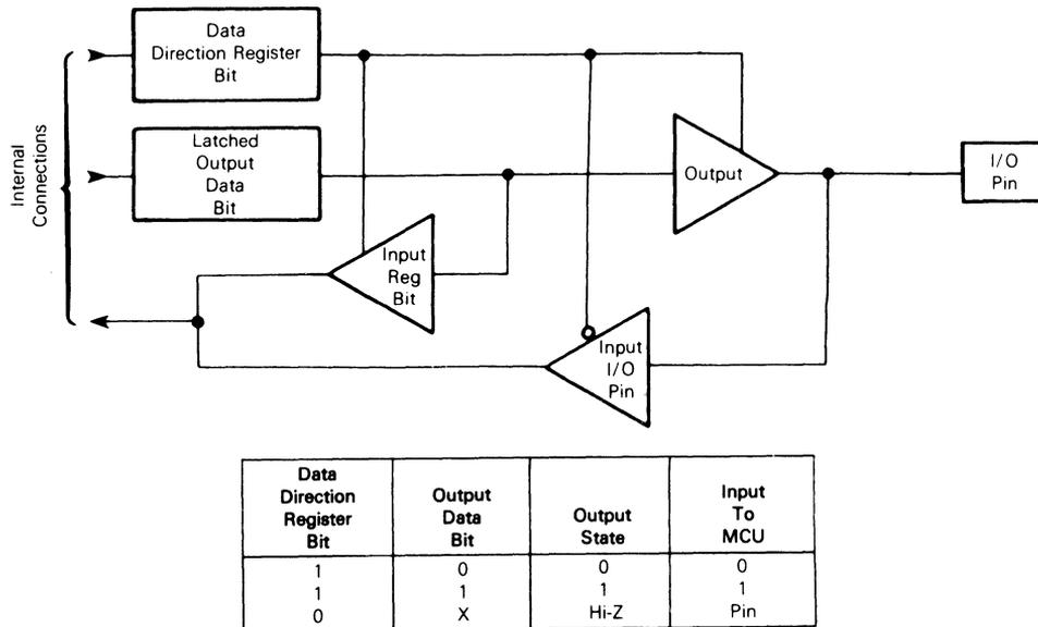
**Figure 2.4. Typical I/O Port Circuitry. The Addresses of Data Direction Registers and I/O Ports are given in the relevant Address Map**
