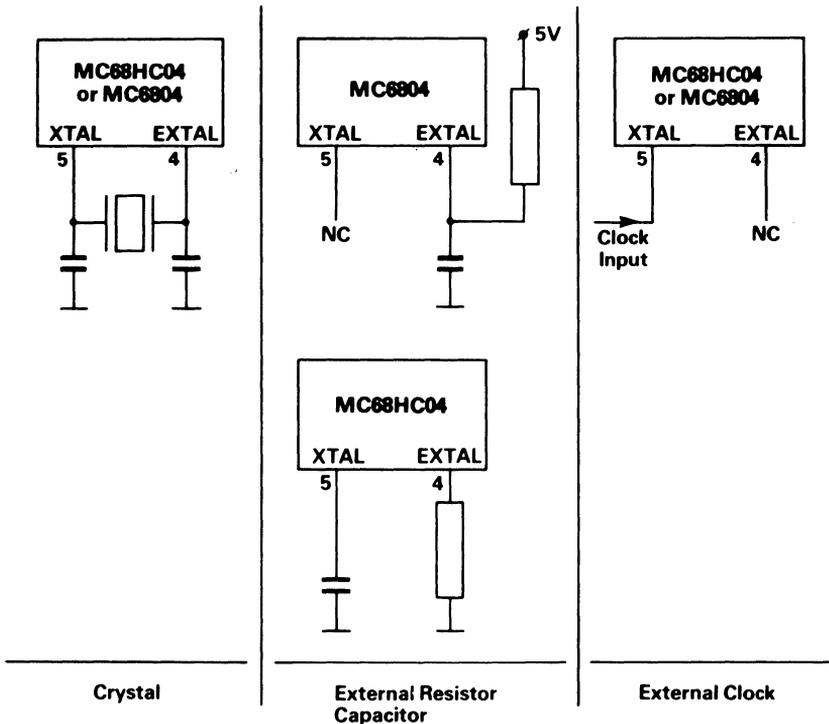
**Figure 2.6. Clock Generator Options of the M6804 Family of MCU's. All options are mask selectable. Note the difference between the External Resistor - Capacitor options for the HMOS and HCMOS versions.**
