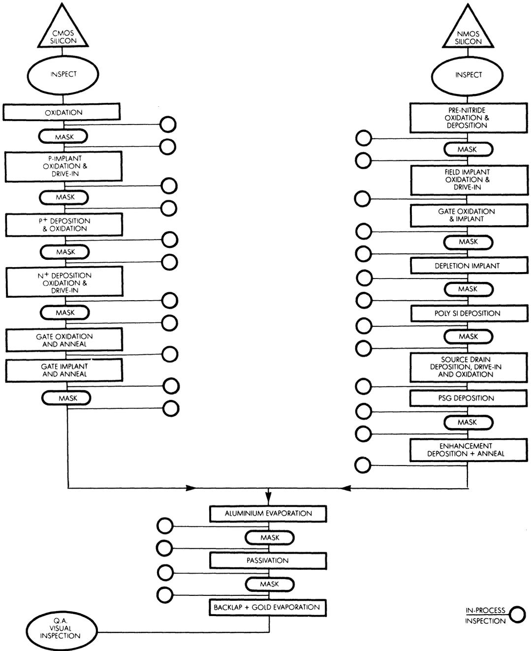
Figure 8.2. MOS Wafer Fabrication Flowchart
