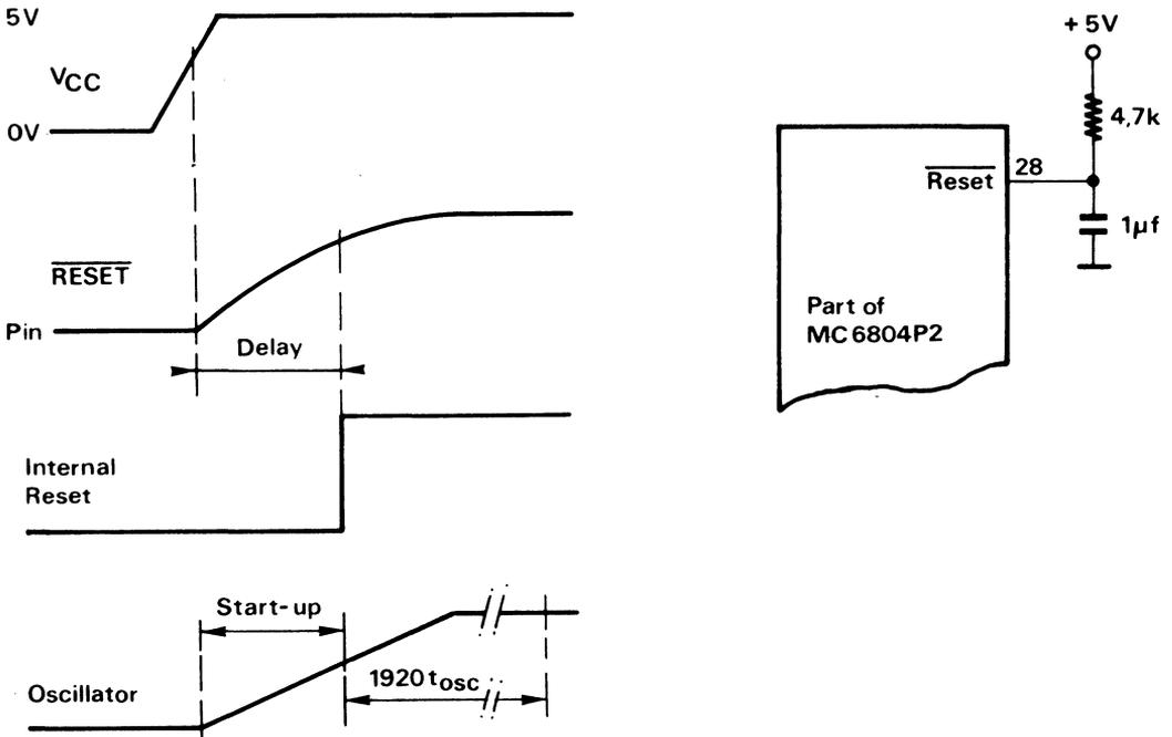
Figure 2.14. Power-on reset delay for MC6804 (MC68HC04 has on-chip power-up detect circuit)
