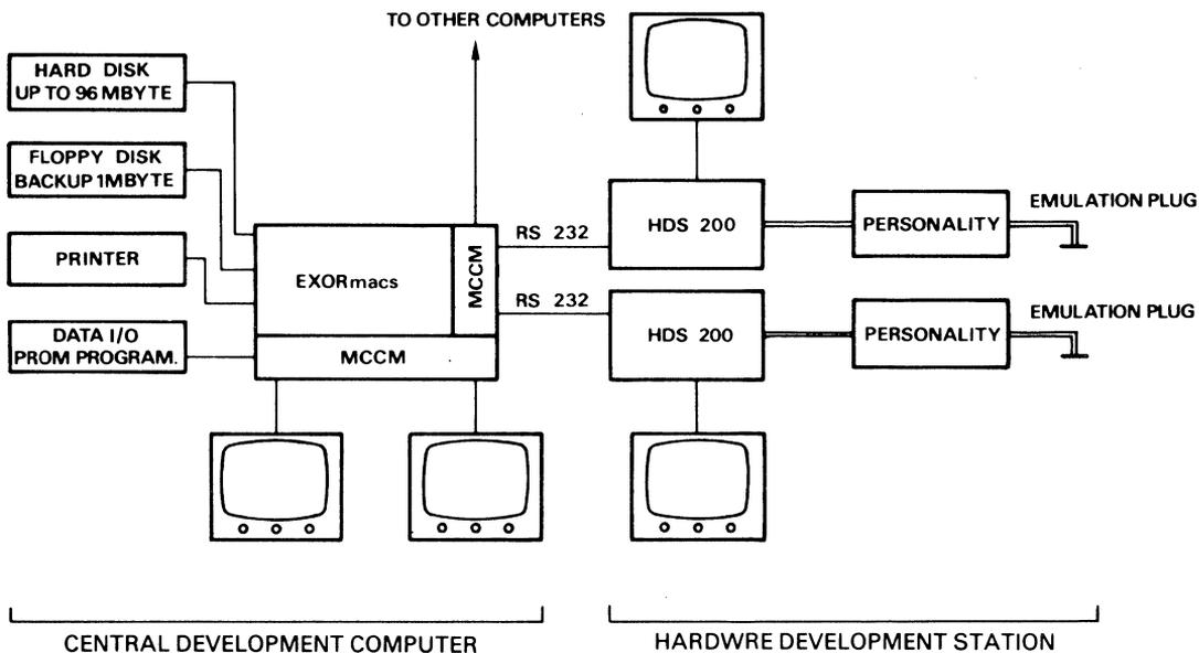
Figure 4.6. Multi-user M6804 development system here: four user EXORmacs configuration
