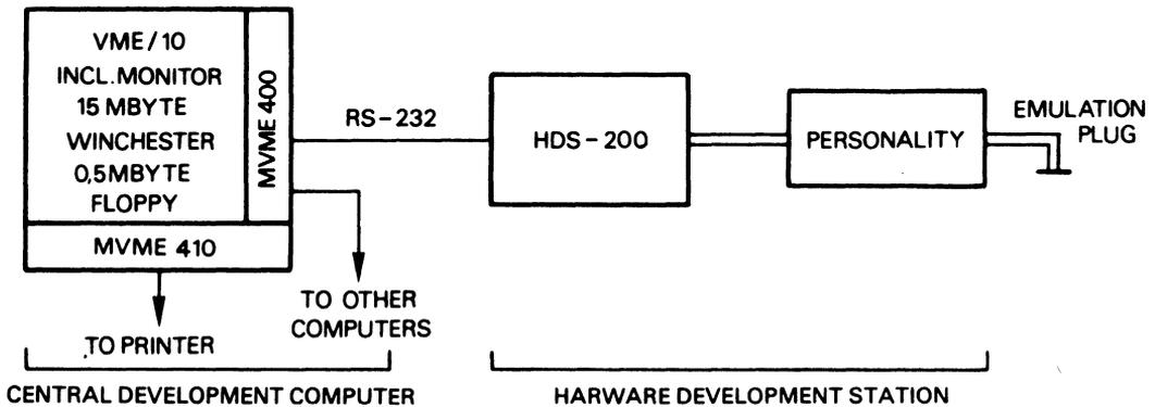
**Figure 4.5. Single-User M6804 Development Workstation Mid-Range Configuration with VME/10**
