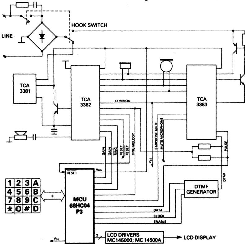
Figure 6.6. Line Powered Feature Telephone
