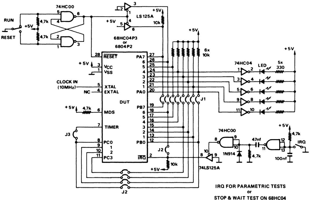
Figure 5.1. Self-Check Circuit
