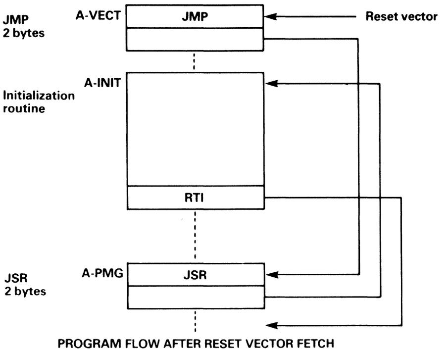
Figure 2.15. Flow Chart of the Initialization of Program after Reset or Power - up
