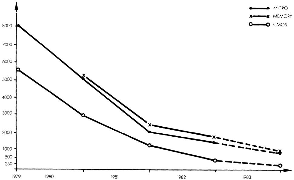
**Figure 8.4. Average Outgoing Quality in PPM for MOS Products Functional/Parametric Failures**
