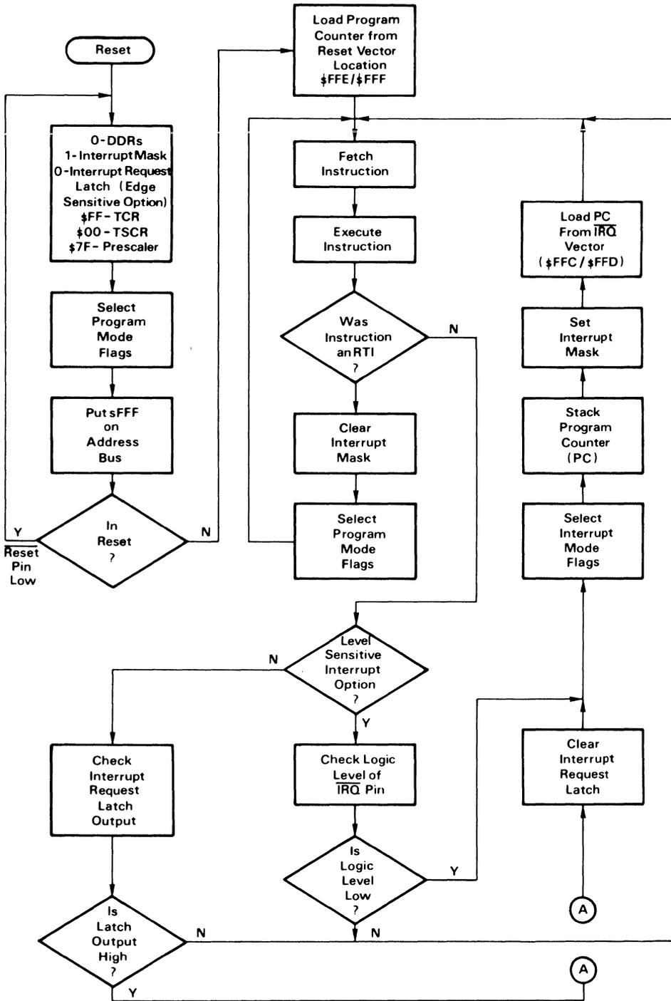
Figure 2.13. Reset and Interrupt Processing Flowchart for the MC6804 (Refer to data sheet for the MC68HC04)
