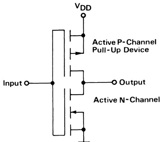
**Figure 1.4. HMOS and HCMOS Inverters**
