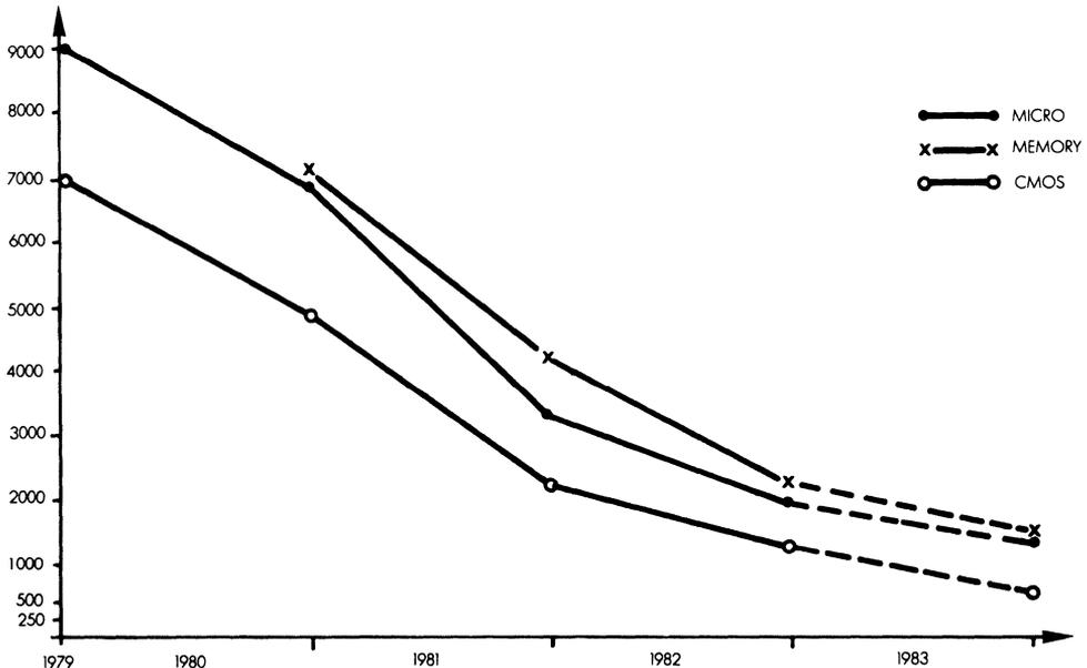
**Figure 8.5. Average Outgoing Quality in PPM for MOS Products Functional/Parametric/Visual/Mechanical Failures**
