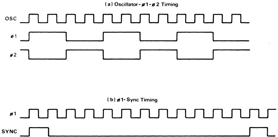
**Figure 2.7. Clock Generator Timing Diagram**
