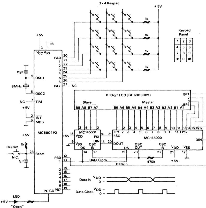
Figure 6.9. Keyboard Encoder/LCD Driver Schematic
