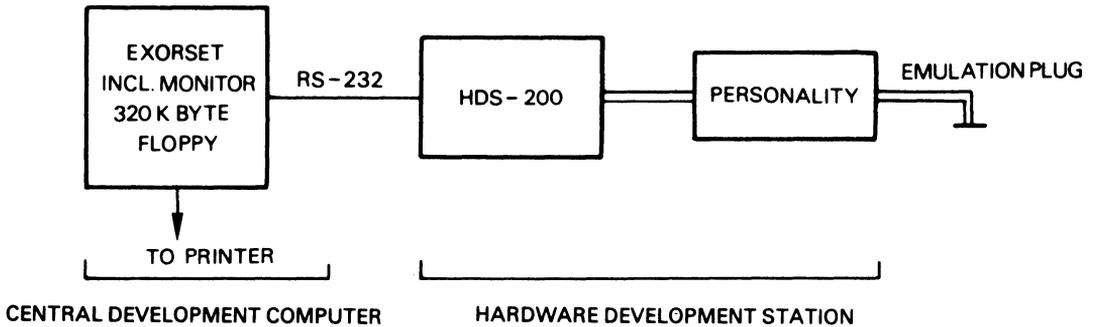
**Figure 4.4. Single-User M6804 Development Workstation Minimum Configuration with EXORset**
