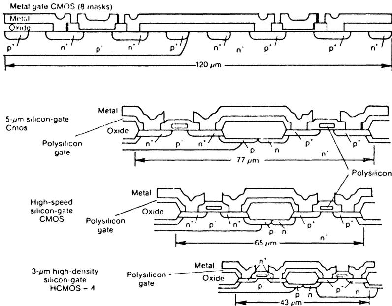
**Figure 1.5. Development of CMOS Technology in the Last Decade**
