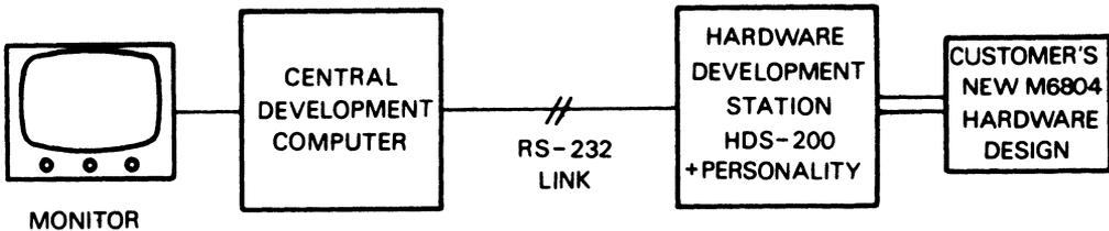
Figure 4.1. General Block Diagram of an M6804 Development Station
