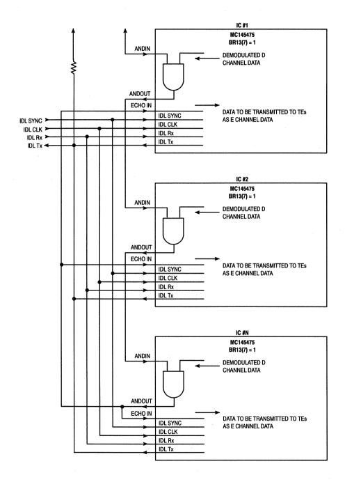
Figure 11-1. NT1 Star Mode of Operation
