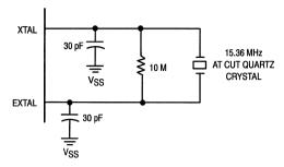
Figure 6-3. Crystal Circuit
