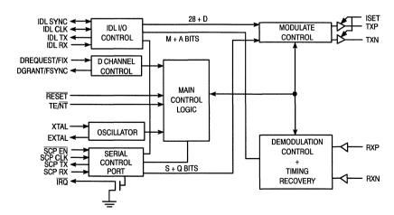
Figure 1-1. MC145474/75 Block Diagram
