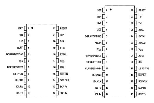
Figure 16-1. MC145474 Pin Assignment
