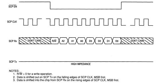
Figure 5-2. Serial Control Port Nibble Write Operation
