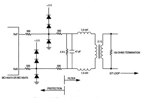
Figure 14-2. Receive Line Interface Circuit
