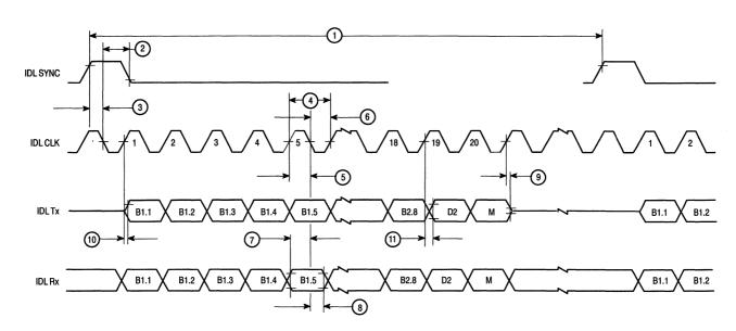
Figure 15-1. IDL Timing Characteristics
