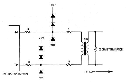
NOTE: 4R + winding resistance = 26.4 ohms.
