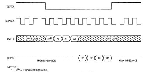
Figure 5-1. Serial Control Port Nibble Read Operation
