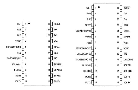
Figure 6-1. MC145474 Pin Assignment
