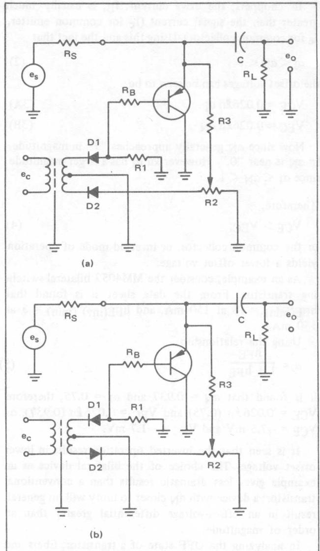
FIGURE 8 — Shunt Chopper Circuits with Offset Voltage Compensation
