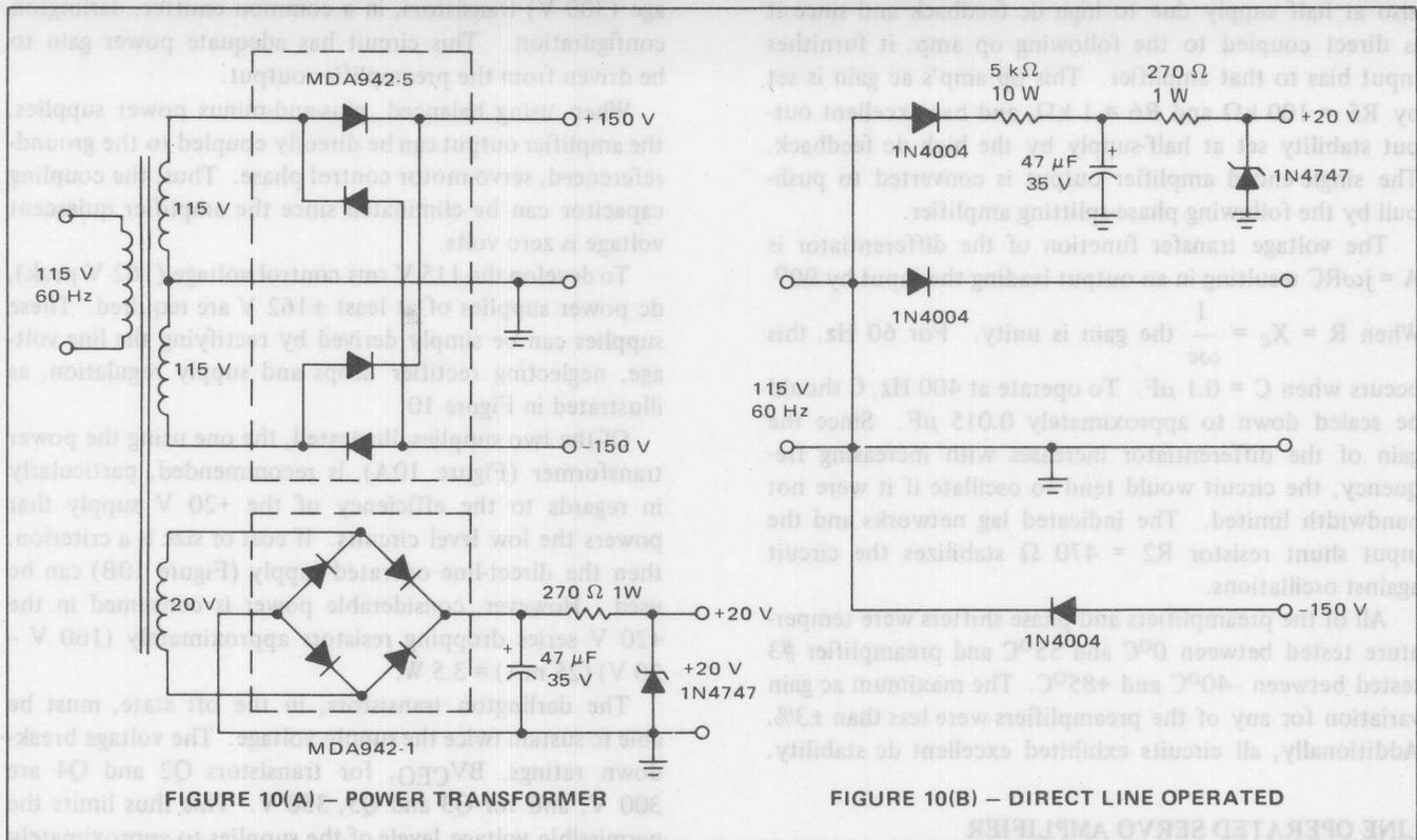
FIGURE 10(A) - POWER TRANSFORMER
