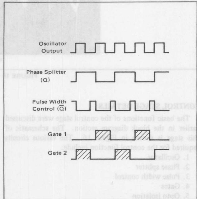
Figure 17 — Timing Diagram
