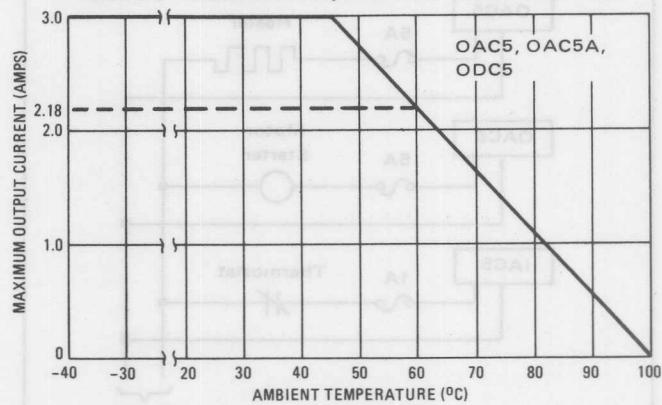
Since the input modules are not power-handling devices, they do not have a derating factor and may be used over the specified temperature range without derating.
