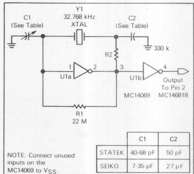
FIGURE 1 — 32.768 kHz Square Wave Oscillator Schematic Diagram
