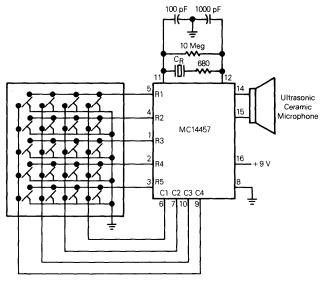
Note:  $C_{\mbox{\scriptsize R}}$  is a ceramic resonator, Radio Materials Corp. type CR30 or equivalent.
