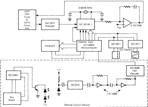
FIGURE 9 - TWO-LOOP SYNTHESIZER PROVIDES 25 AND 100 Hz FREQUENCY STEPS WHILE MAINTAINING HIGH DETECTOR COMPARISON FREQUENCIES OF 10 AND 10.1 kHz
