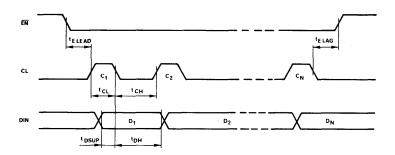
FIGURE 3b - SERIAL INPUT, NEGATIVE CLOCK
