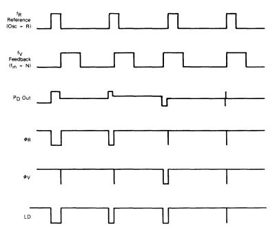
NOTE: The PD output state is approximately equal to either VDD or VSS when active. When not active, the output is high impedance and the voltage at that pin is determined by the low pass filter capacitor.
