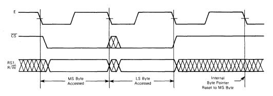
b - Typical 8-Bit ADC Access
