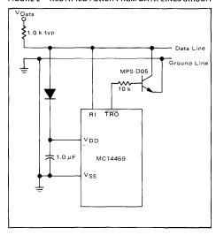
FIGURE 3 – A-D CONVERTER INTERFACE
