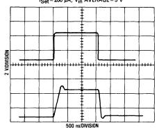
SMALL SIGNAL TRANSIENT RESPONSE VDD = 10 V NON-INVERTING UNITY GAIN
