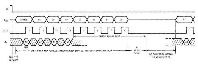
Figure 10. MC145040 Timing Diagram
