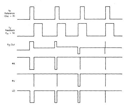
NOTE: The PD output state is equal to either VDD or VSS when active. When not active, the output is high impedance and the voltage at that pin is determined by the low pass filter capacitor.
