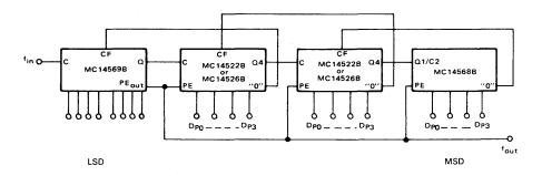
FIGURE 7 — FREQUENCY SYNTHESIZER WITH MC14568B and MC14569B USING A MIXER (Channel Spacing 10 kHz)
