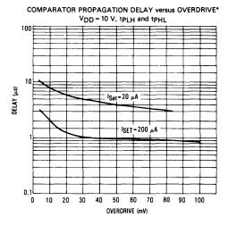
$^{\circ}$ A 10 mV overdrive is a signal on one input of a comparator that ranges from 10 mV less than the other input to 10 mV more than the other input.
