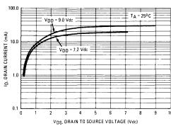
FIGURE 2 — TYPICAL COMPARATOR OUTPUT I-V CHARACTERISTIC
