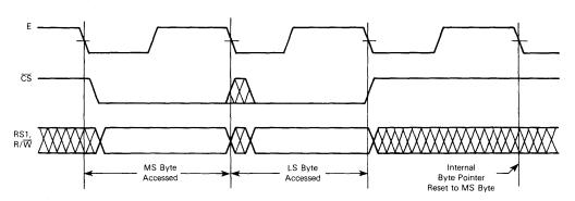
b - Typical 8-Bit ADC Access
