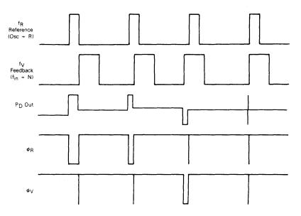
NOTE: The PD output state is equal to either VDD or VSS when active. When not active, the output is high impedance and the voltage at that pin is determined by the low pass filter capacitor.
