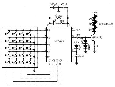
Note:  $C_{\mbox{\scriptsize R}}$  is a ceramic resonator, Radio Materials Corp. type CR30 or equivalent.
