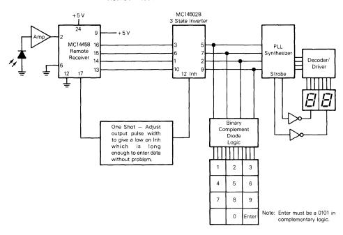
FIGURE 7 — BLOCK DIAGRAM OF A TUNING ADDRESS SYSTEM FOR UP TO 256 CHANNELS
