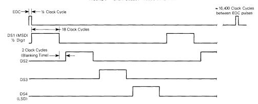
FIGURE 9 - INTEGRATOR WAVEFORMS AT PIN 6
