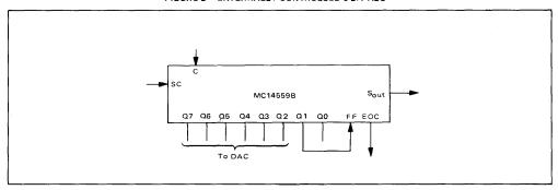
FIGURE 3 - CONTINUOUSLY CYCLING 8-BIT ADC
