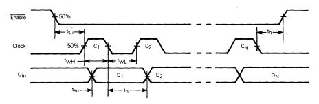
FIGURE 4 - SERIAL INPUT, NEGATIVE CLOCK
