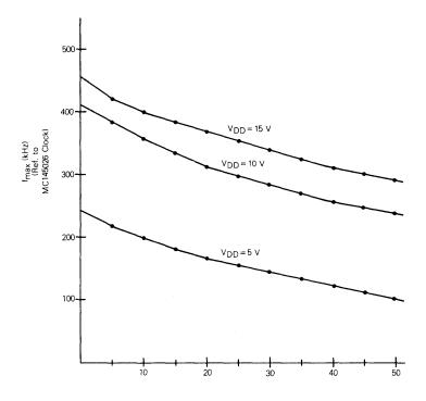
$C_{\mbox{\scriptsize layout}}$  (pF) on Pins 1-5 (MC145027); Pins 1-5 and 12-15 (MC145028); Pins 1-4 (MC145029)
