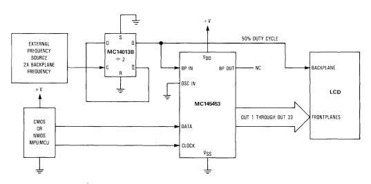
Figure 4. Converting External Backplane Frequency Source to 50% Duty Cycle
