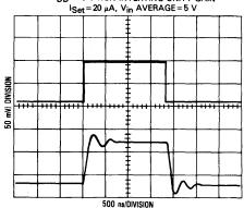
LARGE SIGNAL TRANSIENT RESPONSE V<sub>DD</sub> = 10 V NON-INVERTING UNITY GAIN
