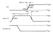
d. Pulse Width: Data DCBA strobed into latches.
