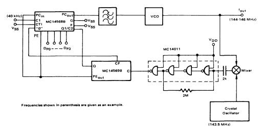
FIGURE 8 - FREQUENCY SYNTHES[ZER USING MC14568B, MC14569B AND MC14522B (Without Mixer)
