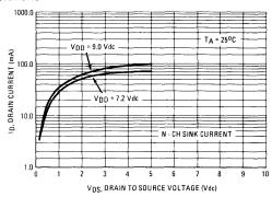
FIGURE 5 — TYPICAL COMPARATOR OUTPUT I-V CHARACTERISTIC
