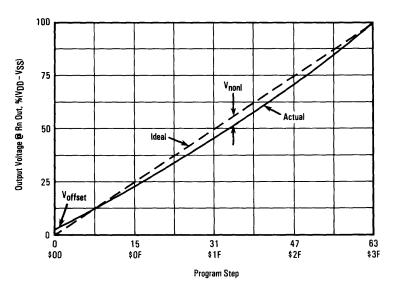
LINEARITY ERROR (integral linearity). A measure of how straight a device's transfer function is, it indicates the worst-case deviation of linearity of the actual transfer function from the best-fit straight line. It is normally specified in parts of an LSB.
