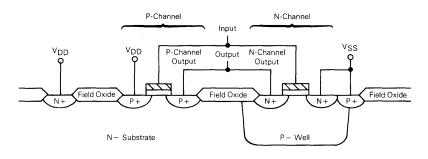
FIGURE 4 - LATCH UP CIRCUIT SCHEMATIC
