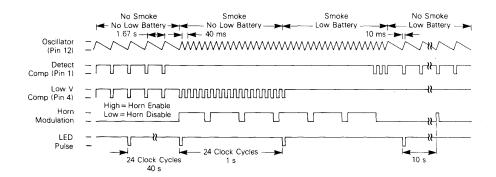
NOTES: 1. Horn modulation is self-completing. When going from smoke to no smoke, the alarm condition will terminate only when horn is off.
