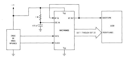
Figure 3. Using On-Chip Oscillator
