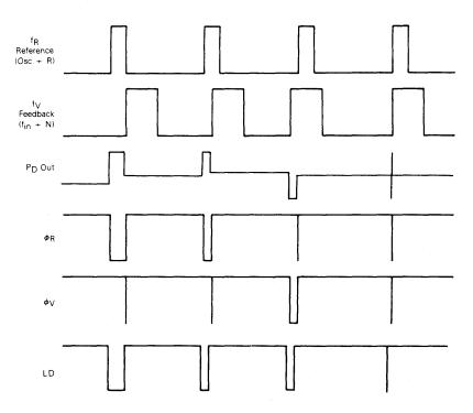
NOTE: The P<sub>D</sub> output state is equal to either V<sub>DD</sub> or V<sub>SS</sub> when active. When not active, the output is high impedance and the voltage at that pin is determined by the low pass filter capacitor.
