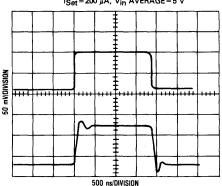
LARGE SIGNAL TRANSIENT RESPONSE V<sub>DD</sub> = 10 V NON-INVERTING UNITY GAIN ISet = 200 µA, Vin AVERAGE = 5 V
