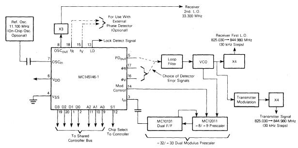
NOTES: 1) Receiver 1st. I.F. = 45 MHz, low side injection; Receiver 2nd. I.F. = 11.7 MHz, low side injection.
