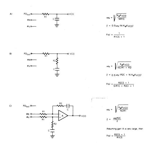
NOTE: Sometimes R1 is split into two series resistors each R1 + 2. A capacitor  $C_C$  is then placed from the midpoint to ground to further filter  $\phi_V$  and  $\phi_R$ . The value for  $C_C$  should be such that the corner frequency of this network does not significantly affect  $\omega_N$
