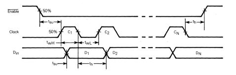
FIGURE 4 - SERIAL INPUT, NEGATIVE CLOCK
