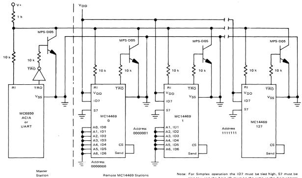
FIGURE 4 – SINGLE LINE, SIMPLEX DATA TRANSMISSION
