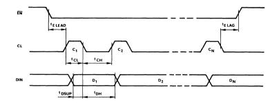
FIGURE 3b - SERIAL INPUT, NEGATIVE CLOCK
