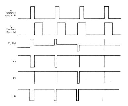
FIGURE 8 PHASE DETECTOR OUTPUT WAVEFORMS
