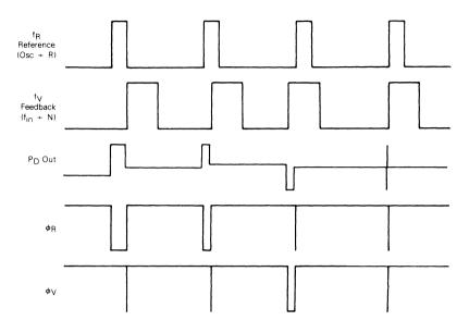
FIGURE 5 PHASE DETECTOR OUTPUT WAVEFORMS
