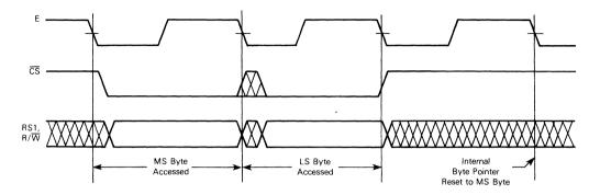
b - Typical 8-Bit ADC Access
