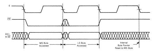
b - Typical 8-Bit ADC Access
