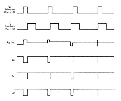
FIGURE 9 PHASE DETECTOR OUTPUT WAVEFORMS
