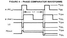
If the input signals have different frequencies, the output signal will be high when signal B has a lower frequency than signal A, and low otherwise.
