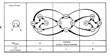
FIGURE 5 – PHASE COMPARATOR STATE DIAGRAM If used in cascade with the programmable divide-by-N counter, practically all usual reference frequencies, or channel spacings of 25, 20, 12.5, 10, 6.25 kHz, etc. are easily achievable.
