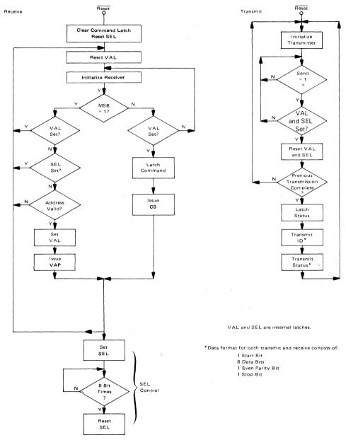
FIGURE 6 - FLOW CHART OF MC14469 OPERATION
