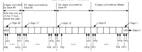
TABLE 2 — THE RELATIONSHIP BETWEEN FRONTPLANE-BACKPLANE INTERSECTIONS AND LCD SEGMENTS FOR THE SYSTEM CONFIGURATION OF FIGURE 7
