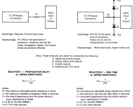
FIGURE 1 - NETWORKS FOR MINIMIZING ESD AND REDUCING CMOS LATCH UP SUSCEPTIBILITY
