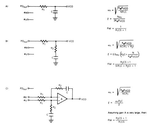
NOTE: Sometimes R<sub>1</sub> is split into two series resistors each R<sub>1</sub>-2. A capacitor C<sub>C</sub> is then placed from the midpoint to ground to further filter  $\phi_V$  and  $\phi_R$ . The value of C<sub>C</sub> should be such that the corner frequency of this network does not significantly affect  $\omega_n$ .
