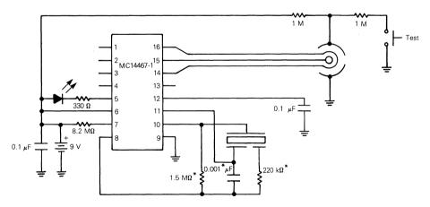
FIGURE 1 - TYPICAL APPLICATION AS IONIZATION SMOKE DETECTOR
