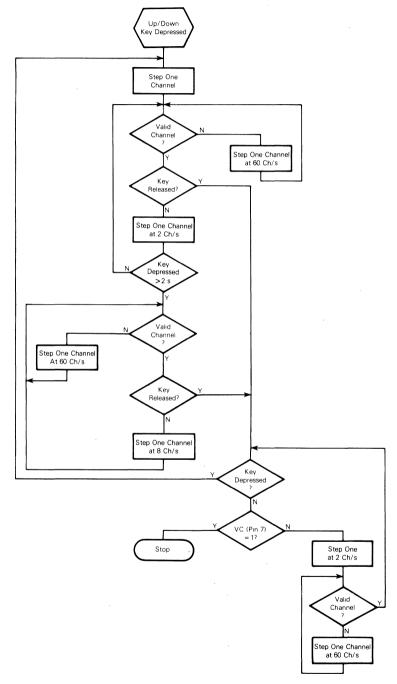
FIGURE 2 - OPERATION OF THE CHANNEL-SCAN CIRCUITRY FOR AC (PIN 14) = 60 Hz
