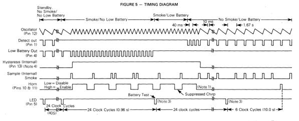
NOTES: 1. Horn modulation is self-completing. When going from smoke to no smoke, the alarm condition will terminate only when horn is off. 2. Comparators are strobed on once per clock cycle (1.67 s for no smoke, 40 ms for smoke).
