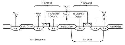
FIGURE 4 - LATCH UP CIRCUIT SCHEMATIC
