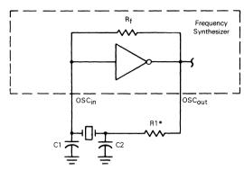
FIGURE A - PIERCE CRYSTAL OSCILLATOR CIRCUIT
