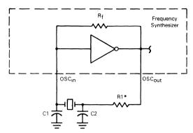
FIGURE A - PIERCE CRYSTAL OSCILLATOR CIRCUIT
