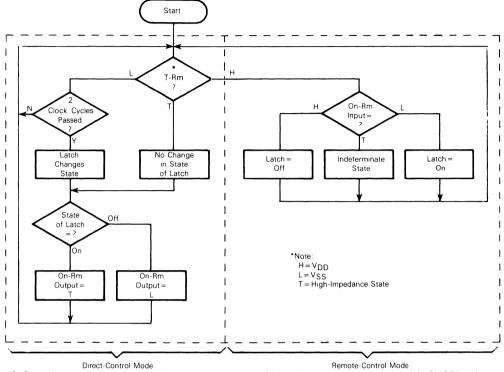
FIGURE 1 - FLOWCHART SHOWING THE RELATIONSHIP OF TMO, ONRM, AND THE STATE OF THE ON/OFF LATCH
