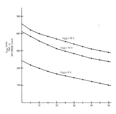
FIGURE 10 — fmax vs Clayout MC145027, MC145028, and MC145029
