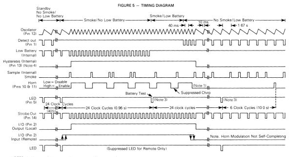
NOTES 1 Horn modulation is self-completing. When going from smoke to no smoke, the alarm condition will terminate only when horn is off
