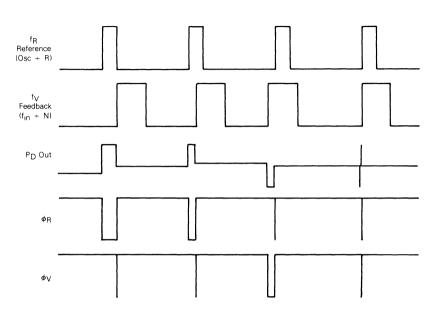
FIGURE 8 PHASE DETECTOR OUTPUT WAVEFORMS
