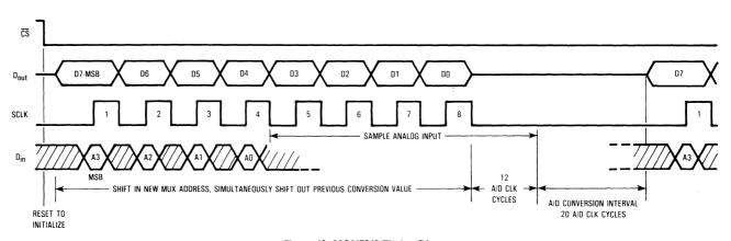
Figure 10. MC145040 Timing Diagram Not Utilizing CS, A/D Conversion Interval Controls Three-State
