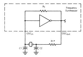
FIGURE A - PIERCE CRYSTAL OSCILLATOR CIRCUIT
