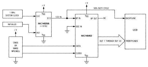
Figure 5. Using Low-Cost Divider to Sync Backplane Frequency
