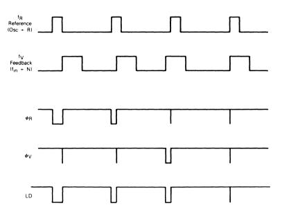
NOTE The PD output state is approximately equal to either VDD or VSS when active. When not active, the output is high impedance and the voltage at that pin is determined by the low pass filter capacitor.
