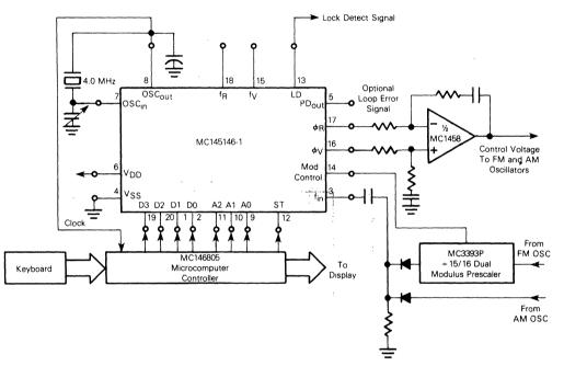
FIGURE 9 - FM/AM BROADCAST RADIO SYNTHESIZER
