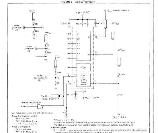
Unused output connected to a 50-ohm resistor to ground
