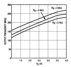
Figure 6. V<sub>C</sub> versus Output Frequency Varying R<sub>X</sub> @ V<sub>CC</sub> = 5.0V; T<sub>A</sub> = 25°C; R<sub>Y</sub> = 1.5k $\Omega$
