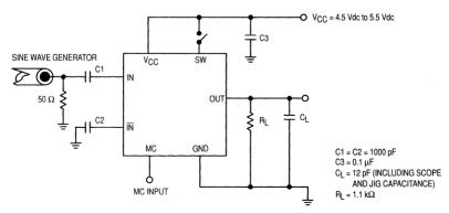
Figure 4A. Input Signal Amplitude versus Input Frequency Divide Ratio = 65
