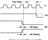
Modulus setup time MC to out is the MC setup or MC release plus the prop delay.
