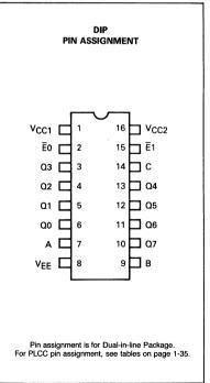
Each MECL 10,000 series circuit has been designed to meet the dc specifications shown in the test table, after thermal equilibrium has been established. The circuit is in a test socket or mounted on a printed circuit board and transverse air flow greater than 500 linear fpm is maintained. Outputs are terminated through a 50-ohm resistor to -2.0 volts. Test procedures are shown for only one input/output combination. Other combinations are tested according to the truth table.
