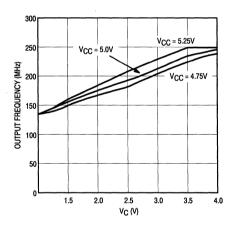
Figure 9. V<sub>C</sub> versus Output Frequency Varying V<sub>CC</sub> @ R<sub>X</sub> = 2.4k $\Omega$ ; R<sub>Y</sub> = 1.5k $\Omega$ ; T<sub>A</sub> = 25°C
