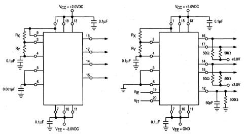
Figure 3. AC Test Circuit (FO/trE/tfE Measurement)
