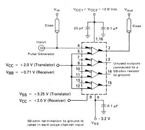
All input and output cables to the scope are equal lengths of 50-ohm coaxial cable. Wire length should be < 1/4 inch from TP $_{\rm In}$  to input pin and TP $_{\rm Out}$  to output pin.
