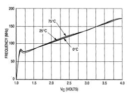
Figure 8. V<sub>C</sub> versus Output Frequency Varying T<sub>A</sub> @ V<sub>CC</sub> = 5.0 V; Rx = 3.3 k $\Omega$ ; Ry = 2.0 k $\Omega$
