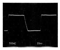
FIGURE 2A  $--\div$  64, 500 MHz, 5.0 V,  $+25^{\circ}$ C, OUTPUT LOADED
