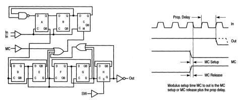
Figure 1. Logic Diagram (MC12033A)
