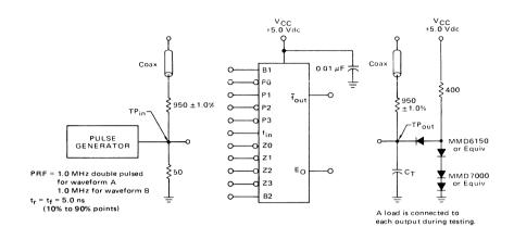
Two pulse generators are required and must be slaved together to provide the waveforms shown.
