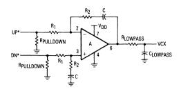
Figure 5-5A. Active Filter Using Op Amp
