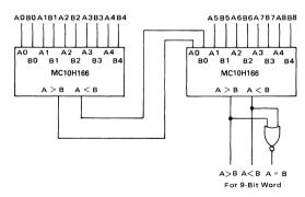
For longer word lengths, the MC10H166 can be serially expanded or cascaded. Figure 1 shows two devices in a serial expansion for a 9-bit word length. The A>B and A<B outputs are fed to the A0 and B0 inputs
