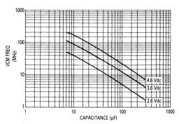
Figure 9-5. VCM Frequency versus Capacitance
