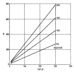
Figure 9-3. One Shot Pulse Width versus Rext/Cext
