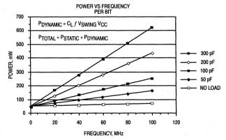
Figure 2. Power versus Frequency (Typical)
