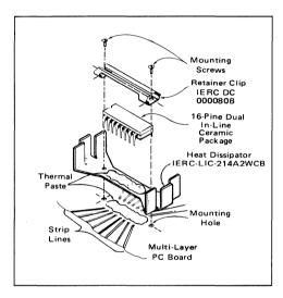
It should be noted that the use of a heatsink on the top surface of the dual-in-line package is not very effective in lowering the  $\bar{\theta}_{\rm JA}$ . This is due to the location of the die near the bottom surface of the package. Also, very little (< 10%) of the internal heat is withdrawn through the package leads due to the isolation from the ceramic by the solder glass seals and the limited heat conduction from the die through 1.0 to 1.5 mil aluminum bonding wires.
