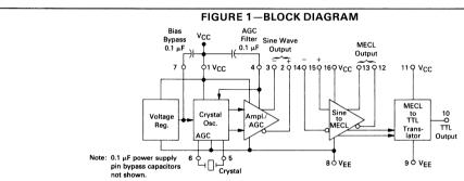
TYPICAL CIRCUIT CONFIGURATIONS Note: 0.1 μF power supply pin bypass capacitors not shown.
