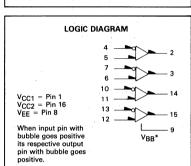
\*V<sub>BB</sub> to be used to supply bias to the MC10H115 only and bypassed (when used) with 0.01  $\mu$ F to 0.1 µF capacitor to ground (0 V). VBB can source < 10 mA
