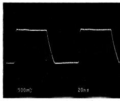
FIGURE 2A - ÷ 64, 500 MHz, 5.0 V, +25°C, OUTPUT LOADED
