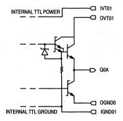
Figure 1. Output Structure
