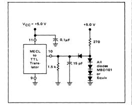
FIGURE 12 — NOISE MEASUREMENT TEST CIRCUIT
