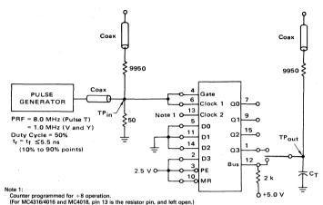
The coax delays from input to scope and output to scope must be matched. The scope must be terminated in 50-ohm impedance. The 9950-50hm resistor and the scope termination impedance constitute a 2001 attenuator probe. Coax shall be CT-070-50 or equivalent.
