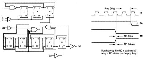
Figure 1. Logic Diagram (MC12031A)
