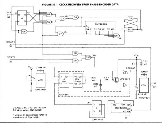
its complement, DGATE, serve to initialize the circuitry and insure that the first transition of the data block (a phase transition) is ignored. The MC7493 binary counter and the G5-G12 latch generate a suitable signal for gating out G3 pulses caused by phase transitions at the end of a data cell, such as the one shown dashed in row 6.
