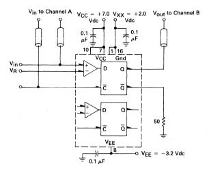
50 ohm termination to ground located in each scope channel input. All input and output cables to the scope are equal lengths of 50 ohm coaxial cable.
