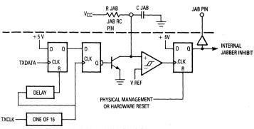
Figure 3-3. Jabber Inhibit Block Diagram
