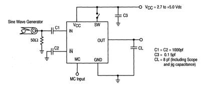
Figure 5. AC Test Circuit
