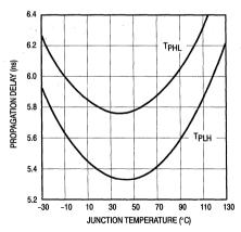
Figure 3. TpD versus Junction Temperature
