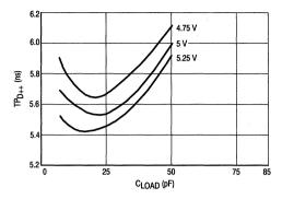
Figure 7. TP versus Load Typical at T<sub>A</sub> = 25°C
