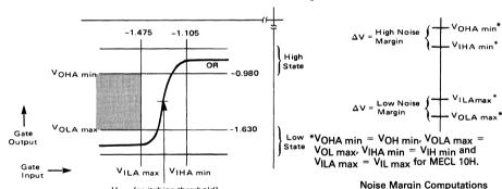
Specification Points for Determining Noise Margin
