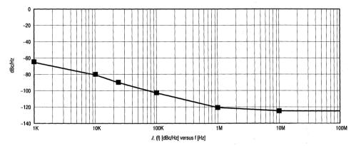
Figure 1. Typical Evaluation Results (CSR MC12148 5.0Vdc; V<sub>CC</sub> @ 25°C; 930MHz CW)
