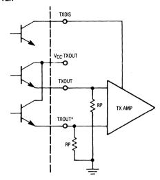
Figure 3-1. Transmitter Outputs
