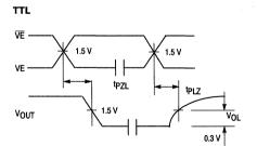
Figure 5. 3-State Output Low Enable and Disable Times
