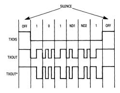
Figure 3-2. Transmit Output Signaling
