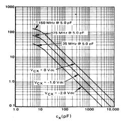
FIGURE 4 — RMS NOISE DEVIATION versus OPERATING FREQUENCY
