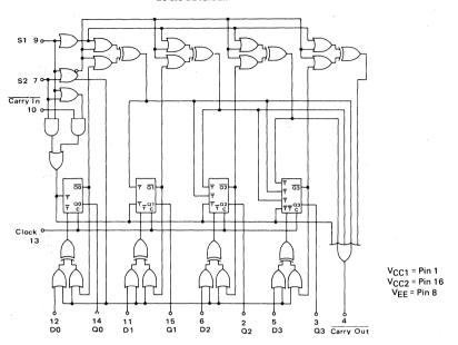
NOTE: FLIP FLOPS WILL TOGGLE WHEN ALL  $\overline{T}$  INPUTS ARE LOW.
