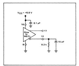
FIGURE 11 — TTL TRANSLATOR LOAD CAPABILITY
