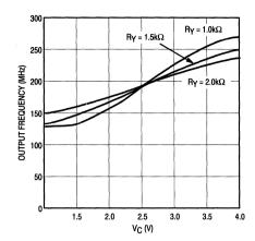
Figure 7. V<sub>C</sub> versus Output Frequency Varying Ry @ V<sub>CC</sub> = 5.0V; T<sub>A</sub> = 25°C; R<sub>X</sub> = 2.4k $\Omega$
