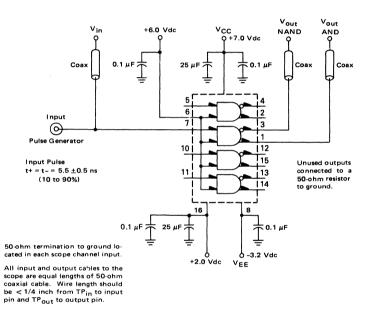
NOTE: All power supply and logic levels are shown shifted 2 volts positive.
