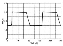
Figure 3. ÷64, 500 MHz, 5.0 V, +25°C, Output Loaded
