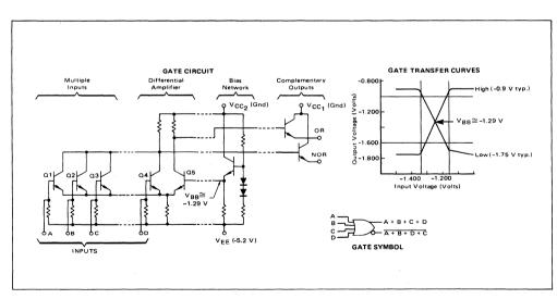
FIGURE 3 — MECL 10K GATE STRUCTURE AND SWITCHING BEHAVIOR
