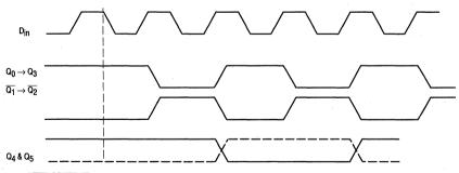
$\frac{\text{AFTER POWER UP}}{\text{OUTPUTS Q}_4 \& \text{Q}_5} \text{ WILL SYN WITH POSITIVE EDGES OF $D_{10}^{} \& \text{Q}_0 \rightarrow \text{Q}_3$ & NEGATIVE EDGES OF $\overline{\text{Q}}_0 \& \overline{\text{Q}}_1$}$
