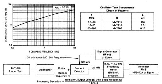
NOTE: Any frequency deviation caused by the signal generator and MC1648 power supply should be determined and minimized prior to testing.
