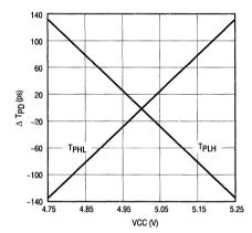
Figure 4. ATpp versus VCC
