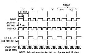
Figure 5-2. Clock Recovery Timing Signals
