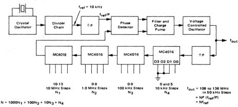
FIGURE 10 — 108 TO 136 MHz FREQUENCY SYNTHESIZER WITH 25 kHz CHANNEL SPACING
