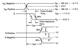
Clock enable time = minimum time between analog and clock signal such that output switches, and tpd (analog to Q) is not degraded by more than 200 ps.
