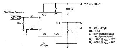
Figure 3. AC Test Circuit
