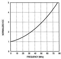
Figure 1. ICC versus f (No Load)
