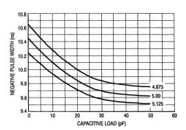
Figure 3. MC10H642 Positive PW versus Load @  $\pm 2.5\%$  V<sub>CC</sub>, T<sub>A</sub> =  $25^{\circ}$ C
