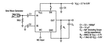
Figure 3. AC Test Circuit
