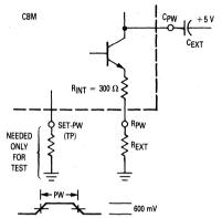
Figure 5-3. One-Shot Timing Components
