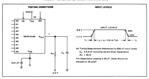
Guaranteed with  $V_{EE}$  = -5.2 Vdc  $\pm$  5.0%,  $T_A$  = 0°C to 75°C (see Note 1). Output Load see Figure 1.
