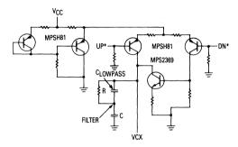
Figure 5-5B. Charge Pump/Filter
