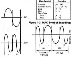
Figure 1-4. Phase-Coherent Modulation Scheme
