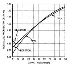
Figure 5. Tpp versus Load
