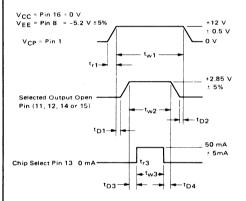
The timing diagram is shown for programming one bit. Note that only one bit is blown at a time. All addressing must be done 100 ns prior to the beginning of the V<sub>CP</sub> pulse, i.e., V<sub>CP</sub> = 0 V. Likewise, strobing of the outputs to determine success in programming should occur no sooner than 100 ns after V<sub>CP</sub> returns to 0 V.
