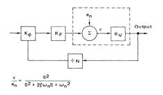
This function has a slope of 12 dB/octave at frequencies less than  $\omega_{\Pi}$  (loop natural frequency), as shown in Figure 24. This means that noise components in the VCO above  $\omega_{\Pi}$  will pass unattenuated and those below will have some degree of suppression. Therefore choice of loop natural frequency may well rest on VCO noise quality.
