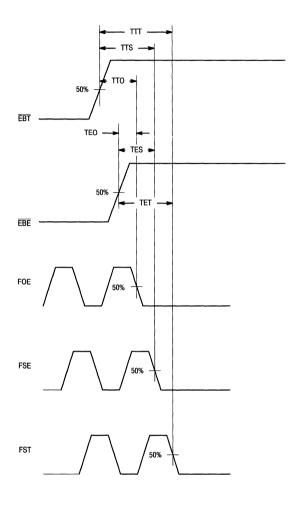
Figure 5. Switching Waveforms
