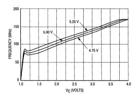
Figure 9. V<sub>C</sub> versus Output Frequency Varying V<sub>CC</sub> @ Rx = 3.3 k $\Omega$ ; Ry = 2.0 k $\Omega$ ; TA = 25°C
