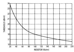
Figure 9-6. Detected Threshold versus Threshold Resistor
