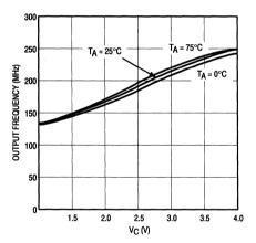
Figure 8. V<sub>C</sub> versus Output Frequency Varying T<sub>A</sub> @ V<sub>CC</sub> = 5.0V; R<sub>X</sub> = 2.4k $\Omega$ ; R<sub>Y</sub> = 1.5k $\Omega$
