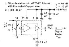
\*The 1200 ohm resistor and the scope termination imped-ance constitute a 25:1 attenuator probe. Coax shall be CT-070-50 or equivalent.
