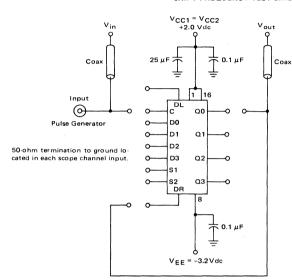
All input and output cables to the scope are equal lengths of 50-ohm coaxial cable. Wire length should be <1/4 inch from TP $_{\rm in}$  to input pin and TP $_{\rm out}$  to output pin.
