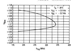
Figure 2 illustrates the variation in toggle frequency with the dc offset voltage ( $V_{\mbox{Bias}}$ ) of the input clock signal.
