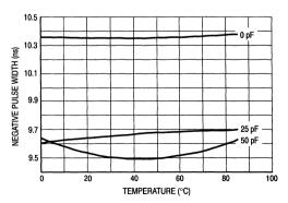
Figure 5. MC10H642 Positive PW versus Temperature, V<sub>CC</sub> = 5.0 V
