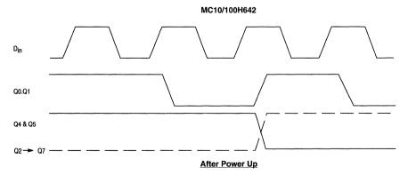
Figure 9. Outputs Q2  $\rightarrow$  Q7 will Synchronize with Pos Edges of D<sub>in</sub> & Q0  $\rightarrow$  Q1
