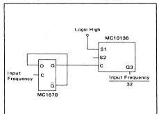
FIGURE 3 — 50 MHz PROGRAMMABLE COUNTER
