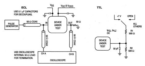
Figure 1. Switching Circuit ECL
