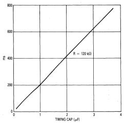
Figure 9-7. Jabber Time Constant versus Capacitance
