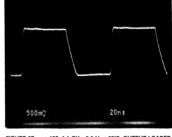
FIGURE 2A — ÷64, 500 MHz, 5.0 V, +25°C, OUTPUT LOADED
