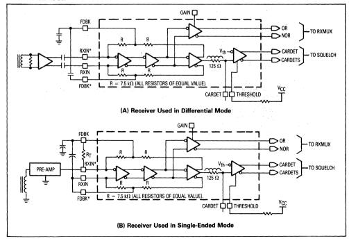
Figure 4-1. Receiver Amplifier With Carrier Detect
