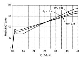
Figure 7. V<sub>C</sub> versus Output Frequency Varying Ry @ V<sub>CC</sub> = 5.0 V;  $T_A$  = 25°C; Ry = 3.3 k $\Omega$
