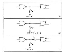
To maintain clean wave fronts, the input impedance of the driven gate must be much greater than the characteristic impedance of the transmission line. This condition is satisfied by MECL circuits which have high impedance inputs. Using the appropriate terminating resistor (Rg) at point A (Figure 24), the reflections in the transmission line will be terminated.
