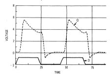
Example 2. In a memory system application, use of an external source resistor is suggested. Simulations run with RS =  $8\Omega$  and CL = 300 pF leads to clean waveforms both at the output, Q, and at point Qp:
