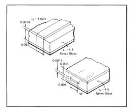
Stripline is used with multilayer circuit boards as shown in Figure 27. Stripline consists of a constant-width conductor between two ground planes.
