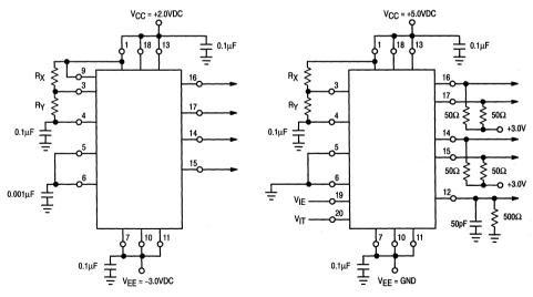
Figure 3. AC Test Circuit (FO/trE/tfE Measurement)
