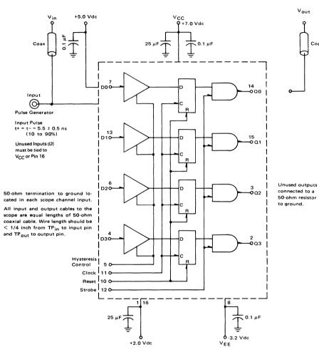
NOTE: All power supplies and logic levels are shifted 2 volts positive .
